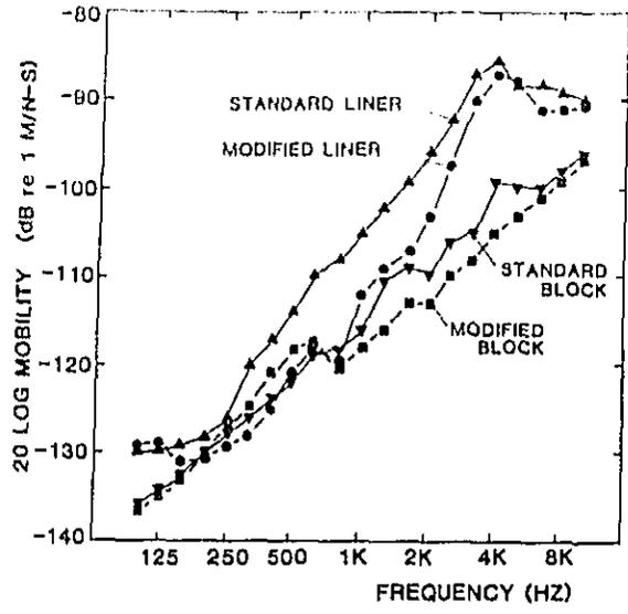
Figure 35. A Comparison of the Measured Vibration Response of the Cylinder Liner and Block for the Standard and Modified Liner Designs in the 6V-92TTA Engine
