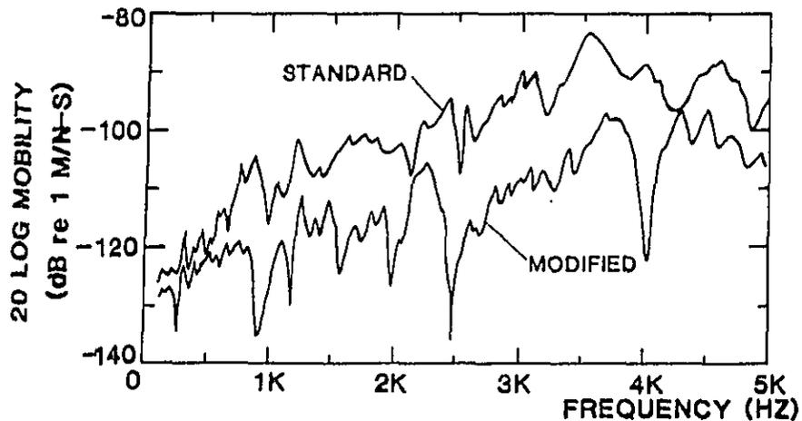
c) Vibration Response of Engine Block at Point of Liner Attachment
