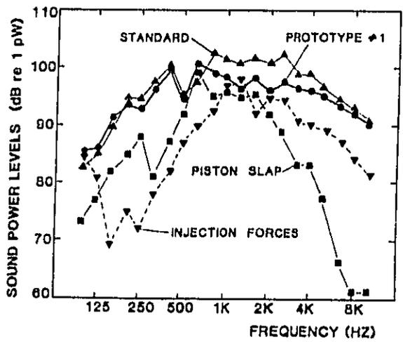
Figure 33. A Comparison of the Measured Sound Power Level of the First Prototype Engine with Those Predicted by the Noise Generation Models and Measured with the Standard 6V-92TTA at 1950 RPM, Full Load
