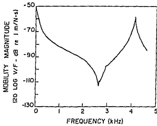
Figure 4. Measured Drive Point Mobility of Piston Top
