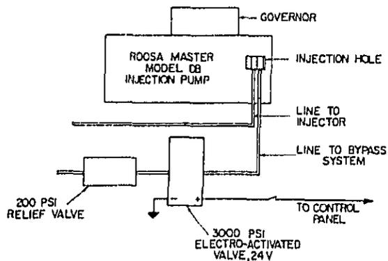
Figure 23. Schematic of Injection Control Mechanism
