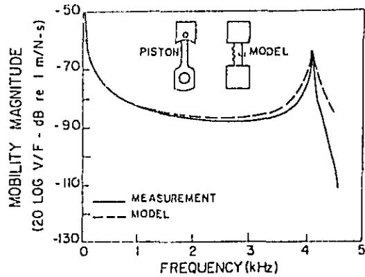
Figure 7. Comparison of Measured and Predicted Transfer Mobility of Piston
