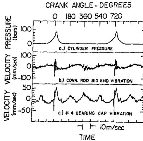
Figure 25. Measurement Signals with Only Cylinders #1 and #4 Firing (1500 RPM, 25% Load)
