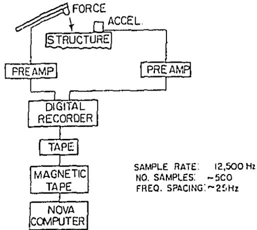
Figure 1. Instrumentation for Mobility Measurements
