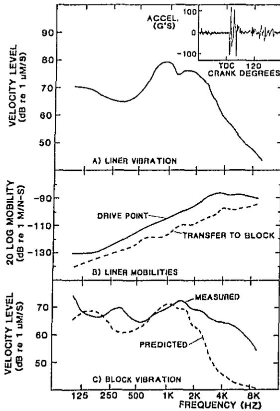
Figure 28. A Summary of Piston Slap Source Model and Block Vibration for the 6V-92TTA Engine at 1950 RPM
