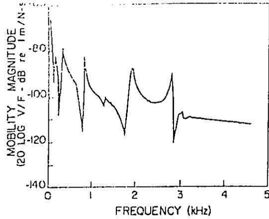
Figure 5. Measured Transfer Mobility of Crankshaft from Pin #2 to Journal #2
