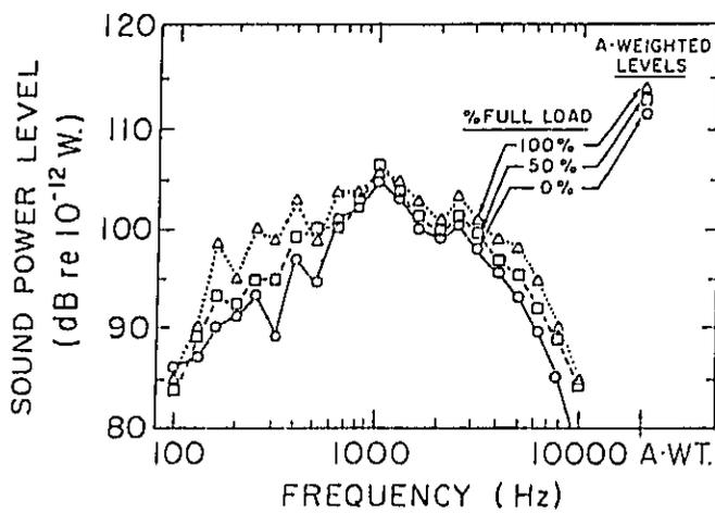
Figure 19. Overall Noise Spectra at 2100 RPM, 3 Load Conditions:
