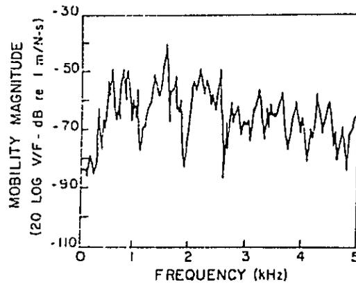
Figure 6. Measured Transfer Mobility of Oil Pan from Flange to Surface Point
