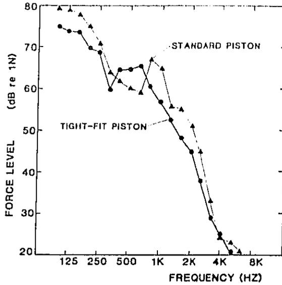
Figure 32. A Comparison of the Estimated Piston Slap Force Spectra for Standard and Tight-Fit Pistons in the 6V-92TTA Engine at 1950 RPM, Full Load
