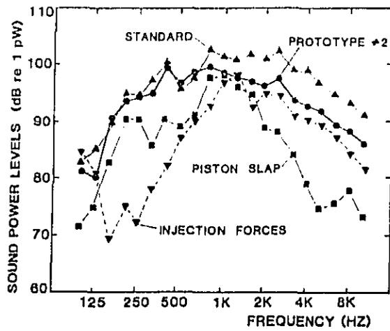
Figure 37. A Comparison of the Measured Sound Power Levels of the Second Prototype Engine with Those Predicted by the Noise Generation Models and Those Measured with the Standard 6V-92TTA Engine at 1950 RPM, Full Load
