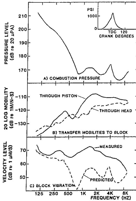
Figure 27. A Summary of the Combustion Source Model and Block Vibration for the 6V-92TTA Engine at 1950 RPM
