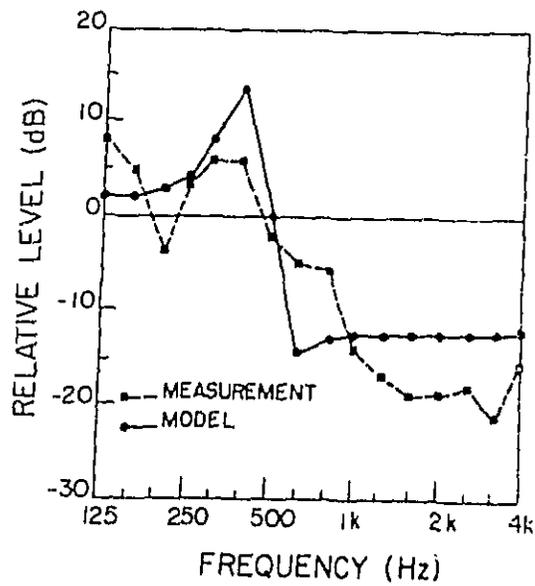
Figure 12. Comparison of Measured and Predicted Change in Vibration Transfer from Piston Top to Block Side Walls
