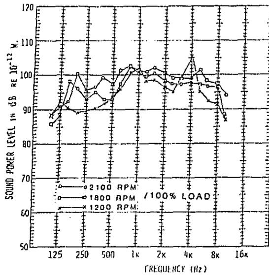
b) NTC-350 Noise Spectra at 100% Load, 3 Speed Conditions
