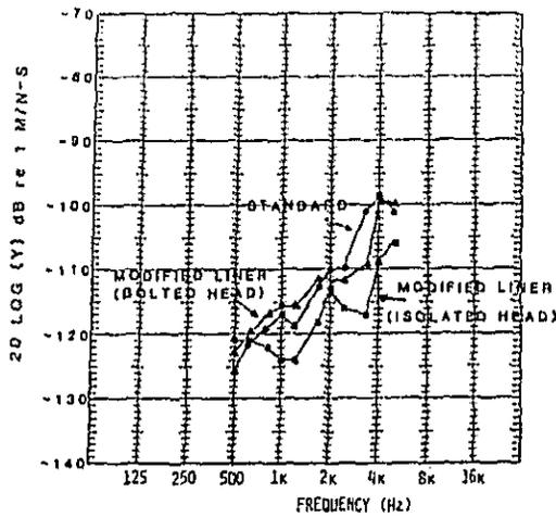
Figure 44. Transfer Mobilities of Piston Slap Force to Block Vibration with New Liner Attachment on NTC-350 Engine
