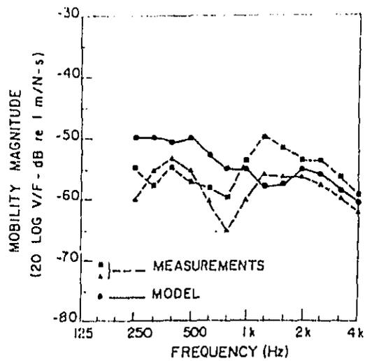
Figure 10. Comparison of Measured and Predicted Transfer Mobility of Oil Pan
