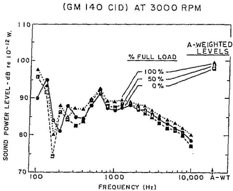
Figure 17. A Comparison of Noise Emission at 3000 RPM, 3 Load Conditions, of Camaro and Vega Engines
