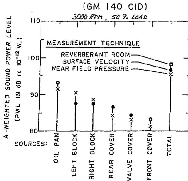
Figure 16. Noise Source Ranking of Vega Engine
