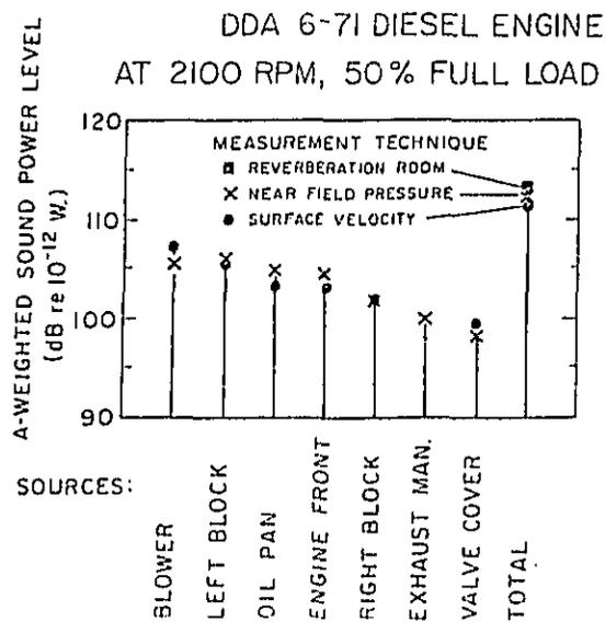
Figure 21. Noise Source Ranking of 6-71 Engine
