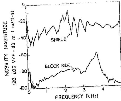
Figure 13. Comparison of Measured Drive Point Mobilities of Engine Block Side and Block Side Shielded with Foam Backing
