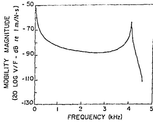
Figure 3. Measured Transfer Mobility of Piston from Top to Big End
