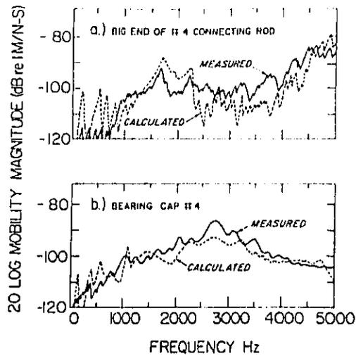
Figure 26. Comparison of Measured and Predicted Transfer Mobilities:
