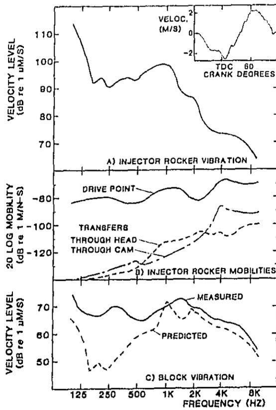
Figure 29. A Summary of the Injector Source Model and Block Vibration for the 6V-92TTA Engine at 1950 RPM
