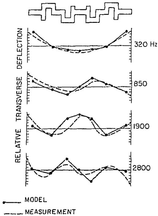
Figure 9. Comparison of Measured and Predicted Mode Shapes of Crankshaft
