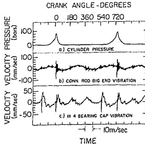
Figure 24. Measurement Signals with All 4 Cylinders Firing (1500 RPM, 25% Load)
