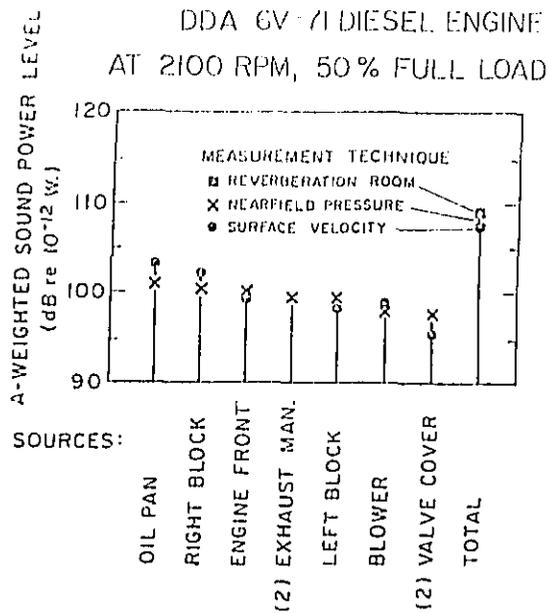
Figure 20. Noise Source Ranking of 6V-71 Engine
