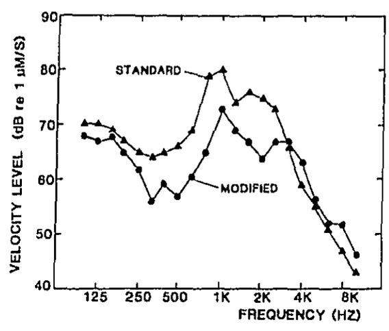
Figure 36. A Comparison of the Measured Cylinder Liner Vibration Levels for the Standard and Modified Liner Designs in the 6V-92TTA Engine at 1950 RPM, Full Load
