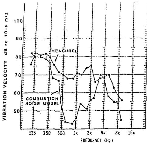
a) Comparison of Vibration Transmission from Combustion with Overall Vibration on NTC-350 Engine at 2100 RPM, Full Load
