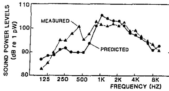
Figure 30. A Comparison of the Measured Sound Power Level with Those Predicted by the Noise Generation Model of the 6V-92TTA Engine at 1950 RPM, Full Load
