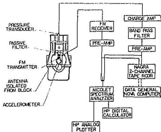
Figure 22. Schematic of Running Engine Data Acquisition System
