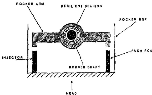
Figure 45. Injector Rocker Isolation Schematic
