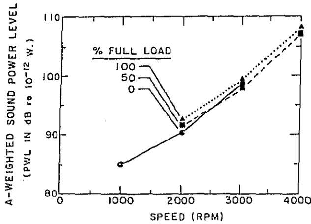
Figure 14. Noise Emission vs. Speed at 3 Load Conditions:
