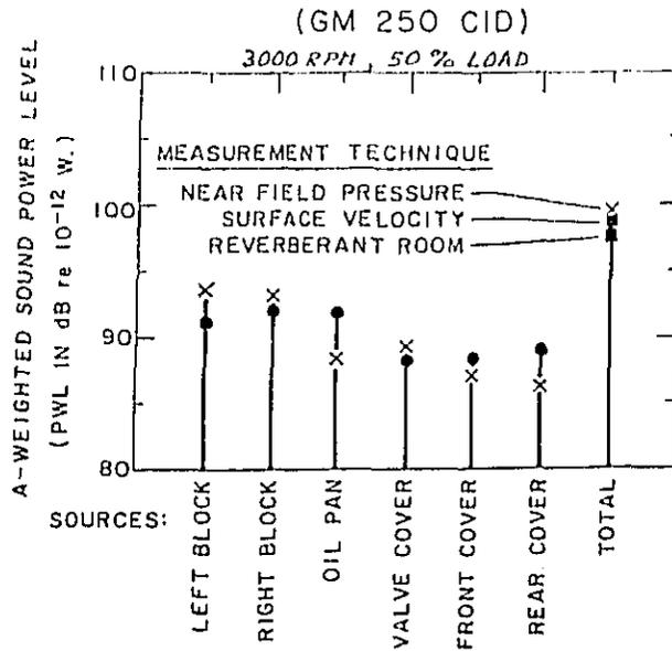
Figure 15. Noise Source Ranking of Camaro Engine
