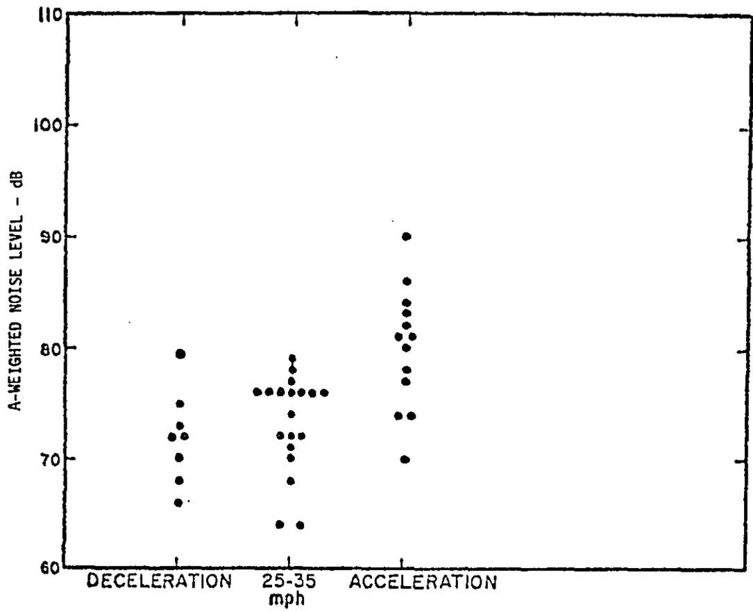
FIGURE G-2 NOISE OF MOTORCYCLES WITH STOCK MUFFLERS
