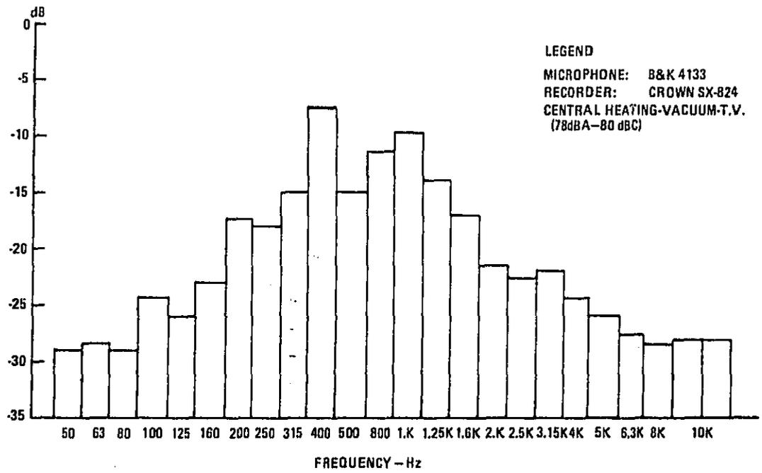
FIGURE 2. 1/3 - OCTAVE BAND SPECTRAL ANALYSIS OF NOISE PROFILE
