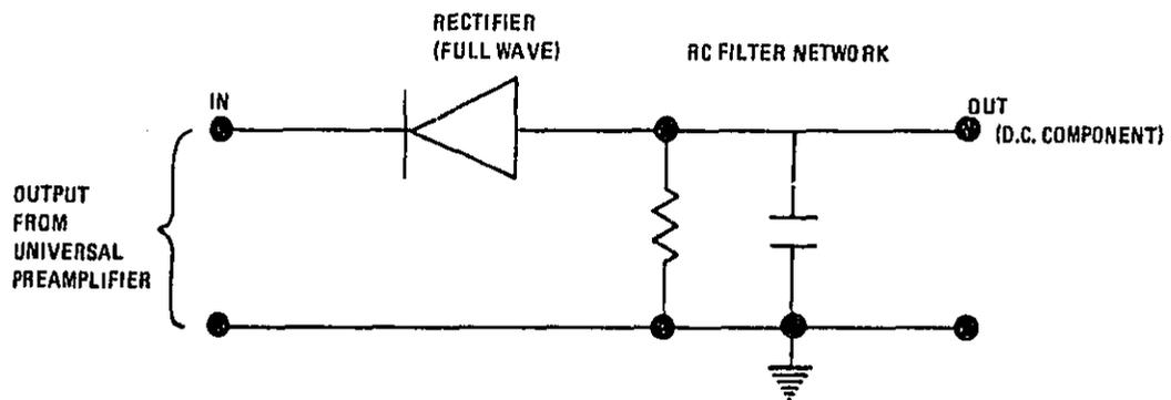
FIGURE 3. SCHEMATIC DIAGRAM OF EMG SIGNAL CONDITIONER CIRCUITRY.
