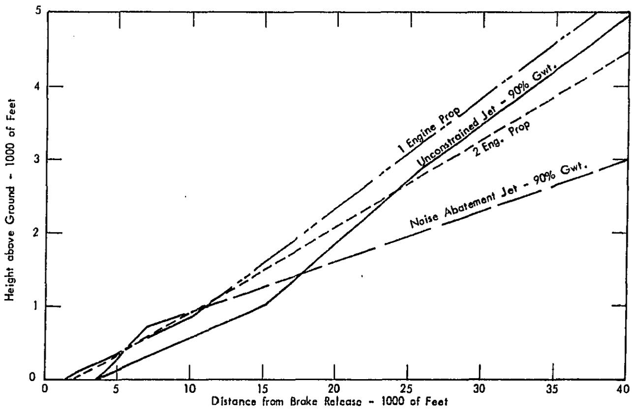
FIGURE 11. TAKEOFF PROFILES FOR COMPOSITE AIRPLANES
