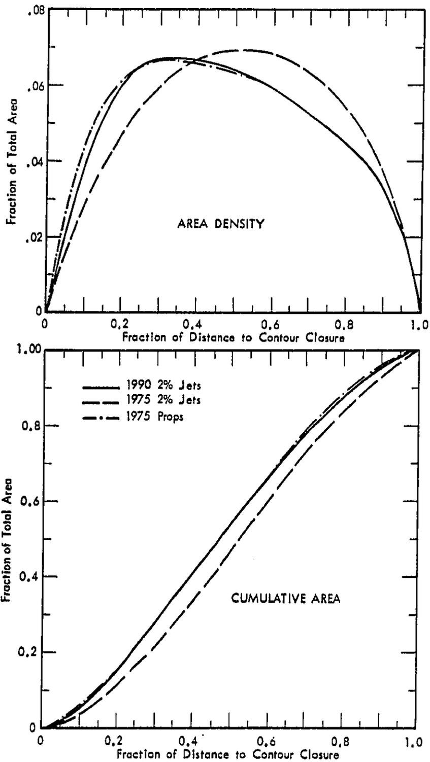
FIGURE 33. GENERALIZED SOUND EXPOSURE LEVEL AREA FUNCTIONS - TAKEOFF
