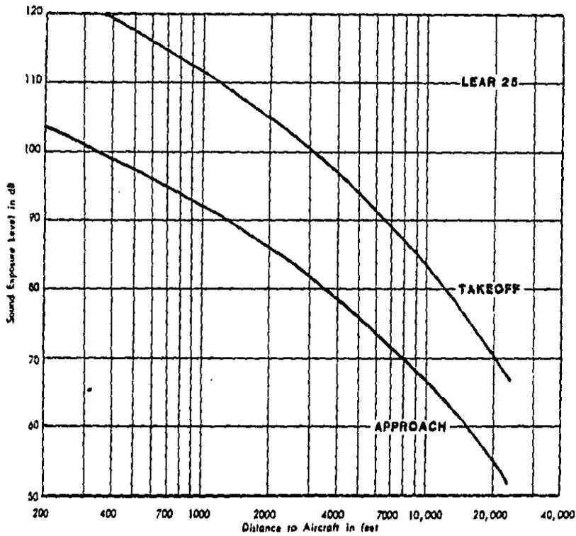
FIGURE 5. SOUND EXPOSURE LEVEL AS A FUNCTION OF DISTANCE - LEAR 25
