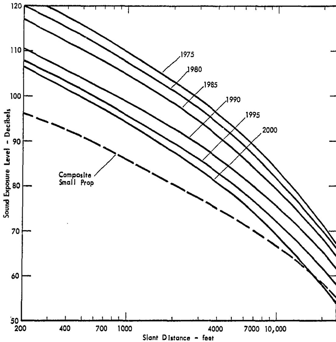
FIGURE 17. SOUND EXPOSURE LEVELS AS A FUNCTION OF SLANT DISTANCE - COMPOSITE BUSINESS JETS FOR YEARS 1975 TO 2000 - TAKEOFF THRUST AND SMALL PROPELLER - DRIVEN AIRPLANES AT TAKEOFF POWER
