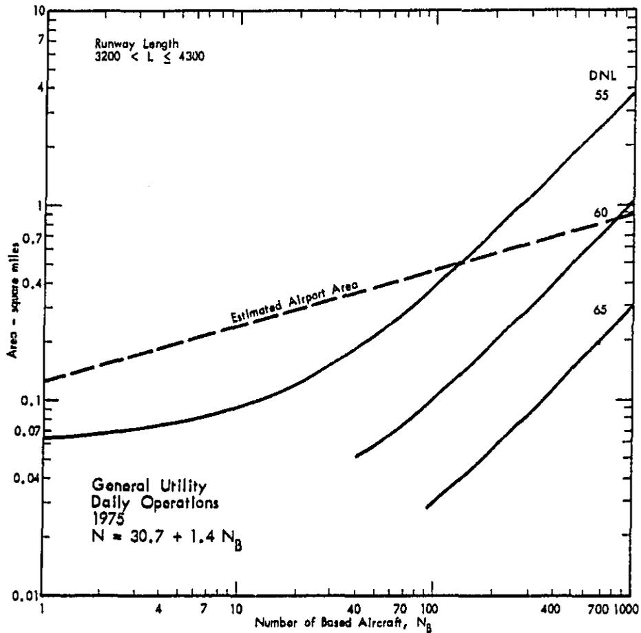
FIGURE 29. AREA ENCLOSED WITHIN VARIOUS CONTOURS OF DAY-NIGHT AVERAGE SOUND LEVEL AS A FUNCTION OF THE NUMBER OF AIRPLANES BASED AT A GENERAL UTILITY AIRPORT
