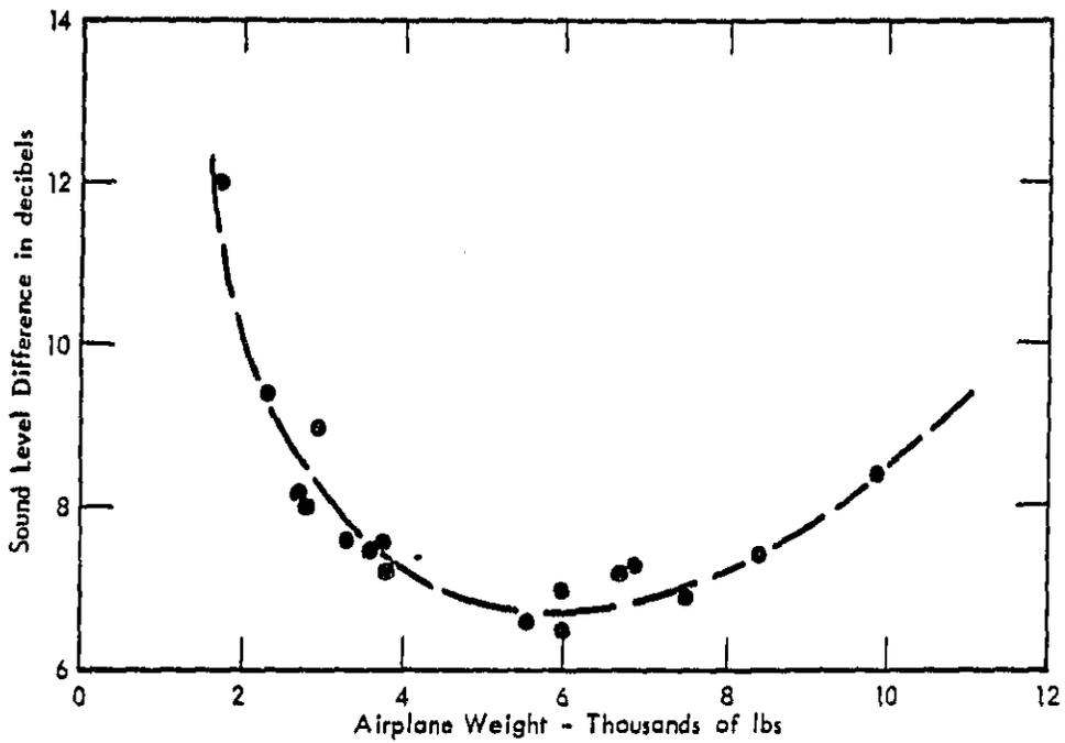
FIGURE 13. DIFFERENCE BETWEEN EPNL AND MAXIMUM A-WEIGHTED SOUND LEVEL FOR PROPELLER-DRIVEN SMALL AIRPLANES UNDER APPENDIX F TESTS
