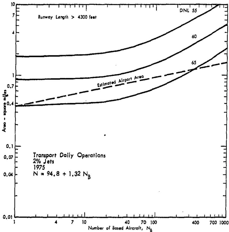
FIGURE 30. AREA ENCLOSED WITHIN VARIOUS CONTOURS OF DAY-NIGHT AVERAGE SOUND LEVEL AS A FUNCTION OF THE NUMBER OF AIRPLANES BASED AT A TRANSPORT AIRPORT
