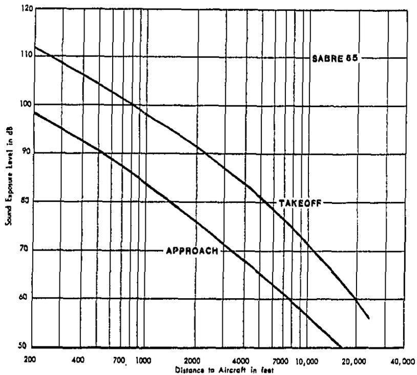
FIGURE 8. SOUND EXPOSURE LEVEL AS A FUNCTION OF DISTANCE - SABRE 65
