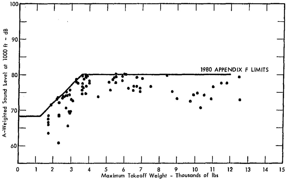
FIGURE 15. MAXIMUM A-WEIGHTED SOUND LEVELS FOR 1980 AIRPLANES - APPENDIX F TESTS
