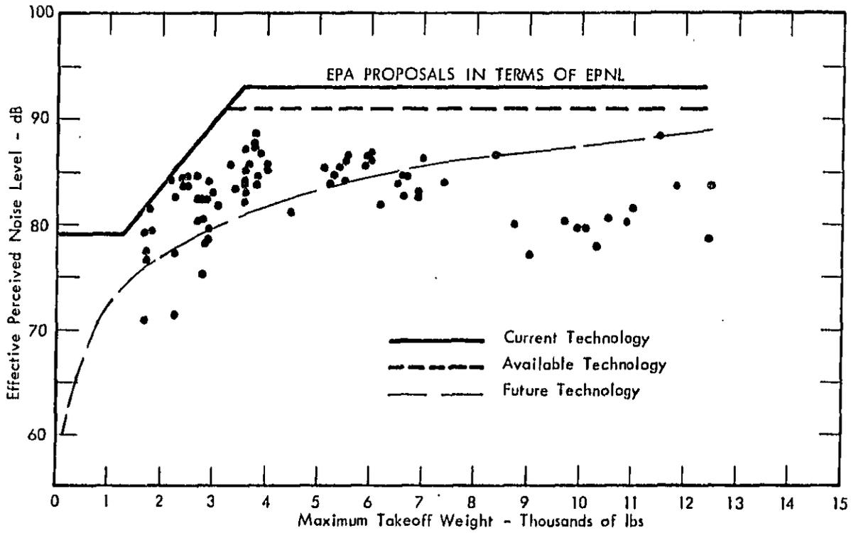
FIGURE 16. EFFECTIVE PERCEIVED NOISE LEVELS FOR 1980 AIRPLANES UNDER APPENDIX F TEST CONDITIONS
