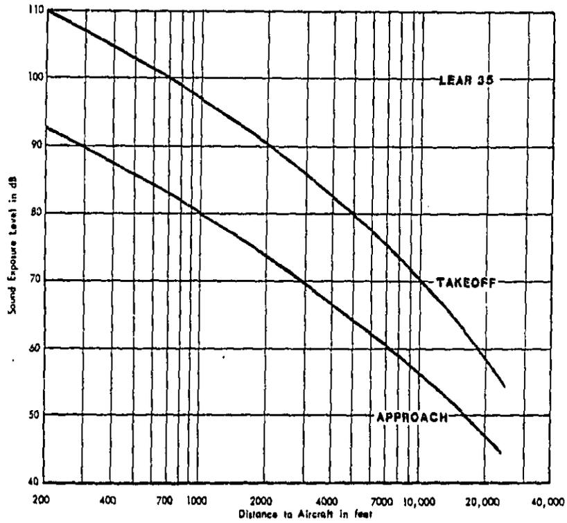
FIGURE 6. SOUND EXPOSURE LEVEL AS A FUNCTION OF DISTANCE - LEAR 35
