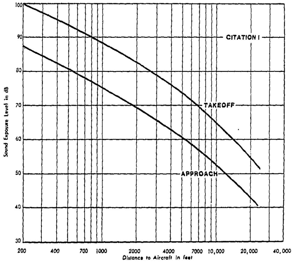
FIGURE 3. SOUND EXPOSURE LEVEL AS A FUNCTION OF DISTANCE - CITATION I
