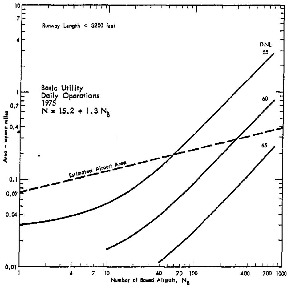
FIGURE 28. AREA ENCLOSED WITHIN VARIOUS CONTOURS OF DAY-NIGHT AVERAGE SOUND LEVEL AS A FUNCTION OF THE NUMBER OF AIRPLANES BASED AT A BASIC UTILITY AIRPORT
