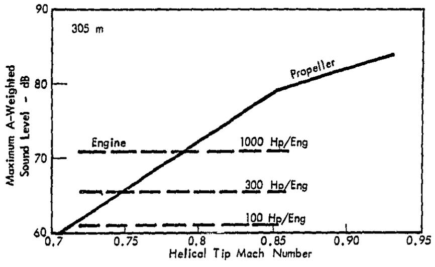
FIGURE 12. COMPARISON OF PROPELLER AND ENGINE NOISE - NORMALLY ASPIRATED RECIPROCATING ENGINE
