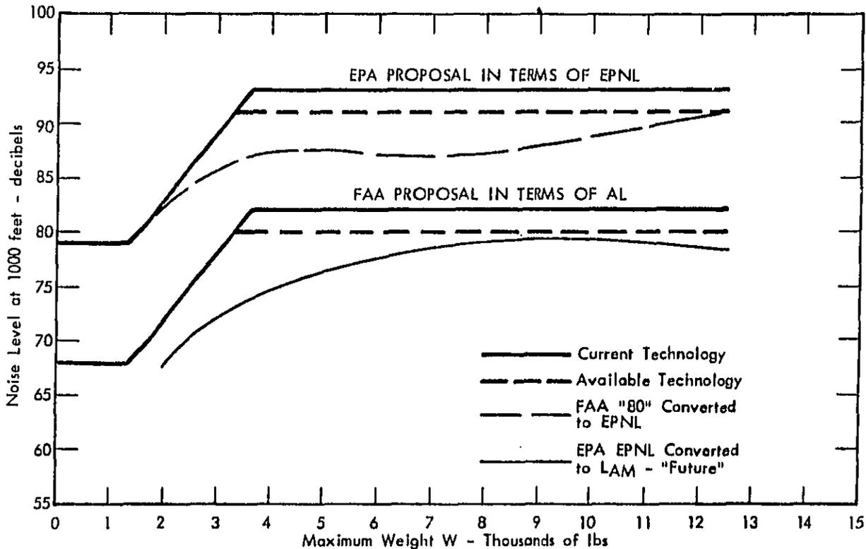
FIGURE 14. NOISE COMPLIANCE LEVELS IN TERMS OF EFFECTIVE PERCEIVED NOISE LEVEL (EPNL) AND A-WEIGHTED LEVEL (AL)
