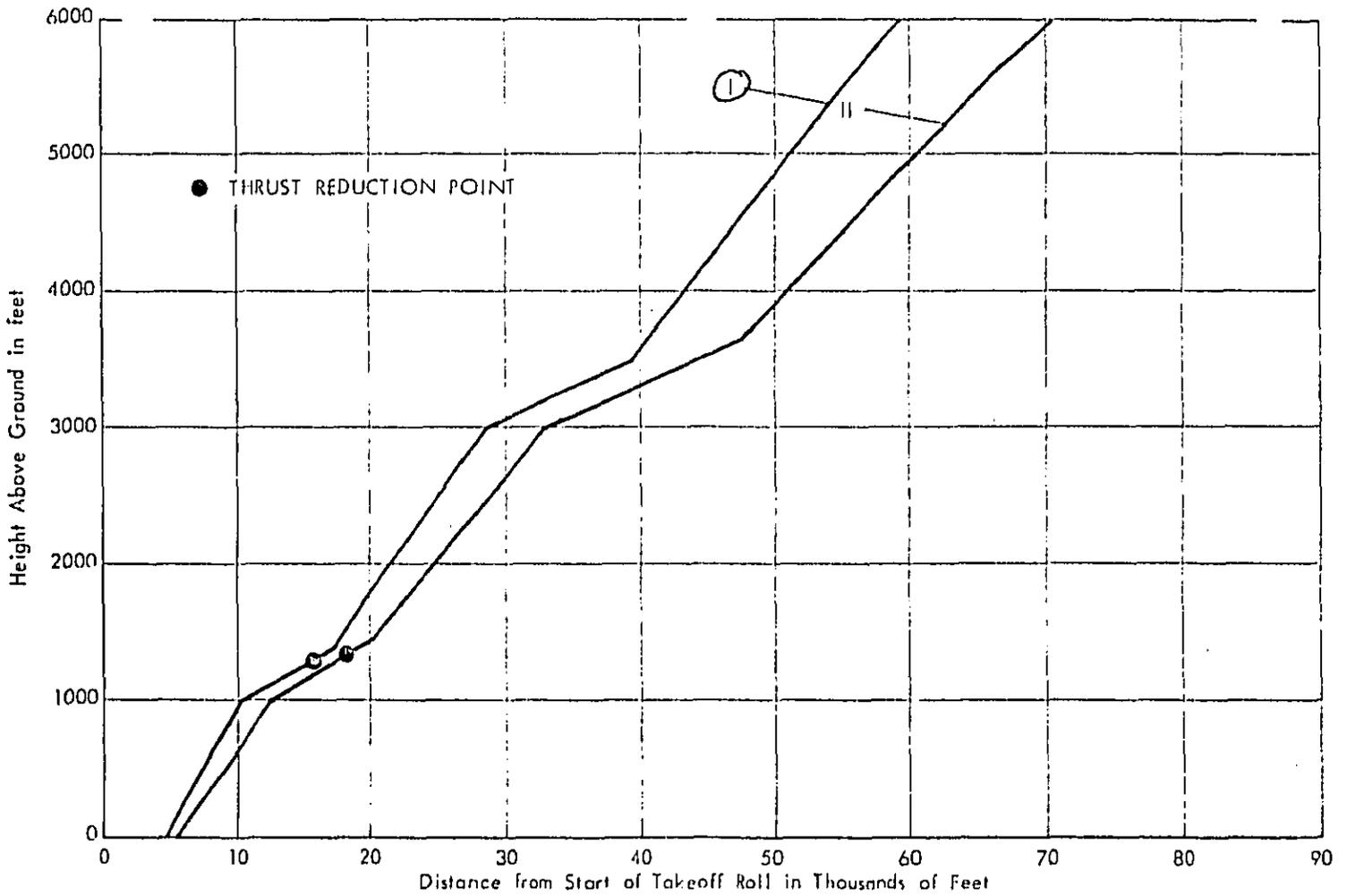
FIGURE A-11.ATA TAKEOFF PROFILES FOR 2-ENGINE LBPR TURBOFAN TRANSPORT AIRCRAFT - DC-9, 737 SERIES (2-T-TFL) - REVISED PROCEDURES ADOPTED DECEMBER 1976
