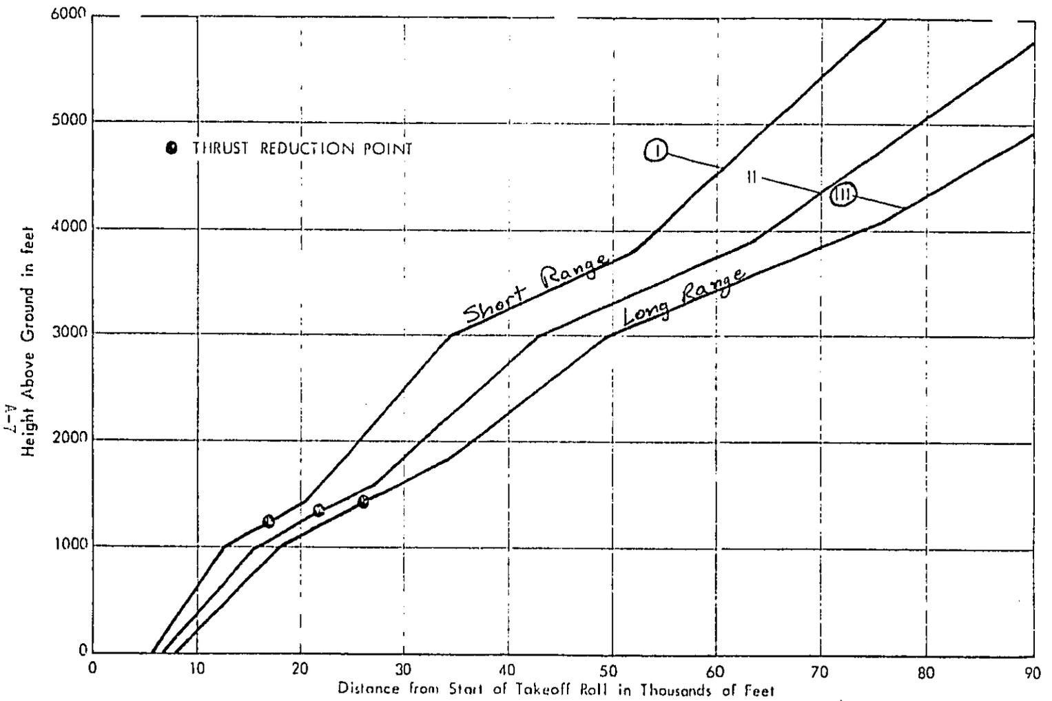
FIGURE A-6. ATA TAKEOFF PROFILES FOR 3-ENGINE HBPR TURBOFAN TRANSPORT - DC-10, L-1011 SERIES (3-T-TFH) - REVISED PROCEDURES ADOPTED DECEMBER 1976
