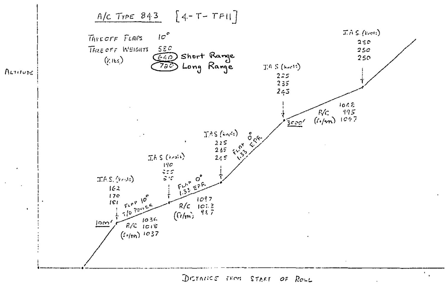
FIGURE A-1. TAKEOFF CHARACTERISTICS FOR 4-ENGINE HBPR TURBOFAN
