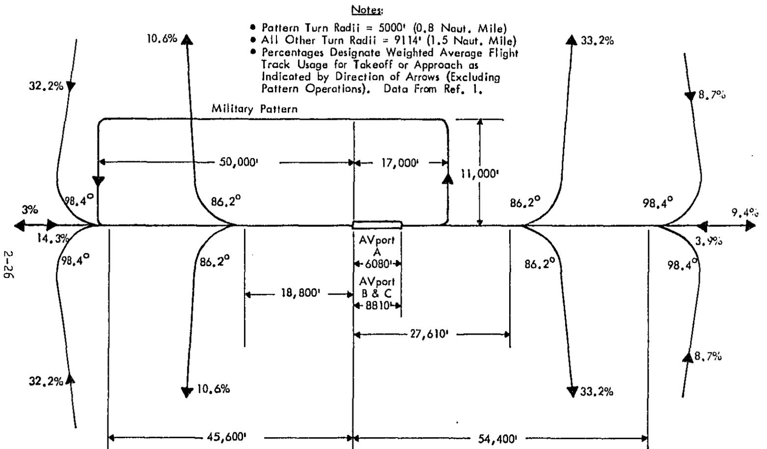
FIGURE 2-1. MILITARY AND AIR CARRIER FLIGHT TRACKS FOR AVPORTS A, B, AND C
