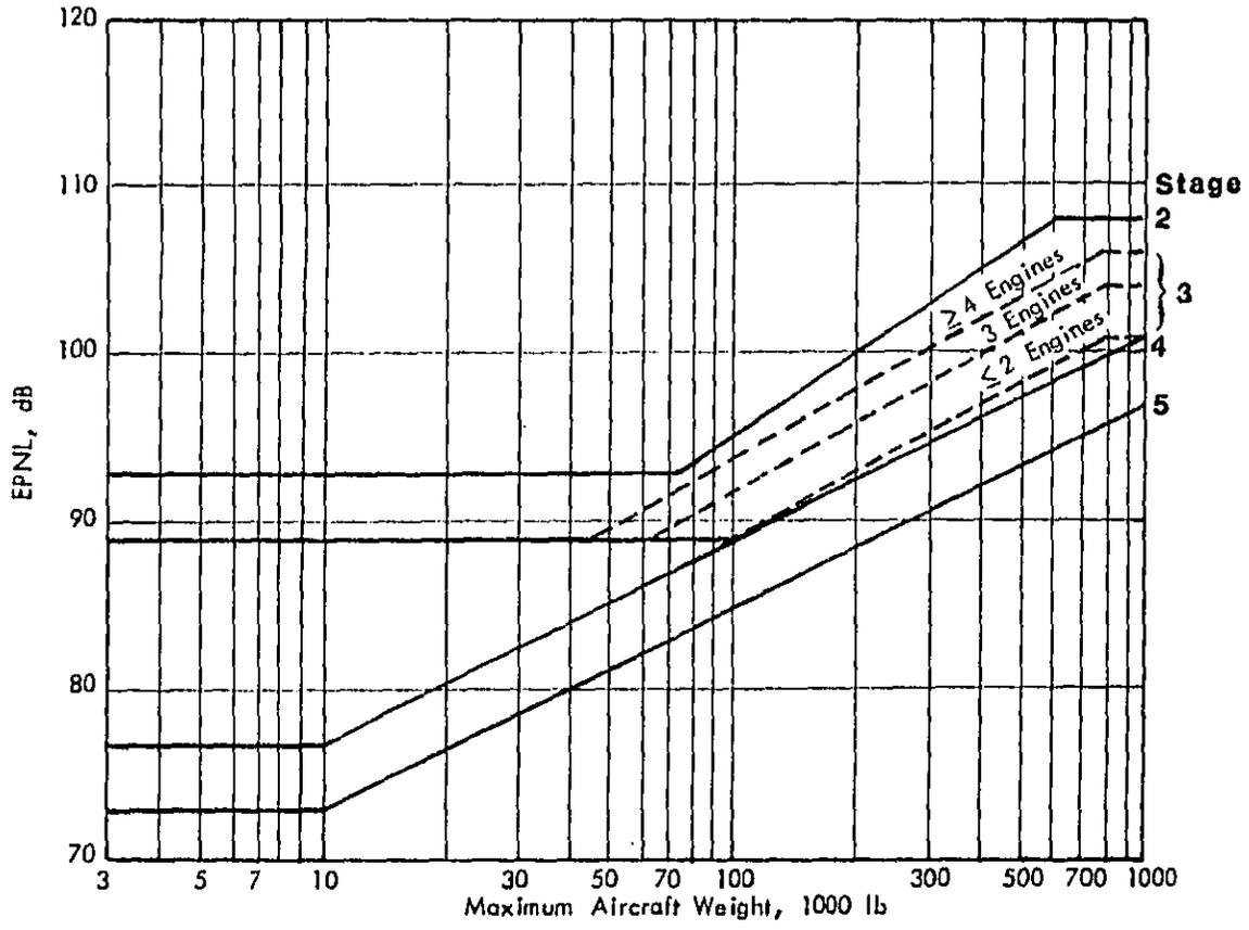
FIGURE 3-1. TAKEOFF NOISE LIMITS FOR STAGES 2-5
