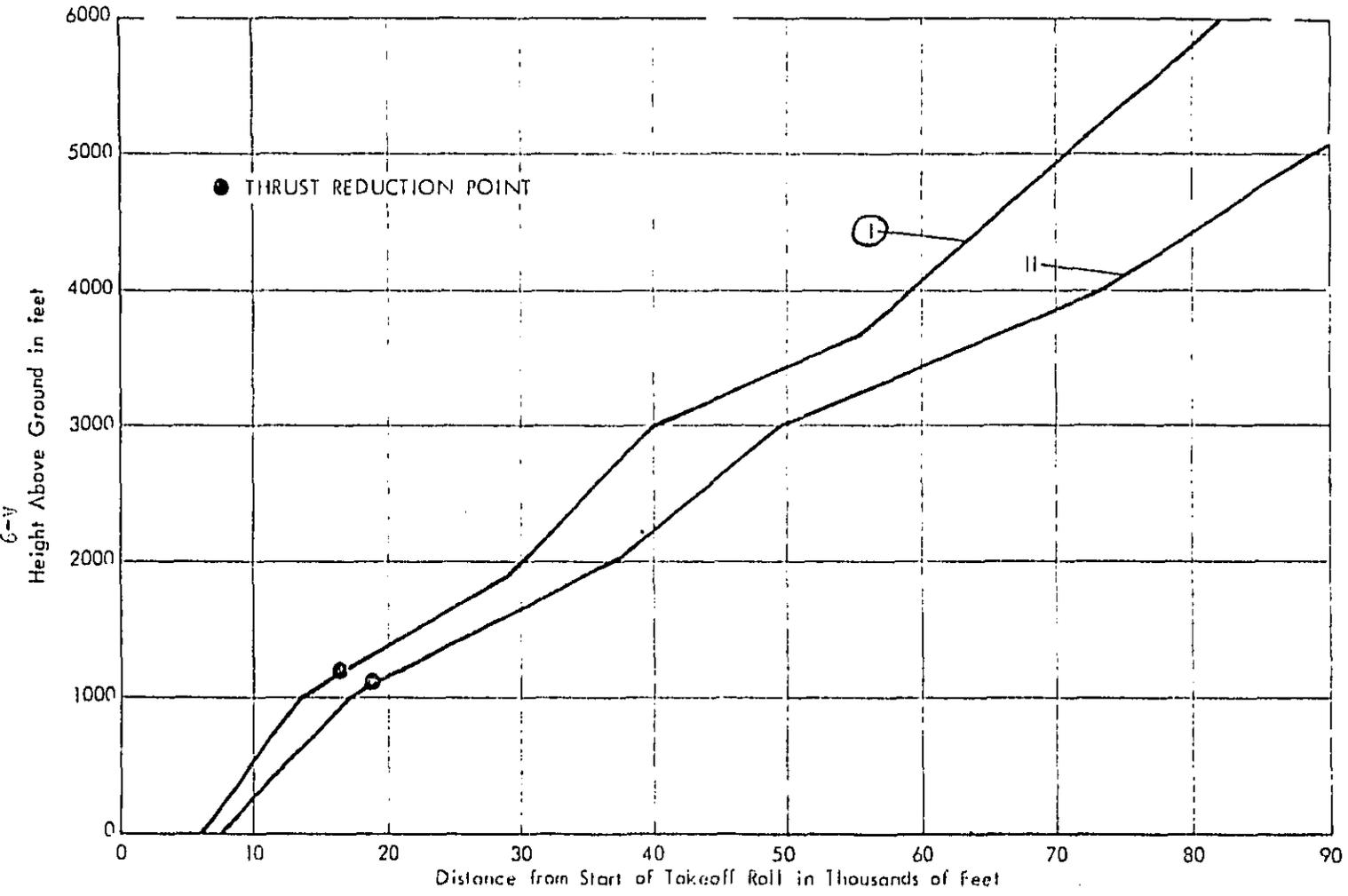
FIGURE A-8. ATA TAKEOFF PROFILES FOR 3-ENGINE LBPR TURBOFAN TRANSPORT AIRCRAFT - 727 SERIES (3-T-TFL) - REVISED PROCEDURES ADOPTED DECEMBER 1976
