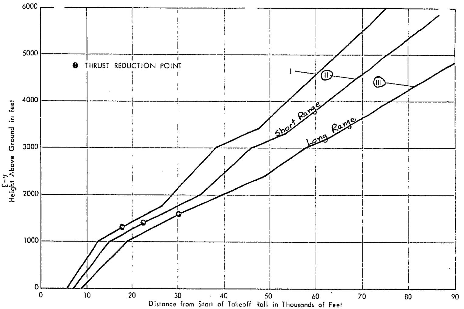
FIGURE A-2. ATA TAKEOFF PROFILES FOR 4-ENGINE HBPR TURBOFAN TRANSPORT AIRCRAFT - 747 SERIES (4-T-TFH) - REVISED PROCEDURES ADOPTED DECEMBER 1976
