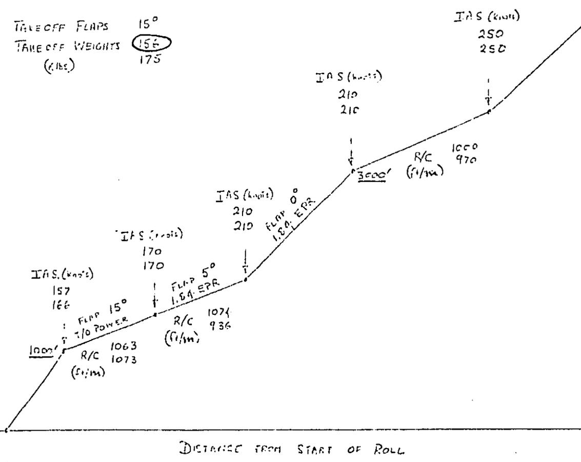
FIGURE A-7. TAKEOFF CHARACTERISTICS FOR 3-ENGINE LBPR TURBOFAN
