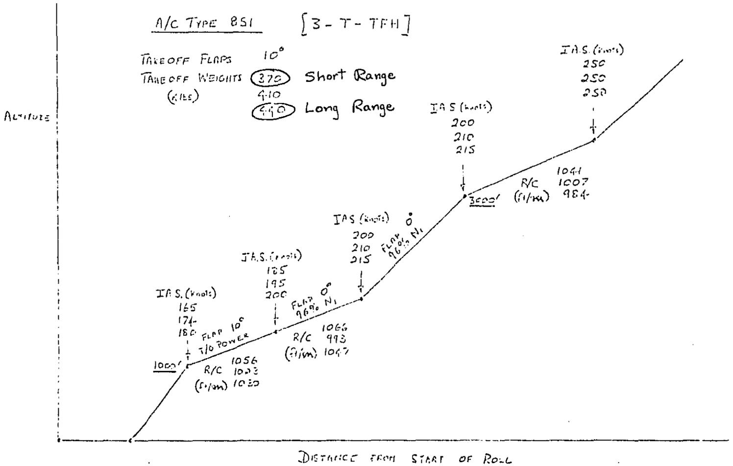
FIGURE A-5. TAKEOFF CHARACTERISTICS FOR 3-ENGINE HBPR TURBOFAN
