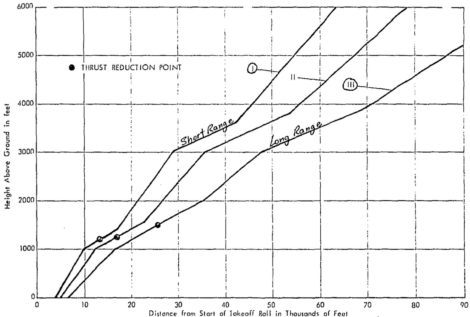
FIGURE A-4. ATA TAKEOFF PROFILES FOR 4-ENGINE LBPR TURBOFAN TRANSPORT AIRCRAFT - DC-8, 707 SERIES (4-T-TFL) - REVISED PROCEDURES ADOPTED DECEMBER 1976
