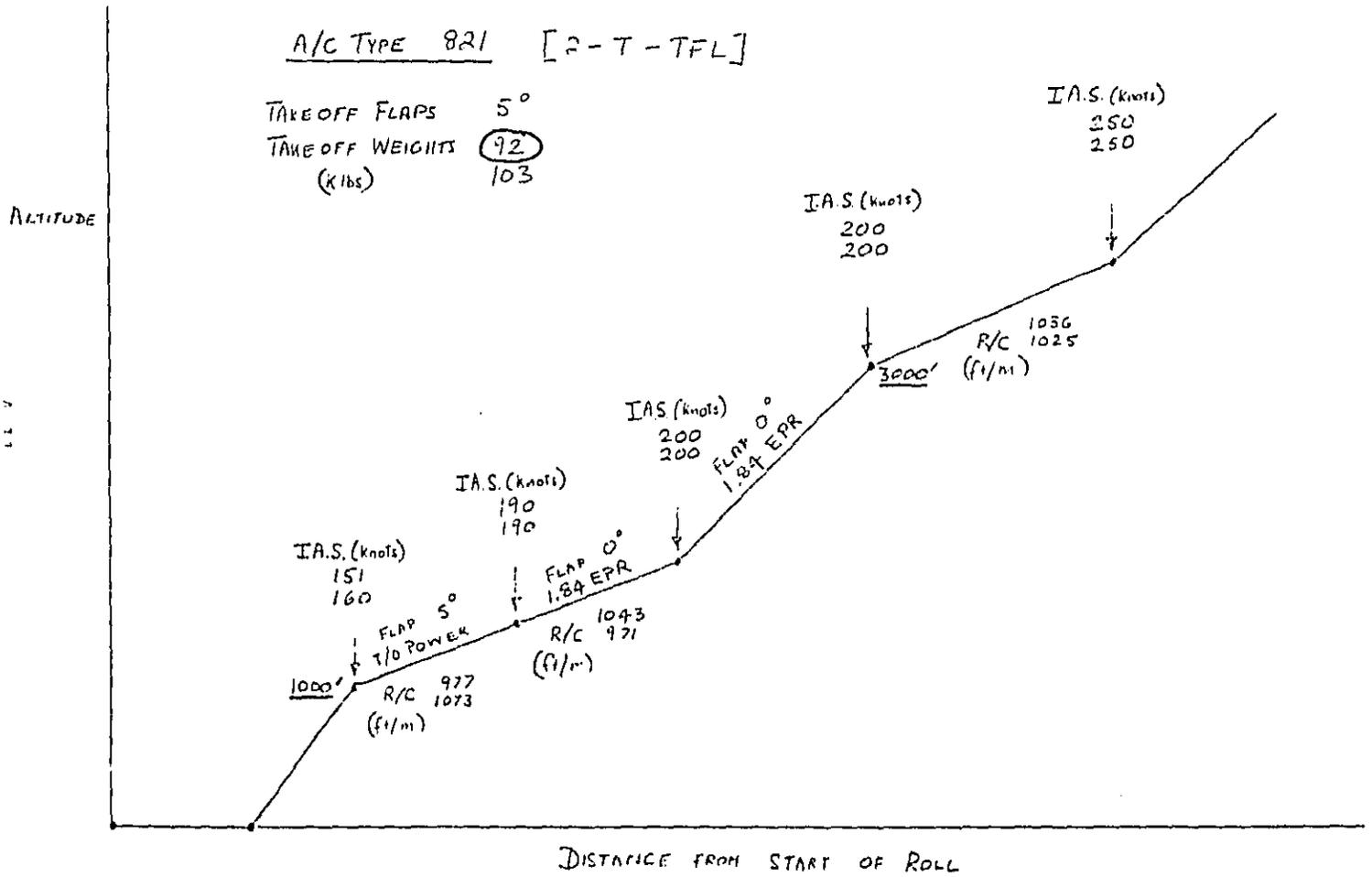
FIGURE A-10. TAKEOFF CHARACTERISTICS FOR 2-ENGINE LBPR TURBOFAN
