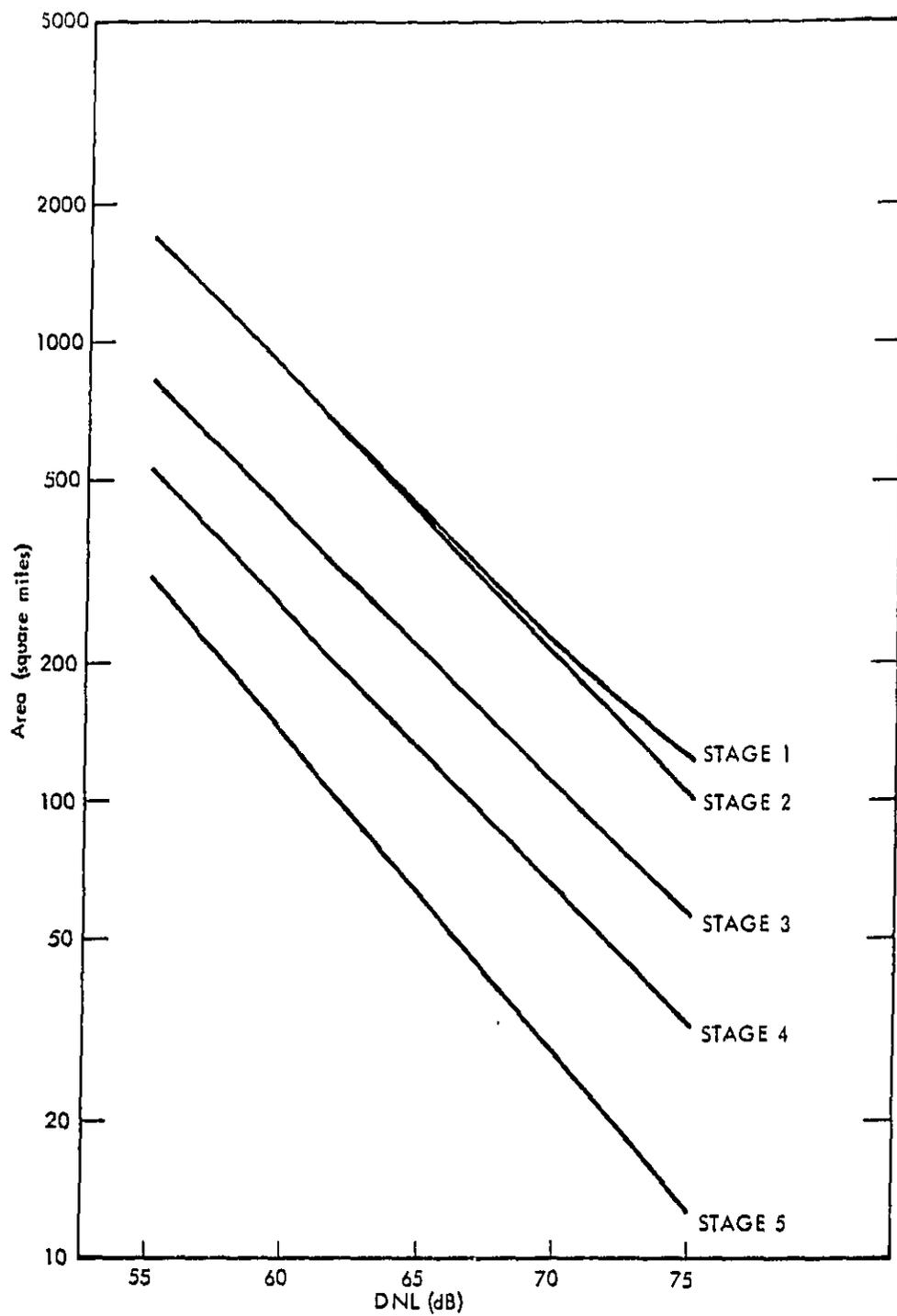
FIGURE 4-3. IMPACTED AREA AS A FUNCTION OF DNL AND REGULATORY STAGE FOR CIVIL OPERATIONS AT JOINT USE AIRPORTS
