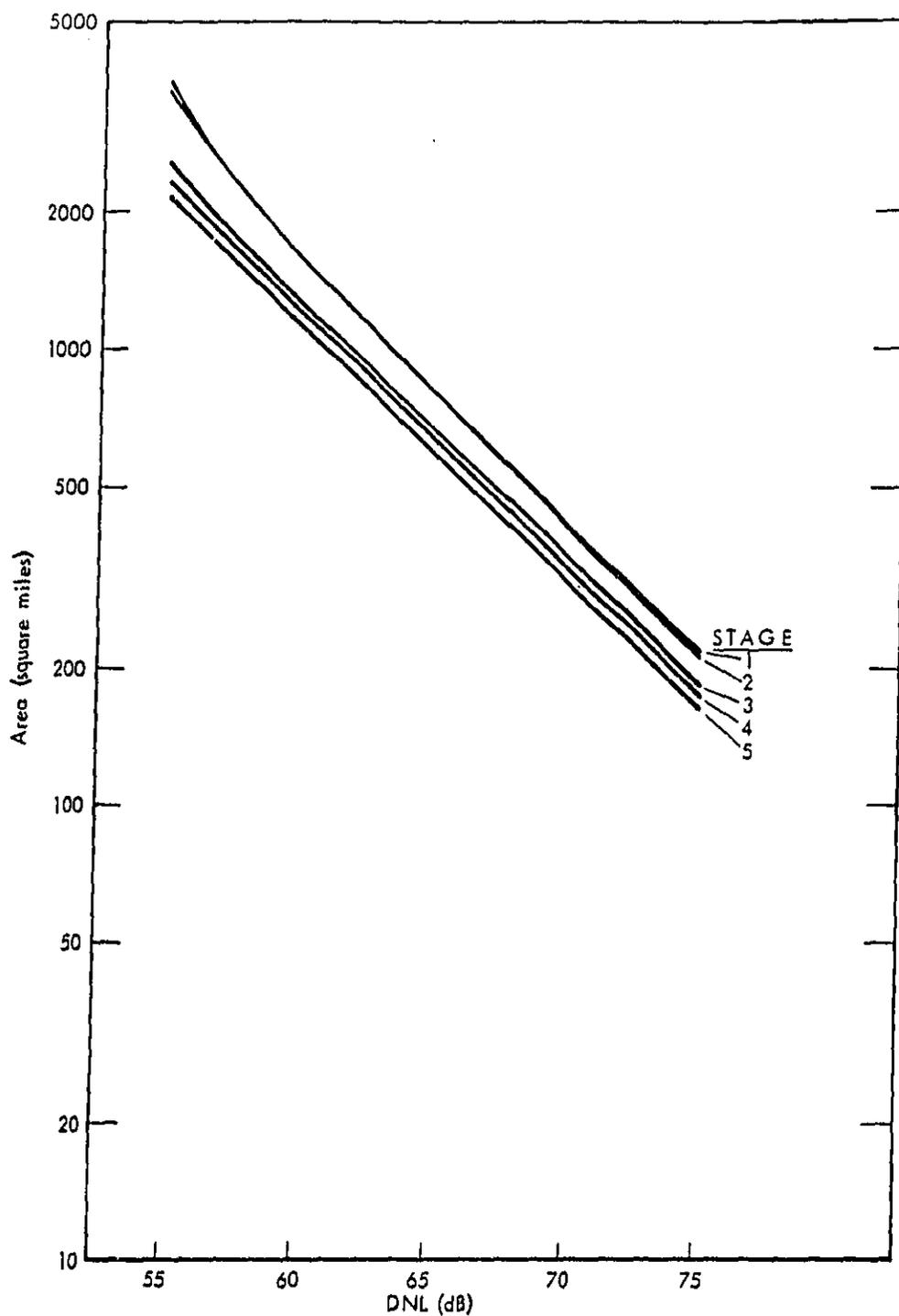
FIGURE 4-4. IMPACTED AREA AS A FUNCTION OF DNL AND REGULATORY STAGE FOR CIVIL AND MILITARY OPERATIONS AT JOINT USE AIRPORTS
