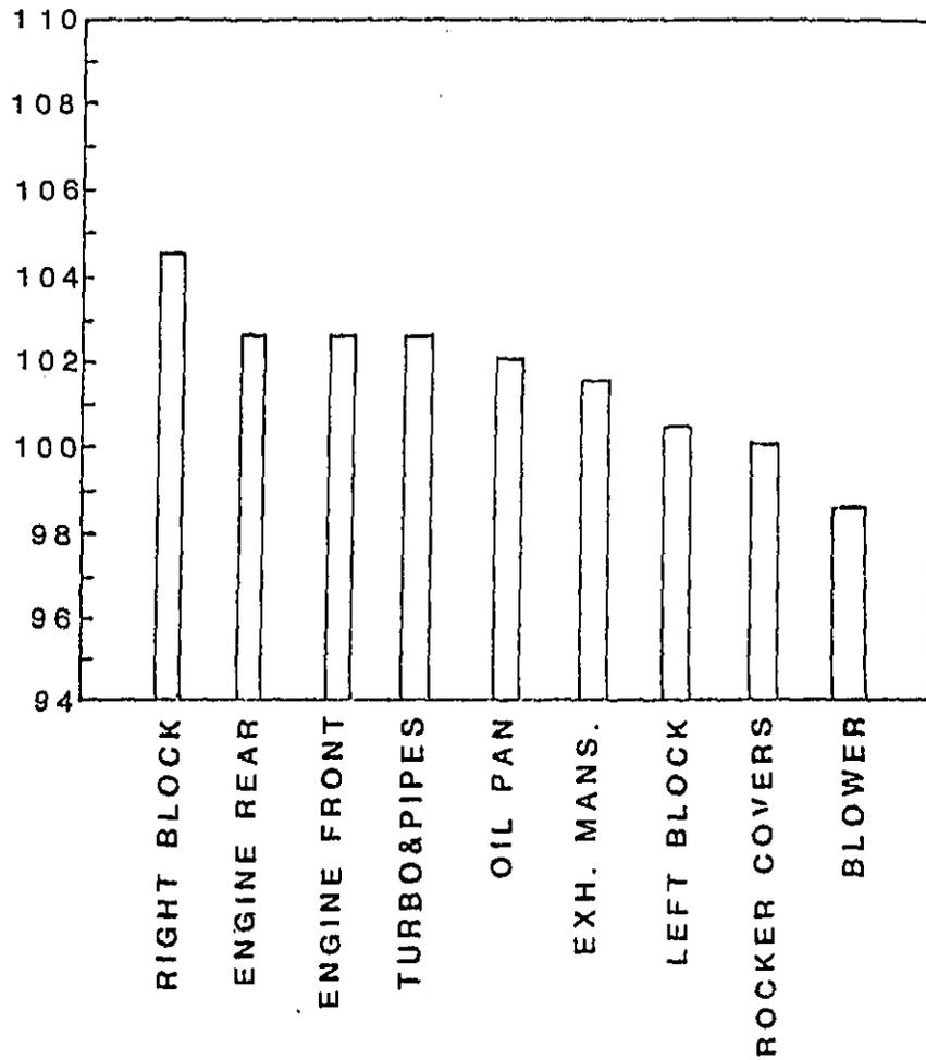
Figure 8. Source Identification of DDA 6V-92TTA Engine at 1950 RPM, Full Load
