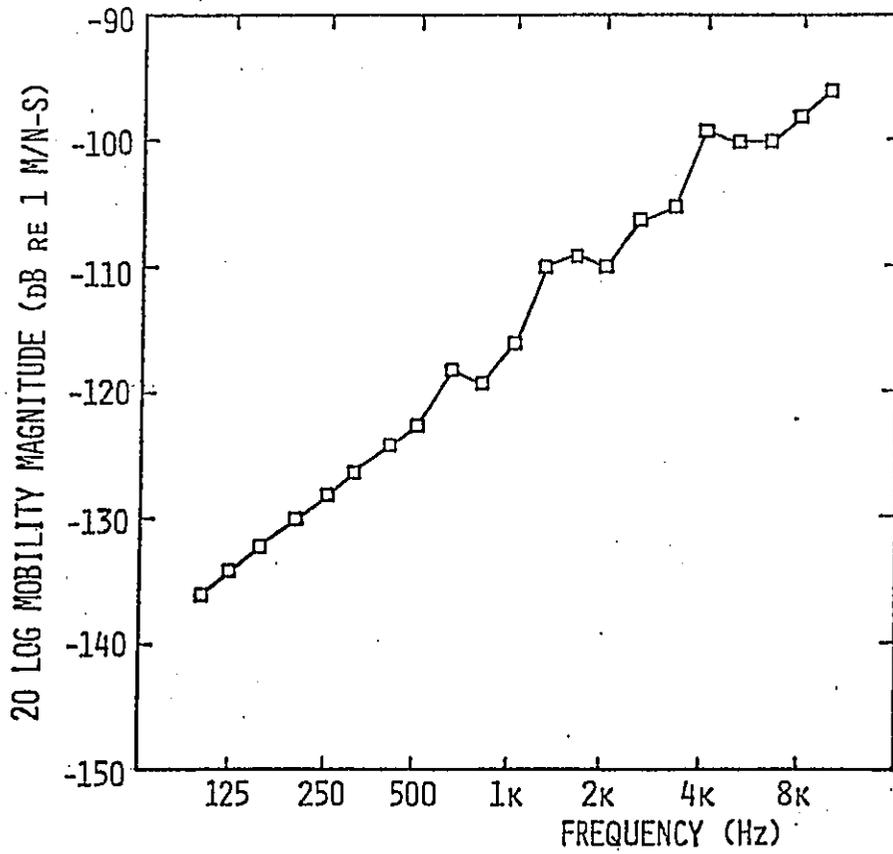
Figure 16. Transfer Mobility of Piston-Slap Force to Block Vibration on DDA 6V-92TTA Engine
