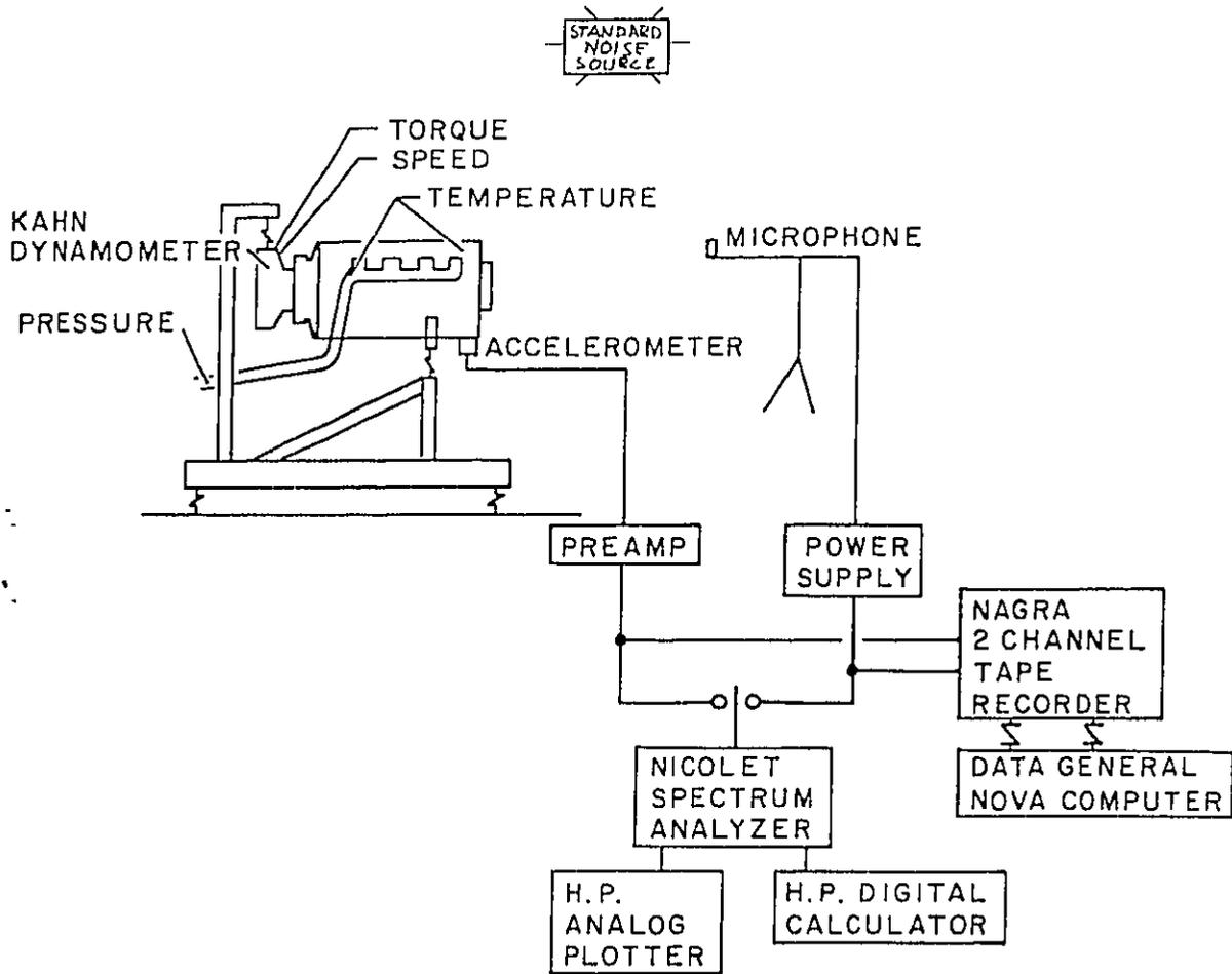
Figure 2. Instrumentation Set-Up
