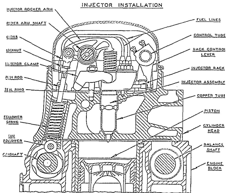
Figure 27. DDA 6V-92TTA Unit Injector Mechanisms
