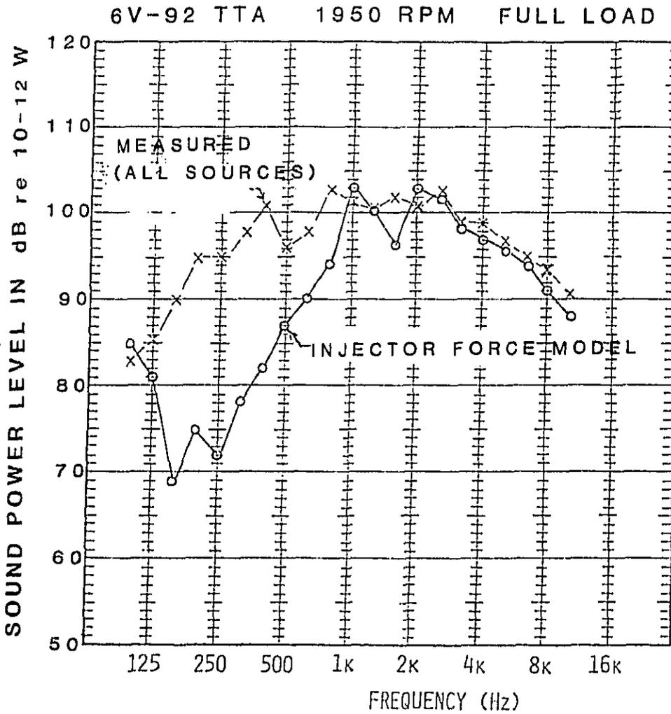
Figure 28. Overall Radiated Noise Levels in DDA 6V-92TTA Engine vs. Injector Force Model
