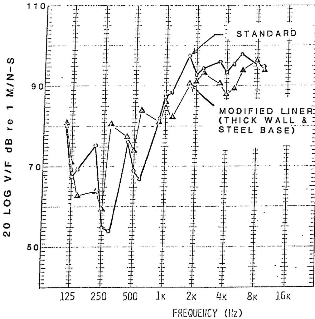
Figure 32. Measured Transfer Mobility: TDC Cylinder Liner to Block Side
