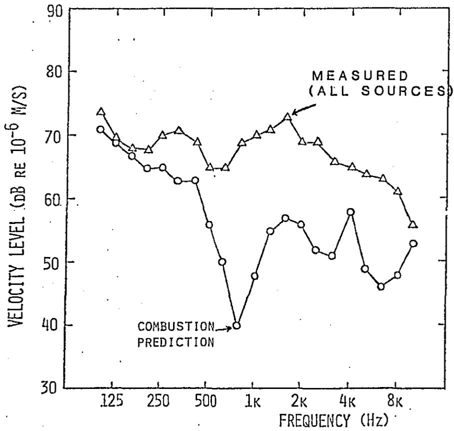
Figure 12. Average Vibration Levels of Engine Block on DDA 6V-92TTA Engine at 1950 RPM, Full Load
