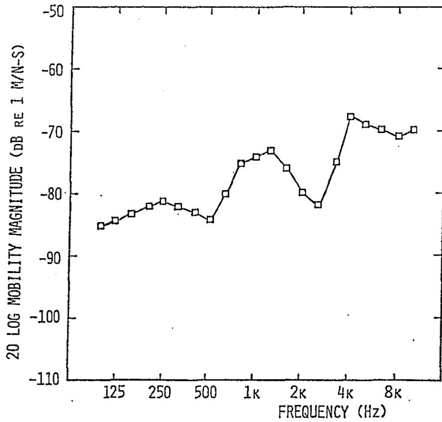
Figure 19. Mobility of Injector on DDA 6V-92TTA Engine
