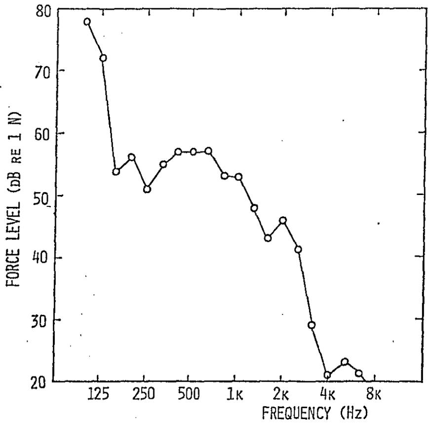
Figure 20. Estimated Injector Force Levels in DDA 6V-92TTA Engine at 1950 RPM, Full Load
