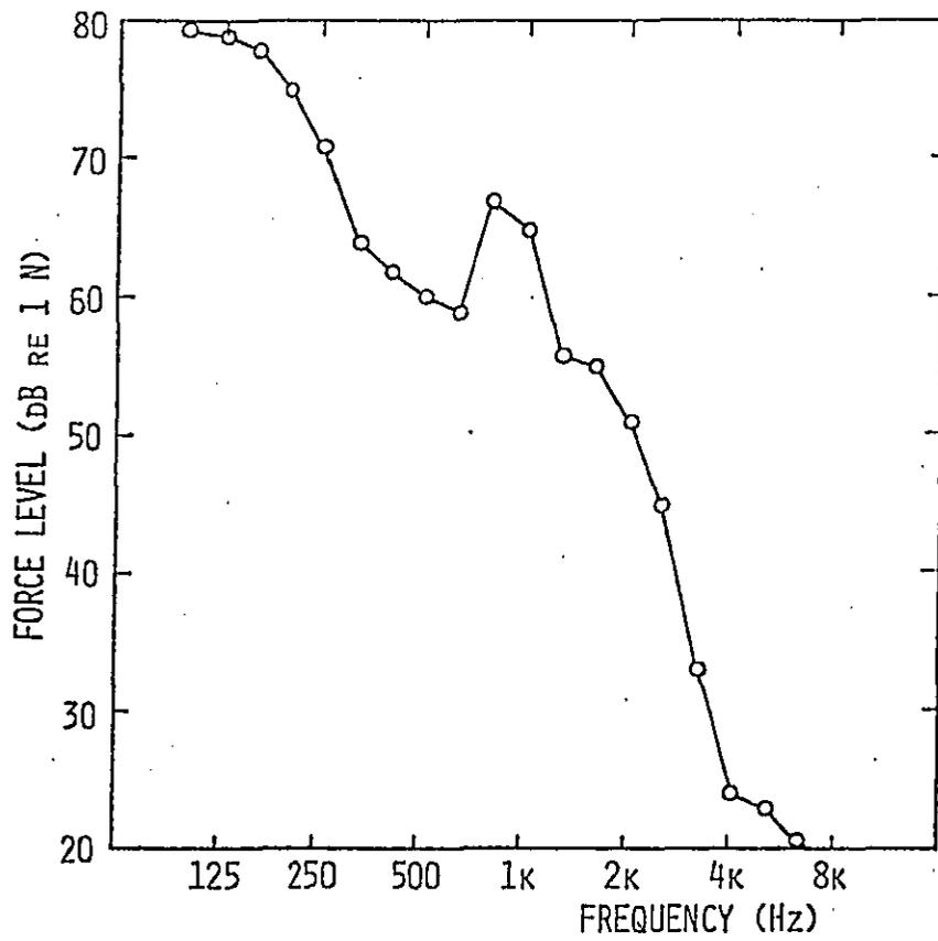
Figure 15. Estimated Force of Piston-Slap in DDA 6V-92TTA Engine at 1950 RPM, Full Load
