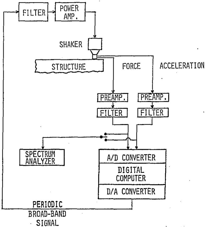
Figure 10. Instrumentation for Mobility Measurements
