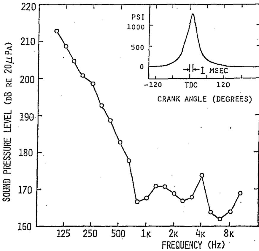
Figure 9. Cylinder Pressure of DDA 6V-92TTA Engine at 1950 RPM, Full Load
