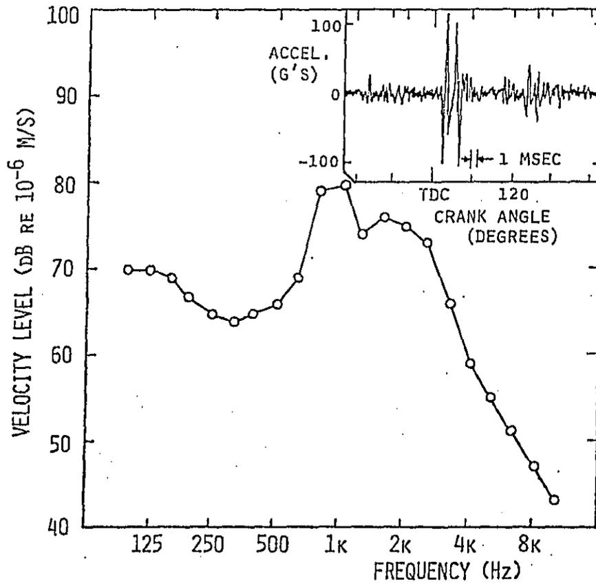
Figure 13. Cylinder Liner Vibration of DDA 6V-92TTA Engine at 1950 RPM, Full Load
