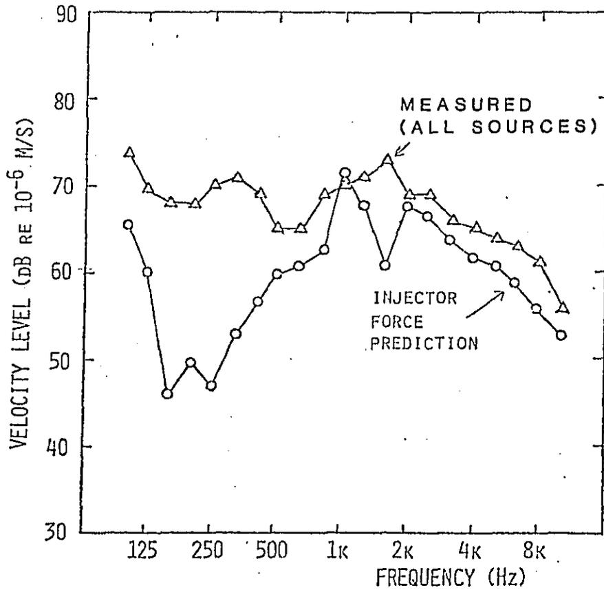
Figure 22. Average Vibration Levels of Engine Block on DDA 6V-92PTA Engine at 1950 RPM, Full Load
