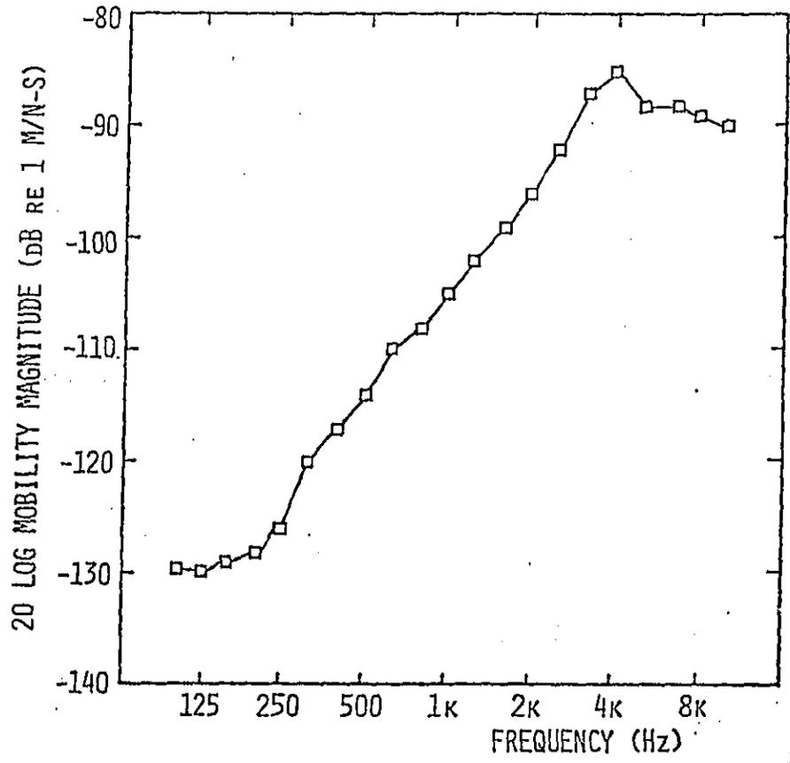
Figure 14. Drive-Point Mobility of Cylinder Liner on DDA 6V-92TTA Engine
