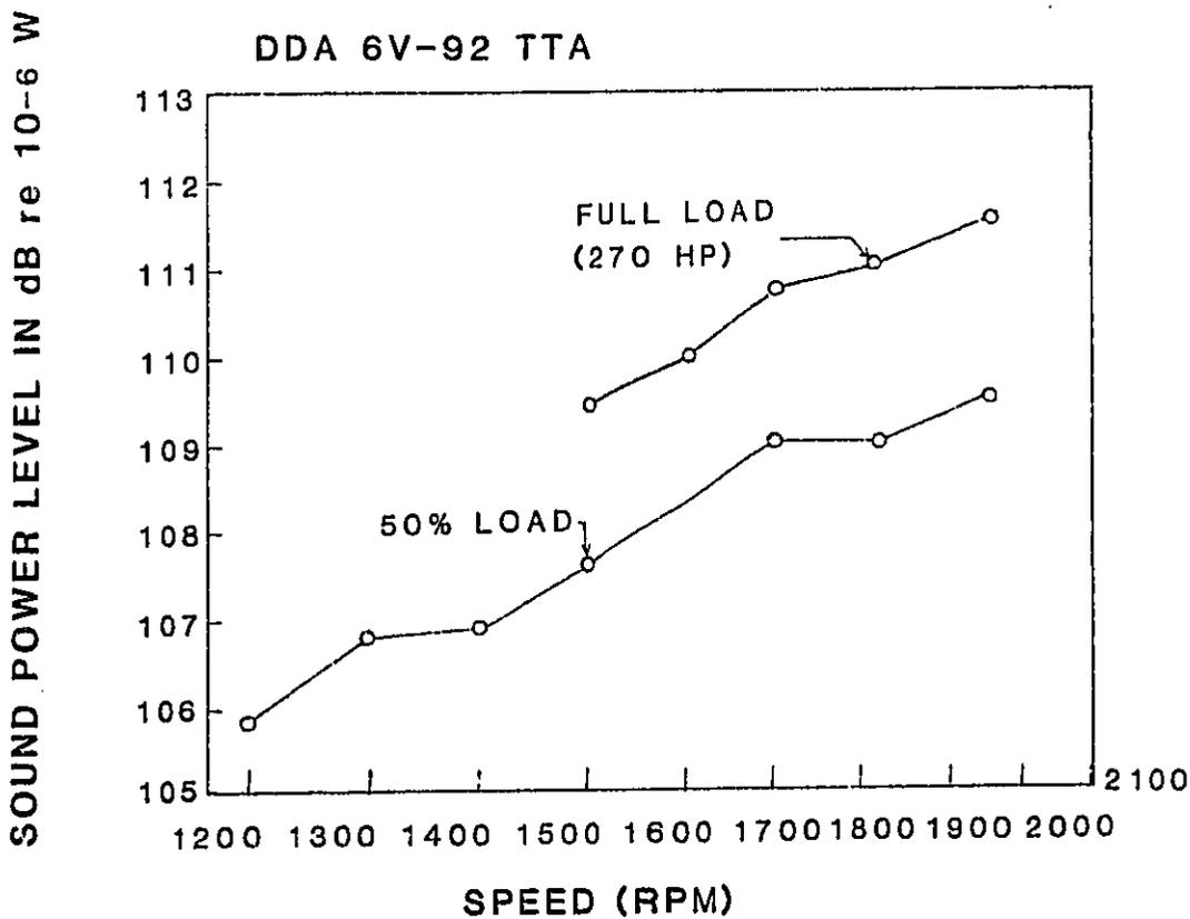
Figure 5. Noise Emissions vs. Engine Speed at Two Load Conditions
