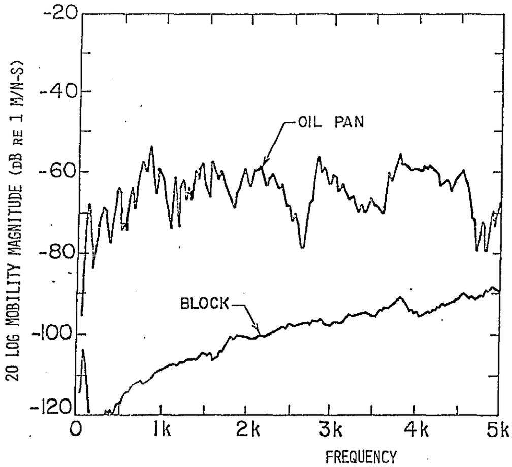
Figure 23. Measured Mobilities of Oil Pan and Block Connection on DDA 6V-92TTA Engine
