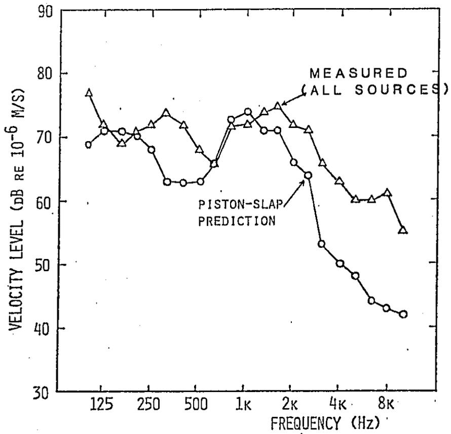
Figure 17. Average Vibration Levels of Right Engine Block on DDA 6V-92TTA Engine at 1950 RPM, Full Load
