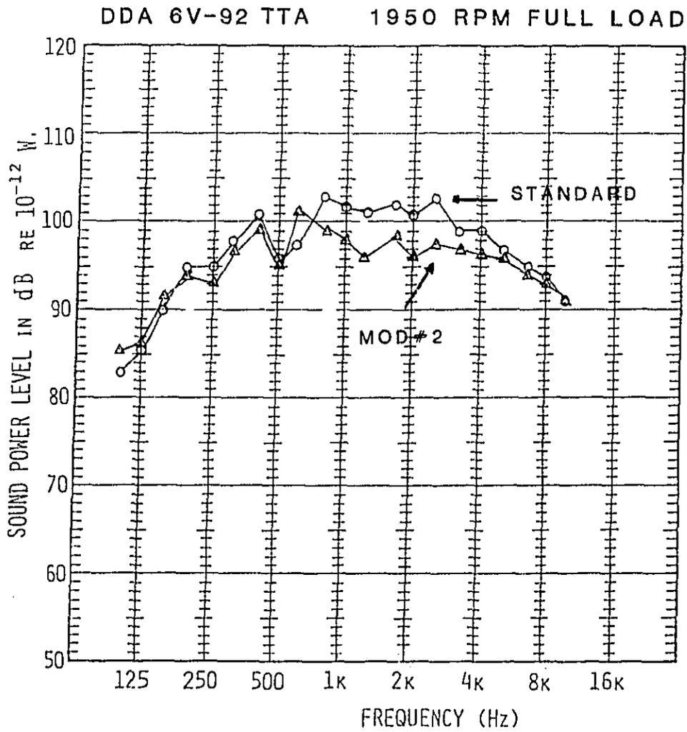
Figure 33. Overall Noise Radiation of Demonstration Engine #1 vs. Standard DDA 6V-92TTA Engine
