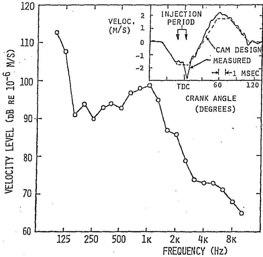
Figure 18. Vibration of Injector Plunger in DDA 6V-92TTA Engine at 1950 RPM, Full Load
