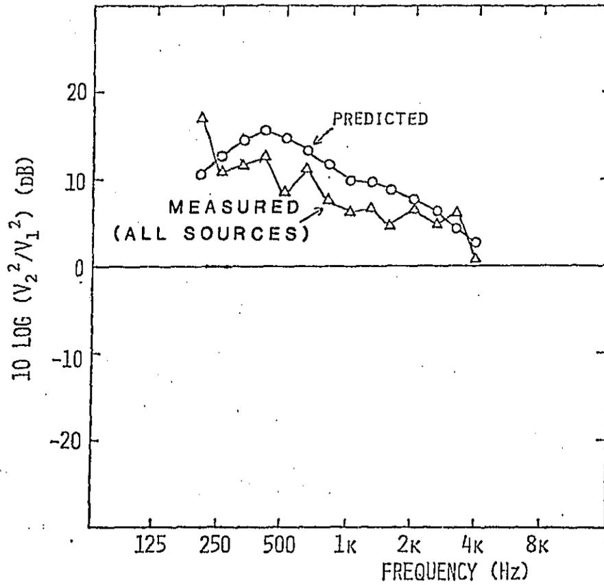
Figure 24. Average Velocity Ratio of Oil Pan to Block on DDA 6V-92TTA Engine
