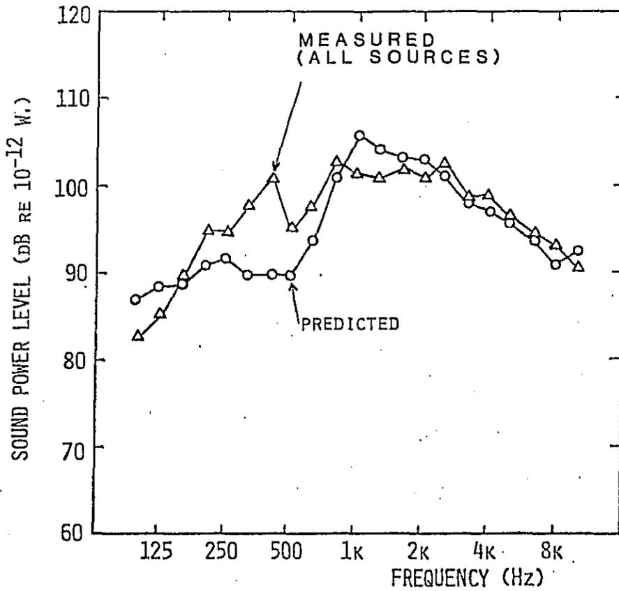
Figure 26. Sound Power Levels of DDA 6V-92TTA Engine at 1950 RPM, Full Load
