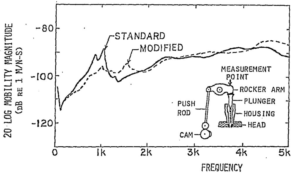
Figure 29. Vibration Response of Injector Assembly on DDA 6V-92TTA Engine
