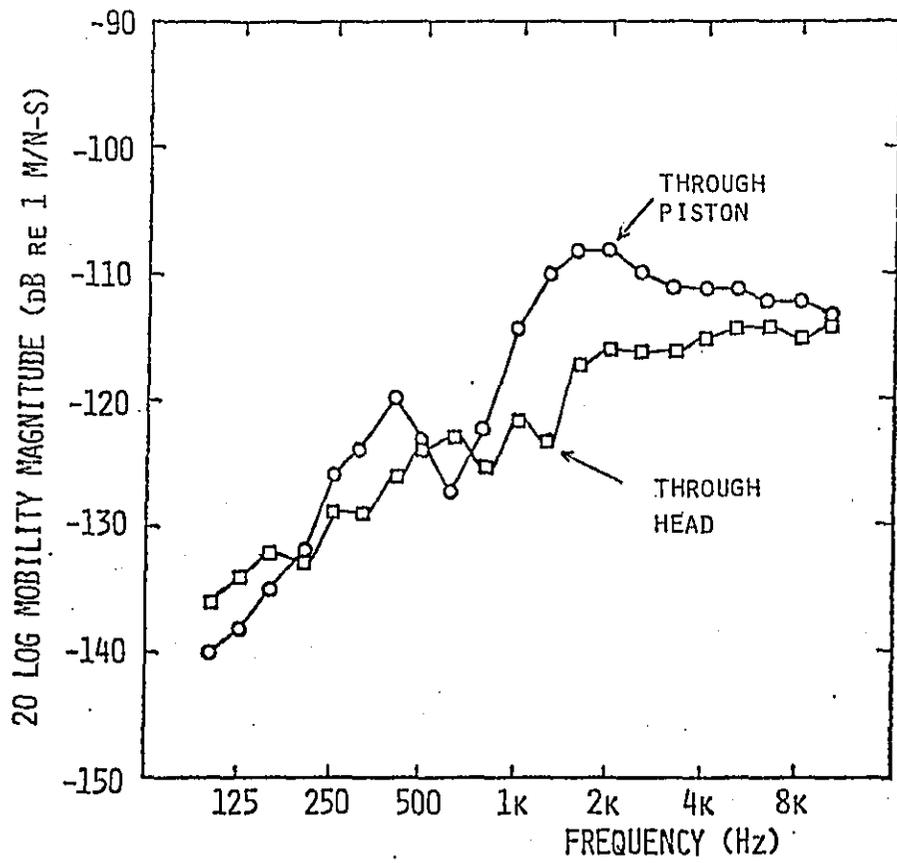
Figure 11. Transfer Mobilities for Combustion Force to Block Vibration on DDA 6V-92TTA Engine
