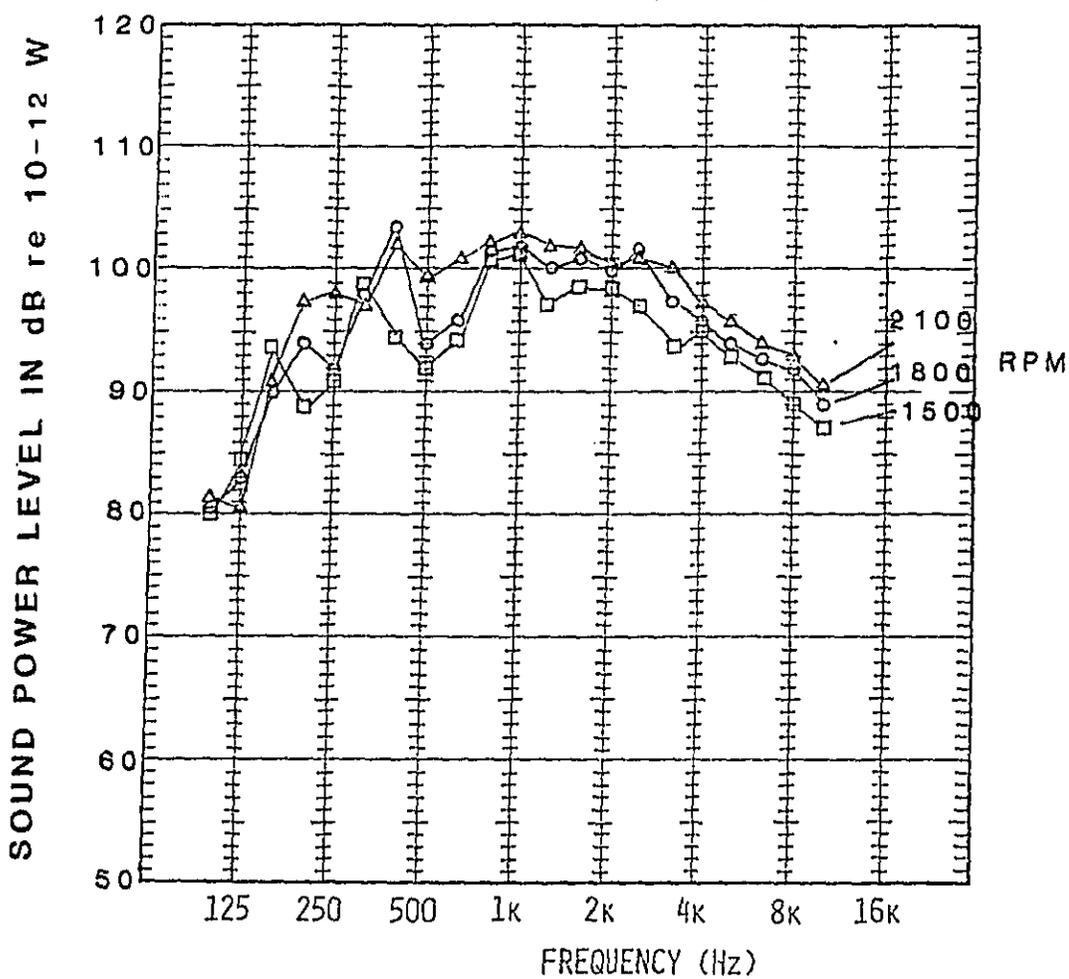
Figure 7. Frequency Spectra of Sound Power Levels of DDA 6V-92TTA Engine for Three Speeds
