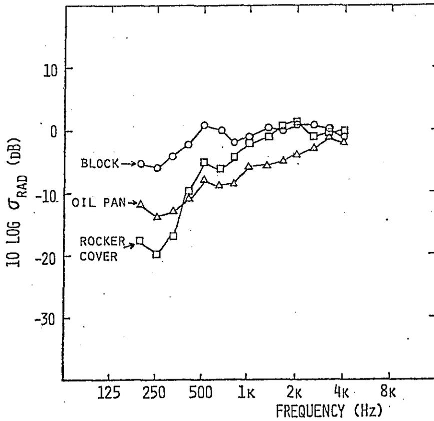
Figure 25. Measured Radiation Efficiencies of Surface Vibration on DDA 6V-92TTA Engine
