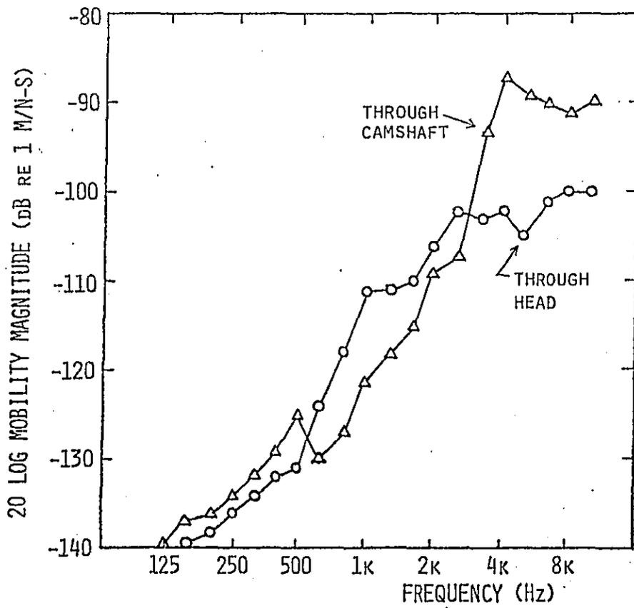
Figure 21. Transfer Mobilities of Injector Forces to Block Vibration on DDA 6V-92TTA Engine
