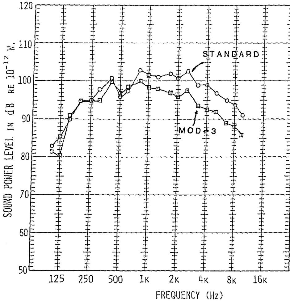
Figure 34. Overall Noise Radiation of Demonstration Engine #2 vs. Standard DDA 6V-92TTA Engine
