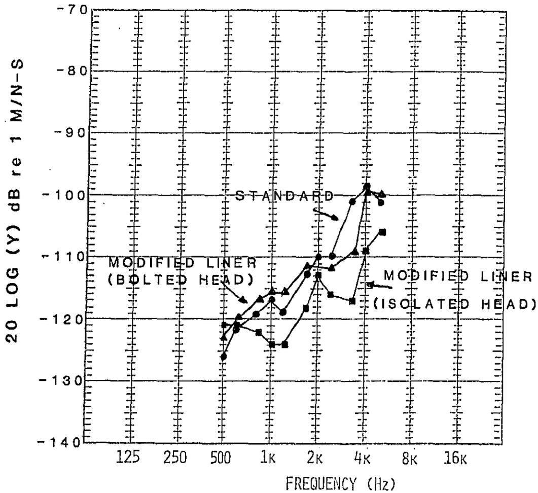
Figure 32. Transfer Mobility of Piston Slap Force to Block Vibration with New Liner Attachments on NTC-350 Engine
