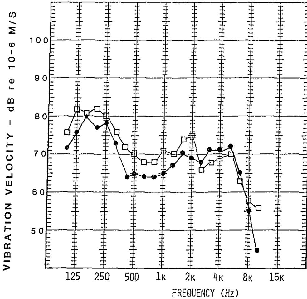
Figure 10. Lower Right and Left Block Surface Vibration Levels on NTC-350 Engine at 2100 RPM, Full Load
