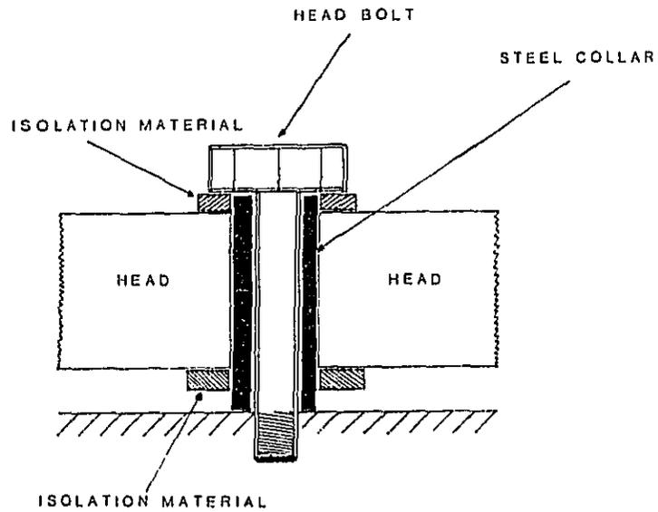
Figure 31. Bolt Isolation Design for NTC-350 Engine
