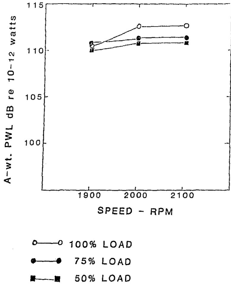
Figure 6. A-Weighted Sound Power Levels of NTC-350 vs. Engine Speed at Three Load Conditions
