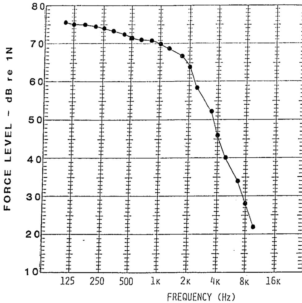
Figure 17. Estimated Force of Piston Slap on NTC-350 Engine at 2100 RPM, Full Load
