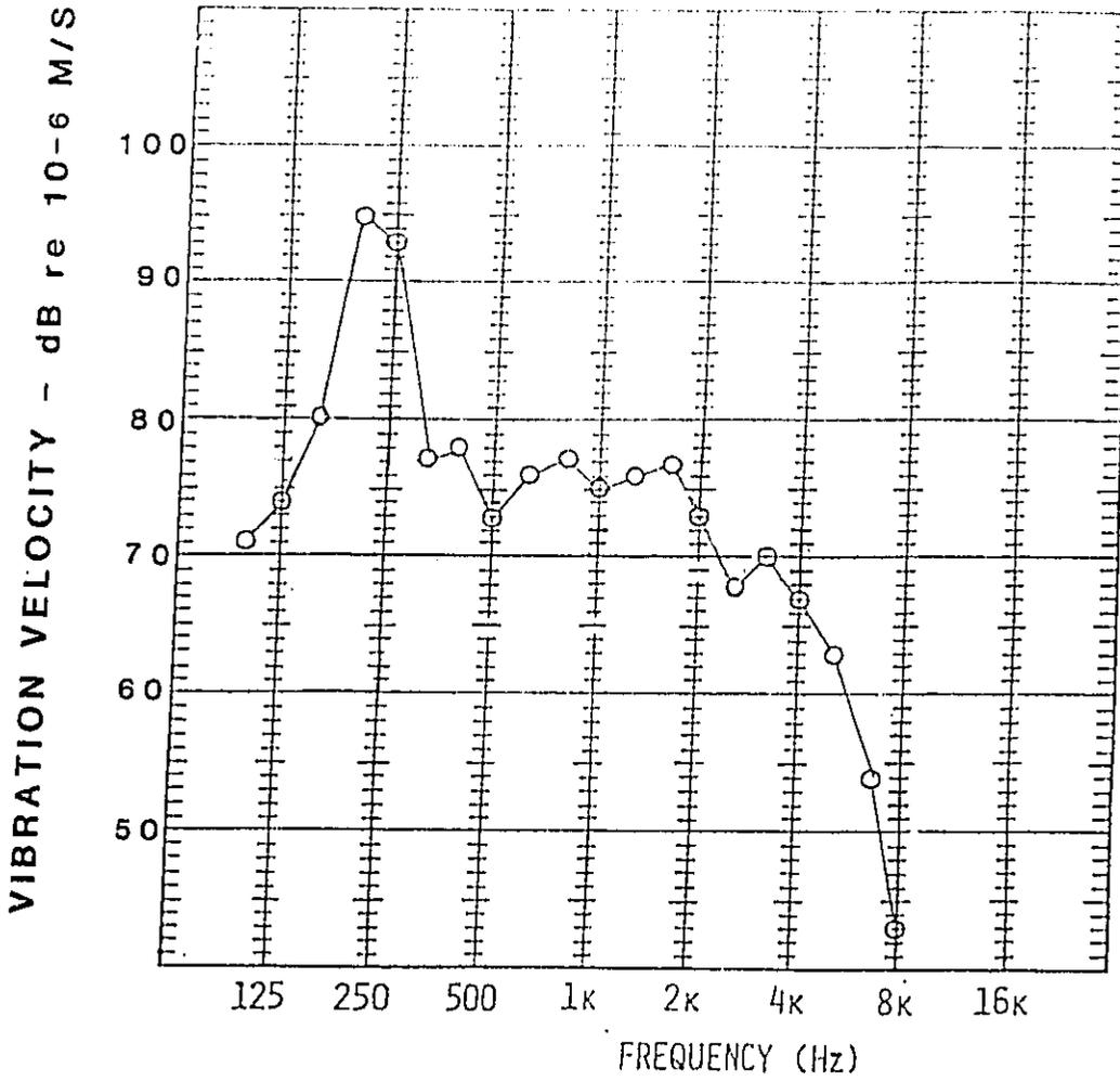
Figure 11. Oil Pan Surface Vibration Levels on NTC-350 Engine at 2100 RPM, Full Load
