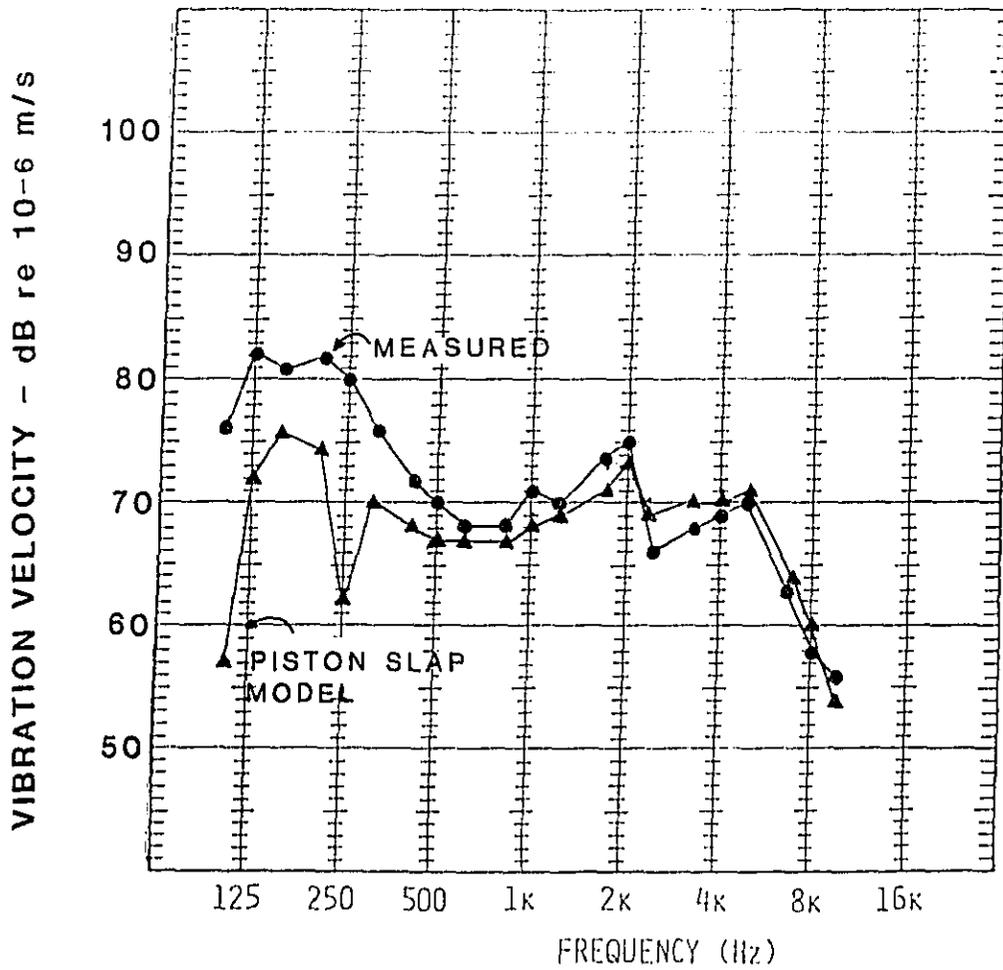
Figure 19. Piston Slap Vibration Levels vs. Measured Block Vibration Levels on NTC-350 Engine at 2100 RPM, Full Load
