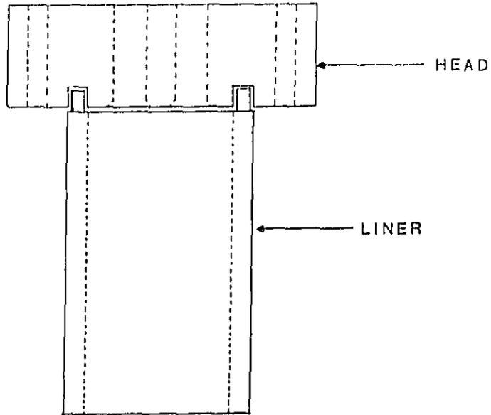
Figure 30. Proposed Liner Attachment to Head on NTC-350 Engine
