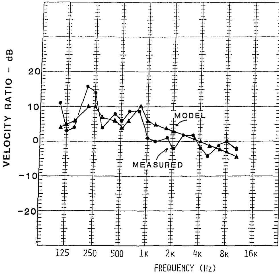
Figure 26. Oil Pan to Lower Block Vibration Ratio on NTC-350 Engine at 2100 RPM, Full Load
