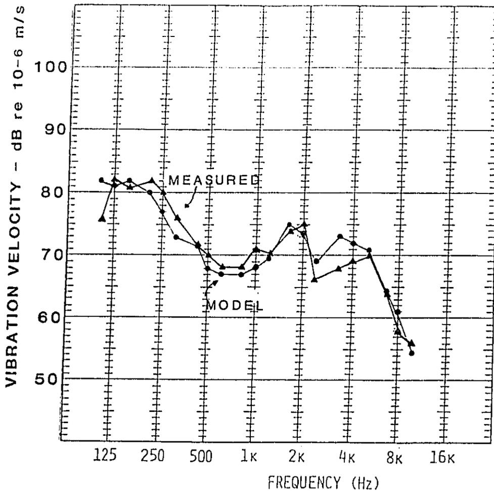
Figure 24. Sum of Piston Slap and Injector Vibration Levels to Lower Left Block vs. Measured Vibration Levels on NTC-350 Engine at 2100 RPM, Full Load
