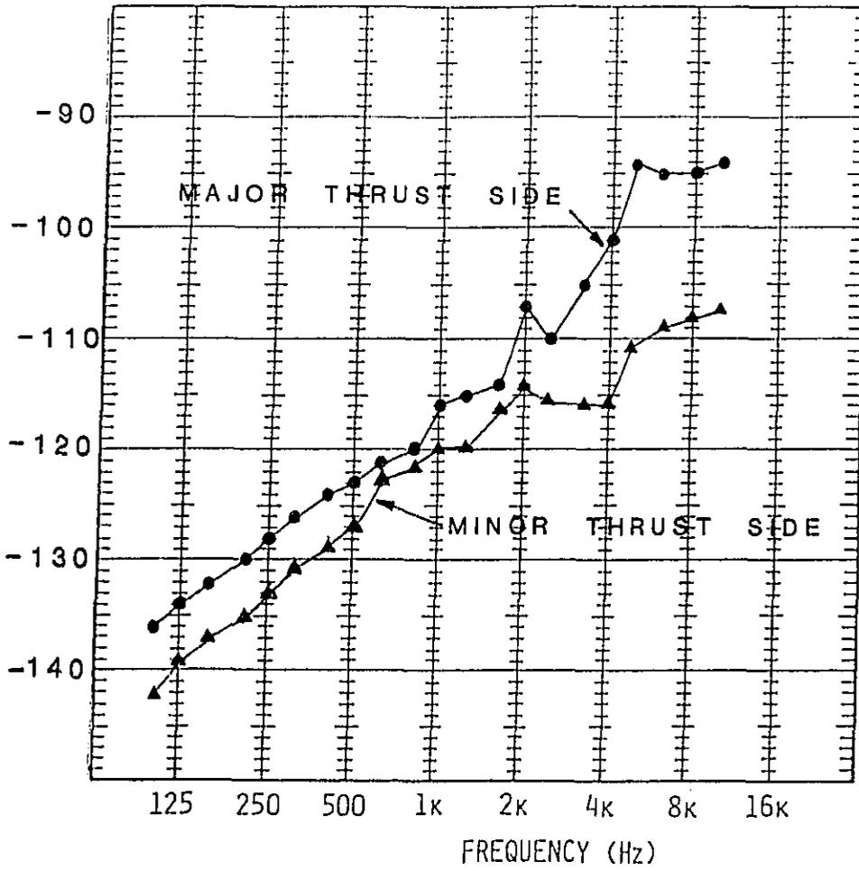
Figure 18. Piston Slap Vibration Transmission from Cylinder Liner to Block on NTC-350 Engine
