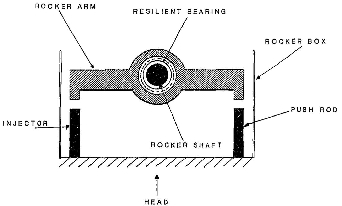
Figure 33. Injector Isolation Design on NTC-350 Engine
