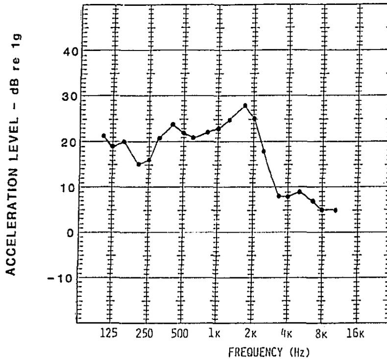
Figure 20b. Frequency Spectra of Injector Vibration Level on NTC-350 Engine at 2100 RPM, Full Load
