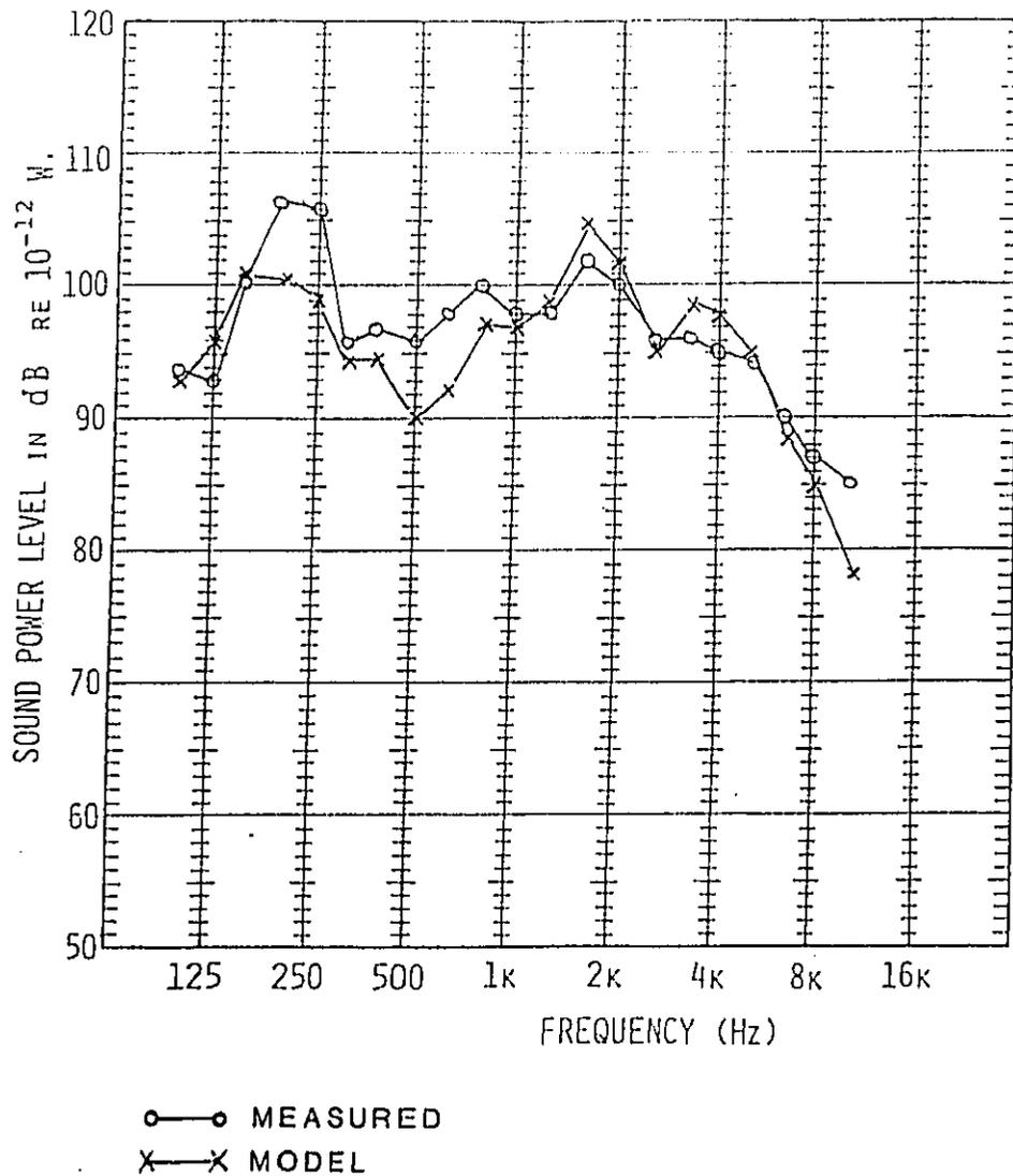
Figure 27. Lower "In-Truck" Sound Power Levels vs. Total Measured Sound Power Levels on NTC-350 Engine
