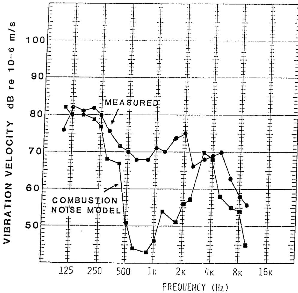
Figure 14. Comparison of Vibration Transmission from Combustion with Overall Vibration on NTC-350 Engine at 2100 RPM, Full Load
