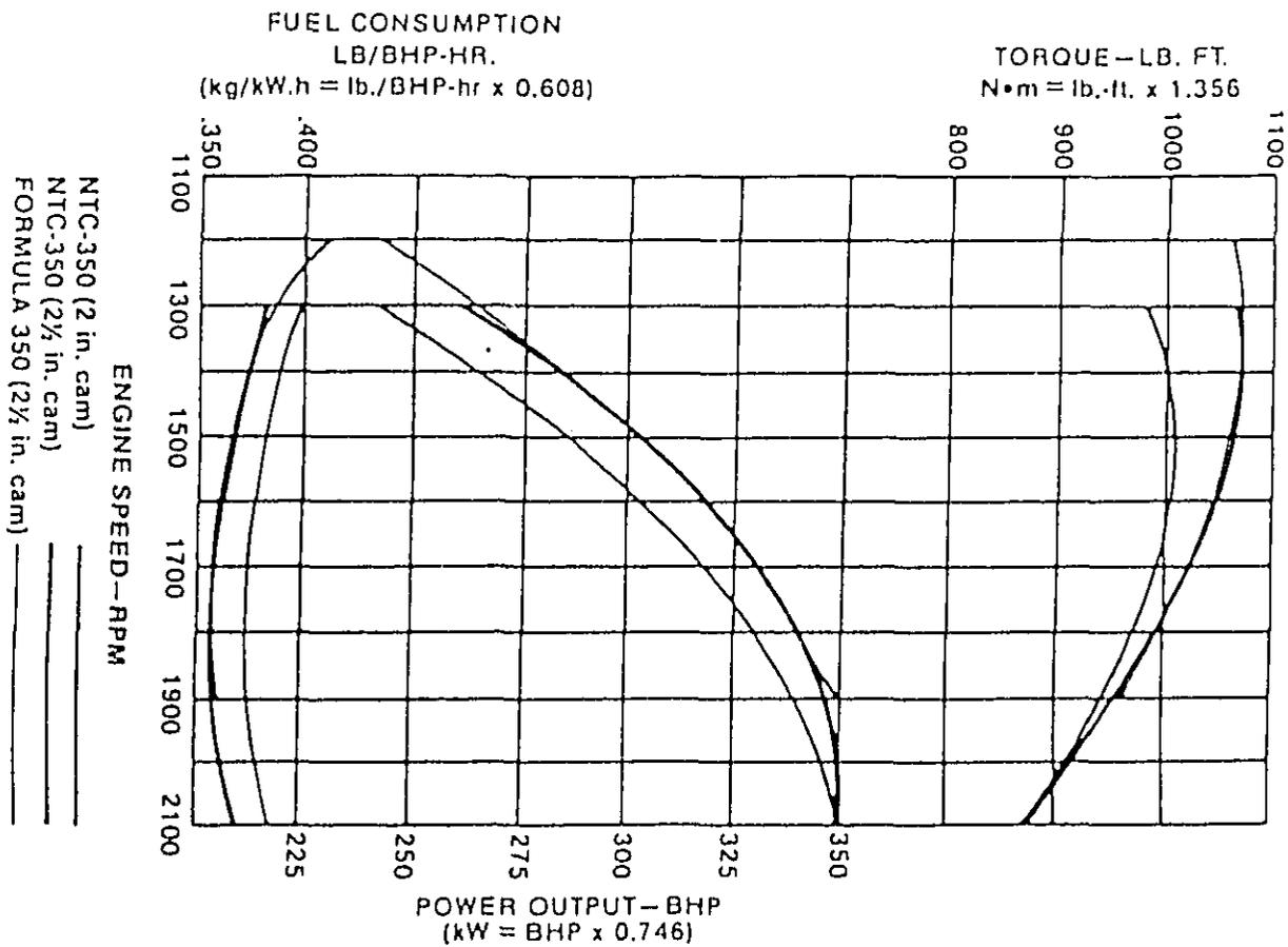
Figure 2. Performance Curve for NTC-350 Engine
