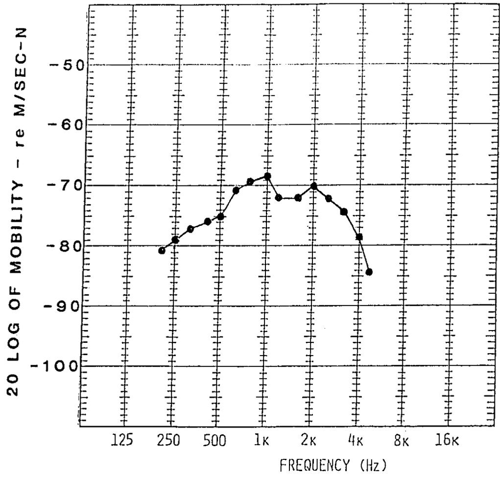
Figure 21. Drivepoint Mobility of Injector on NTC-350 Engine
