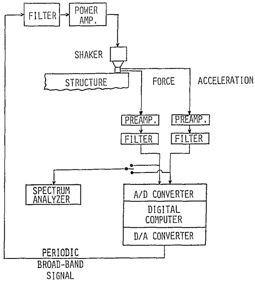
Figure 13. Instrumentation for Mobility Measurements
