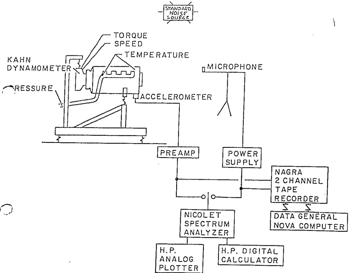
Figure 3. Noise Measurement Instrumentation
