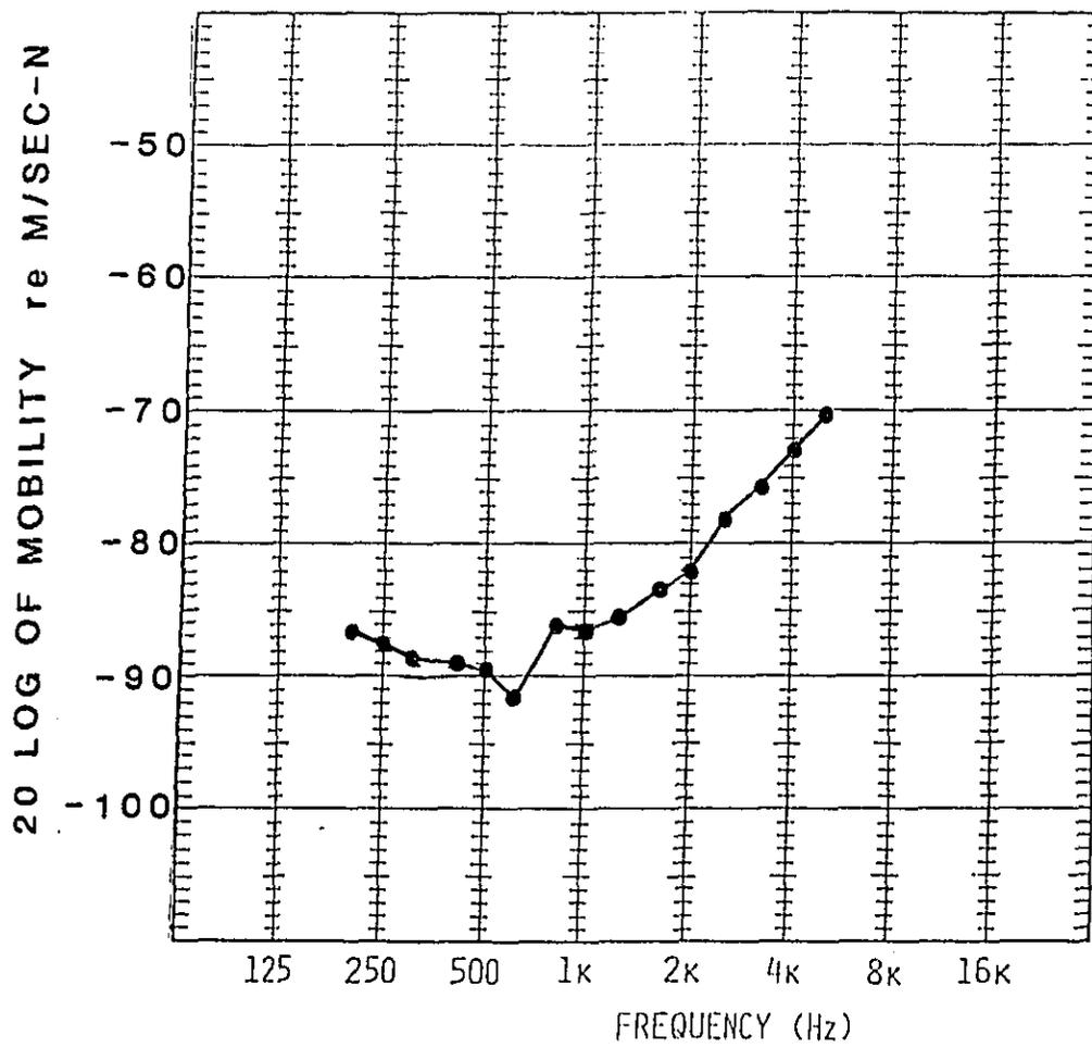
Figure 16. Drivepoint Mobility of Cylinder Liner on NTC-350 Engine
