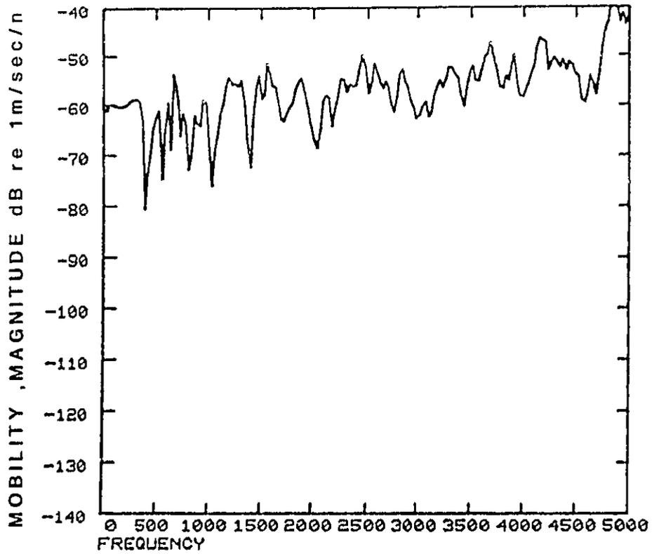
Figure 25. Oil Pan Mobilities, Free, on NTC-350 Engine
