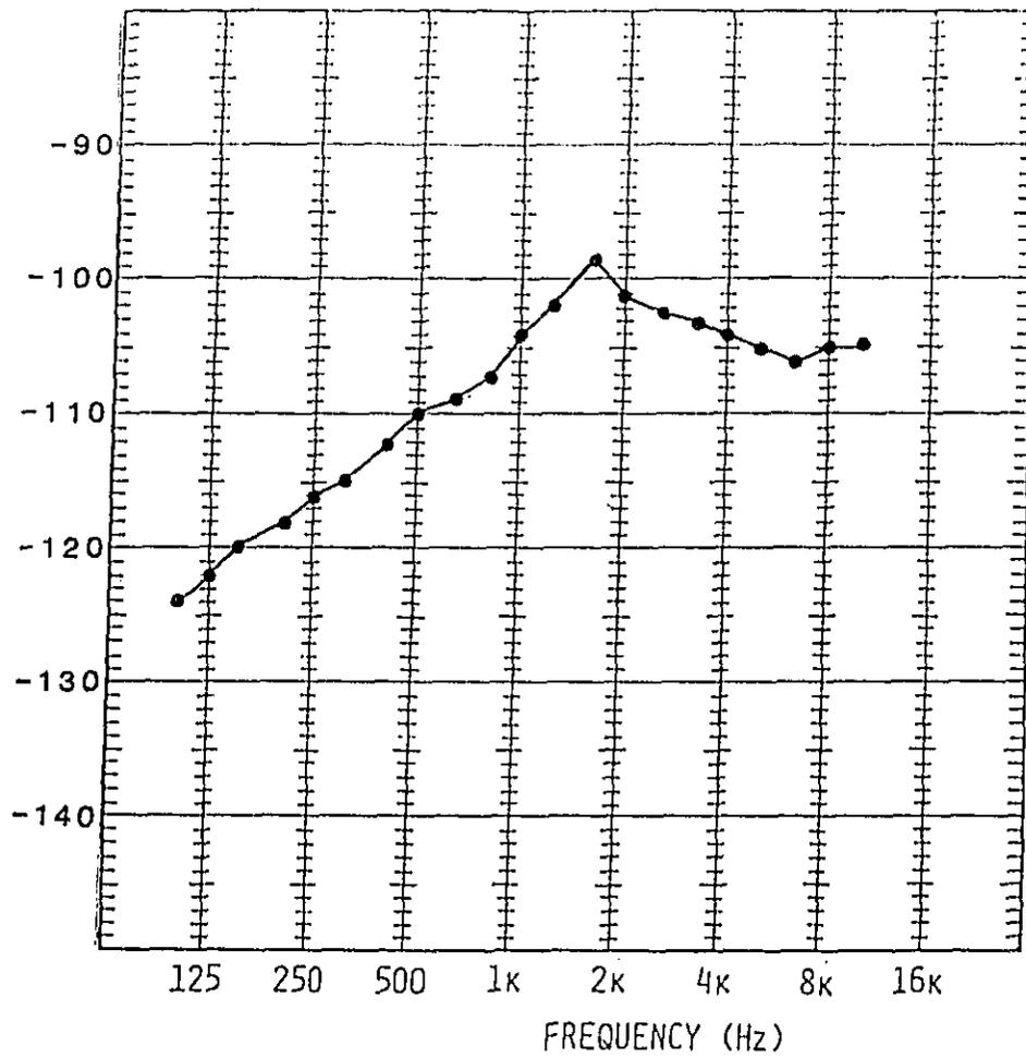
Figure 22. Vibration Transmission from Injector to Block on NTC-350 Engine
