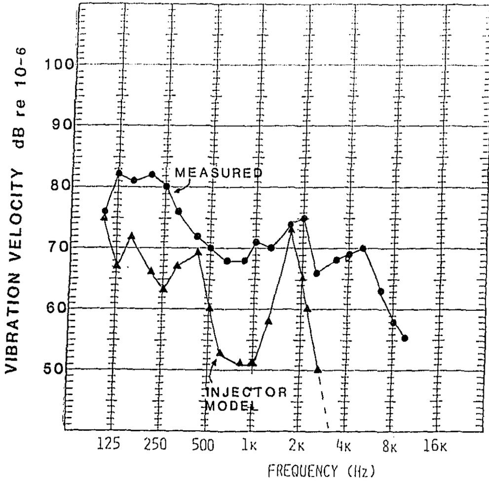
Figure 23. Injector Vibration Levels to Lower Left Block vs. Measured Vibration Levels on NTC-350 Engine at 2100 RPM, Full Load
