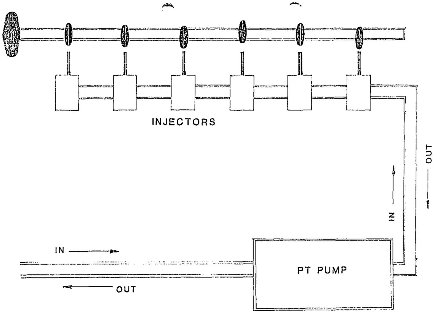
Figure 1. Fuel System of NTC-350 Engine
