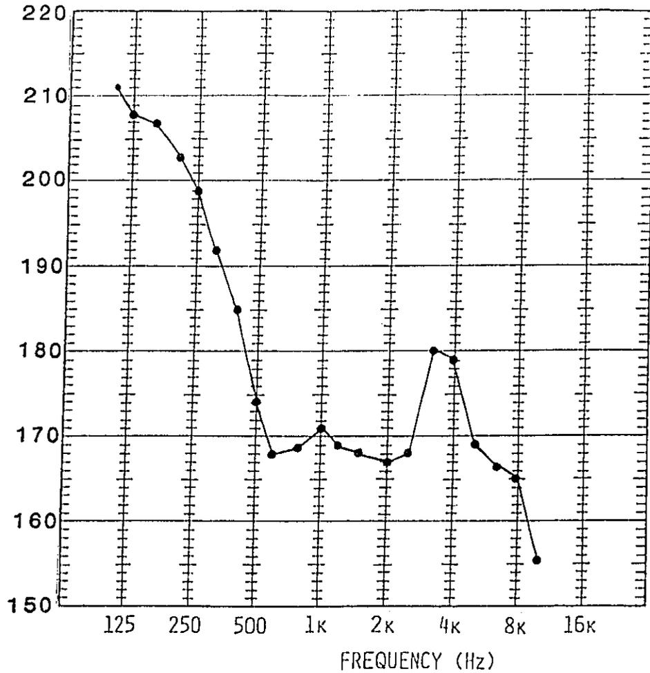
Figure 12. Frequency Spectra of Measured Cylinder Pressure on NTC-350 Engine at 2100 RPM, Full Load
