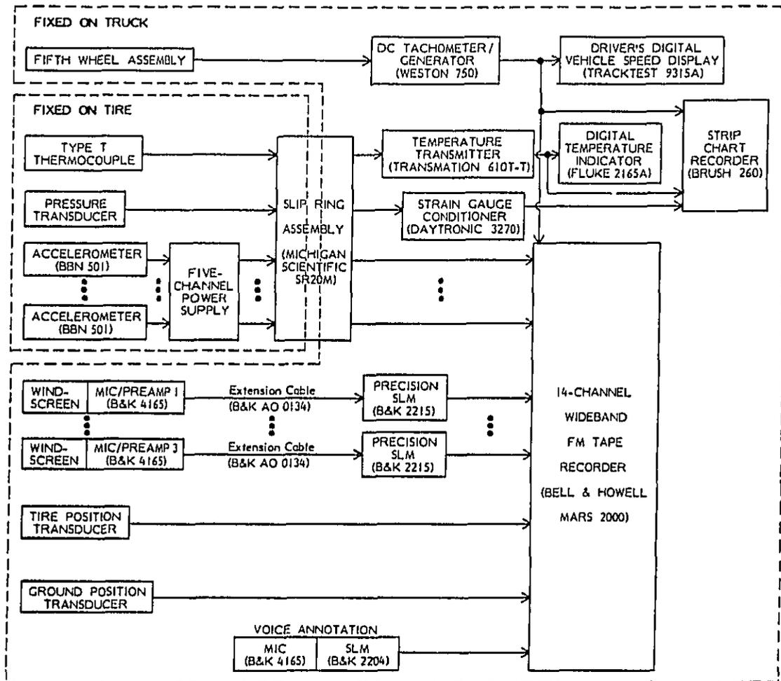
Figure 13. Instrumentation for Outdoor Tests.
