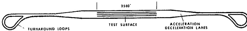
Figure 18. Skid Pad at Ohio TRC.
