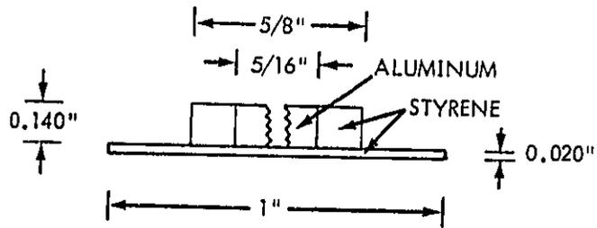
Figure 15. Accelerometer Mount Design.
