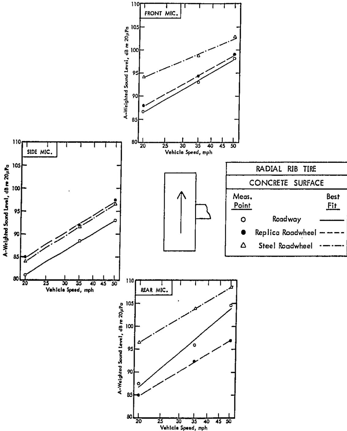
Figure 35 (a). A-Weighted Sound Level Versus Vehicle Speed as a Function of Surface Type for Radial Rib Tire and Concrete Surfaces.
