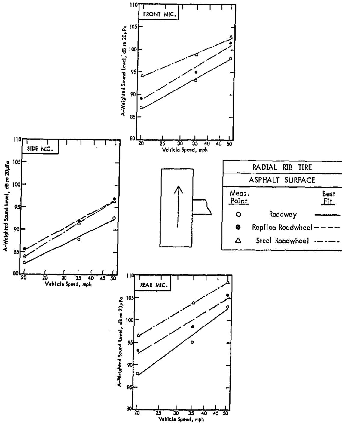
Figure 35 (b). A-Weighted Sound Level Versus Vehicle Speed as a Function of Surface Type for Radial Rib Tire and Asphalt Surfaces.
