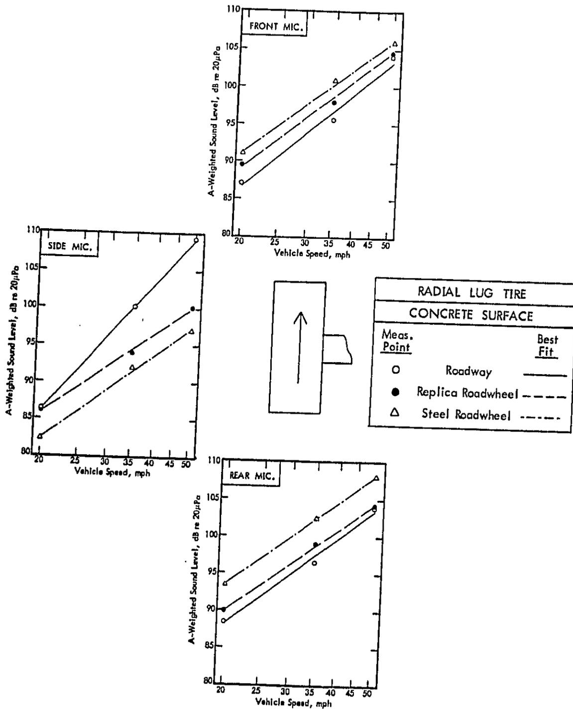
Figure 36 (a). A-Weighted Sound Level Versus Vehicle Speed as a Function of Surface Type for Radial Lug Tire and Concrete Surfaces.
