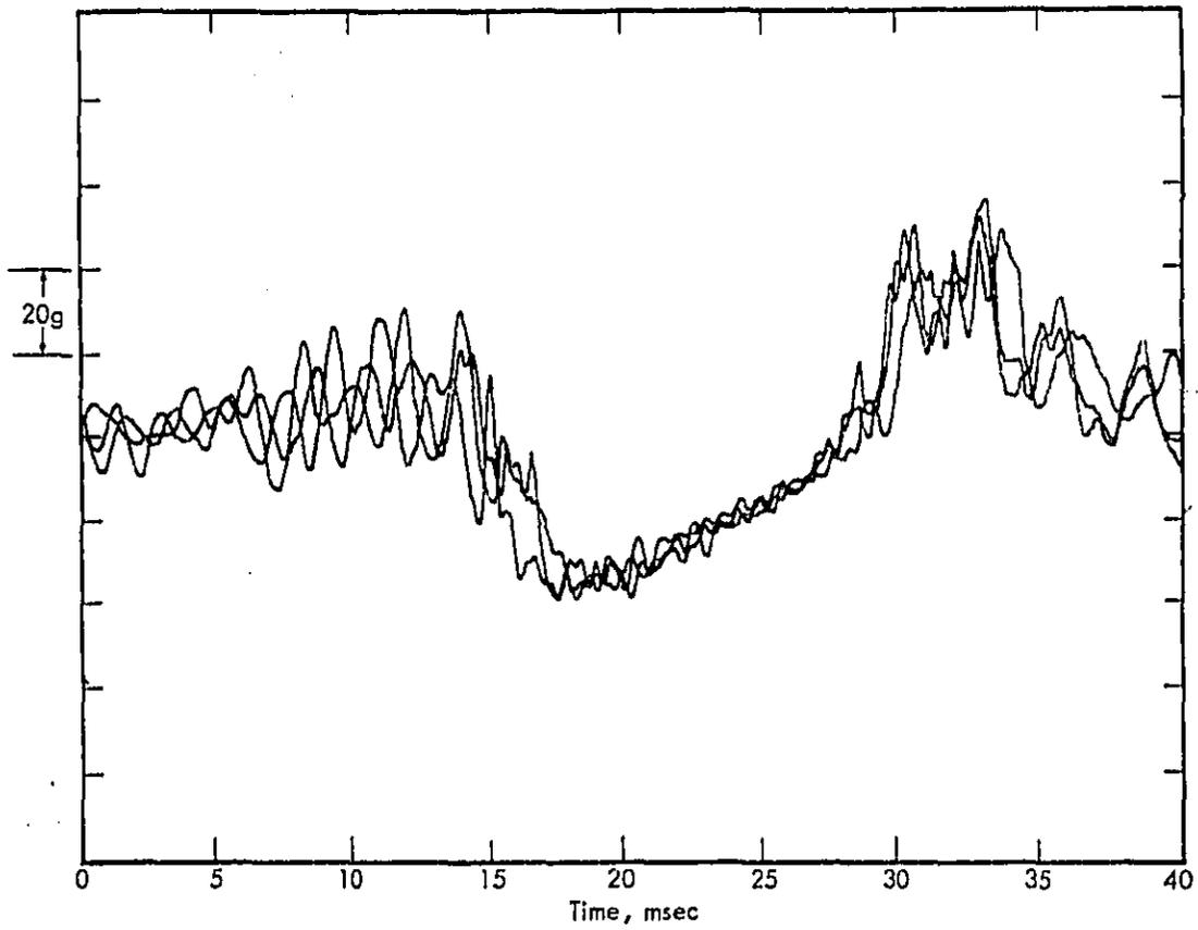
Figure 54. Successive Samples of Carcass Acceleration on Real Surface.
