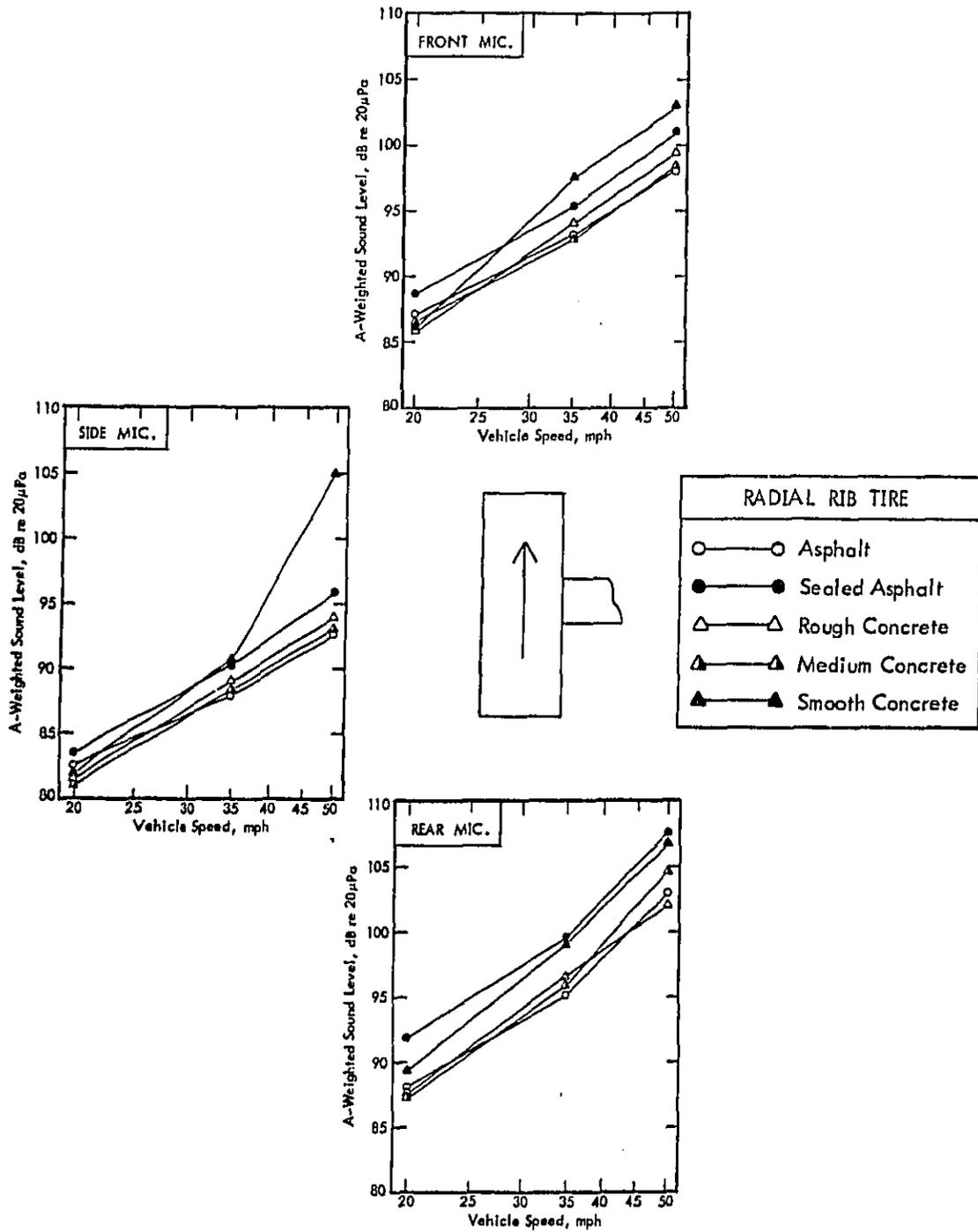
Figure 31. A-Weighted Sound Level Versus Vehicle Speed as a Function of Roadway Surface for Radial Rib Tire.
