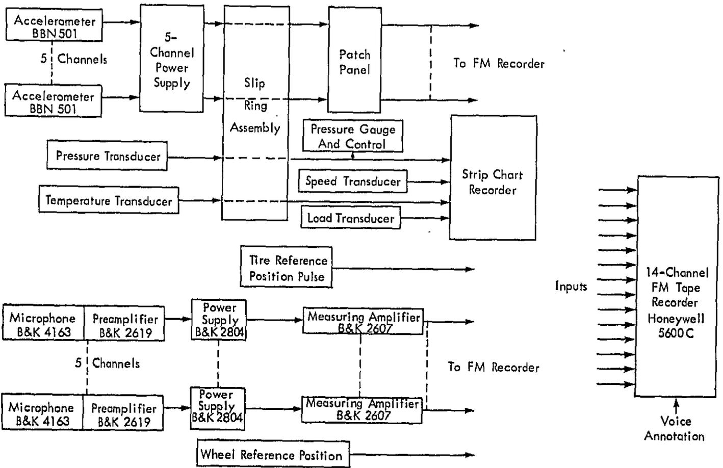
Figure 22. Instrumentation for Roadwheel Measurements.
