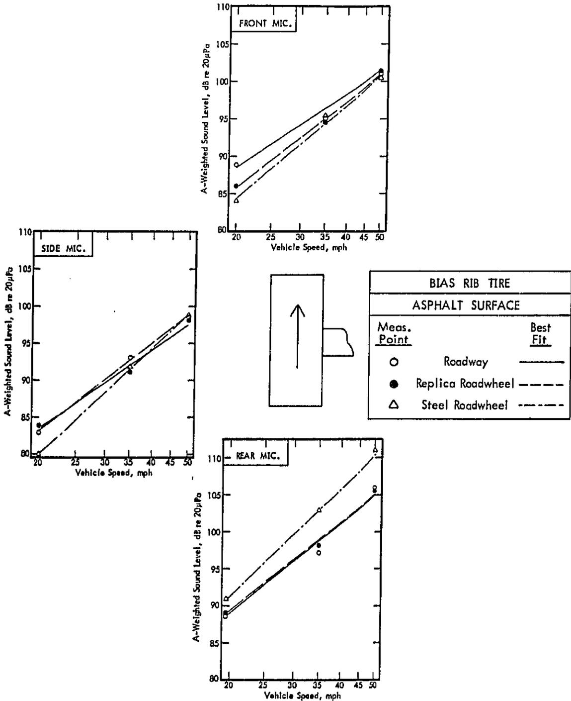
Figure 37 (b). A-Weighted Sound Level Versus Vehicle Speed as a Function of Surface Type for Bias Rib Tire and Asphalt Surfaces.
