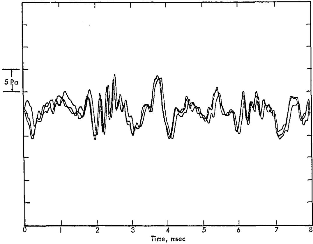
Figure 49. Successive Samples of Sound Pressure on Steel Roadwheel.
