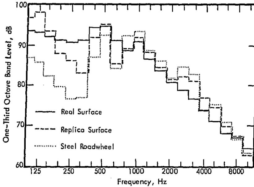
b) Asphalt. Radial Lug Tire, Front Microphone.
