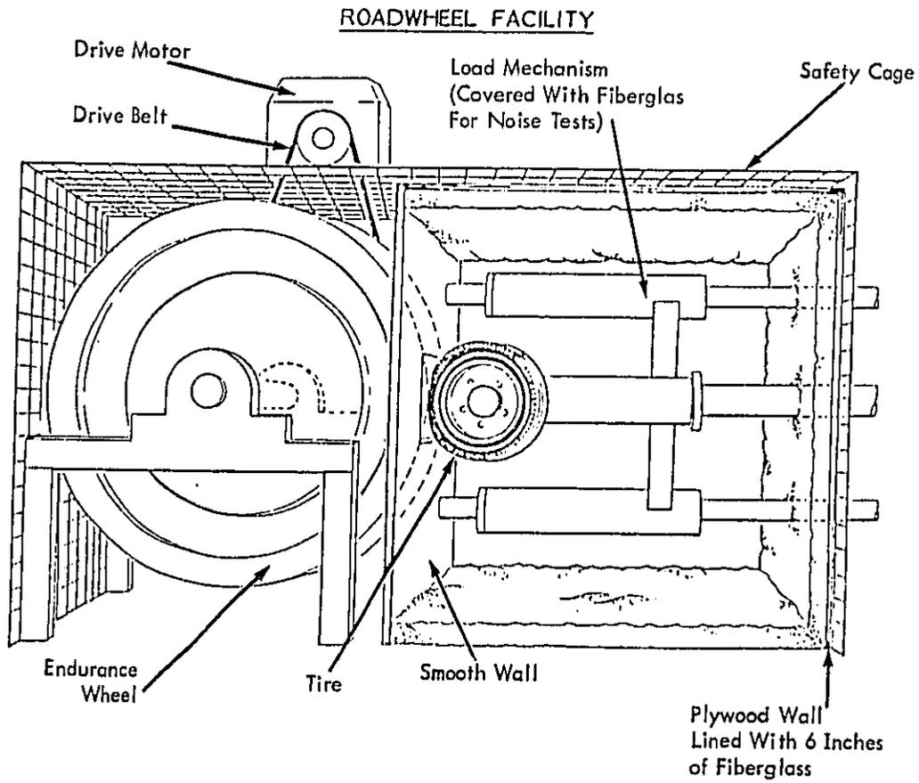
Figure 1. Endurance Wheel Noise Test Facility.
