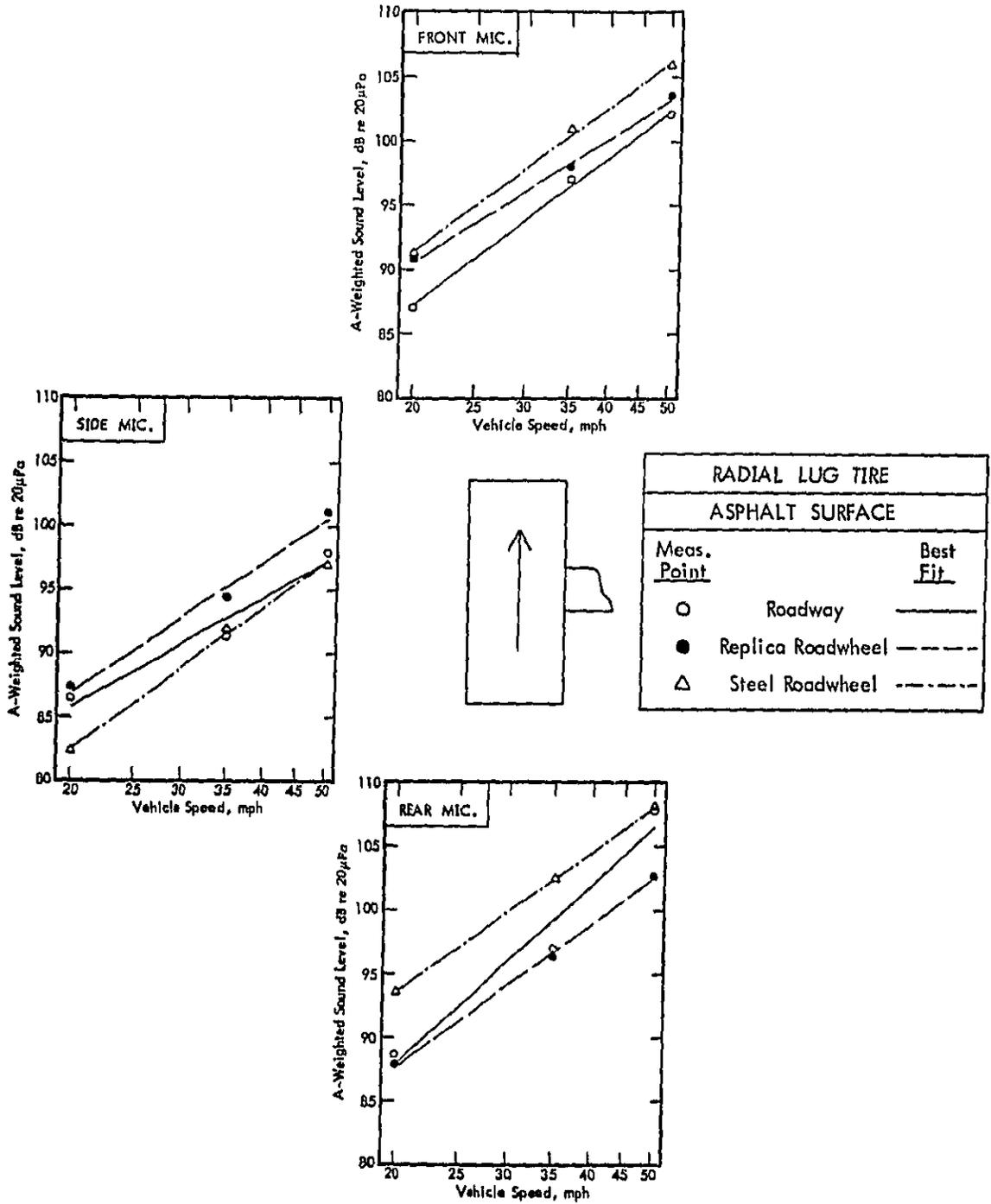
Figure 36 (b). A-Weighted Sound Level Versus Vehicle Speed as a Function of Surface Type for Radial Lug Tire and Asphalt Surfaces.
