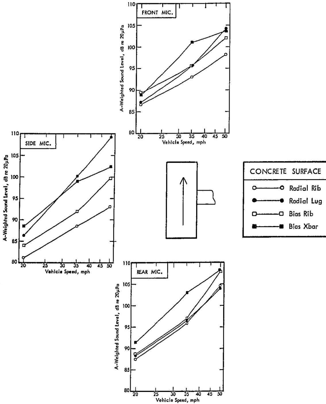
Figure 29. A-Weighted Sound Level Versus Vehicle Speed as a Function of Tire Type for Concrete Surface (CI).
