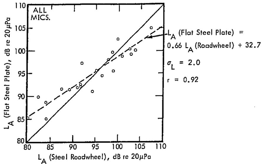
Figure 46. Best Linear Fit of Flat Steel Plate Levels to Steel Roadwheel Levels for All Tires, All Microphone Positions, and Two Vehicle Speeds.
