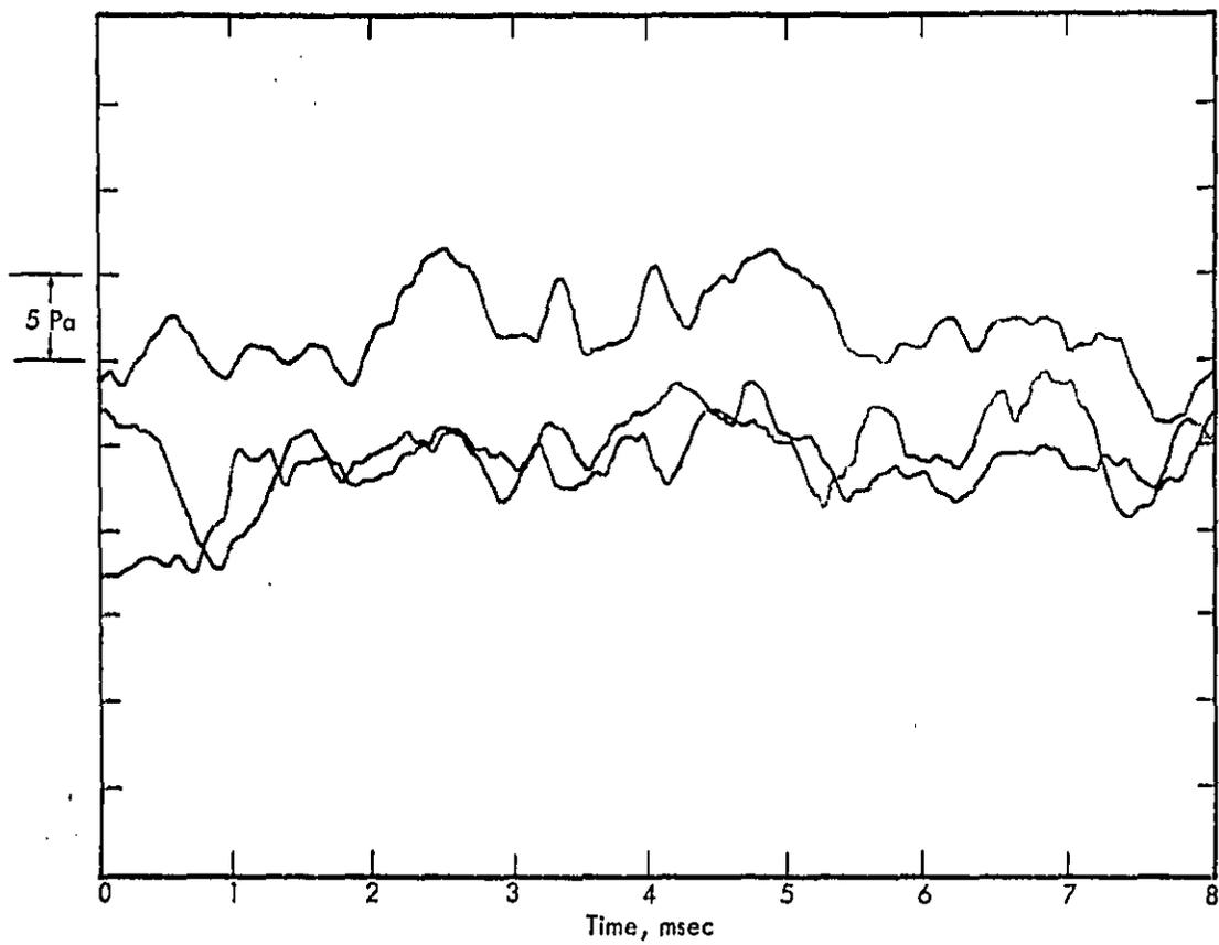
Figure 53. Successive Samples of Sound Pressure on Real Surface.
