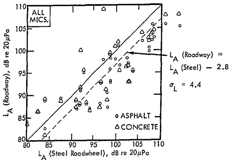
Figure 40. Best Unit-Slope Linear Fit of Roadway Levels to Roadwheel Levels for All Tires, Both Roadway Surfaces, All Vehicle Speeds, and All Microphone Positions.
