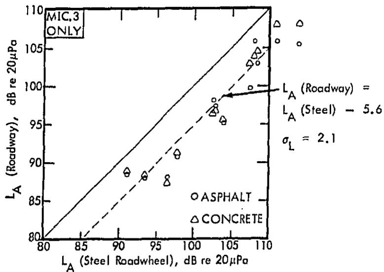
Figure 41. Best Unit-Slope Linear Fit of Roadway Levels to Roadwheel Levels for All Tires, Both Roadway Surfaces, All Vehicle Speeds, and Microphone 3 Only.
