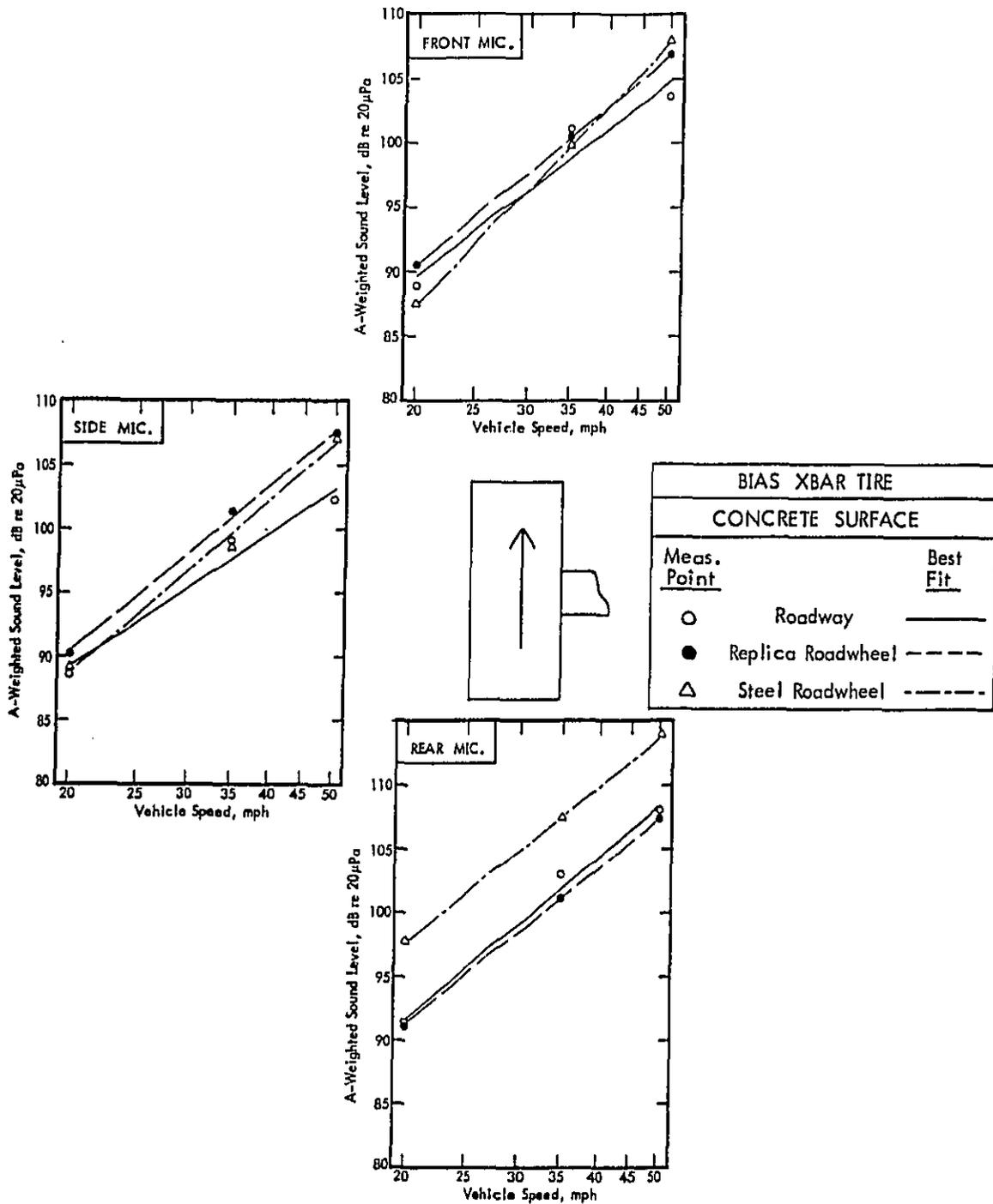
Figure 38 (a). A-Weighted Sound Level Versus Vehicle Speed as a Function of Surface Type for Bias Crossbar Tire and Concrete Surfaces.
