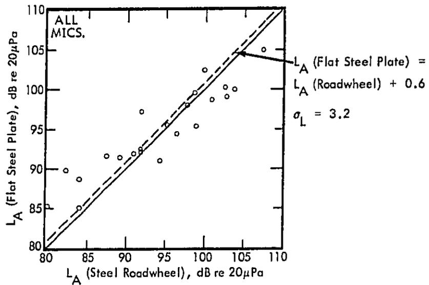
Figure 47. Best Unit-Slope Linear Fit of Flat Steel Plate Levels to Steel Roadwheel Levels for All Tires, All Microphone Positions, and Two Vehicle Speeds.
