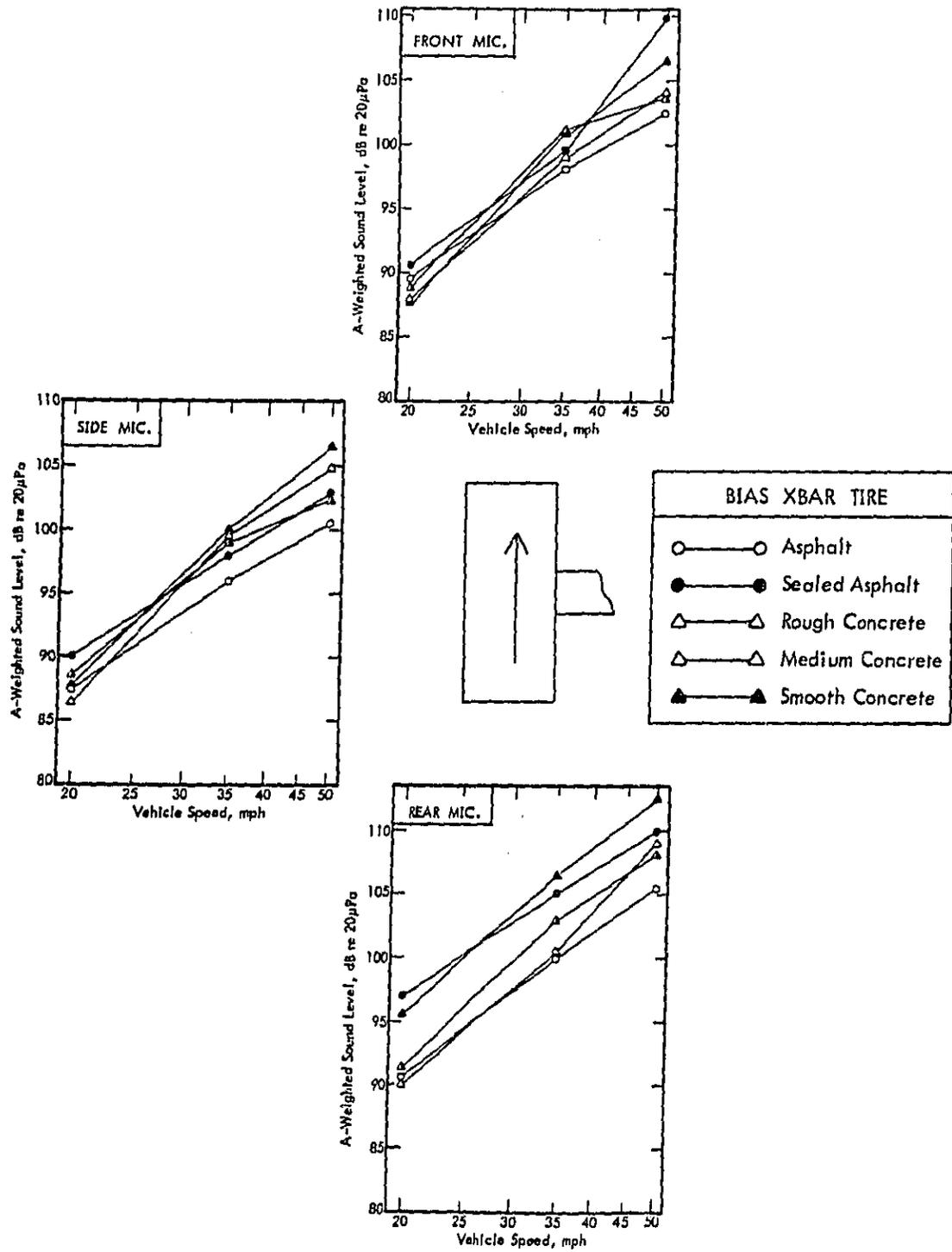
Figure 34. A-Weighted Sound Level Versus Vehicle Speed as a Function of Roadway Surface for Bias Crr
