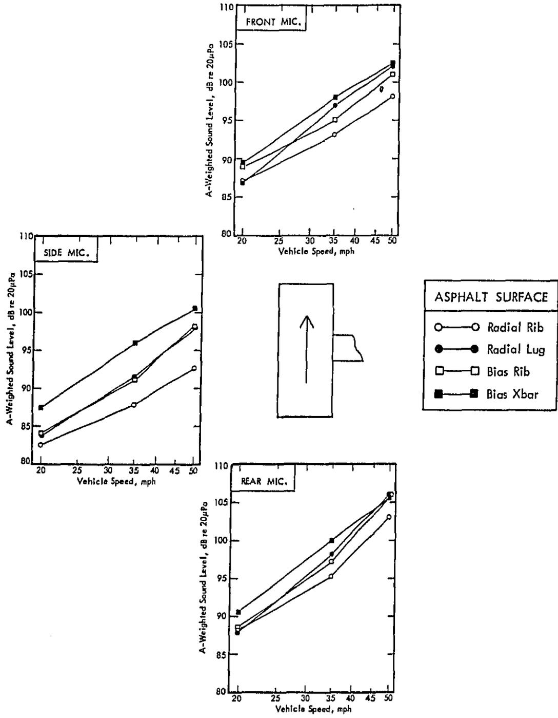
Figure 30. A-Weighted Sound Level Versus Vehicle Speed as a Function of Tire Type for Asphalt Surface (A1).
