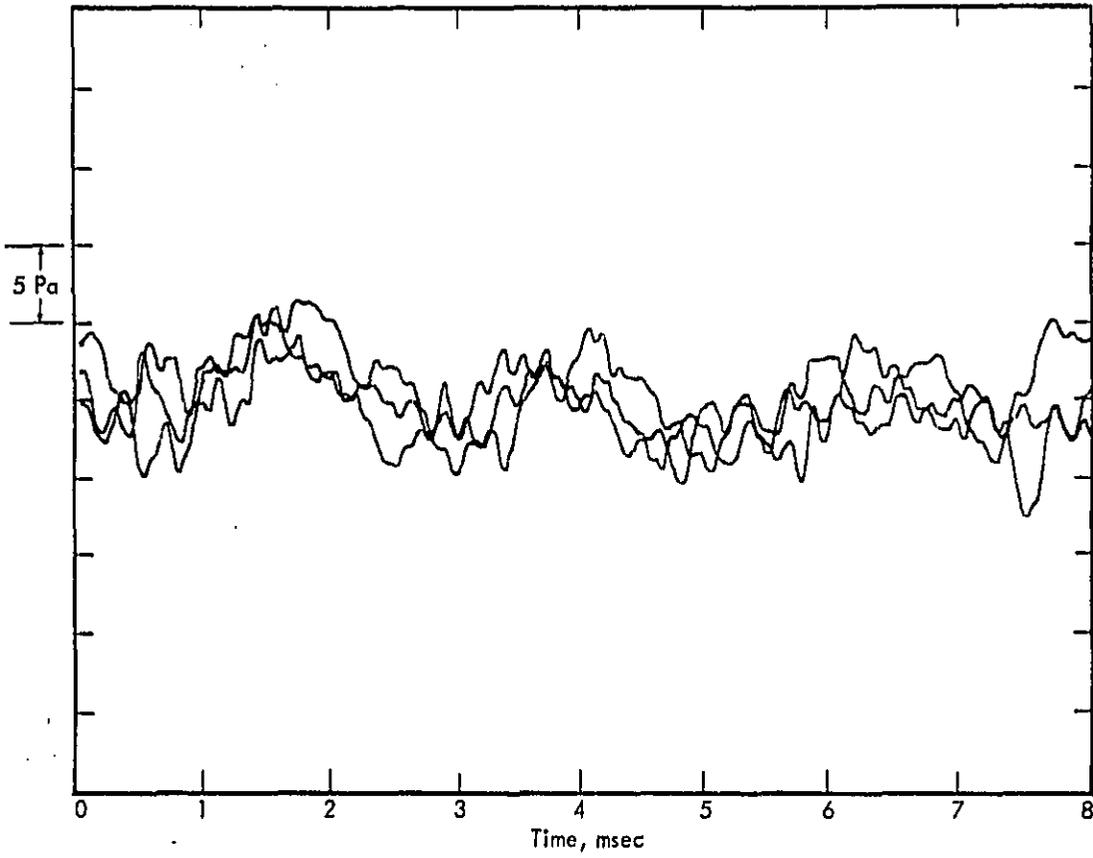
Figure 51. Successive Samples of Sound Pressure on Replica Surface.
