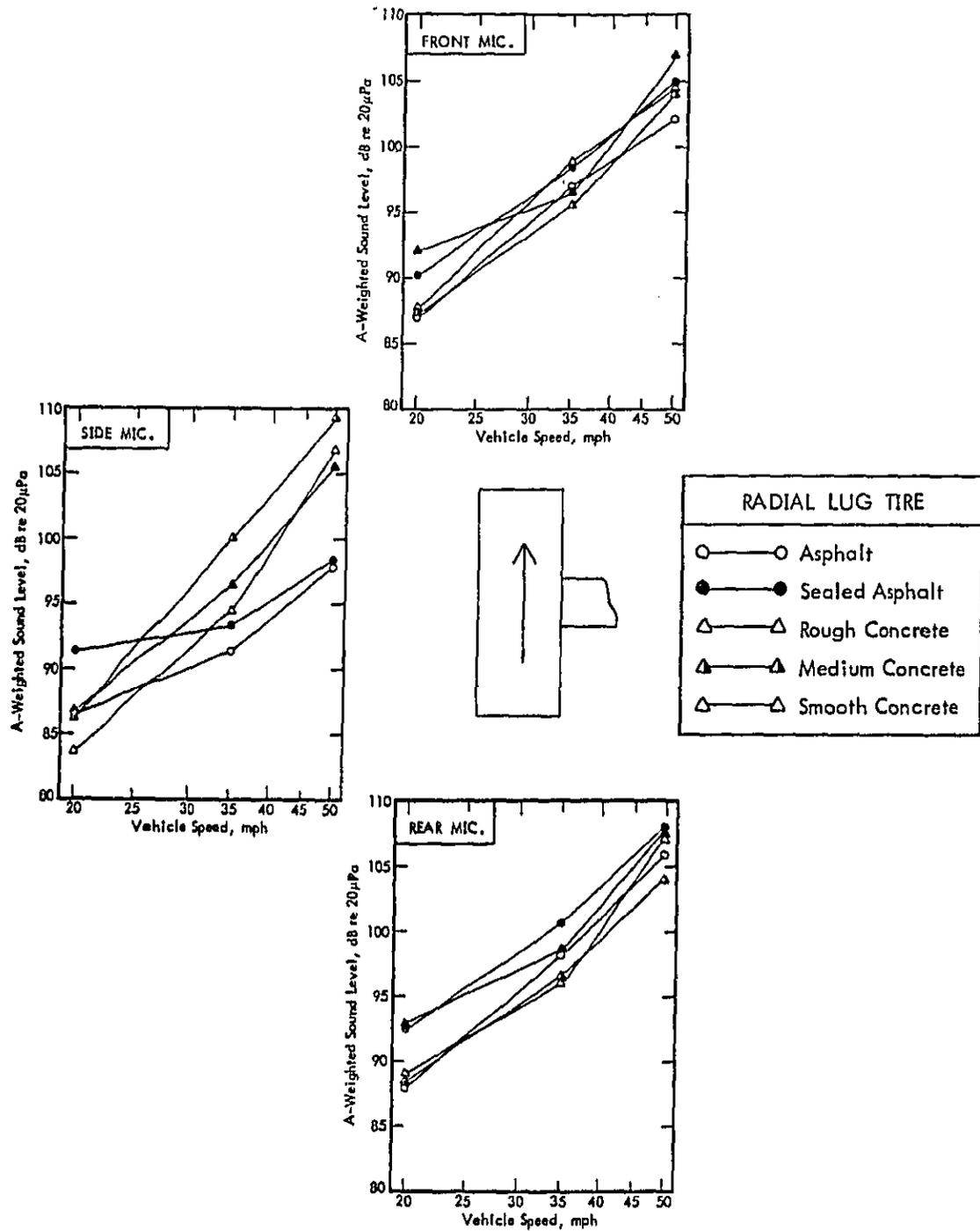
Figure 32. A-Weighted Sound Level Versus Vehicle Speed as a Function of Roadway Surface for Radial Lug Tire.
