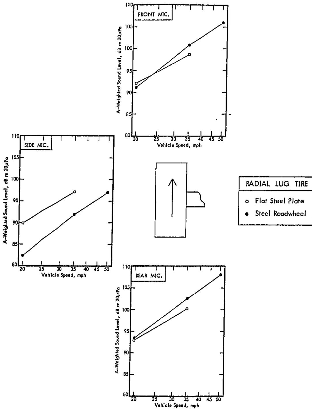
Figure 43. A-Weighted Sound Level Versus Vehicle Speed as a Function of Surface Curvature for Radial Lug Tire.
