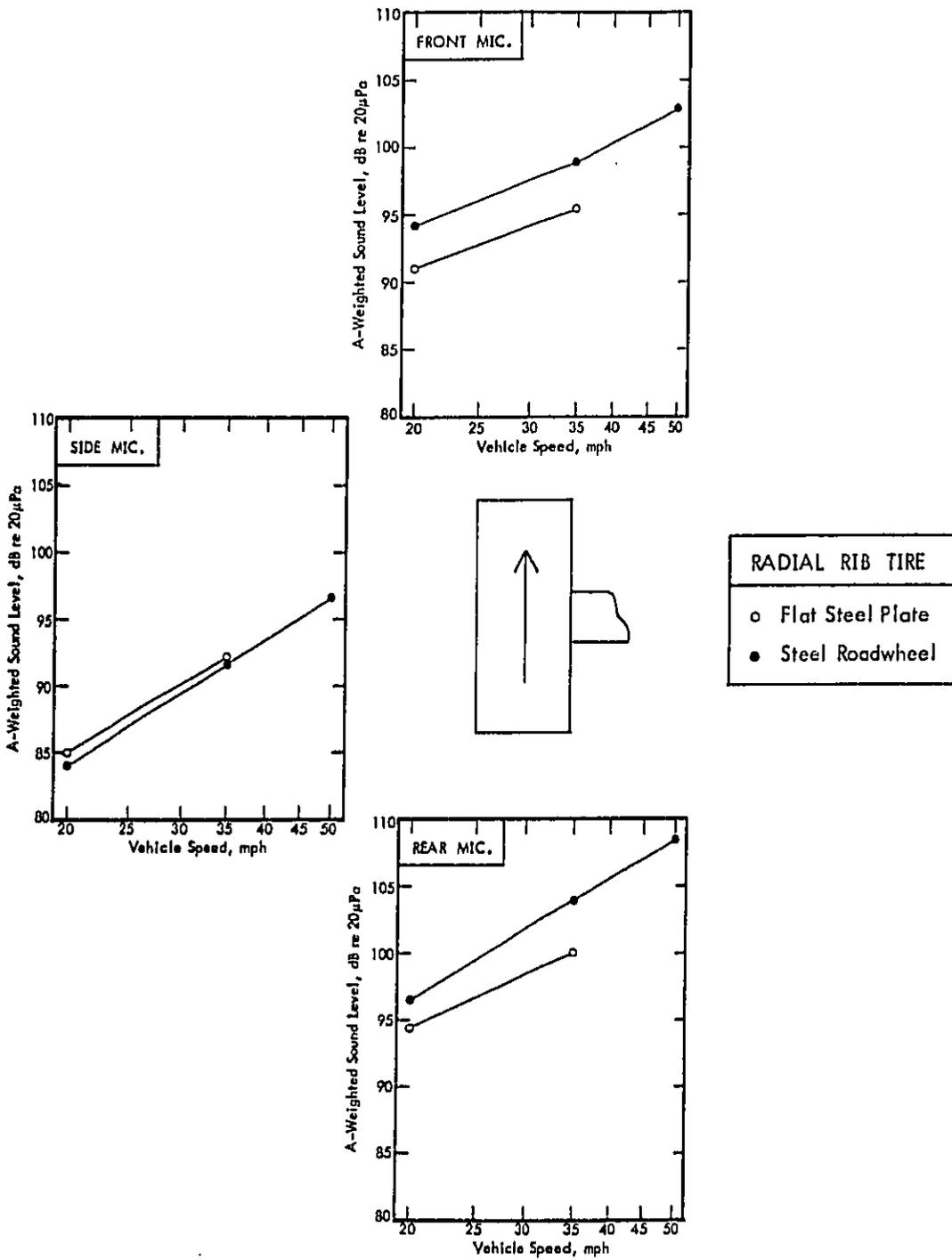
Figure 42. A-Weighted Sound Level Versus Vehicle Speed as a Function of Surface Curvature for Radial Rib Tire.
