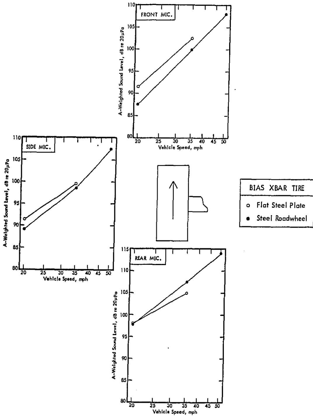
Figure 45. A-Weighted Sound Level Versus Vehicle Speed as a Function of Surface Curvature for Bias Crossbar Tire.
