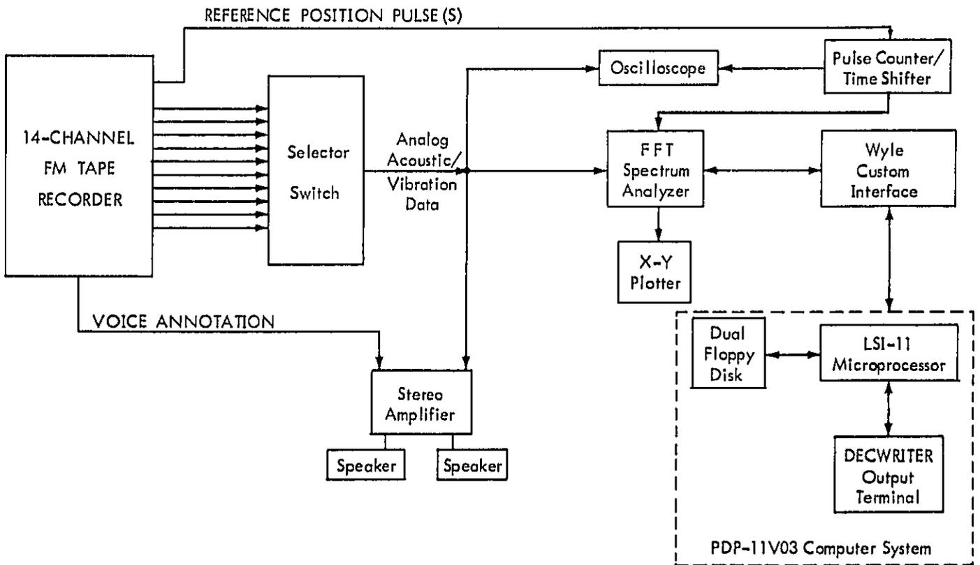
Figure 23. Instrumentation for Data Reduction.
