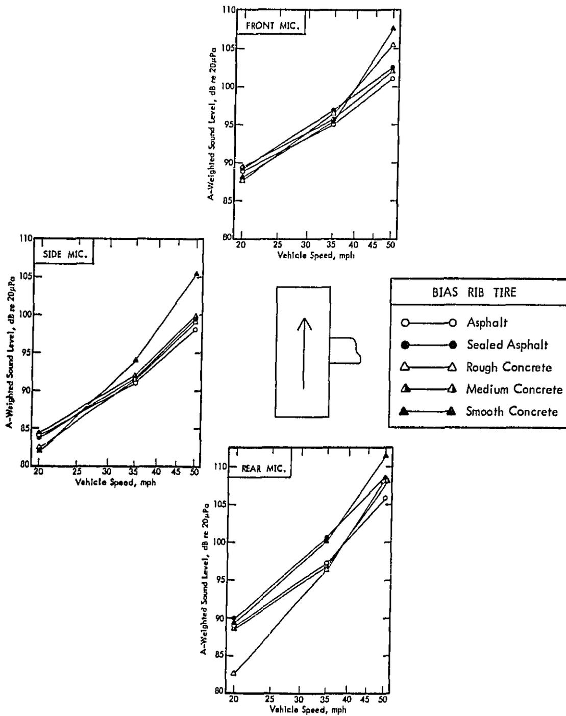
Figure 33. A-Weighted Sound Level Versus Vehicle Speed as a Function of Roadway Surface for Bias Rib Tire.
