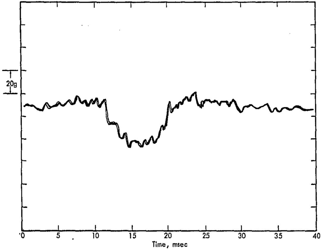
Figure 50. Successive Samples of Carcass Acceleration on Steel Roadwheel.
