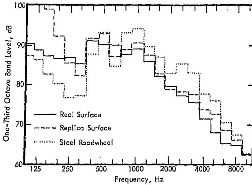
a) Concrete. Radial Lug Tire, Front Microphone.
