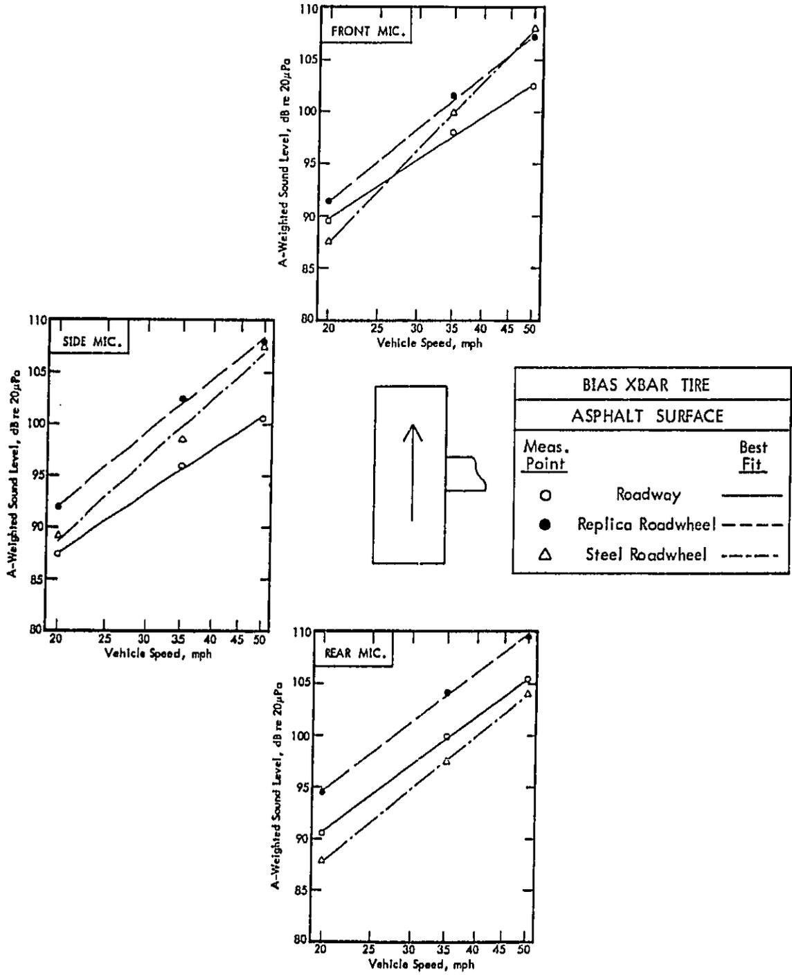
Figure 38 (b). A-Weighted Sound Level Versus Vehicle Speed as a Function of Surface Type for Bias Crossbar Tire and Asphalt Surfaces.
