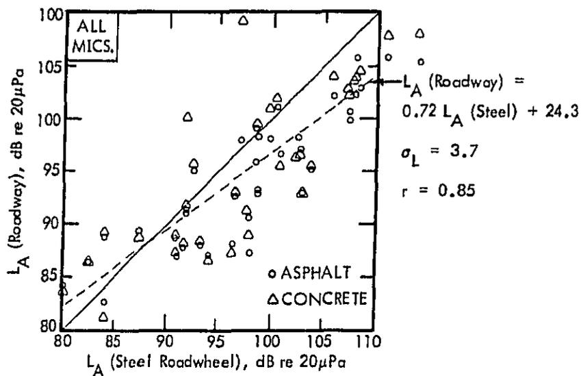
Figure 39. Best Linear Fit of Roadway Levels to Roadwheel Levels for All Tires, Both Roadway Surfaces, All Vehicle Speeds, and All Microphone Positions.
