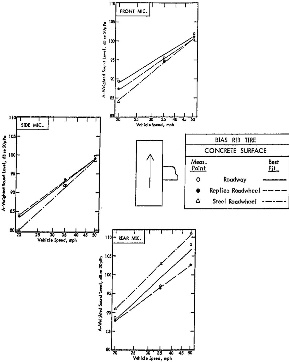
Figure 37 (a). A-Weighted Sound Level Versus Vehicle Speed as a Function of Surface Type for Bias Rib Tire and Concrete Surfaces.
