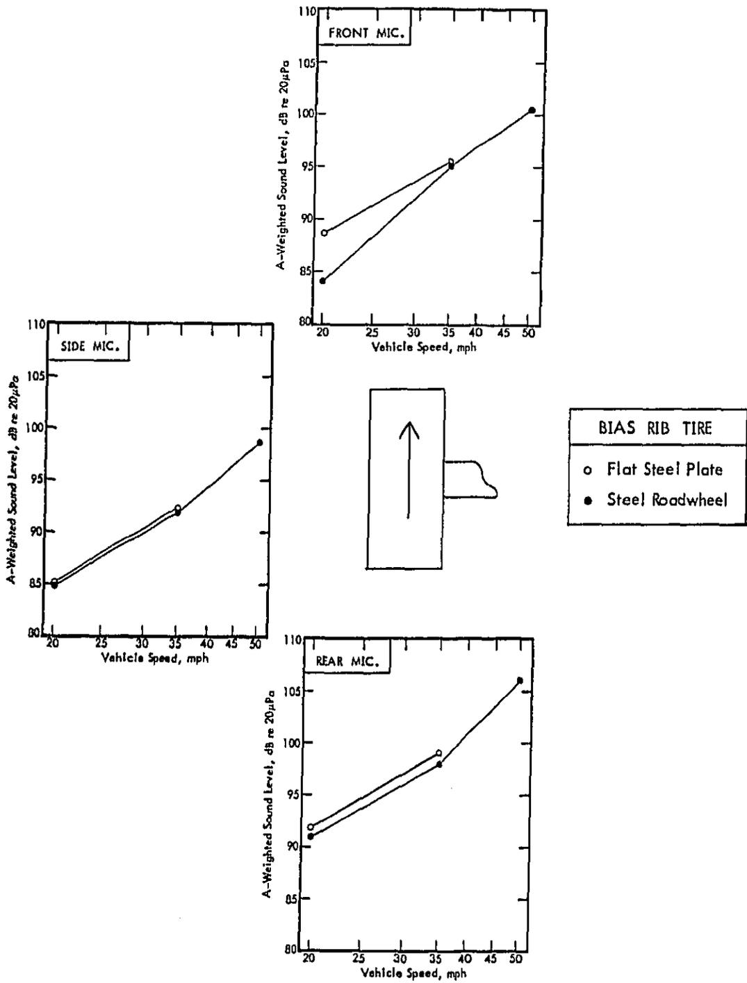
Figure 44. A-Weighted Sound Level Versus Vehicle Speed as a Function of Surface Curvature for Bias Rib Tire.
