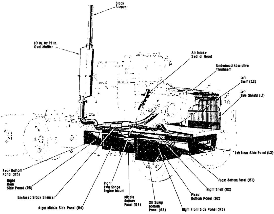
FIG. 21. THE MACK R686 WITH NOISE CONTROL TREATMENTS.
