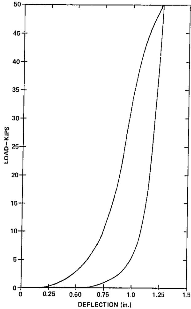
FIG. 46. LOAD/DEFLECTION CURVE FOR THE MACK TWO-STAGE MOUNT COMPONENTS ILLUSTRATED IN FIGS. 44 AND 45.
