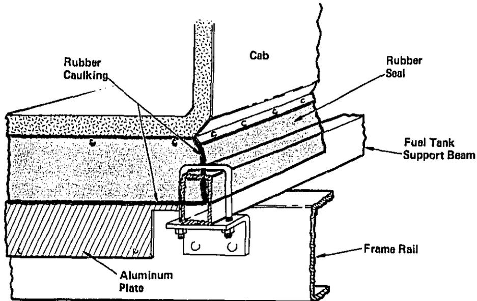
FIG. 32. CAB GAP SHIELD.
