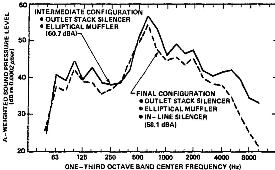
FIG. 17. NOISE SPECTRA AT 50 FT ESTIMATED FROM NEAR MICROPHONE MEASUREMENTS (FIG. 15) AND A TRANSFER FUNCTION (FIG. 16).
