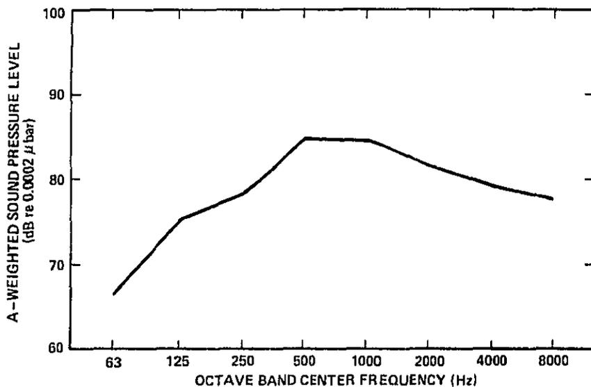
FIG. 13. PEAK OCTAVE BAND LEVELS MEASURED DURING LABORATORY RUNUP TESTS.
