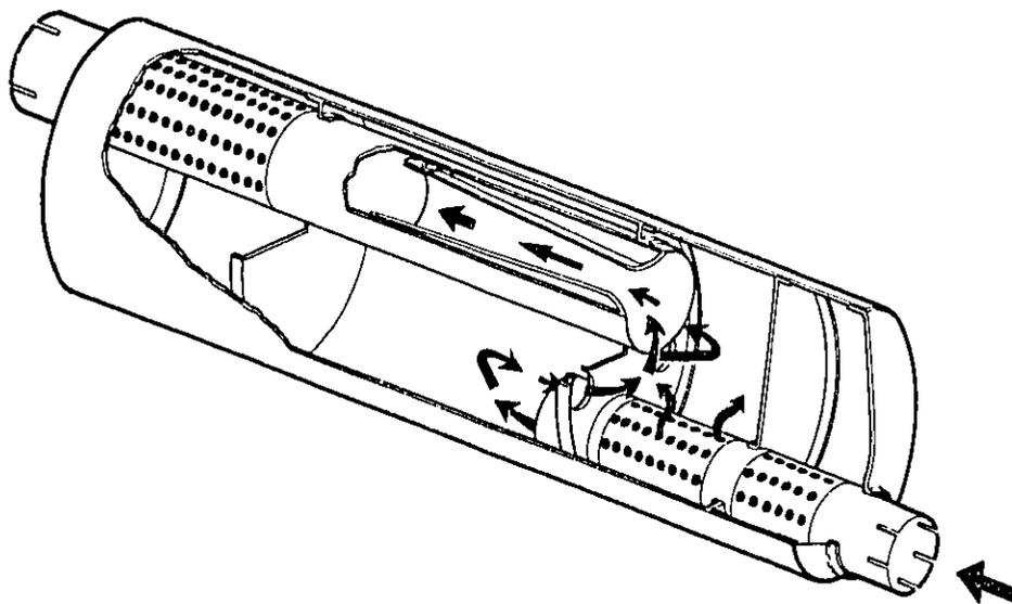
FIG. 10. CUTAWAY VIEW OF 10- x 15-IN. ELLIPTICAL MUFFLER.
