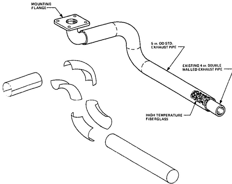
**FIG. 19. ENCLOSED EXHAUST PIPE.**
