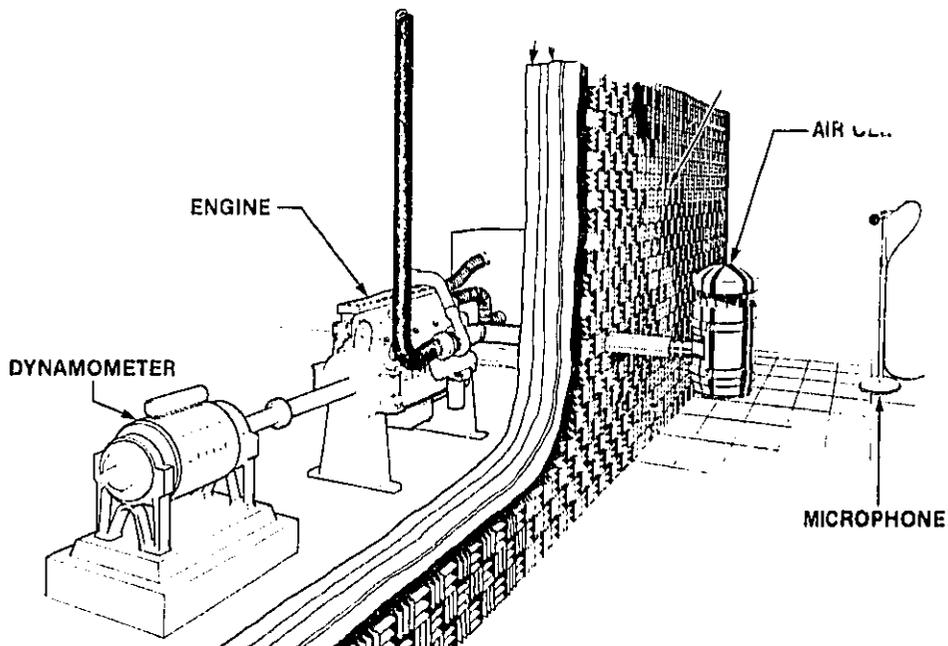
FIG. 7. EXPERIMENTAL CONFIGURATION FOR INTAKE NOISE MEASUREMENT.
