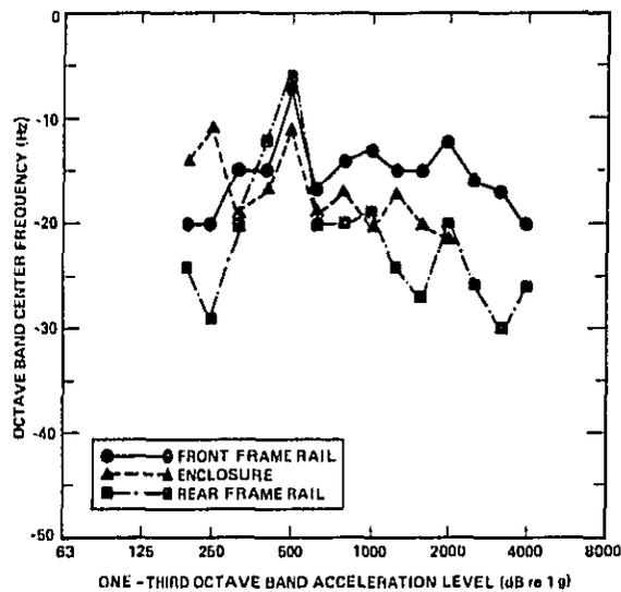
FIG. C.2. VIBRATION LEVELS ON FRAME RAIL AND ENCLOSURE.
