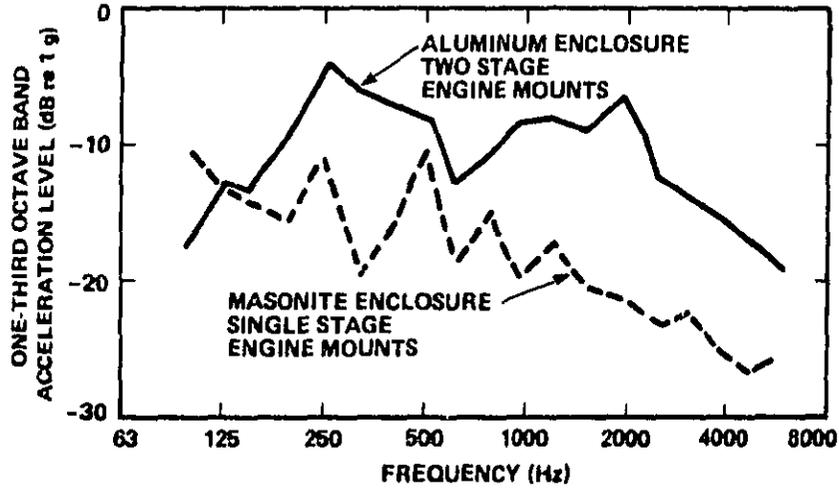
FIG. 37. COMPARISON OF MASONITE AND ALUMINUM ENCLOSURE PANEL VIBRATION WITH THE TRUCK OPERATED ACCORDING TO EPA TEST PROCEDURE - PANEL R3 OPPOSITE THE FRONT AXLE.
