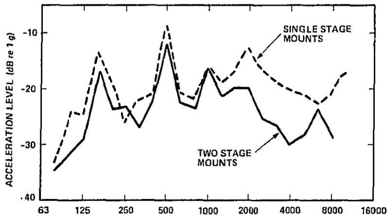
FIG. 41. CHANGE IN AFT FRAME RAIL VIBRATION DUE TO INSTALLATION OF TWO-STAGE ENGINE MOUNTS.
