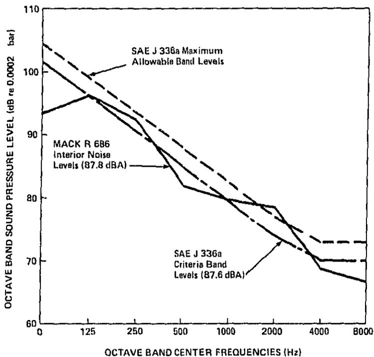
FIG. 42. INTERIOR NOISE LEVELS COMPARED WITH SAE J336a CRITERIA.
