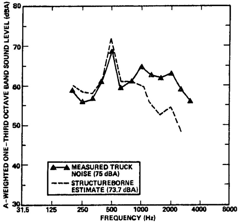
FIG. C.3. COMPARISON OF ESTIMATED STRUCTUREBORNE NOISE AND MEASURED TRUCK NOISE.
