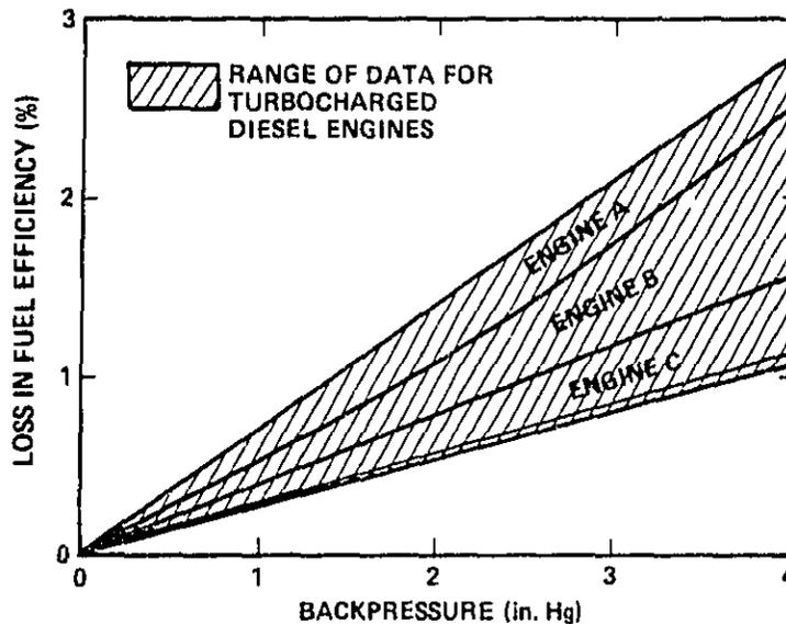
FIG. 43. RELATIONSHIP OF DIESEL ENGINE FUEL EFFICIENCY TO EXHAUST BACKPRESSURE.
