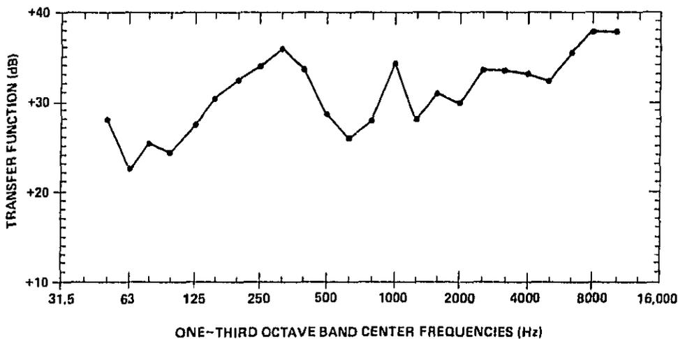
FIG. 16. TRANSFER FUNCTION RELATING NOISE LEVEL AT 18 IN. FROM EXHAUST OUTLET TO LEVEL AT 50 FT.
