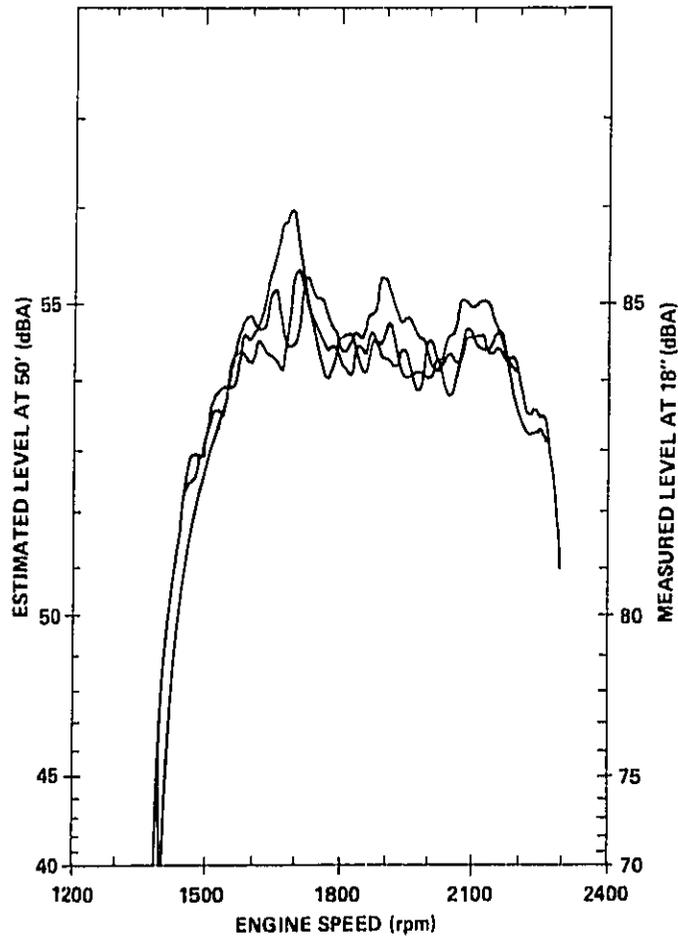
FIG. 12. NOISE LEVELS FOR THE EXHAUST SYSTEM MEASURED DURING THREE RUNUP TESTS.
