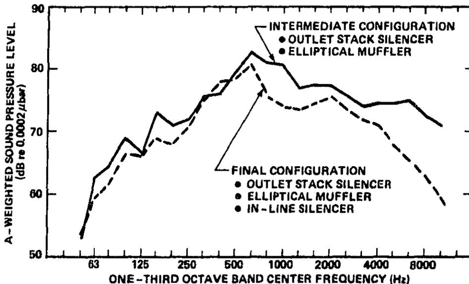
FIG. 15. NOISE LEVELS MEASURED 18 IN. FROM EXHAUST OUTLET DURING ACCELERATION PASSBY TEST.
