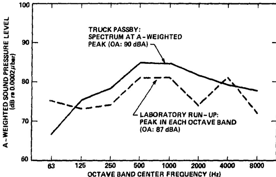
FIG. 18. COMPARISON OF LABORATORY RUNUP AND TRUCK PASSBY LEVELS MEASURED 18 IN. FROM EXHAUST OUTLET.
