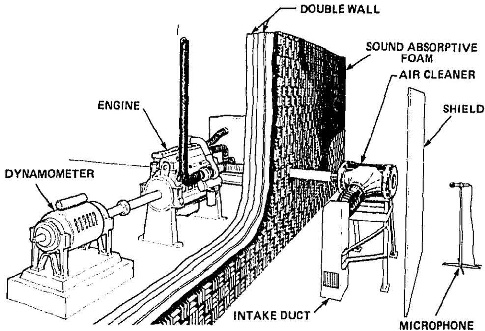
FIG. 4. EXPERIMENTAL CONFIGURATION FOR INTAKE NOISE MEASUREMENT.
