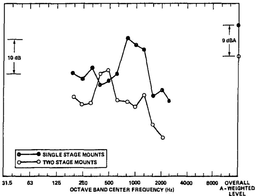
FIG. B.2. ANALYTICAL ESTIMATE OF THE CHANGE WITH A-WEIGHTED ONE-THIRD OCTAVE BAND.
