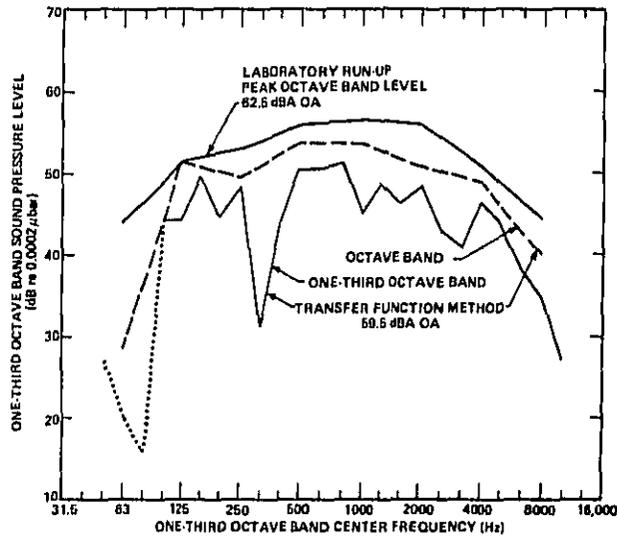
FIG. 10. ESTIMATED EXHAUST NOISE SPECTRA AT 50 FT. (Data includes a 2-dBA correction for the presence of dual exhaust lines.)
