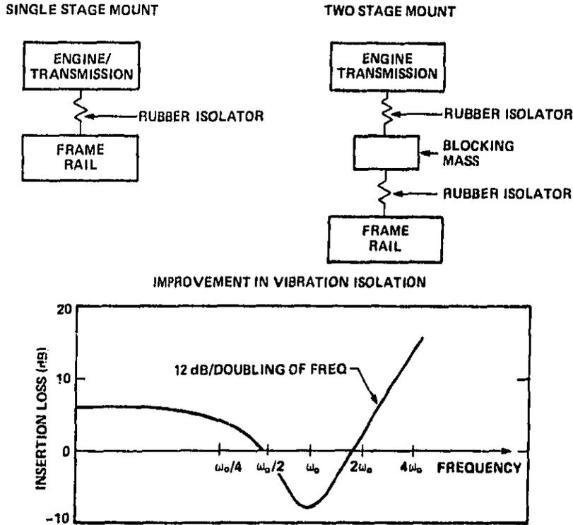
FIG. 22. SCHEMATIC ILLUSTRATION OF SINGLE AND TWO-STAGE ENGINE MOUNTS.
