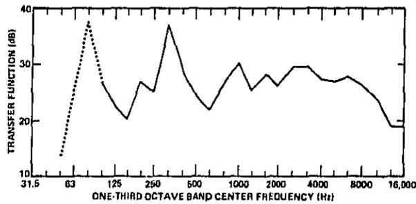
FIG. 11. TRANSFER FUNCTION FOR IH F-4370 EXHAUST.
