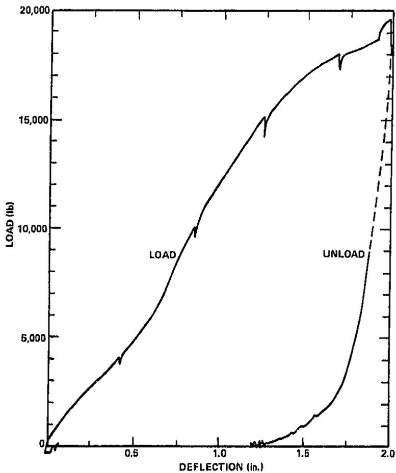
FIG. 27. FORCE DEFLECTION CURVE FOR THE TWO-STAGE ENGINE MOUNT.
