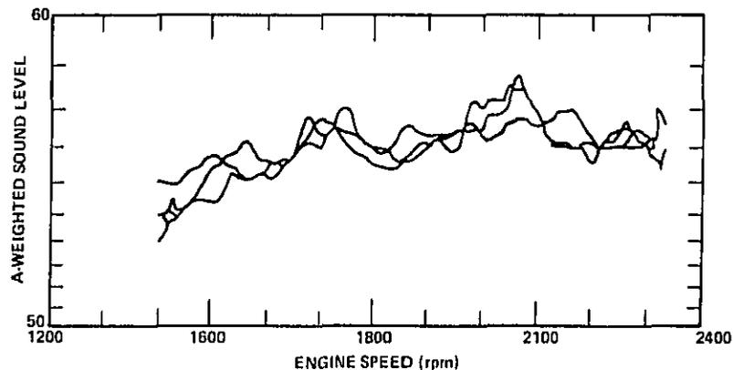
FIG. 9. EXHAUST SYSTEM NOISE LEVELS DURING RUNUP TESTS.
