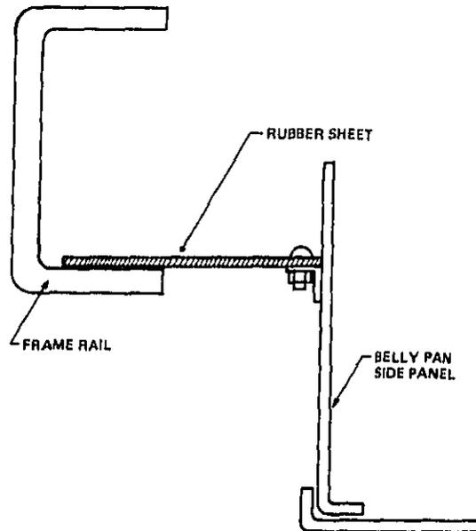
FIG. 21. SEALING ARRANGEMENT FOR FORWARD HALF OF BELLYPAN AT FRAME RAIL.
