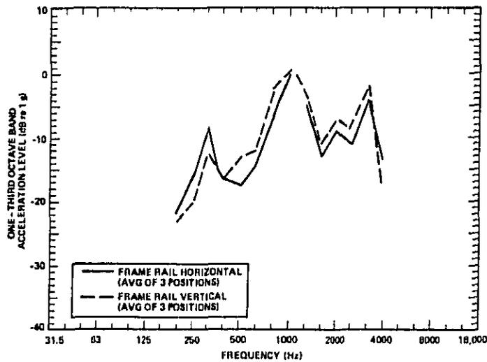
FIG. C.2. ONE-THIRD OCTAVE BAND ACCELERATION LEVELS ON FRAME RAIL.
