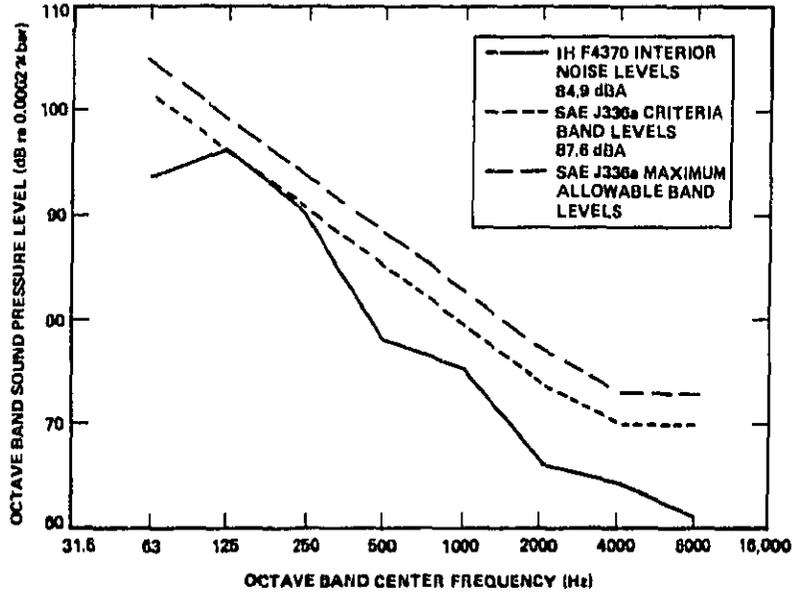
FIG. 29. TRUCK INTERIOR NOISE LEVELS MEASURED ACCORDING TO THE SAE J336a TEST PROCEDURE.
