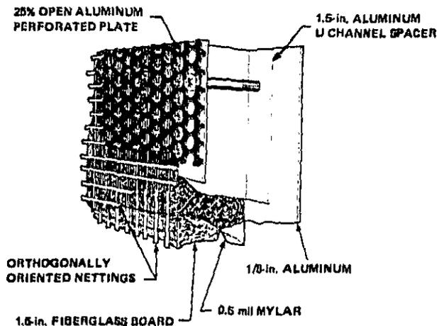
FIG. 13. DRAWING OF MYLAR-WRAPPED SOUND ABSORPTIVE TREATMENT.
