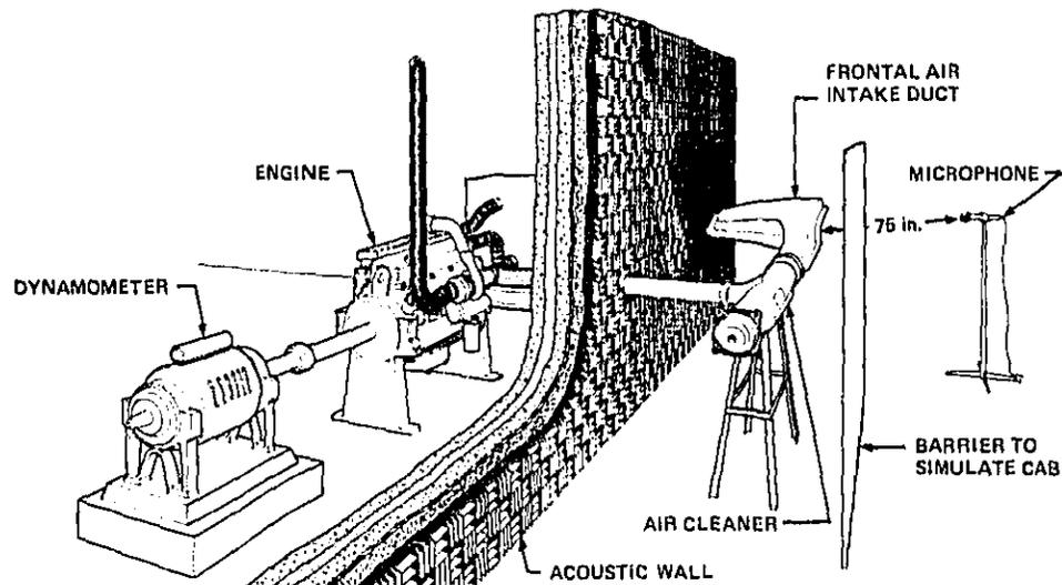
FIG. 5. EXPERIMENTAL CONFIGURATION FOR INTAKE NOISE MEASUREMENT.
