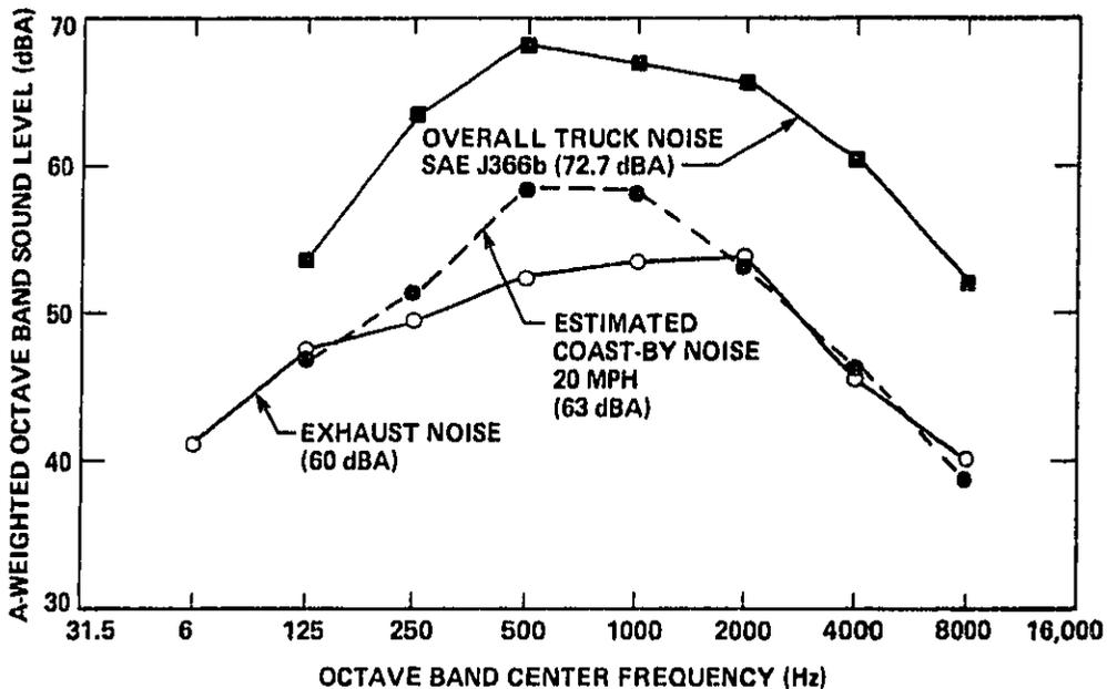
FIG. 10. ESTIMATED A-WEIGHTED OCTAVE BAND SPECTRUM OF EXHAUST NOISE: COMPARISON WITH OVERALL VEHICLE AND COASTBY SPECTRA.
