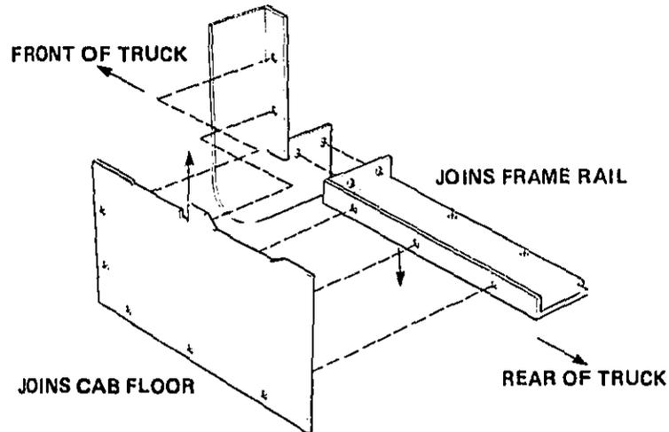
FIG. 17. ASSEMBLY DRAWING OF LEFT GAP SHIELD.
