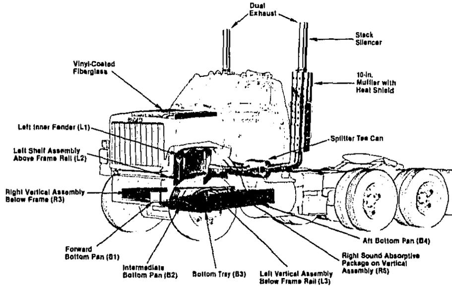
FIG. 11. NOISE CONTROL TREATMENTS INSTALLED ON GMC BRIGADIER.
