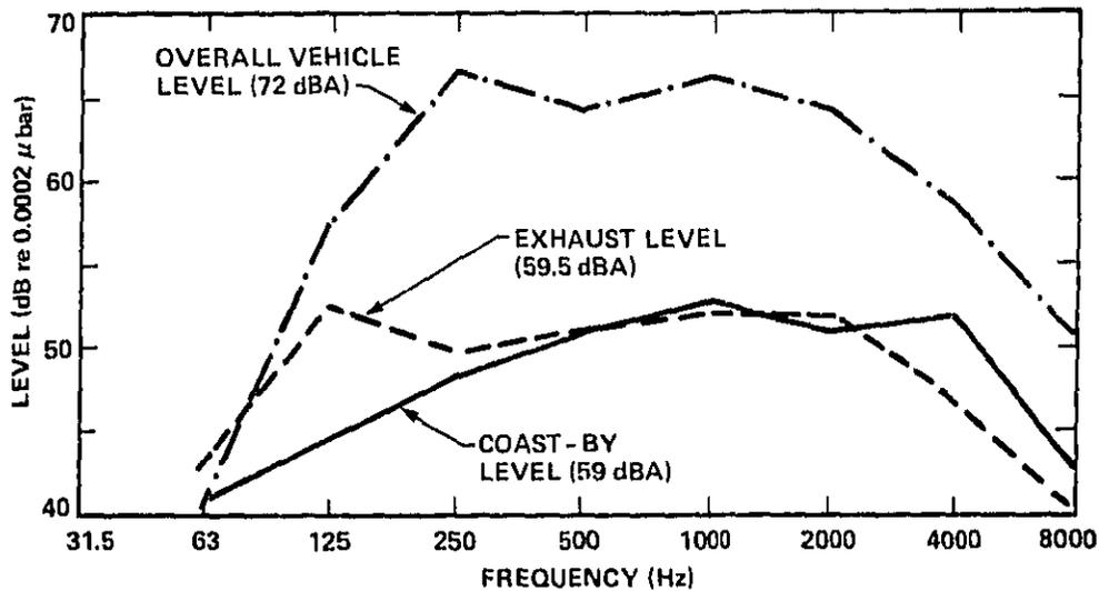
FIG. 8. ESTIMATED A-WEIGHTED OCTAVE BAND SPECTRUM OF EXHAUST NOISE: COMPARISON WITH OVERALL VEHICLE AND COASTBY SPECTRA.
