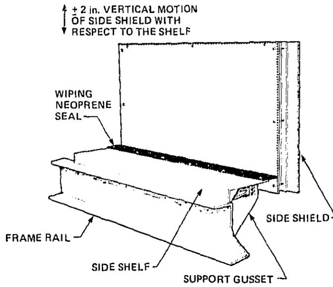
FIG. 15. CROSS SECTION DETAIL OF SHELF AND JUNCTION WITH SIDE SHIELD.
