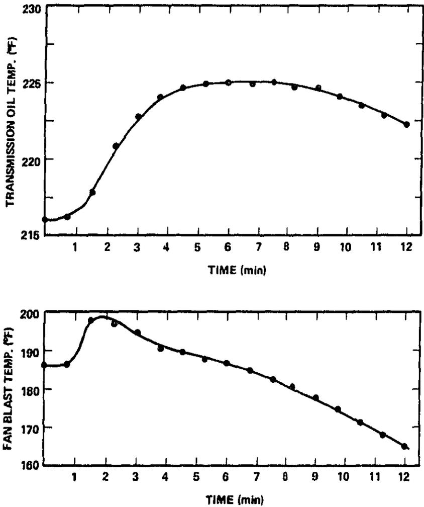
FIG. 24. TRANSMISSION OIL AND FAN BLAST TEMPERATURES. (ENGINE LOAD WAS ELIMINATED DURING THE FIRST MINUTE.)
