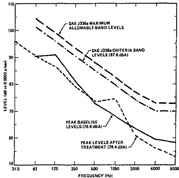
FIG. 22. INTERIOR NOISE LEVELS COMPARED WITH SAE J336a CRITERIA.
