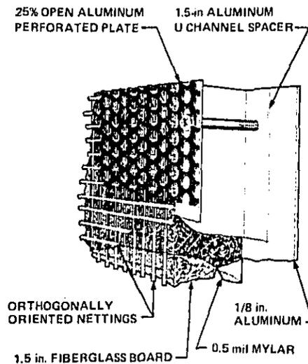
**FIG. 12. DRAWING OF MYLAR-WRAPPED SOUND ABSORPTIVE TREATMENT.**
