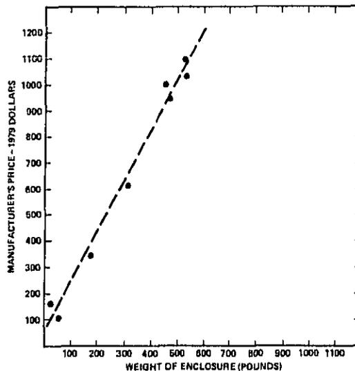
FIG. 25. RELATIONSHIP BETWEEN ENCLOSURE WEIGHT AND MANUFACTURER'S PRICE.
