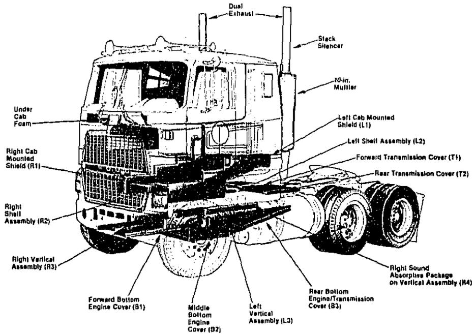
FIG. 9. NOISE CONTROL TREATMENTS INSTALLED ON FORD CLT 9000.
