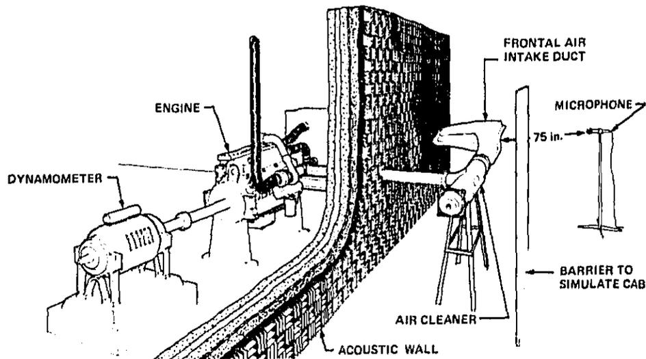
FIG. 4. EXPERIMENTAL CONFIGURATION FOR INTAKE NOISE MEASUREMENT.
