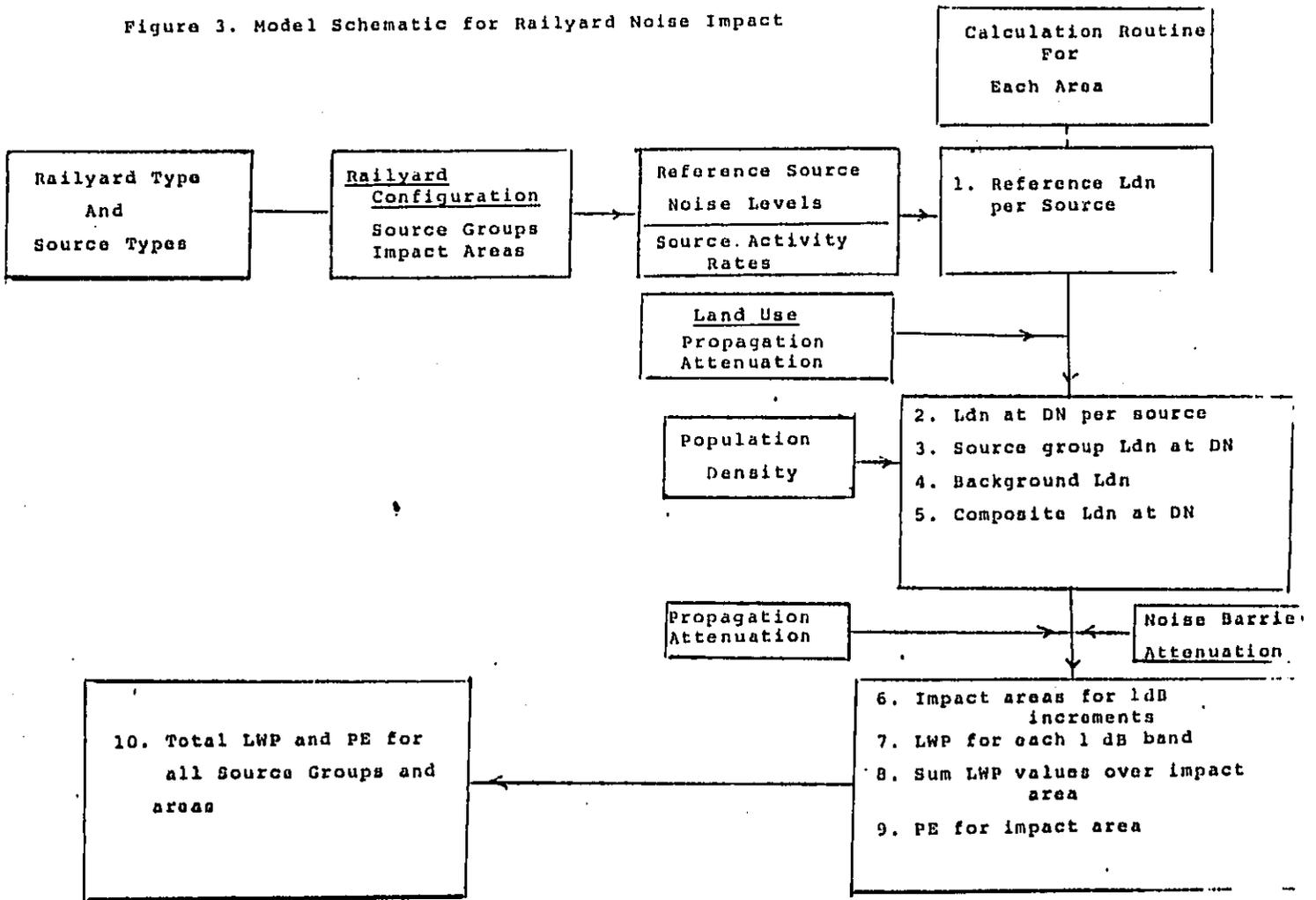
source group, and combined with the background noise level. In the baseline case (no barrier wall) the composite noise level is then propagated across the impact area integrating the Ldn vs. distance relationship with the impact weighting factors and population density in 1dB increments to obtain the PE and LWP values. This procedure is followed for all impact areas and sources (groups) at the railyard, and the resulting PE and LWP values are summed to obtain the total impact.
