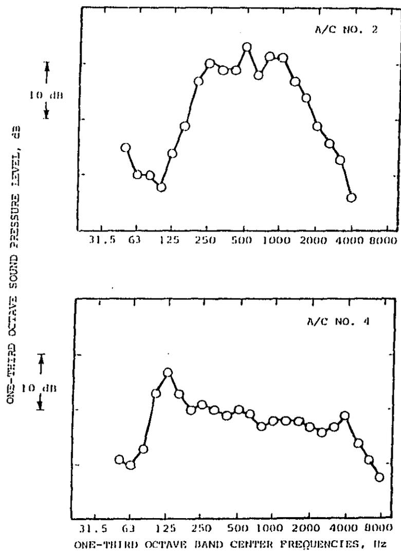
FIGURE 2-2. TYPICAL ACOUSTIC SPECTRA FOR TURBOJET (GA) AIRCRAFT
