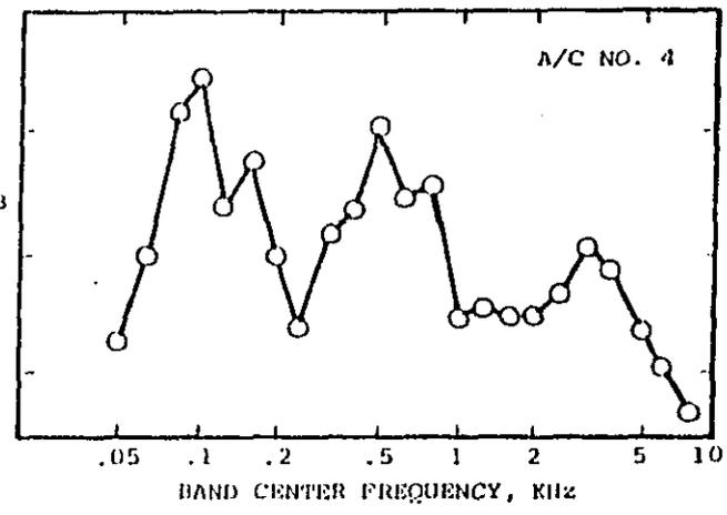
FIGURE 2-1. TYPICAL ACOUSTIC SPECTRA FOR PROPELLER-DRIVEN (GA) AIRCRAFT
