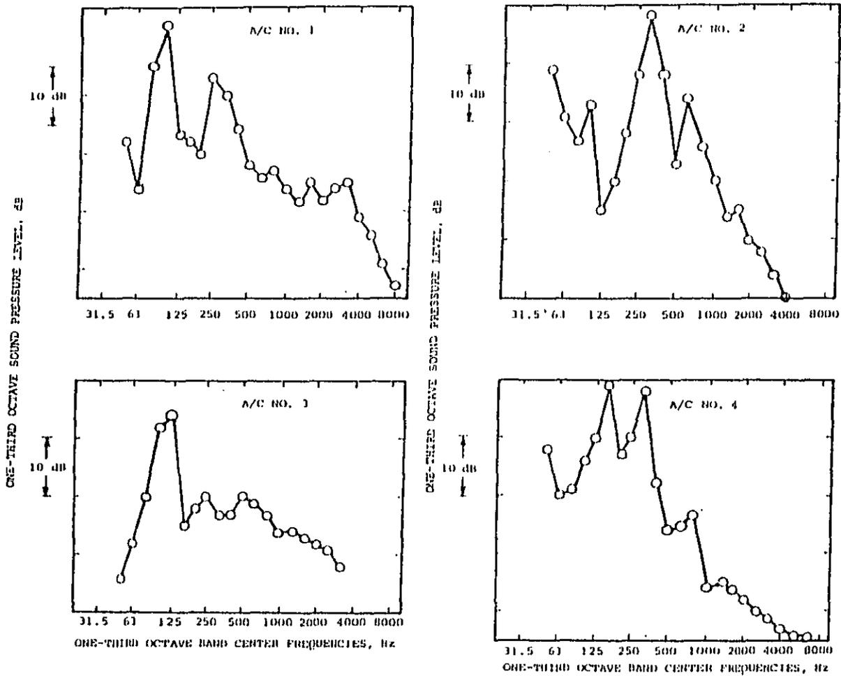
Figure 2-3. TYPICAL ACOUSTICAL SPECTRA FOR HELICOPTER (GA) AIRCRAFT
