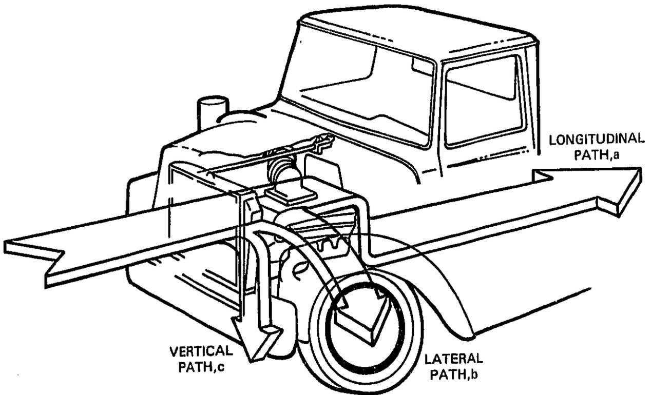
FIGURE 2.1. ENGINE COMPARTMENT FLOW PATHS
