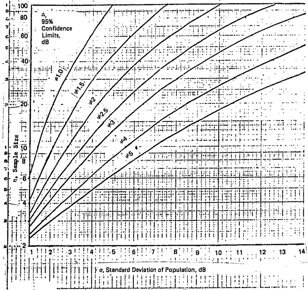
Figure B-2. Sample Size Needed to Measure a Population Mean with 95 Percent Confidence
