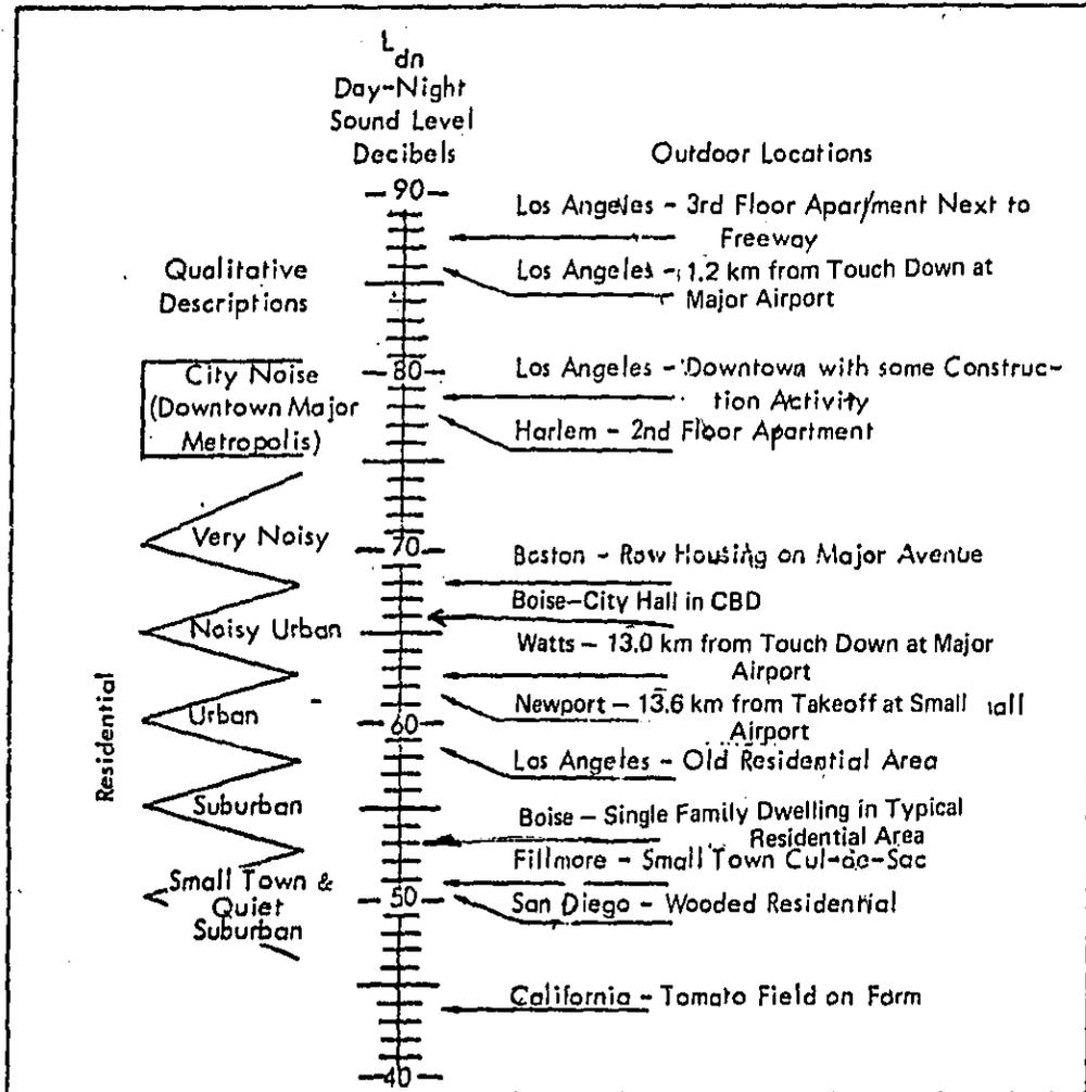
Figure 3-2. Outdoor Day-Night Average Sound Level, L<sub>dn</sub> - in Decibels at Various Locations
