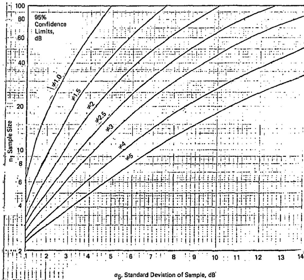
Figure A-1. Required Sample Size for Various 95 Percent Confidence Limits On Population Standard Deviation
