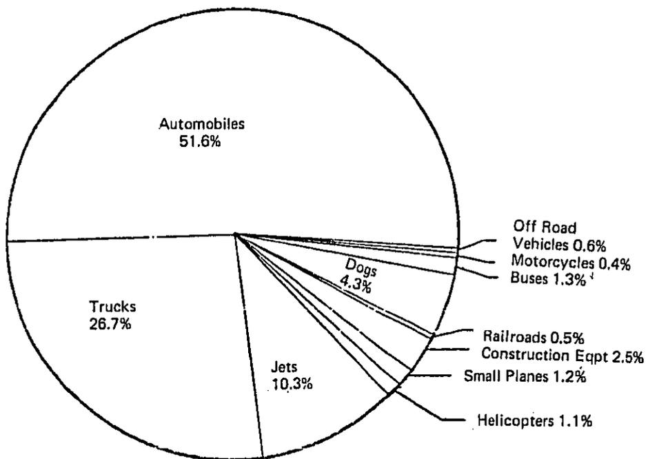
42 Readings of A-Weighted Sound Level Over 80 dB
