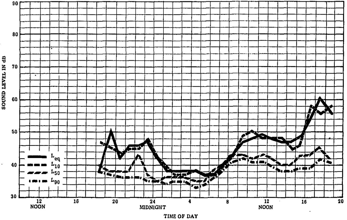
Figure 5-4. Hourly Noise Levels in a Typical Residential Site Near Open Foothills Near Eastern City Limits of Boise
