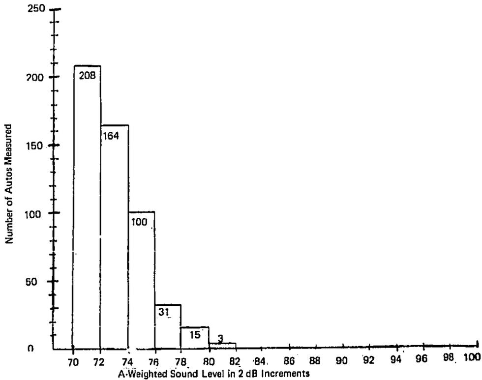
Figure 5-8. Distribution of Automobile Sound Levels Above 70 dB Measured at Various Community Locations in Boise
