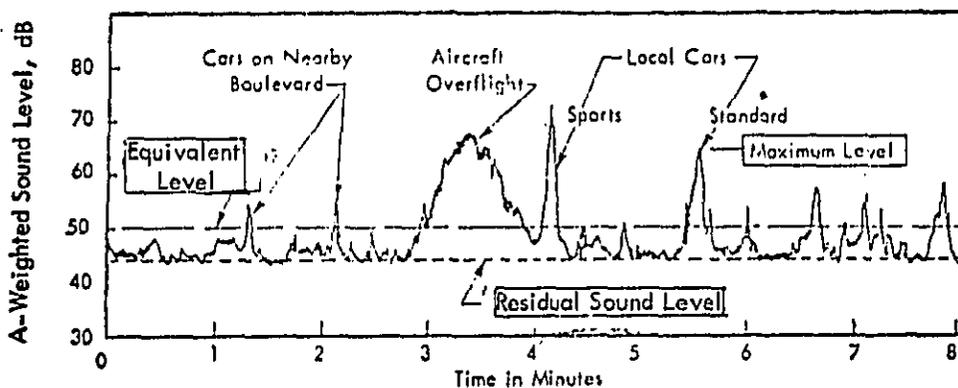
Figure 3-1. Eight Minute Sample of Typical Fluctuating Sound Level in Residential Area Showing Maximum, Equivalent, and Residual Sound Levels for the Period
