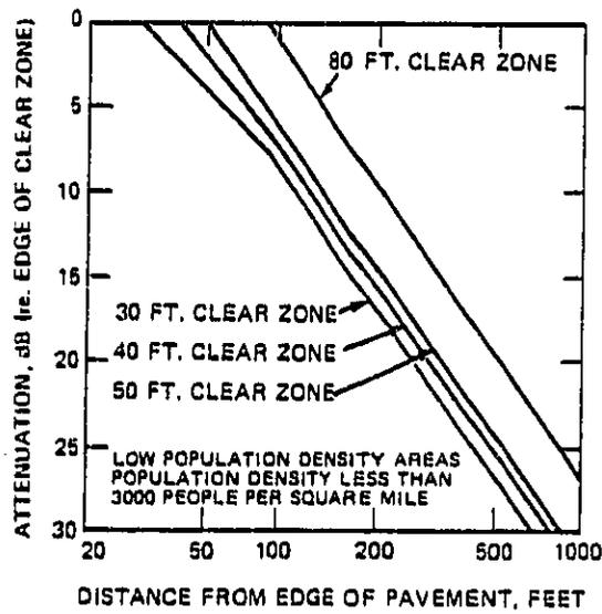
FIGURE F-8 SOUND LEVEL ATTENUATION CURVES: POINT SOURCE
