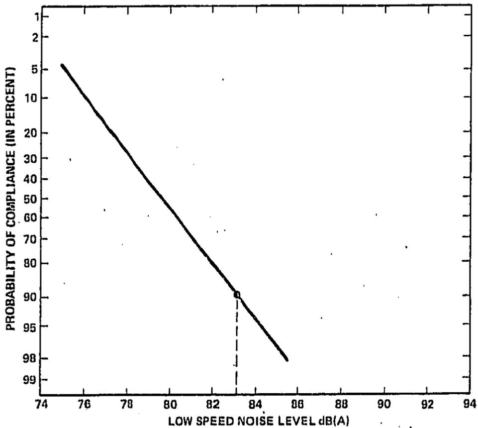
FIG. 10. ESTIMATED PROBABILITY OF POST-1978 MEDIUM AND HEAVY TRUCK COMPLIANCE AS A FUNCTION OF LOW-SPEED NOISE LEVEL\*.
