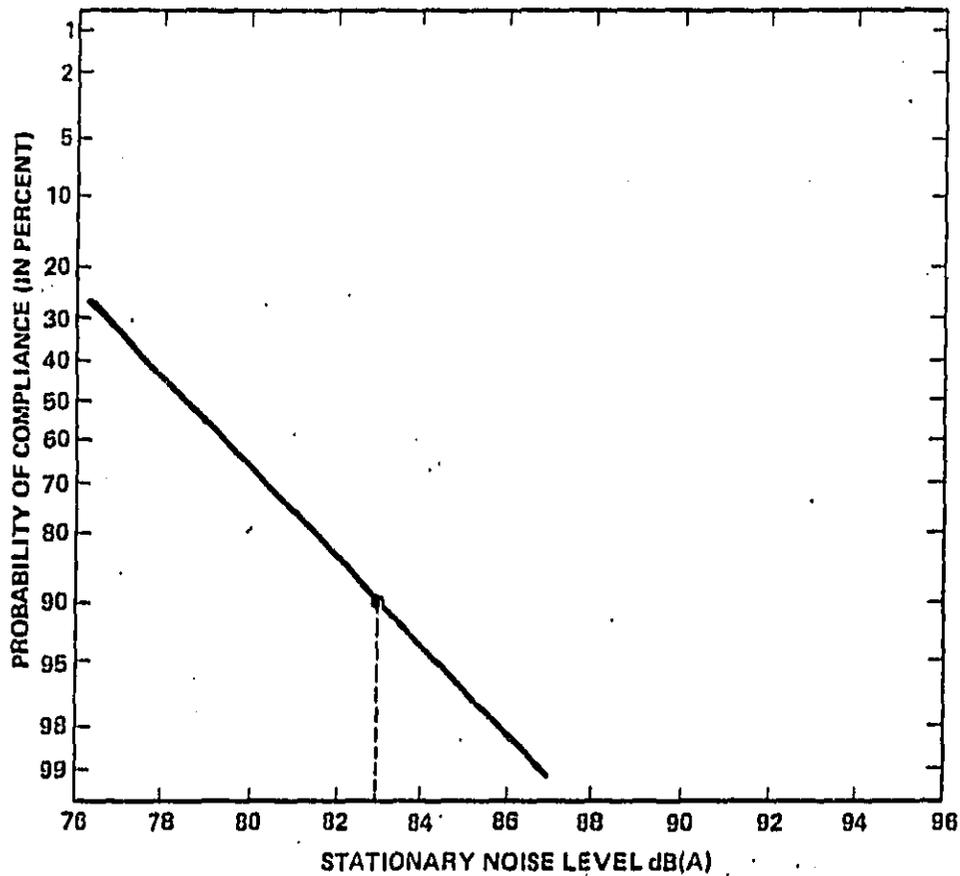
FIG. 11. ESTIMATED PROBABILITY OF POST-1978 MEDIUM AND HEAVY TRUCK COMPLIANCE AS A FUNCTION OF STATIONARY TEST NOISE LEVEL\*.
