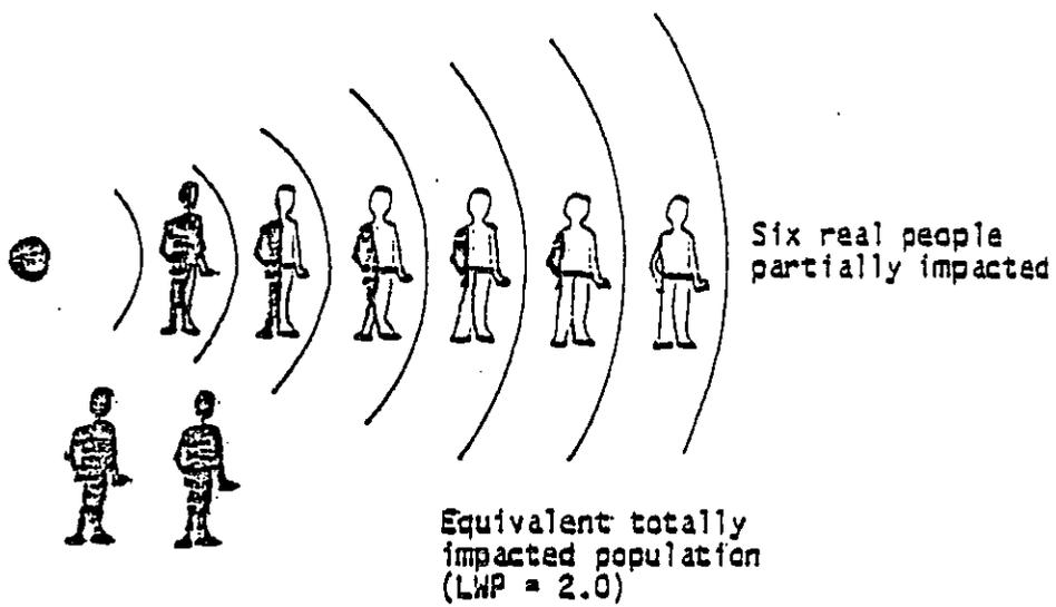
Figure 4.1 LEVEL-WEIGHTED POPULATION: A METHOD TO ACCOUNT FOR THE EXTENT AND SEVERITY OF NOISE IMPACT
