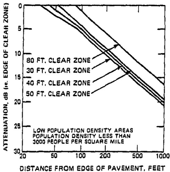
FIGURE F-7 SOUND LEVEL ATTENUATION CURVES: LINE SOURCE
