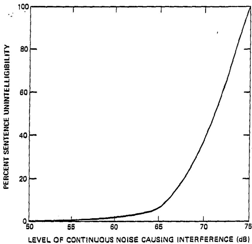
FIGURE F-10 WEIGHTING FUNCTION FOR INDOOR SPEECH INTERFERENCE (RELAXED CONVERSATION AT GREATER THAN 1 METER SEPARATION, 45 dB BACKGROUND IN THE ABSENCE OF INTERFERING NOISE)
