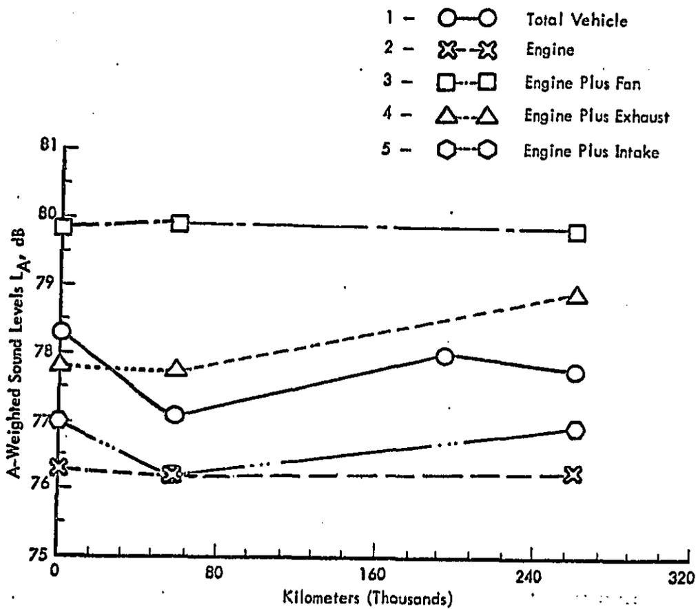
Figure 5-42. Component Exterior Noise Level Versus Cumulative Kilometers
