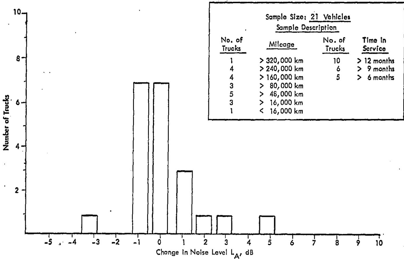
Figure 5-36. Change in Noise Levels with Time as Measured by Stationary (IMI) Testing
