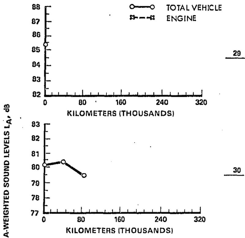
Figure 5-35. Vehicle Exterior Noise Levels versus Cumulative Kilometers
