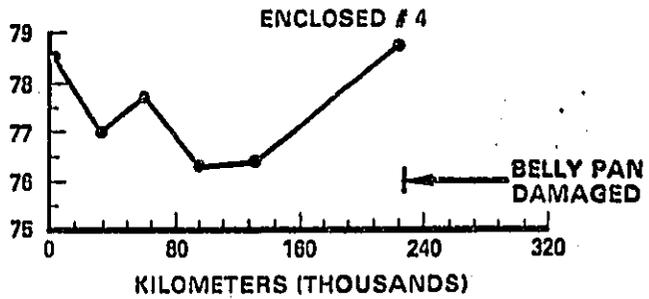
Figure 5-43. Vehicle Exterior Noise Levels versus Cumulative Kilometers
