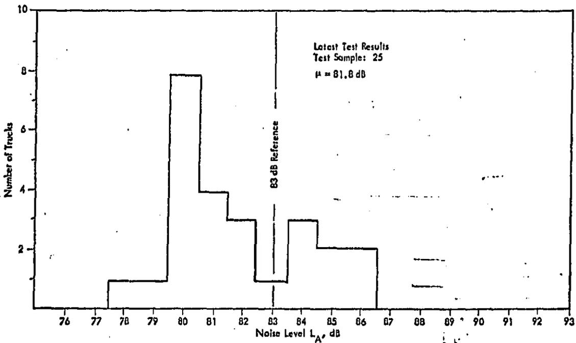
Figure 5-37. Measured Noise Levels Compared to New Truck Regulation (83 dB)
