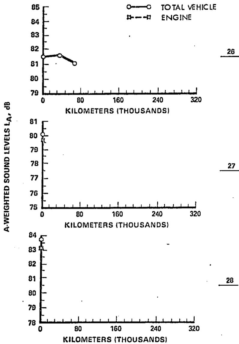
Figure 5-34. Vehicle Exterior Noise Levels versus Cumulative Kilometers
