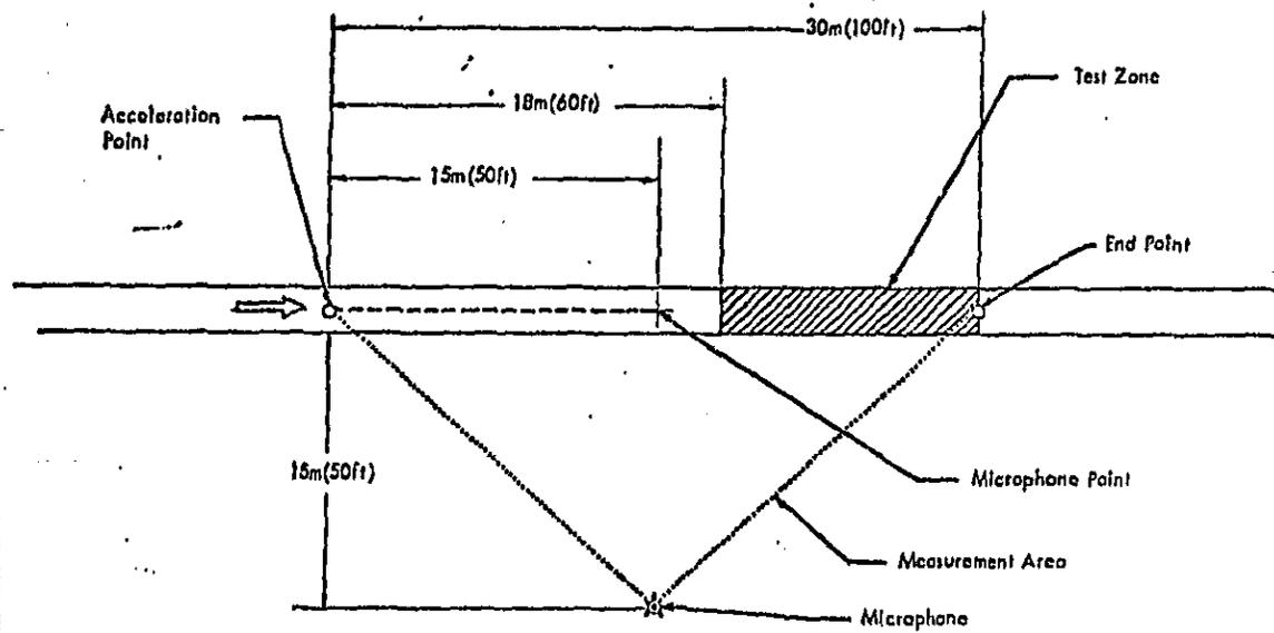
Figure 5-15. Passby Test Site Configuration and Microphone Position
