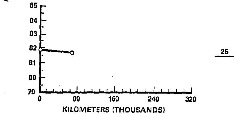
Figure 5-33. Vehicle Exterior Noise Levels versus Cumulative Kilometers
