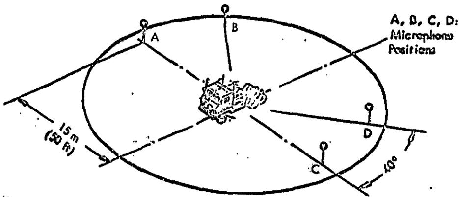
Figure 5-24. Microphone Positions for Stationary Testing
