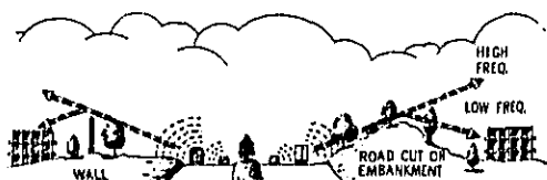
Fig. 5.8. Use of Various Noise Barriers.
