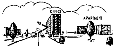
Fig. 5.9. Use of Buildings as Noise Barriers.
