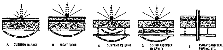
Fig. 7.1. Basic Sound Insulating Floor Constructions.
