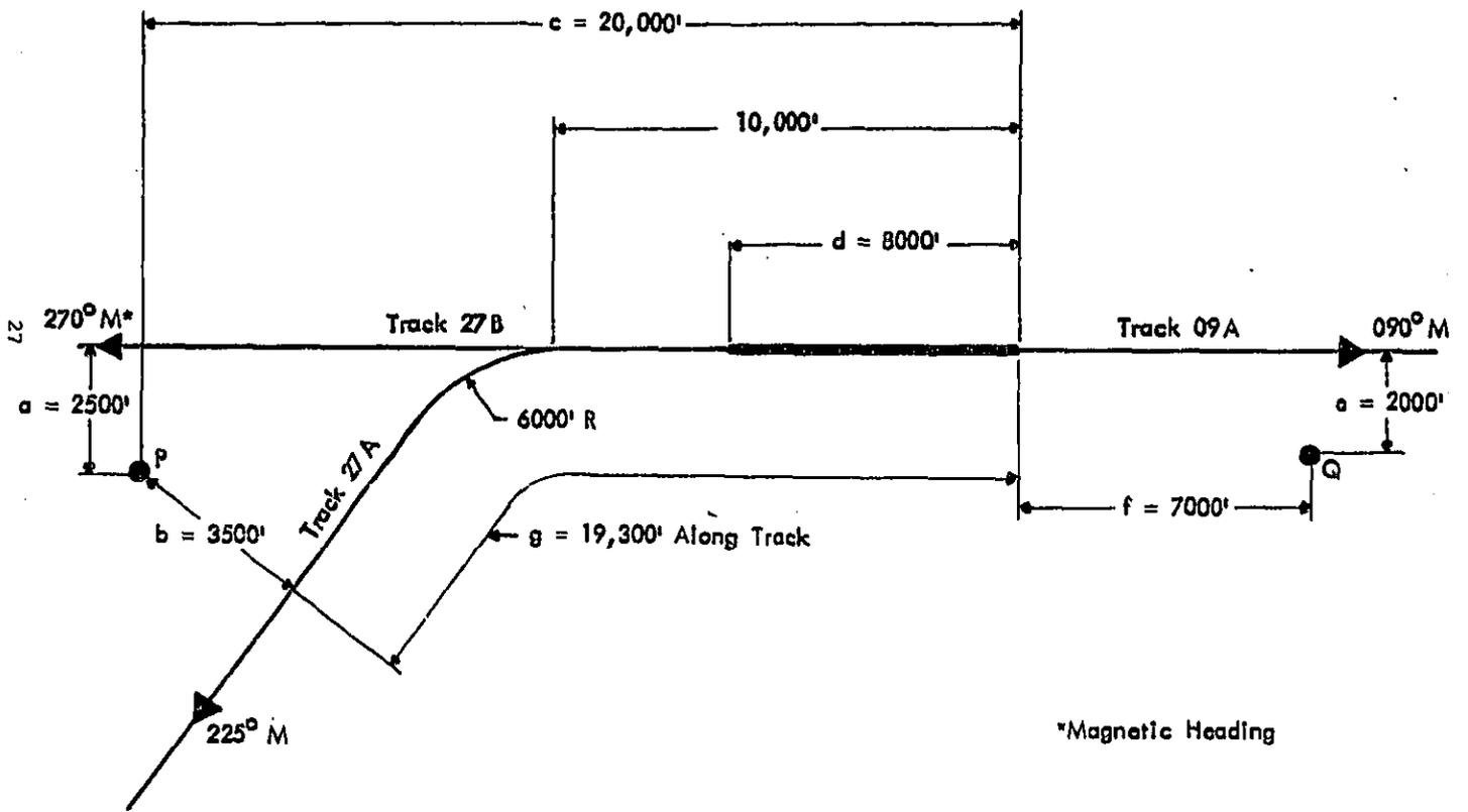
FIGURE 6. EXAMPLE: FLIGHT TRACKS AT MYTHICAL AIRPORT
