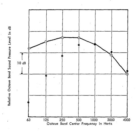
Note: Closed Circles show the corresponding relative A-Weighted octave band sound pressure levels.
