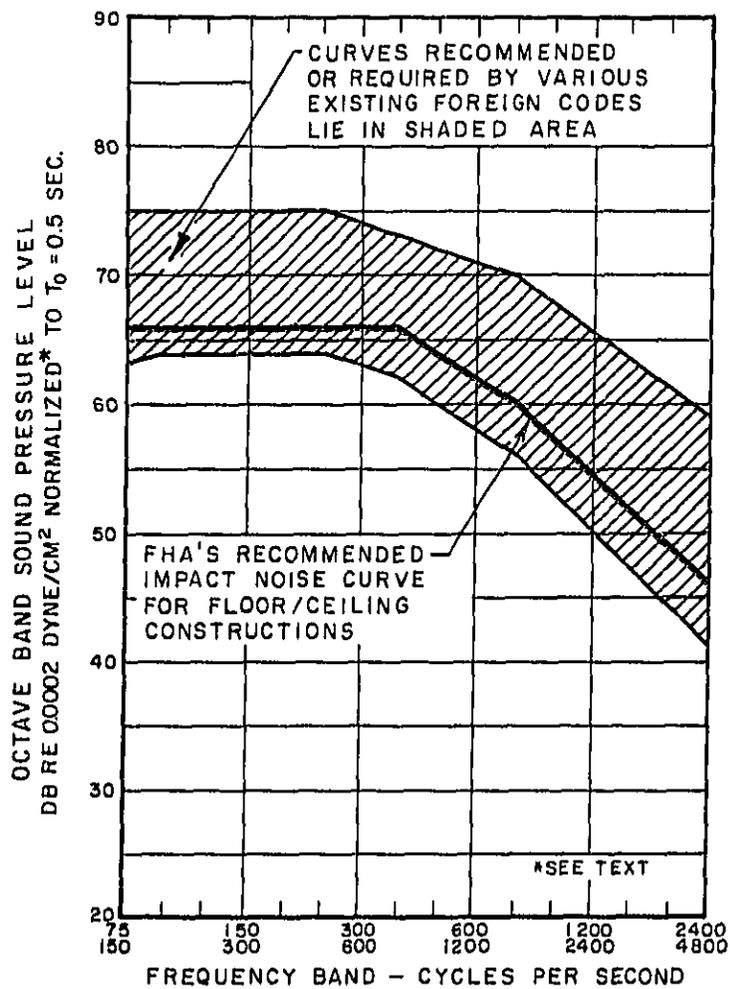
Fig. 1 Field Measurements of Sound Pressure Levels in the room underneath a floor construction on which a standard tapping machine is operating should not exceed this curve by more than the tolerances specified in section III-A-3 of the text.
