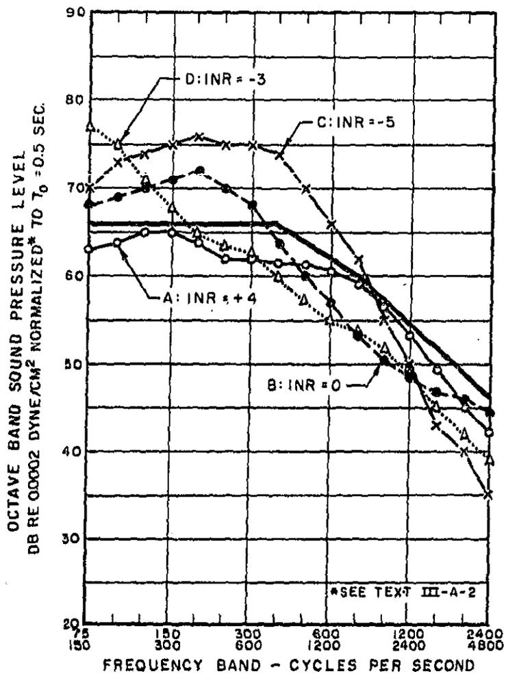
Fig. 2 Single Number Impact Noise Rating. A Replot of the FHA Recommendation Curve with the Measured ISPL of Four Typical Constructions (See Section III-A-4 of the Text).
