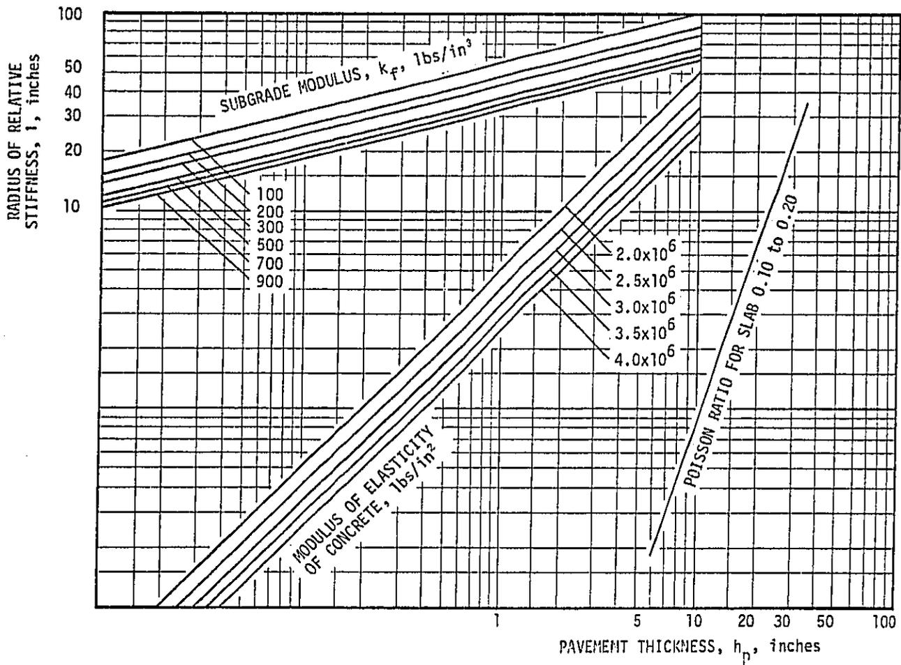
Figure 3-6. DESIGN NOMOGRAPH FOR RADIUS OF RELATIVE STIFFNESS
