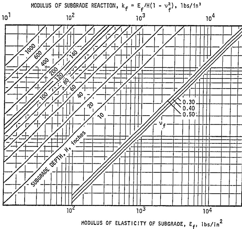
Figure 3-5. DESIGN NOMOGRAPH FOR MODULES OF SUBGRADE REACTION
