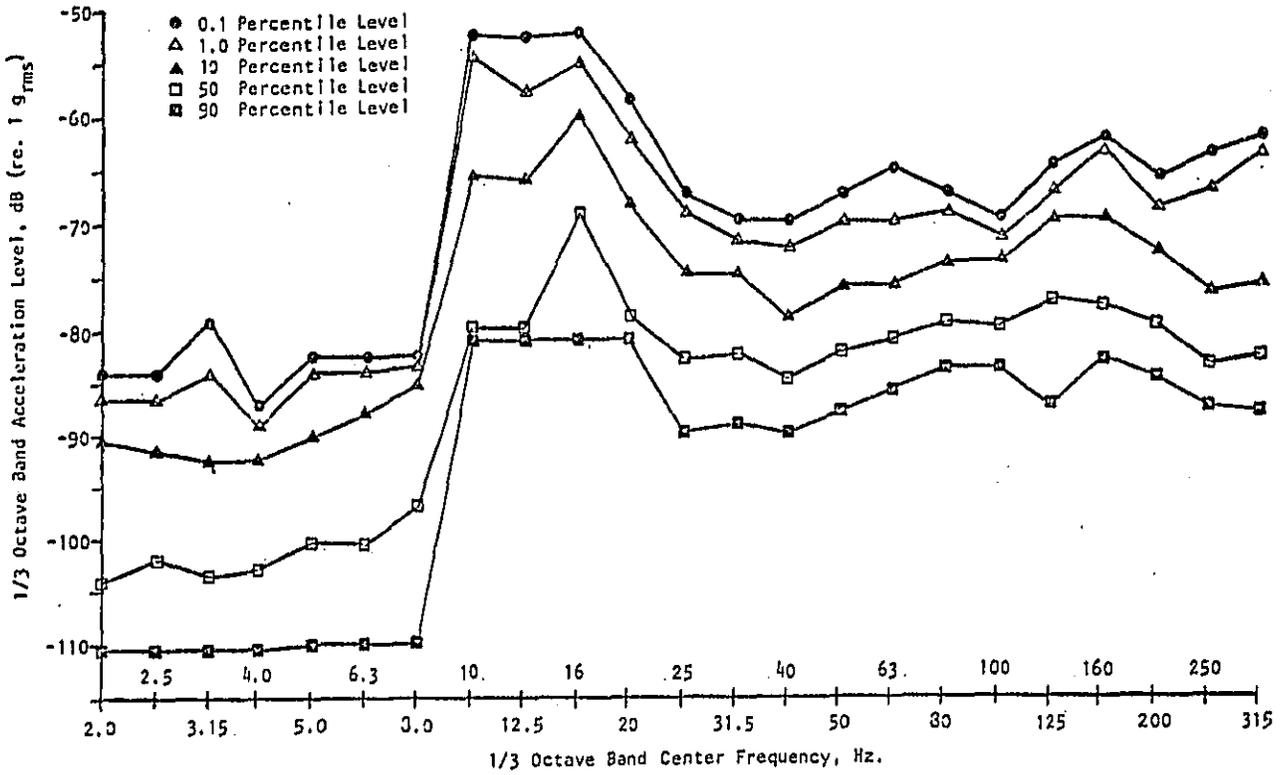
FIGURE 4-9 - THIRD OCTAVE TRAFFIC-INDUCED VIBRATION SPECTRUM:
