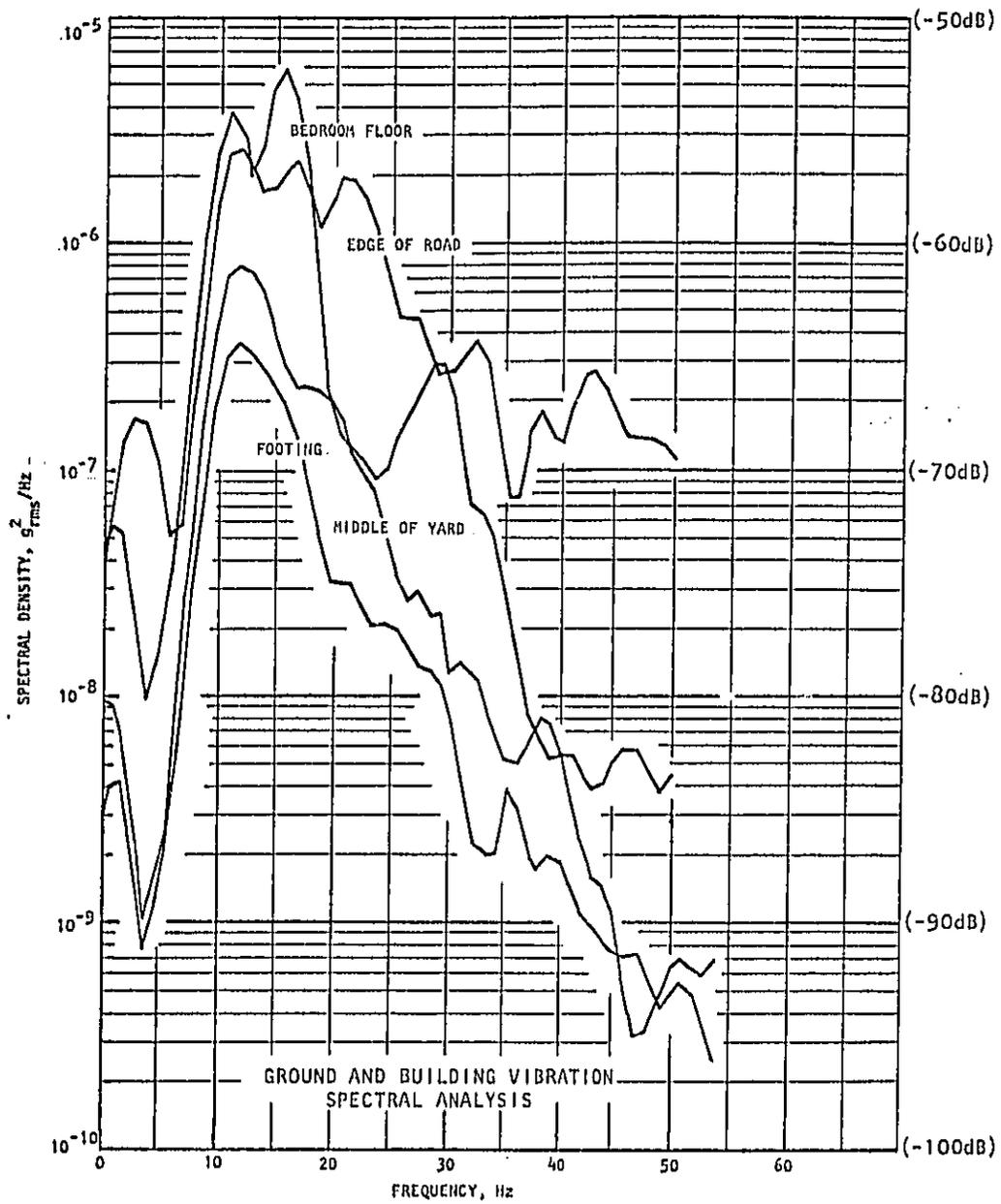
Figure 2-6. GROUND AND BUILDING VIBRATION SPECTRA FOR A BUS PASSING A RESIDENCE
