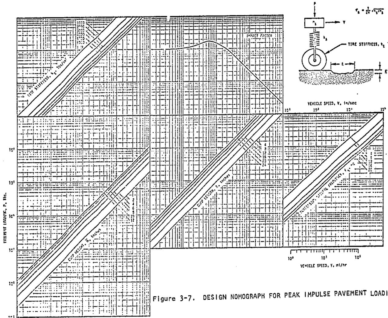
Figure 3-7. DESIGN NOMOGRAPH FOR PEAK IMPULSE PAVEMENT LOADING
