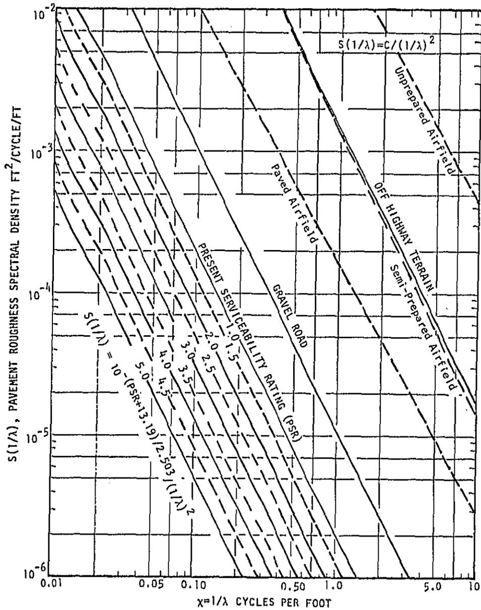
Figure 2-5. PAVEMENT ROUGHNESS POWER SPECTRAL DENSITY FUNCTIONS
