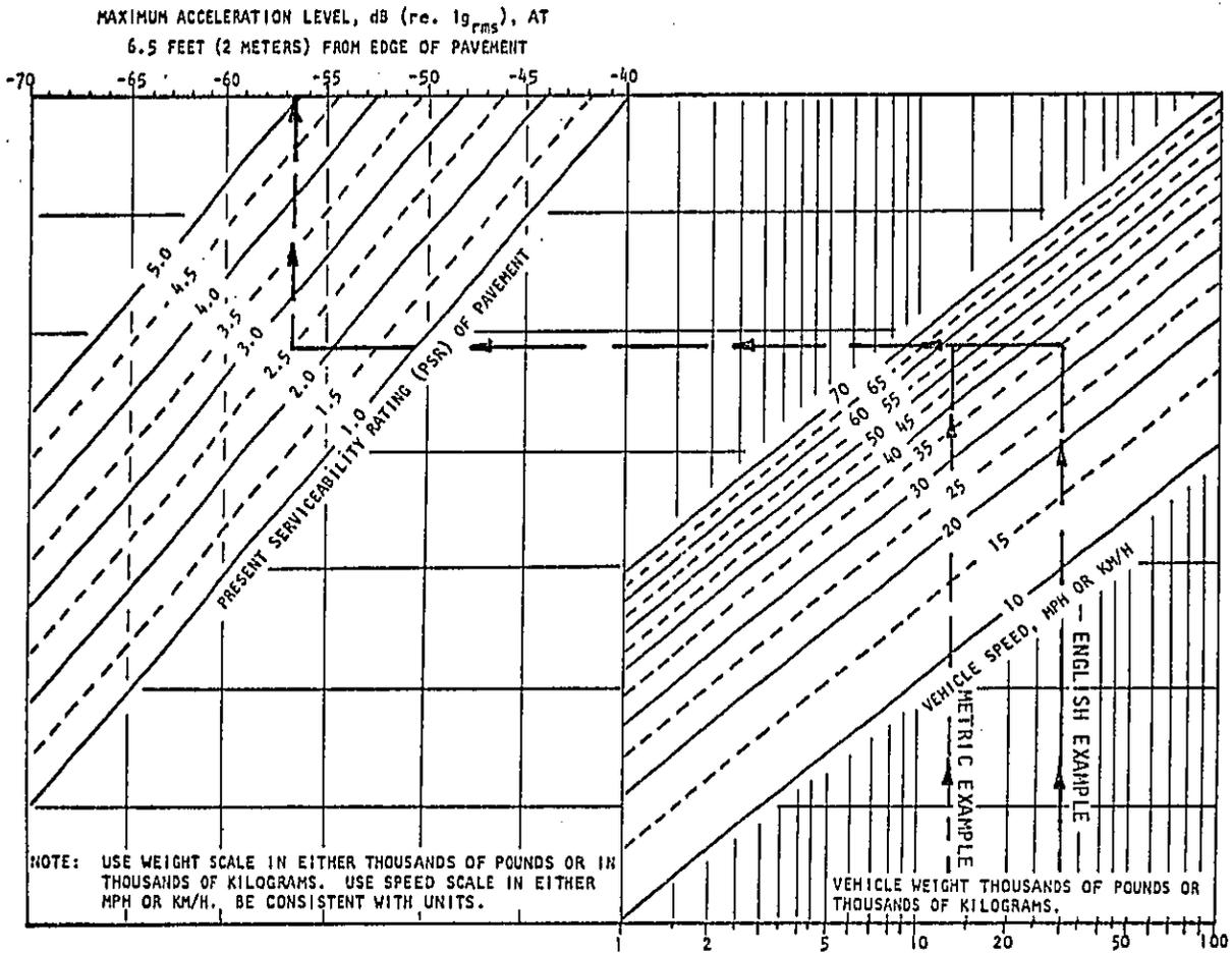
FIGURE 5-1 - EXAMPLE OF USE OF VIBRATION REFERENCE EMISSION LEVEL NOMOGRAPH
