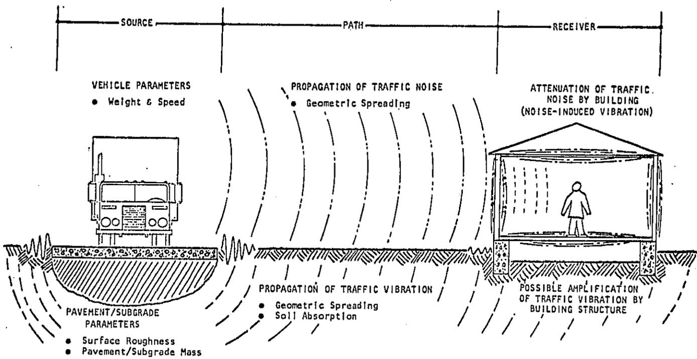
FIGURE 2-2 - SOURCE-PATH-RECEIVER SCENARIO FOR TRAFFIC NOISE AND VIBRATION
