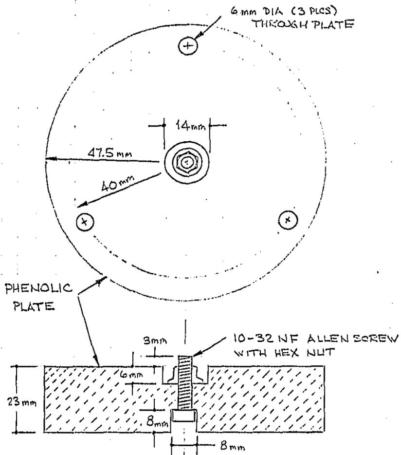
FIGURE 4-6 - ACCELEROMETER SUPPORT PLATE
