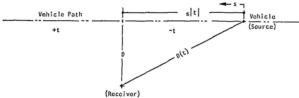
(a) Source-Receiver Geometry: Straight Highway Segment
