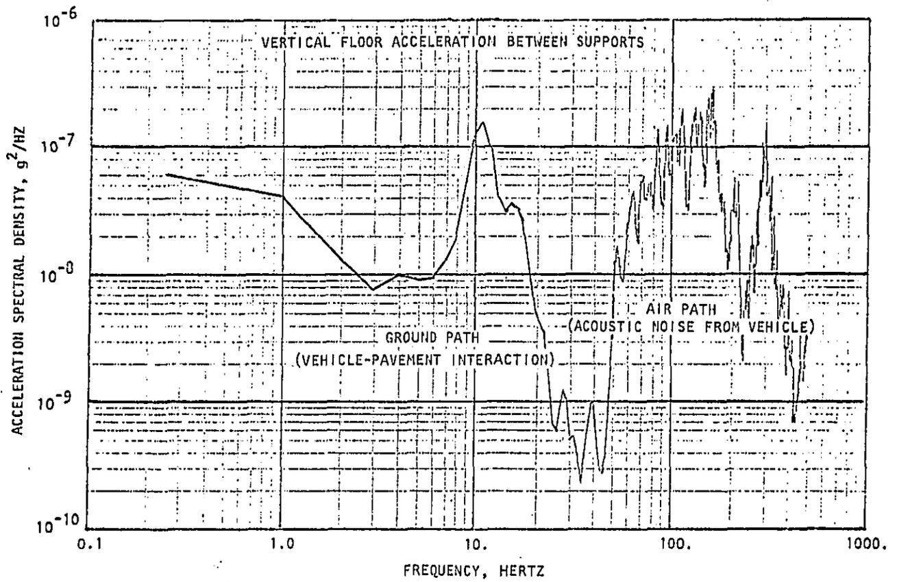
Figure 2-7. BUILDING RESPONSE TO COMBINED TRAFFIC NOISE AND VIBRATION
