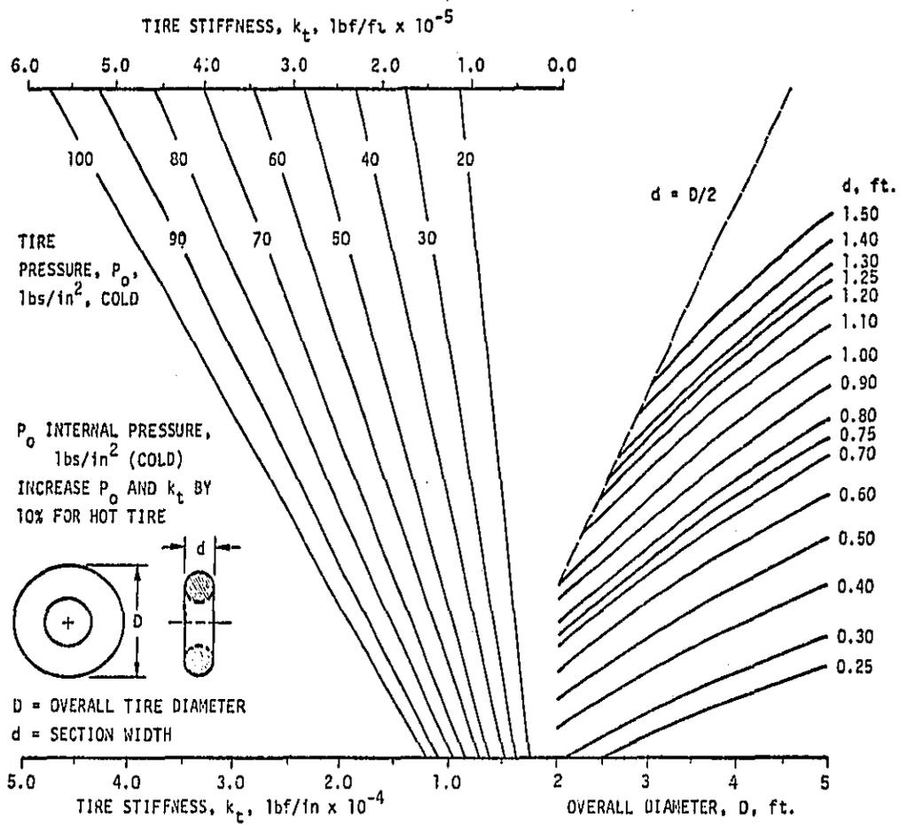
Figure 3-4. DESIGN NOMOGRAPH FOR TIME STIFFNESS
