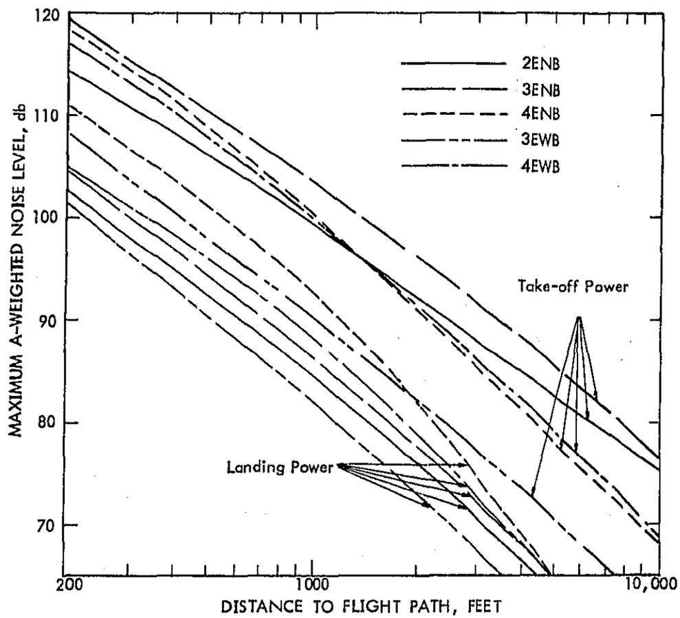
FIGURE 3-1. NOISE LEVELS FOR COMMERCIAL JET AIRCRAFT
