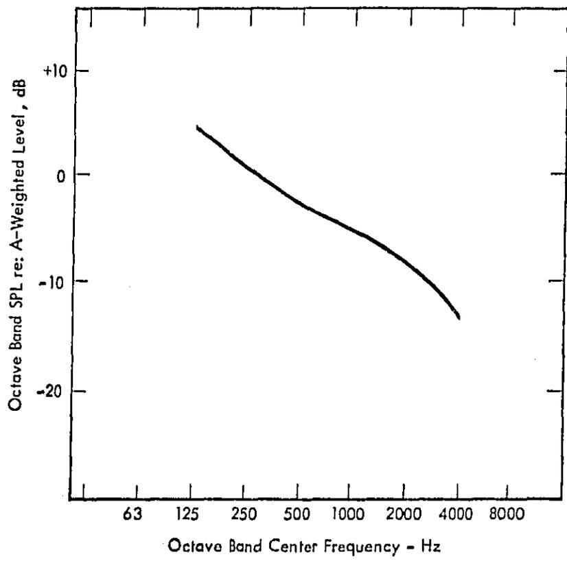
FIGURE B-6. AIRCRAFT NOISE SPECTRUM
