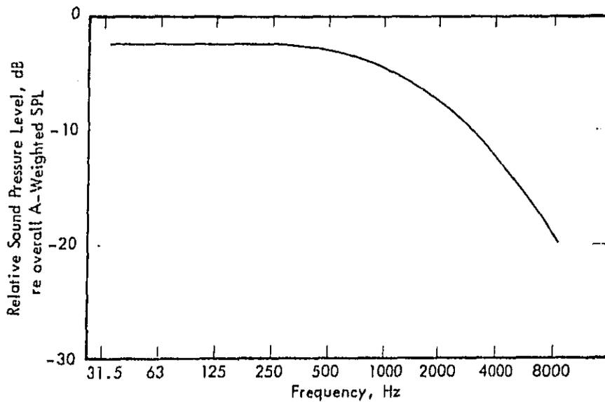
FIGURE B-3. STANDARD HIGHWAY NOISE SPECTRUM
