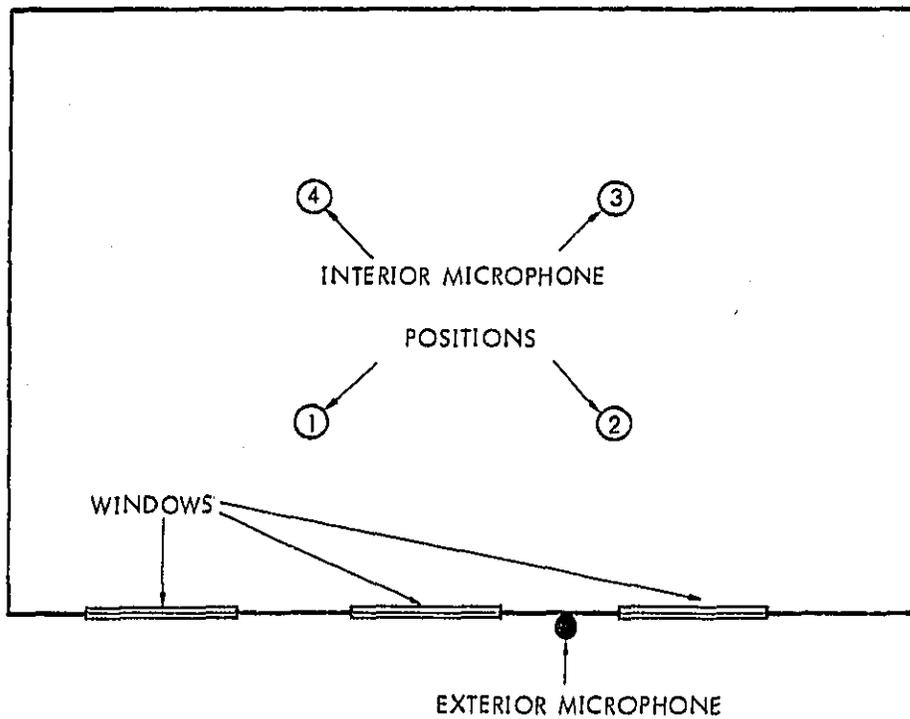
FIGURE 4-1. TYPICAL MICROPHONE ARRANGEMENT FOR NOISE REDUCTION MEASUREMENTS.
