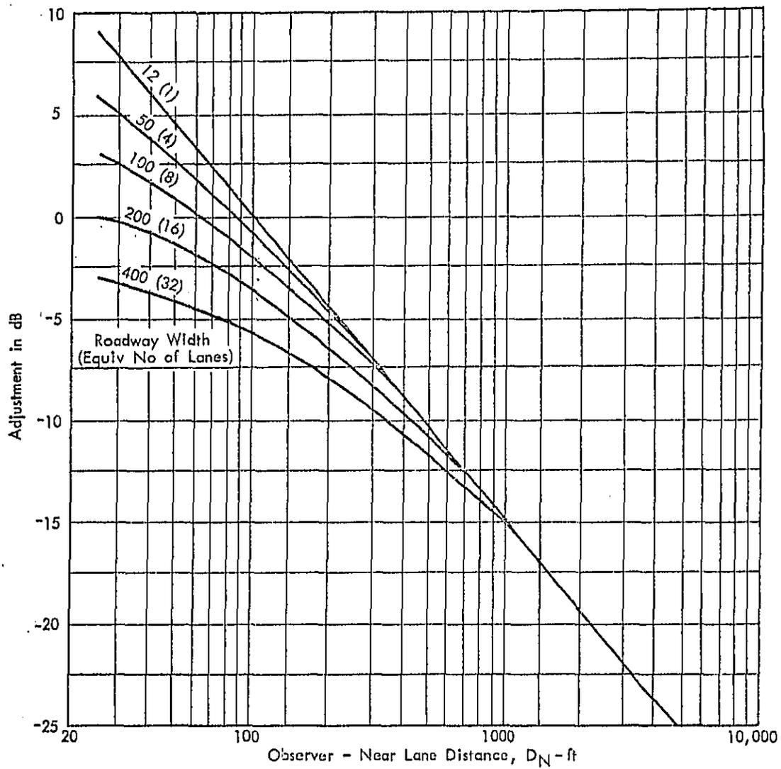
FIGURE B.5 DISTANCE ADJUSTMENT TO ACCOUNT FOR OBSERVER - NEAR LANE DISTANCE AND WIDTH OF ROADWAY
