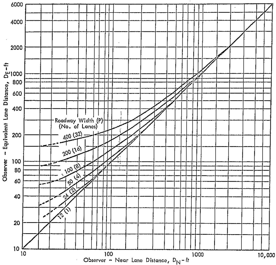
FIGURE B.2 OBSERVER - EQUIVALENT LANE DISTANCE AS FUNCTION OF NEAR LANE DISTANCE AND WIDTH OF ROADWAY
