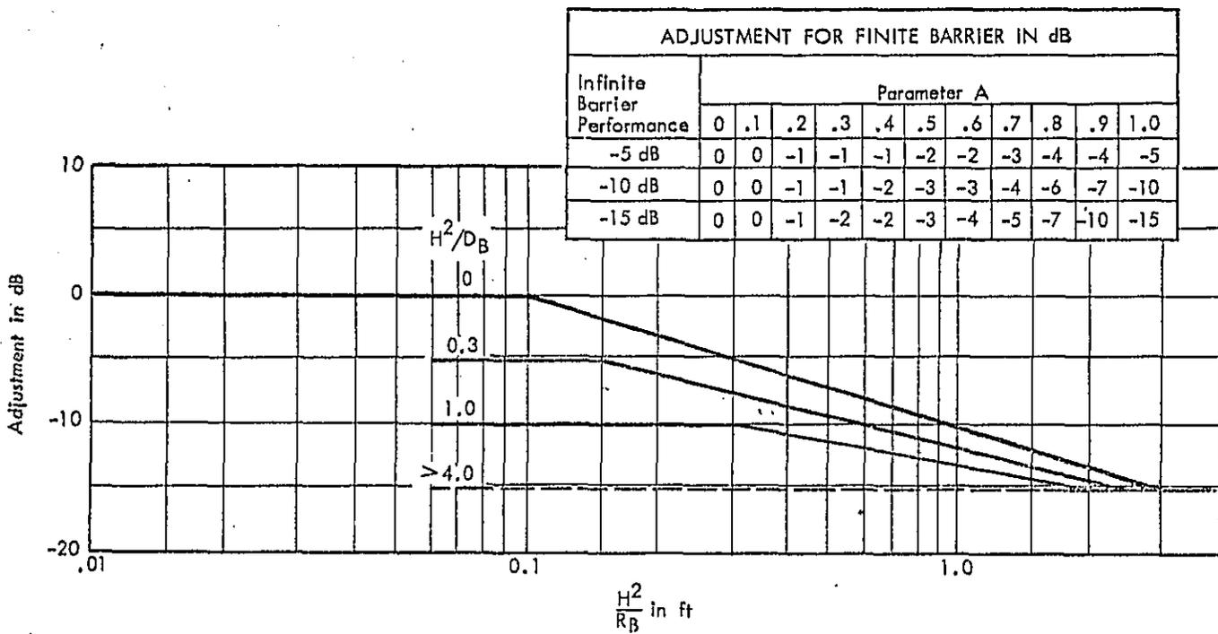
FIGURE B.9 ADJUSTMENT FOR ROAD-SIDE INFINITE BARRIERS
