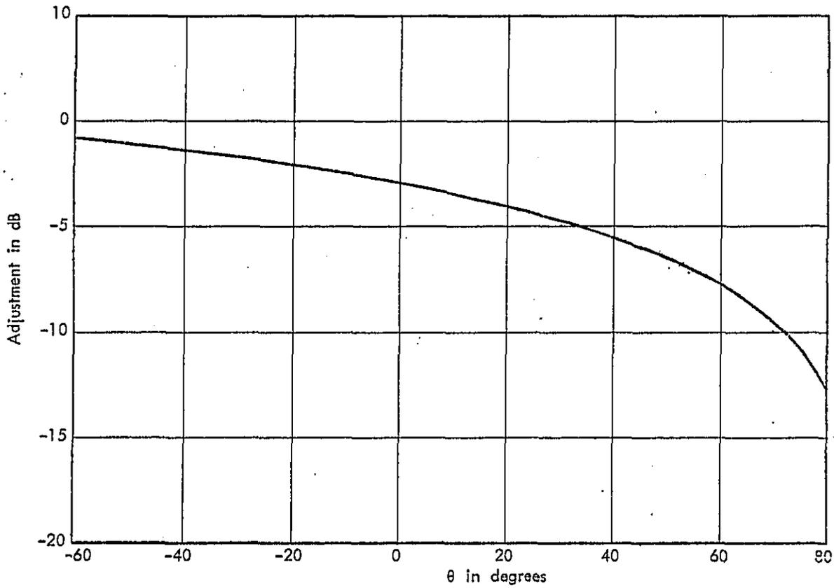
FIGURE B.6 ADJUSTMENT TO ACCOUNT FOR SEMI-INFINITE ELEMENT LENGTH
