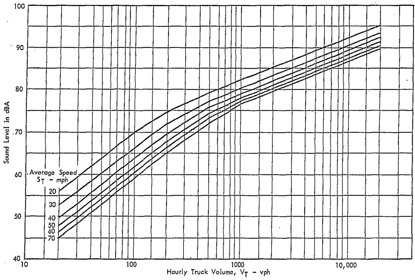
FIGURE B.4 PLOT OF  $L_{50}$  FOR TRUCKS AS FUNCTION OF VOLUME FLOW AND AVERAGE SPEED
