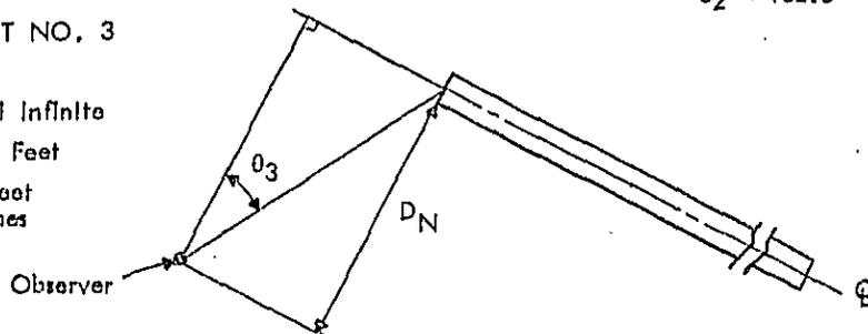
FIGURE 2. IDENTIFIED ROADWAY ELEMENTS SHOWING APPLICABLE PARAMETERS (COMPLETE METHOD)
