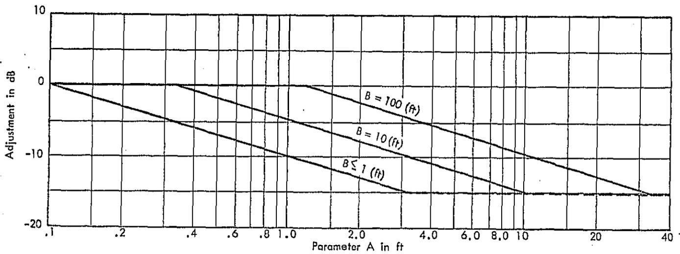
FIGURE B.8 ADJUSTMENT FOR ELEVATED AND DEPRESSED ROADWAY
