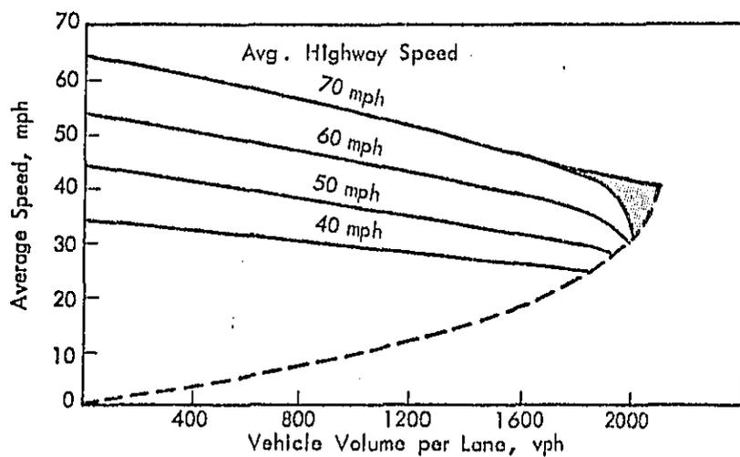
FIGURE C.3 ILLUSTRATIVE RELATIONSHIP BETWEEN TRAFFIC VOLUME PER LANE AND AVERAGE SPEED OF VEHICLE TRAVEL FOR UNINTERRUPTED FLOW
