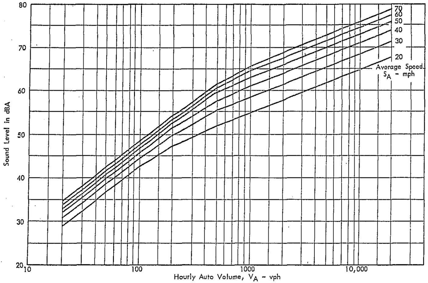
FIGURE B.3 PLOT OF  $L_{50}$  FOR AUTOMOBILES AS FUNCTION OF VOLUME FLOW AND AVERAGE SPEED
