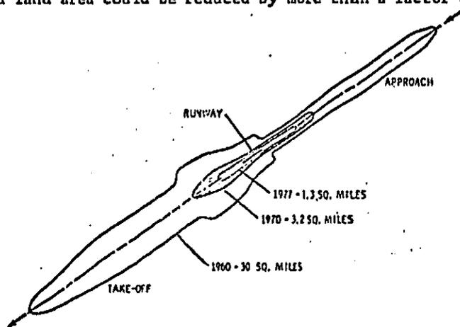
Fig. IV-1 Land Area Exposed to High Noise Levels (90PNdb) by Aircraft Designed with 1960, 1970 and 1977 Technologies<sup>(6)</sup>
