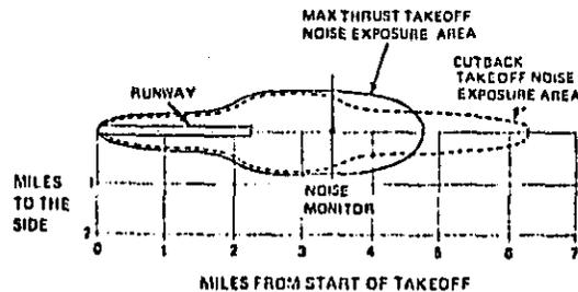
Fig. IV-3 Effect on Noise of Take-Off Procedures (90 EPNdb Contours)<sup>(11)</sup>
