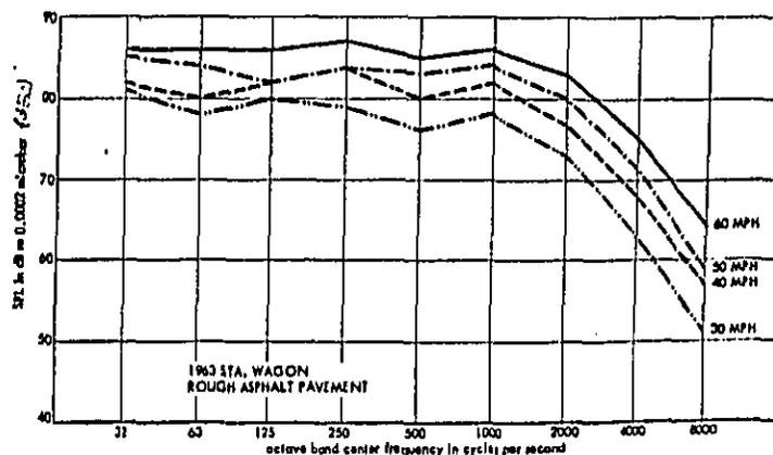
The noise spectra illustrate a consistent increase in each octave band for each increase in speed. The merging of the 40 mph and 50 mph curves at the lower frequency is probably due to a shift in spectra from engine-exhaust to tire roadway dominated.
