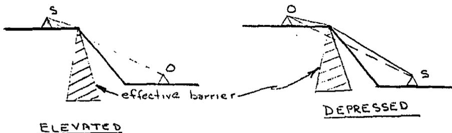
The basic principle involved is that of sound diffraction: sound energy spills over the barrier in the shadow zone on the observer side. The diffracted sound energy at the observer location is less than the energy that would reach the location if the noise followed a straight path.
