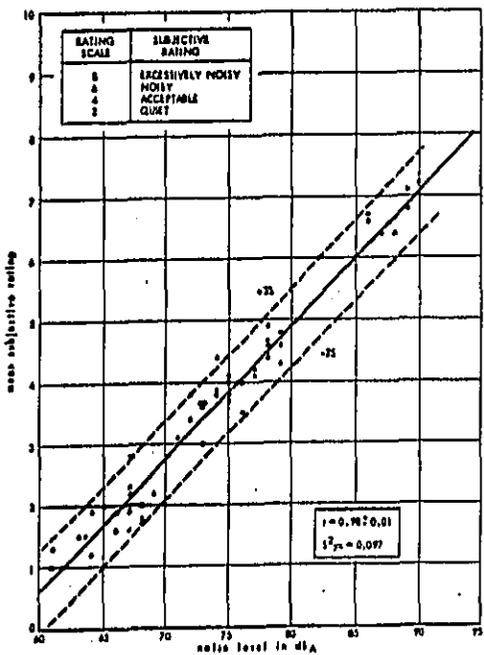
Correlation of subjective ratings of noise from gas-engined vehicles (petrol) in MIRA experiment with noise level in dBA.
