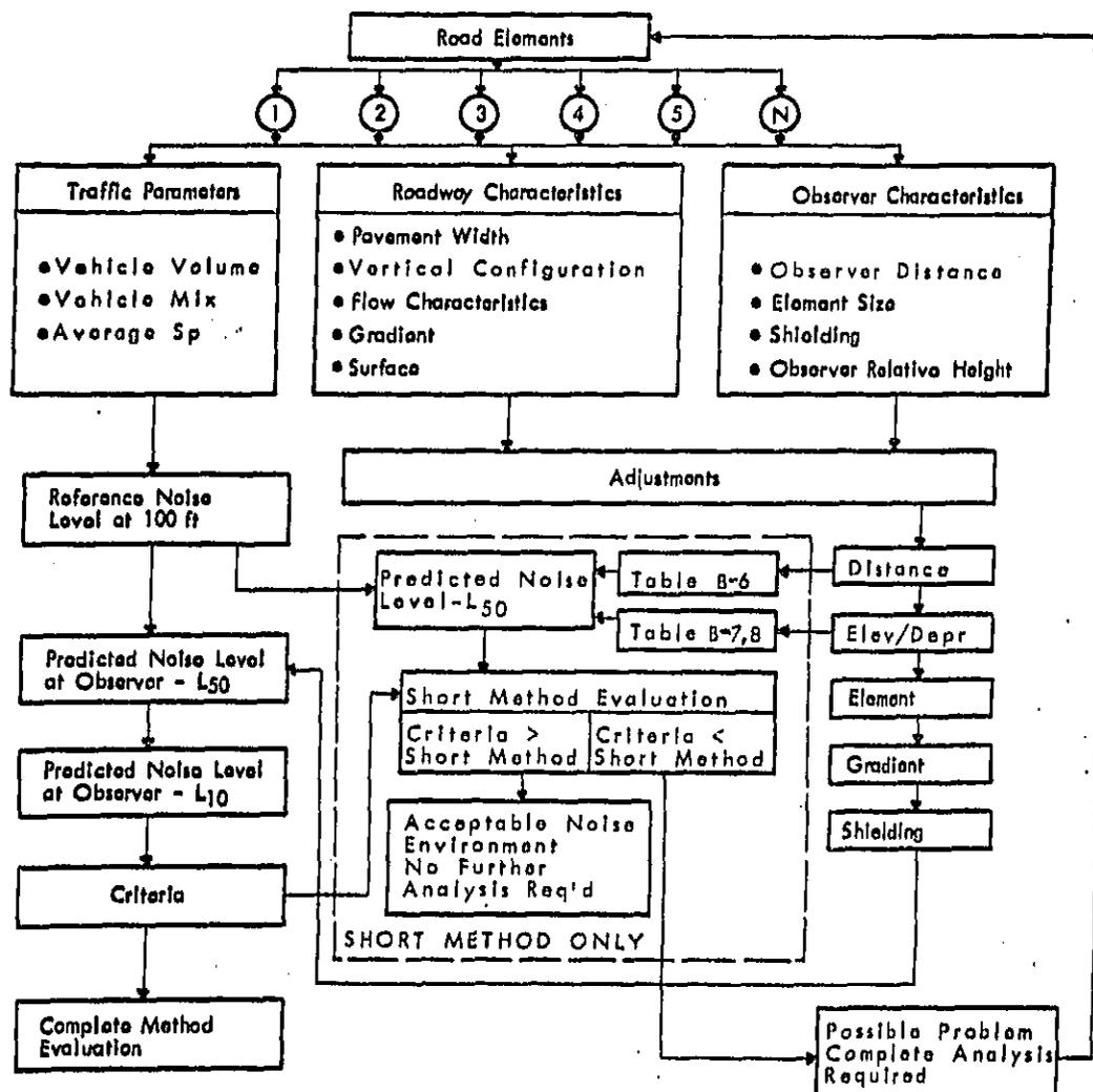
The use of the Design Guide method requires identification of roadway elements with constant geometric characteristics. Each element that is identified is then described by a series of parameters. The parameters required for utilization of the method can be grouped as follows:
