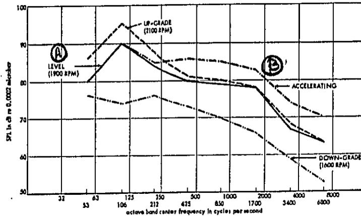
In the data presented to date, no clear cut relationship has been found to exist between noise level and truck speed. This is thought to be due to two factors: first, trucks tend to operate at relatively constant rpm, thus
