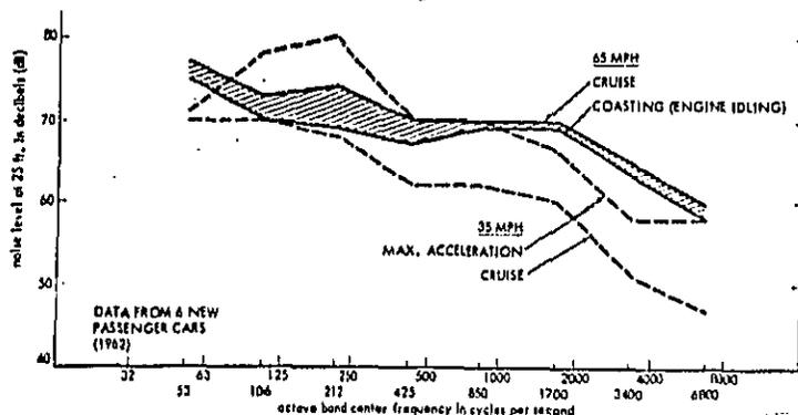
The noise generated by a motor vehicle is dependent upon its speed. A graph of the noise level-frequency band distribution as a function of various speeds is shown in Figure 12
