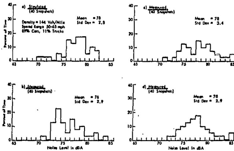
Comparison of distributions of simulated and measured noise levels in dBA from an 8-lane freeway for a distance of 50 ft from the edge of the nearest lane.
