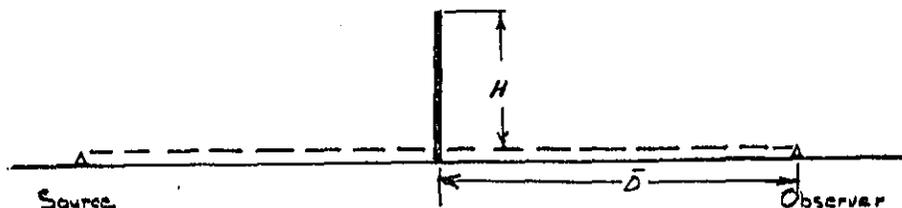
In the study done in Toronto by Harmelink & Hajek<sup>(11)</sup>, two roadways were analyzed. The pre-barrier field measurements of  $L_{10}$  were made, barriers of four different materials were constructed, and the after  $L_{10}$  noise measurements were taken. Noise measurements were made for the before and after condition during times of similar traffic volumes and vehicle mix. The barrier height was limited to ten feet.
