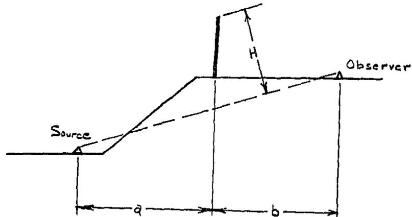
The noise reduction factor ( $Y$ ) can then be converted to a corresponding decibel reduction from the relationship shown in Figure 33, on page 67. From these relationships, series of curves can be drawn for various effective barrier heights, at various distances. Such a series of curves for an effective barrier height of 10 feet is shown in Figure 34, page 68.
