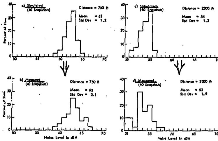
Comparison of distributions of simulated and measured noise levels in dBA from an 8-lane freeway, for distances of 750 ft and 2,300 ft from the edge of the nearest lane.
