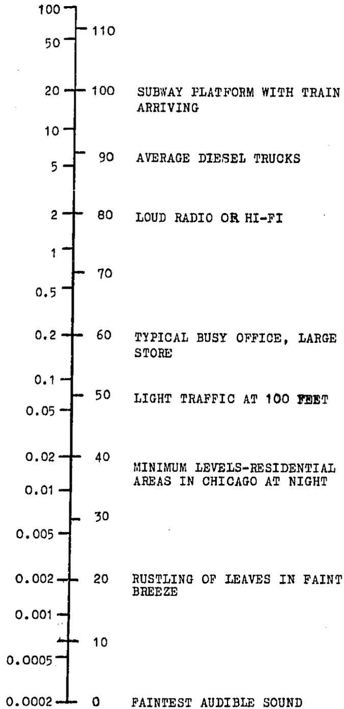
SOUND PRESSURE (microbars) vs. SOUND PRESSURE LEVEL (dB)
