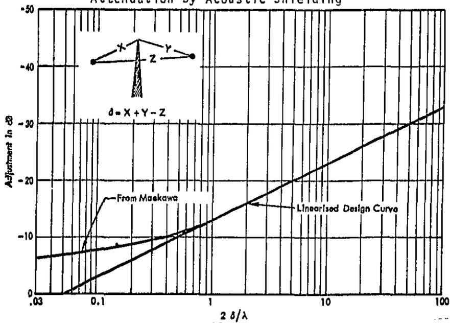
Figure 26 shows relationships that have been developed on the basis of the linearised design curve for adjustments to the basic model in regard to elevated or depressed configurations. The curves given are for the noise levels produced by automobiles only. Truck noise attenuation due to roadway configuration is assumed to be 5 dBA less.
