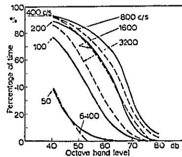
Fig. 7. Statistics of peak levels in radio-programmes. For each of eight octave bands the percentage of the time that certain octave band levels are surpassed is indicated, based on about 55 hours of mixed radio-programmes (v. den Bjrk).
