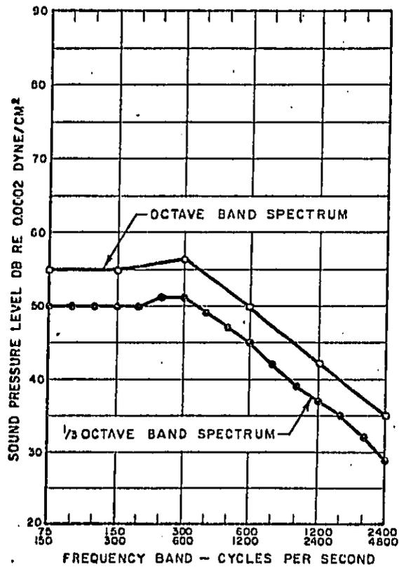
FIG. D.3. COMPARISON OF THE SAME NOISE, AS MEASURED IN OCTAVE BANDS AND 1/3-OCTAVE BANDS.
