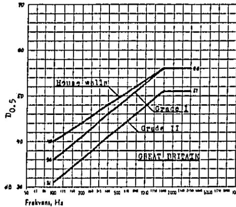
Fig. 14 C. Requirements and recommendations for airborne insulation in Great Britain. Symbols for R, R', etc. as in the preceding section.
