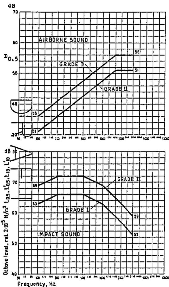
Fig. 6. From the English flat survey the conclusion was to use two grading curves for airborne and impact insulation.
