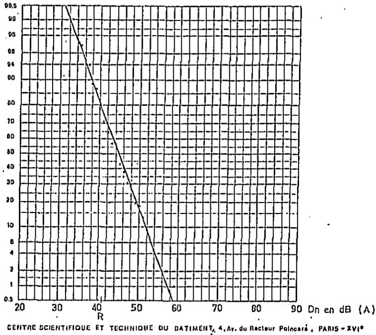
FIG. B.3. DISTRIBUTION OF TEST RESULTS IN FRENCH FIELD TESTS (1969-72) OF NOISE ISOLATION.
