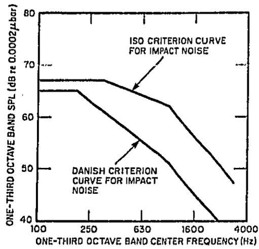
FIG. A.4. DANISH IMPACT NOISE REQUIREMENT, IN COMPARISON WITH THE ISO REFERENCE CURVE.
