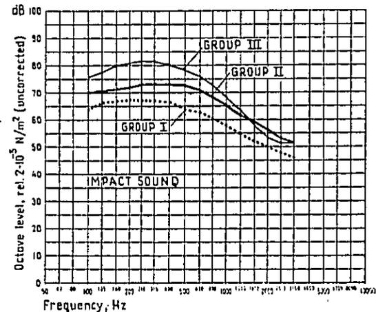
Fig. 5. Measured values for airborne and impact sound for the English flat survey. The values are average figures and uncorrected.
