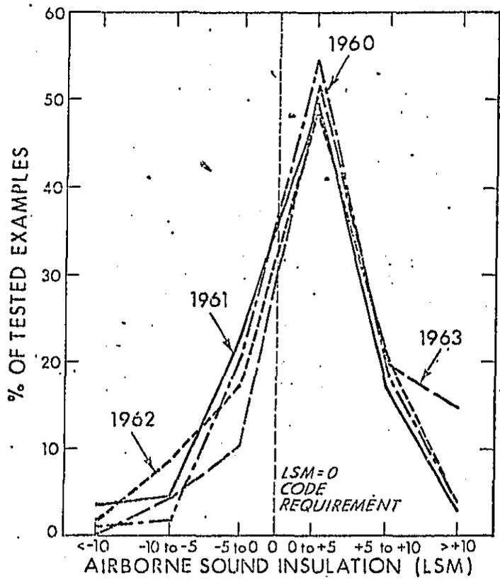
FIG. B.5. WALLS: AIRBORNE SOUND INSULATION FIELD TESTS, 1960 TO 1963, MULLER-BBN, MUNICH.
