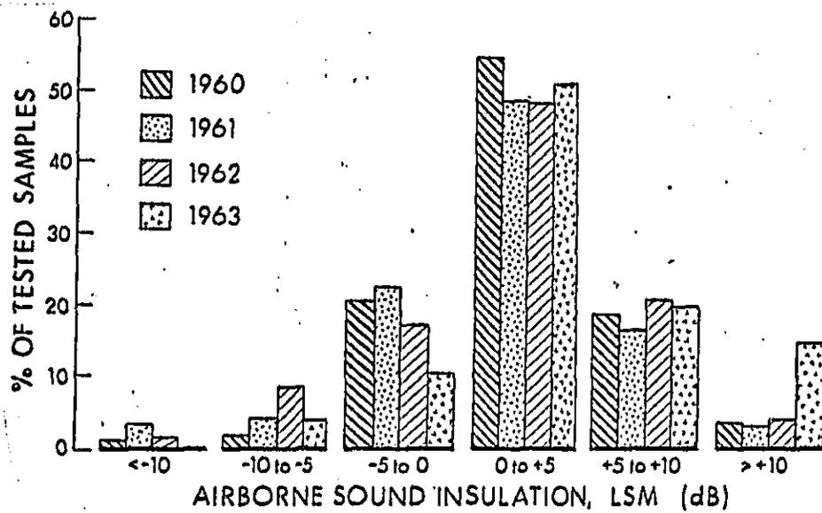
FIG. 6. WALLS: AIRBORNE SOUND INSULATION
