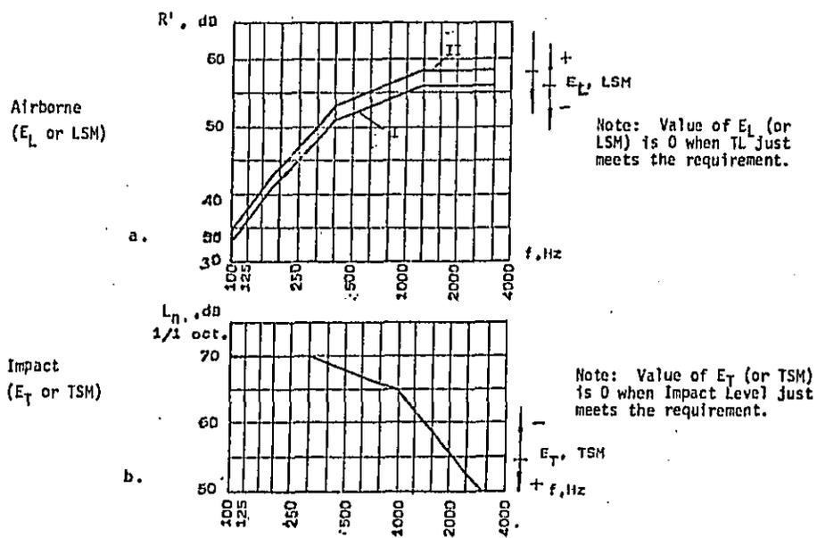
FIG. A.3. REFERENCE CURVES FOR AIRBORNE ( $E_L$ ) AND IMPACT ( $E_T$ ) SOUND INSULATION USED IN THE RATINGS OF CMEA, POLAND, CZECHOSLOVAKIA, AND EAST AND WEST GERMANY (LSM AND TSM).
