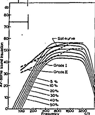
Fig. 9. Required airborne sound insulation based on a disturbing neighbour's radio level surpassing 20 phons during, in the mean, 5, 10, 20, 30, 40 or 50 per cent of the time. For comparison the German (Soli-Kurve) and the British (Grade I and II) requirements for dwellings are added (v. den Eijk).
