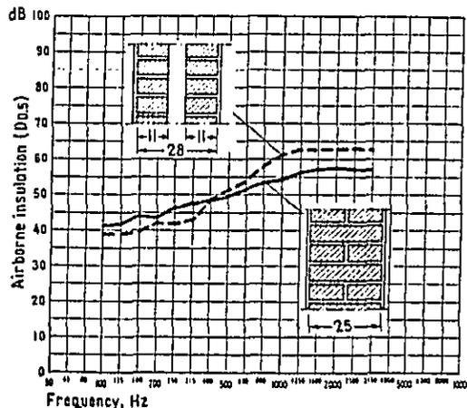
Fig. 3. Airborne insulation (D) for the English party walls in social survey. Average of two: one 25 cm solid brick wall, five 27 cm cavity brick wall houses.
