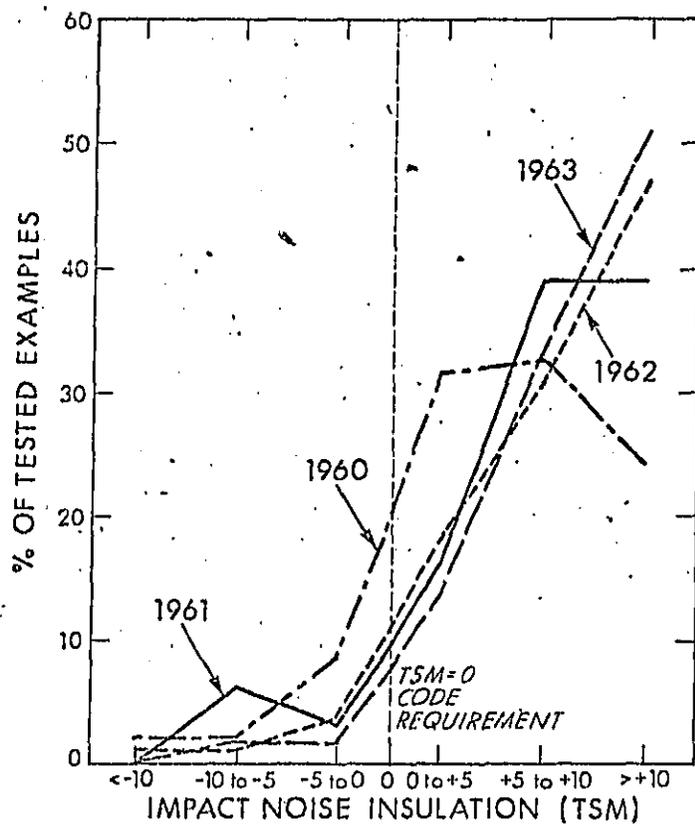
FIG. B.6. FLOORS: IMPACT NOISE INSULATION FIELD TESTS, 1960 TO 1963, MULLER-BBN, MUNICH.
