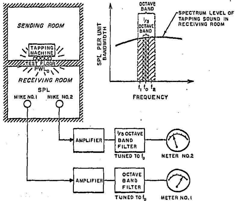
FIG. D.2. COMPARISON OF IMPACT NOISE MEASUREMENTS IN OCTAVE BANDS AND  $1/3$ -OCTAVE BANDS.
