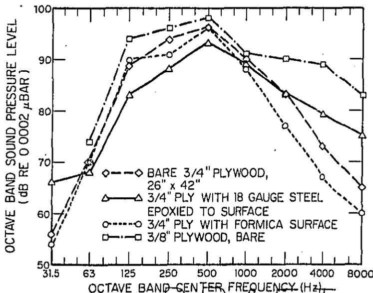
Figure 3—Spectrum of Sound Generated by Standard Tapping Machine Operating on a Resiliently Suspended Sheet of Plywood, 26" Above Floor
