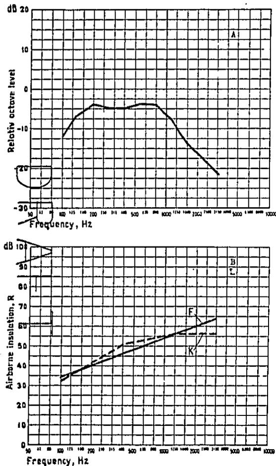
Fig. 11. When the observers listened to "coloured" noise, see A, through the wall filters with the responses F (6 dB/octave) and K, see B, it was judged to be equally loud. The average figure  $\bar{R}$  and Luftschallschutzmass LSM are for F:  $\bar{R} = 49$  dB,  $LSM = 0$  dB; for K:  $\bar{R} = 50$  dB and  $LSM = 2$  dB.
