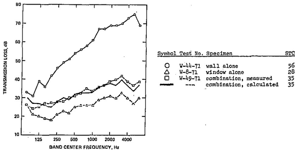
Figure 42. Comparison of measured sound transmission loss vs frequency data for a 6 x 5 ft picture window, glazed single strength, in a brick veneer wall with that predicted from the transmission losses and areas of the wall and window (window area = 25.6 sq ft, wall plus window area = 126 sq ft).
