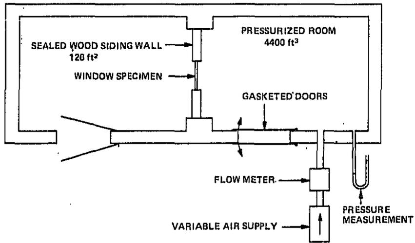
Figure 67. Experimental setup for measuring air filtration of doors and windows in the sound transmission facility.
