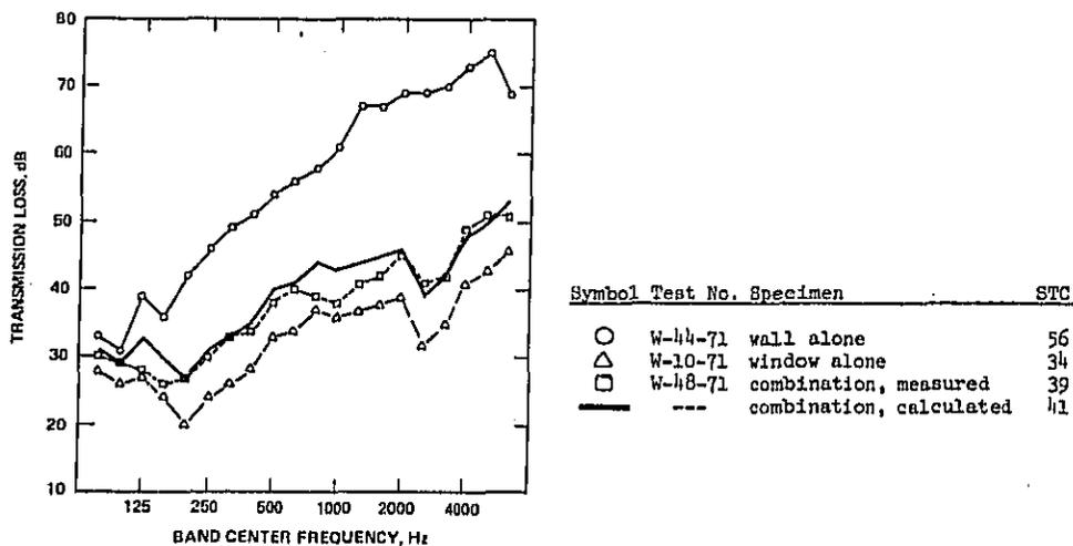
Figure 43. Comparison of measured sound transmission loss vs frequency data for a 6 x 5 ft picture window, glazed 1 in insulating glass, in a brick veneer wall with that predicted from the transmission losses and areas of the wall and window (window area = 25.6 sq ft, wall plus window area = 126 sq ft).
