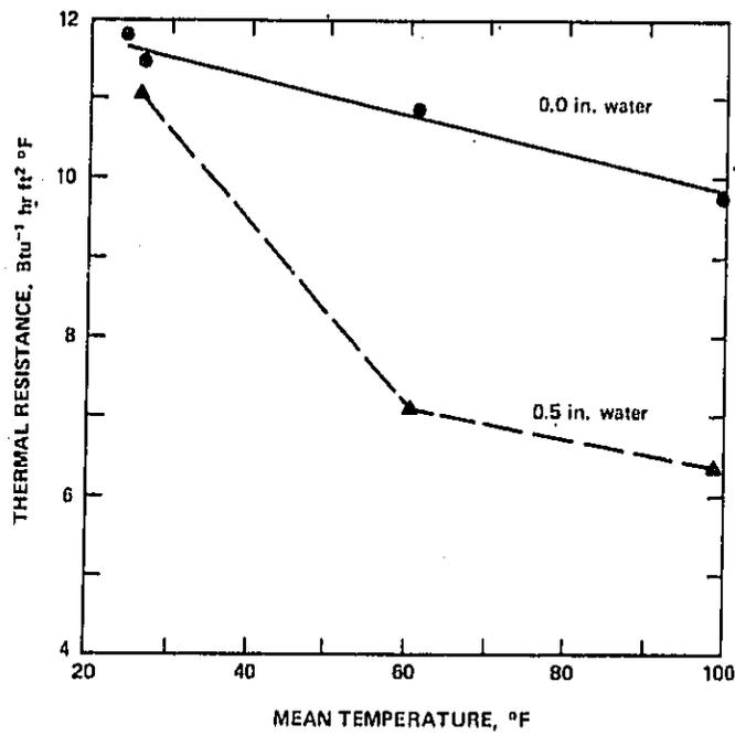
Figure 64. Thermal resistance vs mean temperature data for a 2 x 4 in. stud wall with 1/2 in. gypsum board on the interior surface, redwood lap siding over 1/2 in. wood fiber sheathing on the exterior surface, and 3 1/2 in. Fiberglas Friction Fit Building Insulation plus a polyethylene vapor barrier in the cavity.
