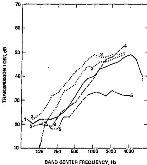
Figure 56. Sound transmission loss vs frequency data for double glazing with an average nominal spacing of about 2 to 3 in. between the two panes.
