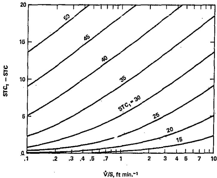
Figure 73. Expected decrease in Sound Transmission Class as a function of air leakage rate divided by area. The air leakage rate,  $\dot{V}$ , measured according to ASTM E283-73 [125] is expressed in  $\text{scfm}$  at a pressure difference of 0.3 in. water. The window or door area,  $S$ , is in  $\text{sq ft}$ . The parameter on the curves is the Sound Transmission Class of the sealed unit (window or door).
