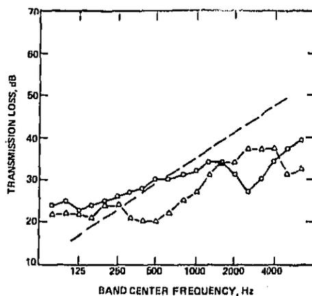
Figure 30. Comparison of sound transmission loss vs frequency data for insulating glass with data for single glazing of the same surface density (nominally  $2.6 \text{ lb/ft}^2$ ). The dashed curve represents field incidence mass law (see Figure 14 and accompanying text).
