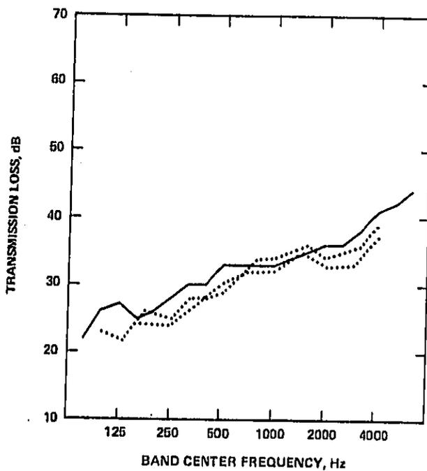
Figure 53. Sound transmission loss vs frequency data for  $1/4$  in. laminated glass with an internal damping layer. The solid curve represents the data from the present investigation (Test No. W-22-72) while the dotted curves represent the envelope of data from Table A8 of Marsh [63] (the two sets of data are that of Pilkington Bros. and the 1st of Libbey-Owens-Ford).
