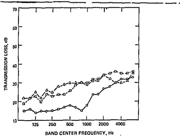
Figure 22. Sound transmission loss vs frequency data for the three wood doors sealed into the frame.
