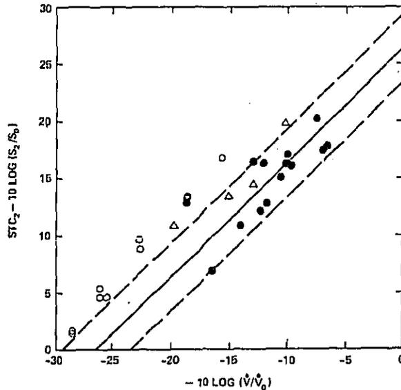
Figure 71. Experimentally determined values for  $STC_2 - 10 \log (S_2/S_0)$  plotted vs experimentally determined values for  $-10 \log (V/V_0)$ ; see text.
