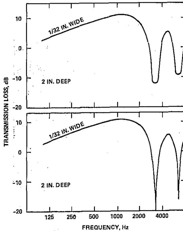
Figure 58. Theoretical sound transmission loss vs frequency data for slits in the middle of a wall between two reverberant rooms. The lower curve represents pure tone behavior while the upper curve corresponds to values averaged over a frequency band that is  $1/3$  octave in width. The lower curve was computed from eq. (69) of Comperts [76] while the upper curve was derived by numerical integration of the transmission coefficient corresponding to the lower curve.
