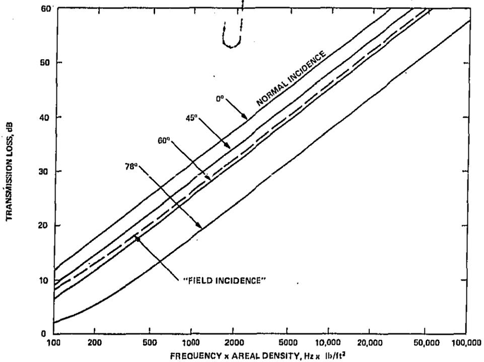
Figure 14. Limp-wall mass law transmission loss. The solid curves correspond to a plane wave arriving at a discrete angle of incidence. The dashed curve corresponds to "field-incidence mass law", a sum over all angles of incidence up to 78°.
