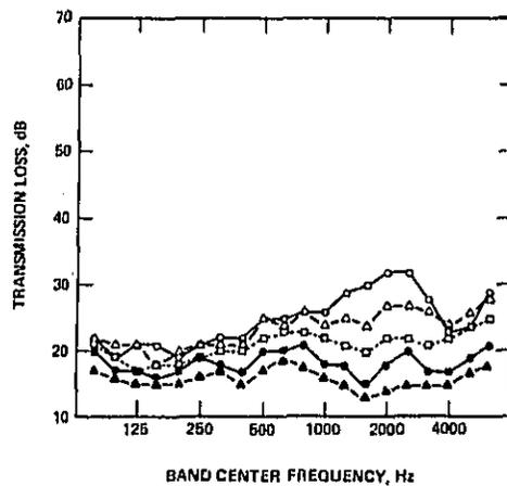
Figure 33. Sound transmission loss vs frequency data for 6 x 5 ft picture window, double-strength glazing, with perimeter cracks of controlled size.
