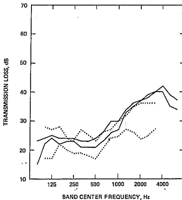
Figure 54. Sound transmission loss vs frequency data for 7/16 in. insulating glass units consisting, nominally, of two 1/8 in. panes of glass separated by a 3/16 in. air space. The solid curves represent the envelope of data obtained in the present investigation (Tests W-31-71 and W-29-72). The dotted curves represent the envelope of data from Table B1 of Marsh [63]. (the sets of data included are the 2nd of Wooley and the two of Saint-Gobain).
