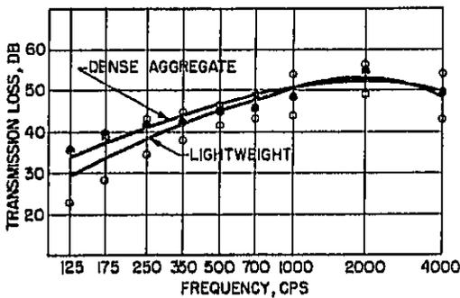
Fig. 9. Sound Transmission Loss Curves for Painted 4 in. Hollow Block
