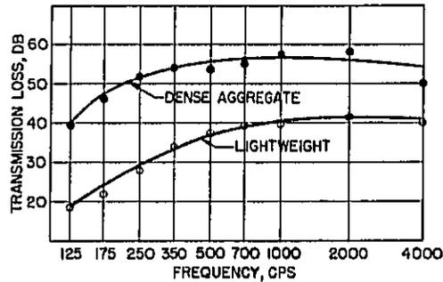
Fig. 10. Sound Transmission Loss Curves for Unpainted 8 in. Hollow Block
