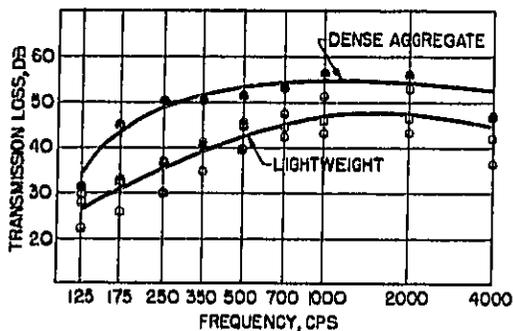
Fig. 13. Sound Transmission Loss Curves for Unpainted 6 in. Hollow Block
