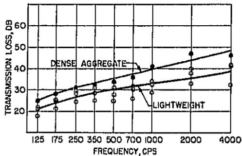
Fig. 12. Sound Transmission Loss Curves for Unpainted 4 in. Solid Block
