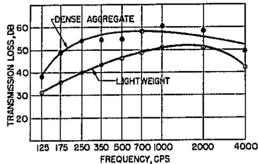
Fig. 11. Sound Transmission Loss Curves for Painted 8 in. Hollow Block
