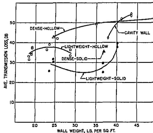
Fig. 7. Effect of Wall Weight on Sound Transmission Loss
