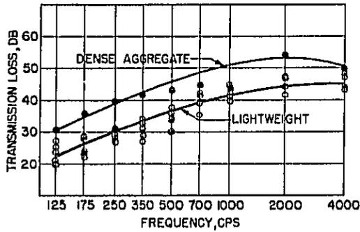
Fig. 8. Sound Transmission Loss Curves for Unpainted 4 in. Hollow Block
