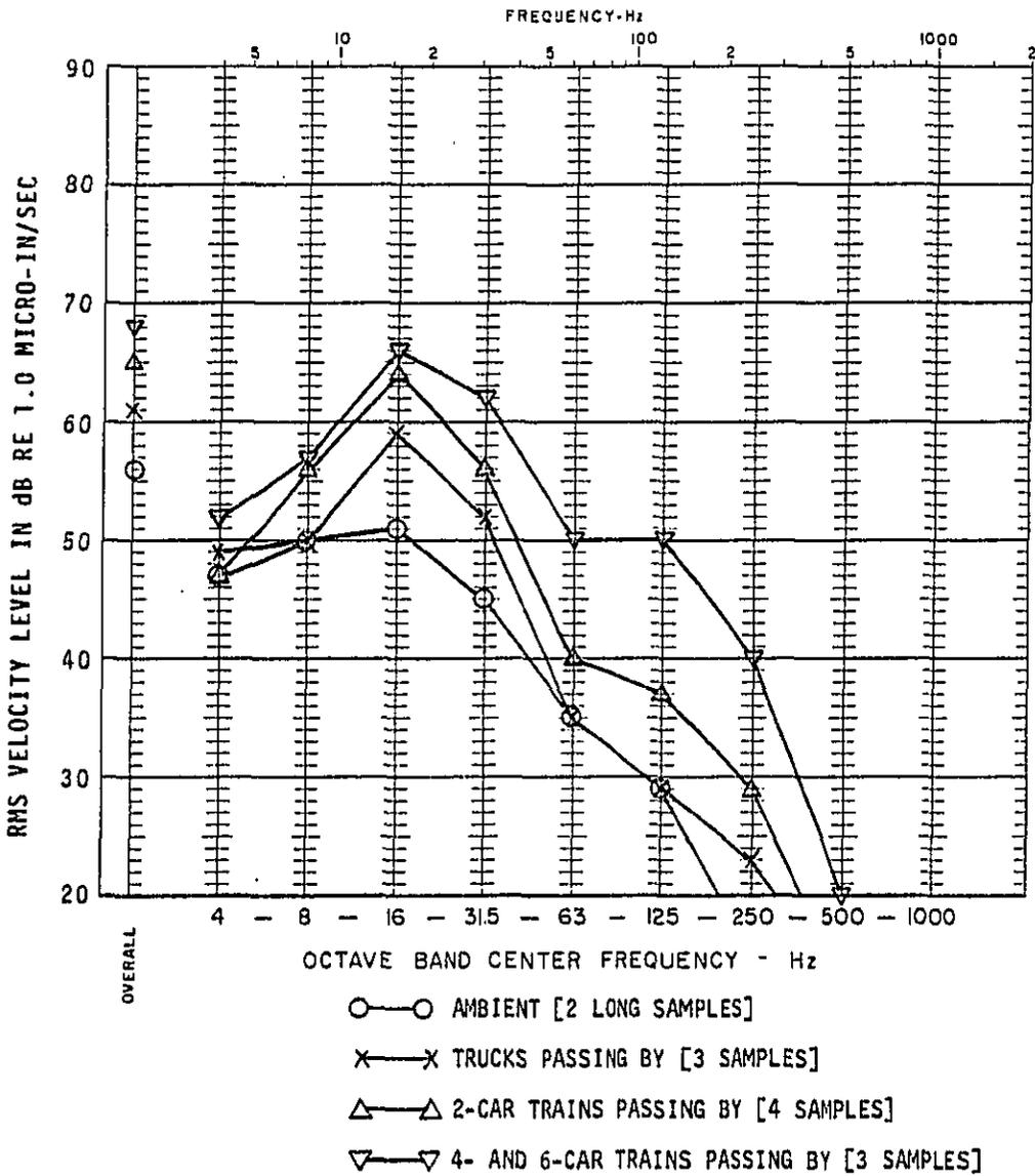
FIGURE 23<sup>6</sup> OCTAVE BAND ANALYSIS OF INDIVIDUAL EVENTS AT LOCATION 14e
