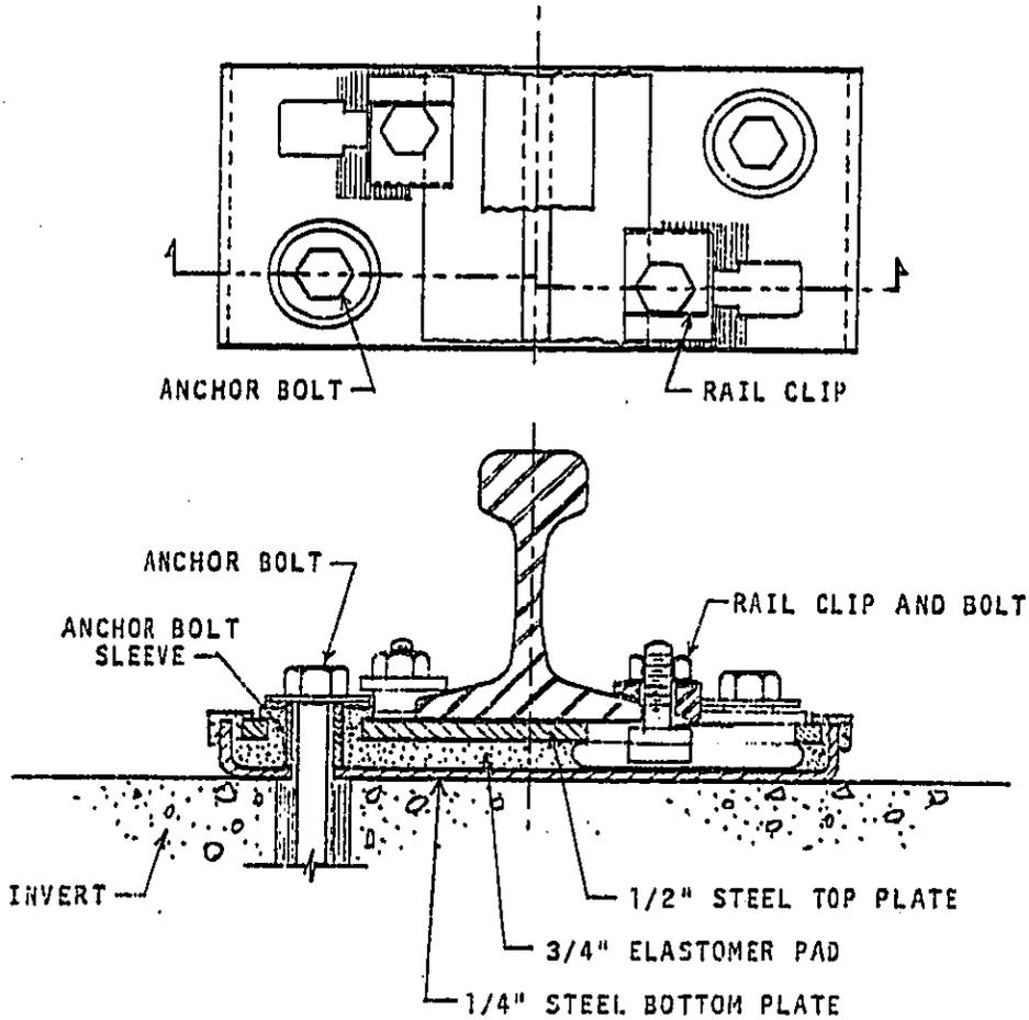
FIGURE 37 BART [LANDIS] RESILIENT DIRECT FIXATION RAIL FASTENER WITH BONDED ELASTOMER PAD
