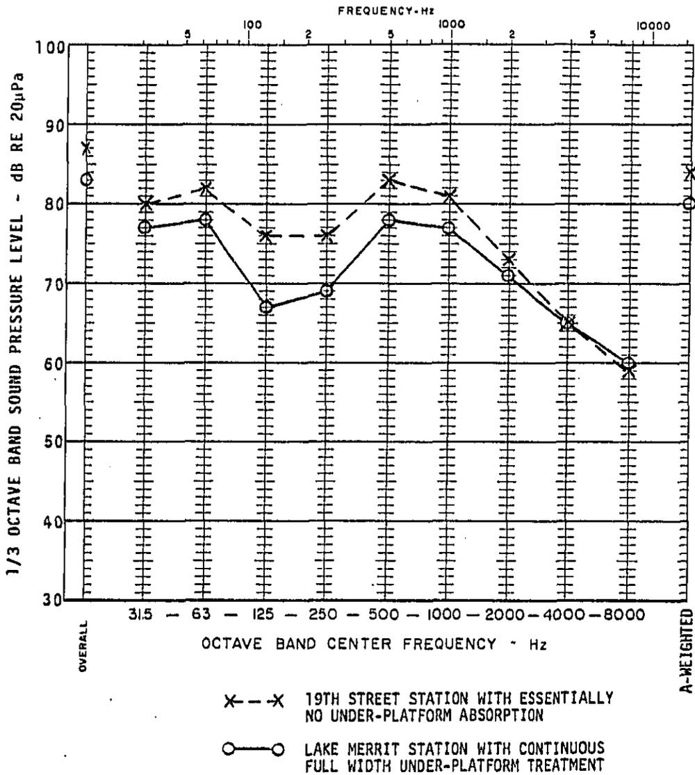
FIGURE 38 NOISE LEVELS ON BART UNDERGROUND STATION PLATFORMS WITH TRAINS PASSING THROUGH AT A CONSTANT SPEED OF 20 MPH
