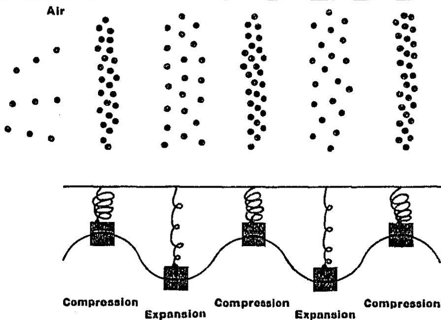
What does the vibration of a spring have to do with sound in air? Let's look at a hi-fi loudspeaker emitting a single tone. As the speaker cone moves forward and backward like the spring, it alternately compresses and expands the air in front of the cone. The compression and expansion then moves out away from the loudspeaker as a sound wave.
