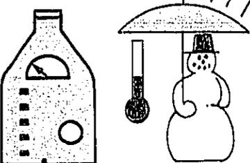
Allow the SLM to come to the same temperature as the surroundings. Do not make measurements when it is raining or snowing, or when the temperature is lower than the manufacturer's recommendation.
