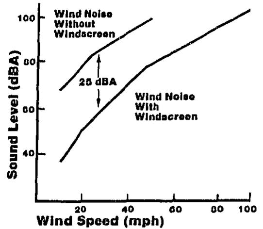
Does wind affect SLM accuracy? Yes! For example, a 25 mph breeze blowing across a typical SLM microphone can cause readings of 80dBA. It is for this reason we place a plastic foam ball called a windscreen over the microphone. The windscreen attenuates the noise caused by wind by approximately 25 dBA, yet it does not noticeably affect the level caused by noise. The windscreen also protects the microphone from rain, dirt, birds, etc; it should normally be used at all times.
