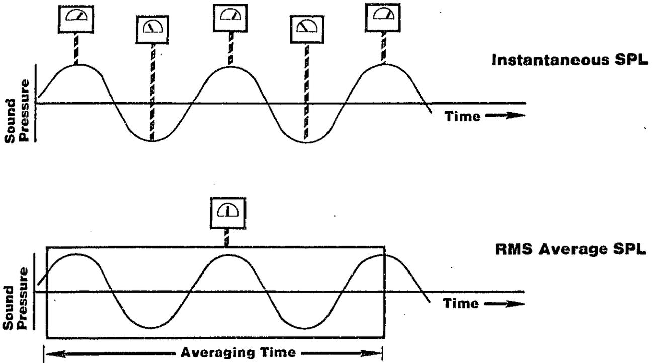
Another setting on the SLM is "meter response". If the SLM responded to instantaneous sound pressure what would happen? Looking at a 1000 Hz tone, the meter pointer would rise and fall 1000 times per second as it followed the sound pressure. All we would see is a blur.
