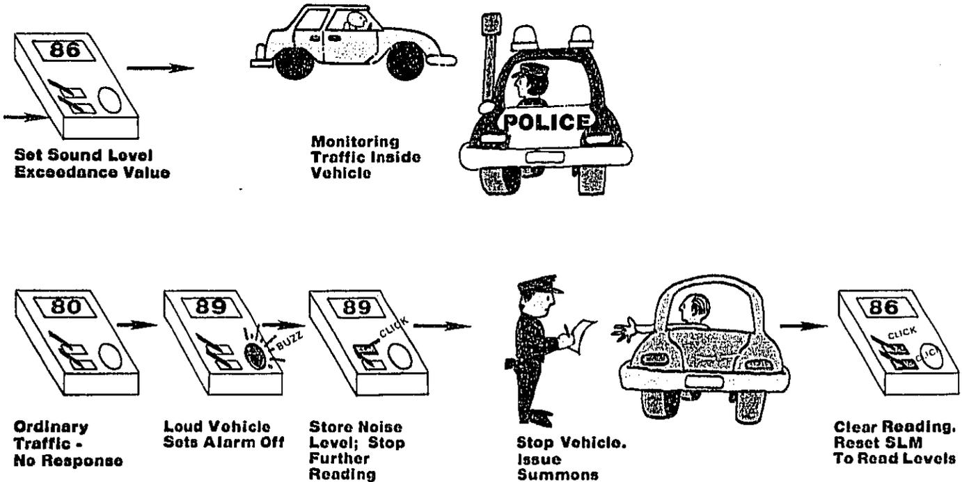
New innovations are appearing in SLMs, making their use easier and more convenient for motor vehicle enforcement. Several SLMs now allow monitoring from inside a patrol car at the same time an officer is doing radar speed enforcement.
