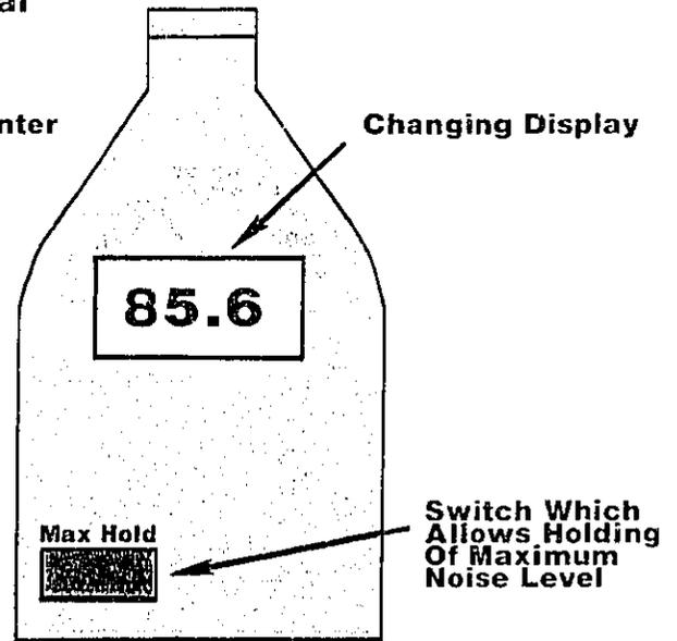
Two types of SLM display are available on SLM's today - digital and analog. Each has its own advantages and disadvantages.
