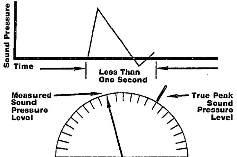
**RULE: The sound level meter will always read less than the true maximum value for an impulsive noise.**
