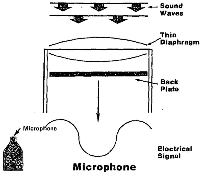
An important part of the SLM is the MICROPHONE. The microphone works like a drum in reverse. When you hit a drum the drumhead vibrates causing the air in front of it to alternately compress and expand. As you know from the previous discussion, this causes a sound wave to be propagated outward toward your ear.
