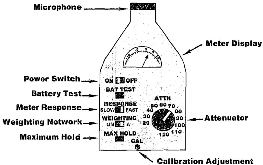
This illustration depicts a sound level meter having features found on many SLMs used in motor vehicle enforcement. Your particular SLM may not have some of the features, and others of them may be incorporated into the instrument so that no switch is necessary. You may also have some special features not discussed here.
