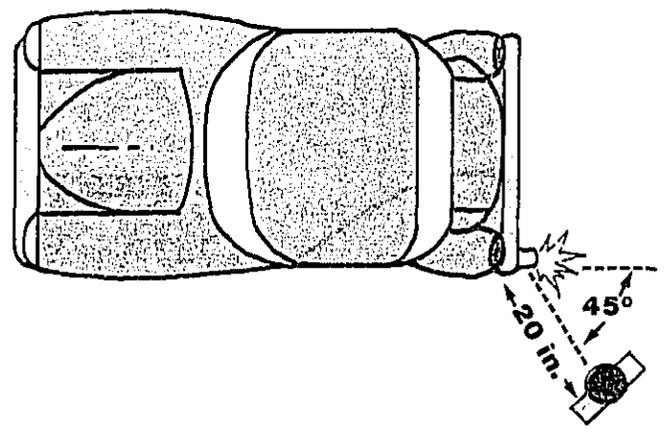
**SLM at 45° angle to tailpipe exhaust axis and 20 inches from outlet**
