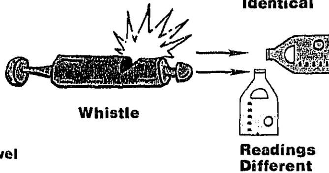
orientations will vary hardly at all. However, if you try measuring the sound level of a high frequency source such as a siren or a whistle, the sound level measured will depend very much on the angle at which the sound hits the microphone.
