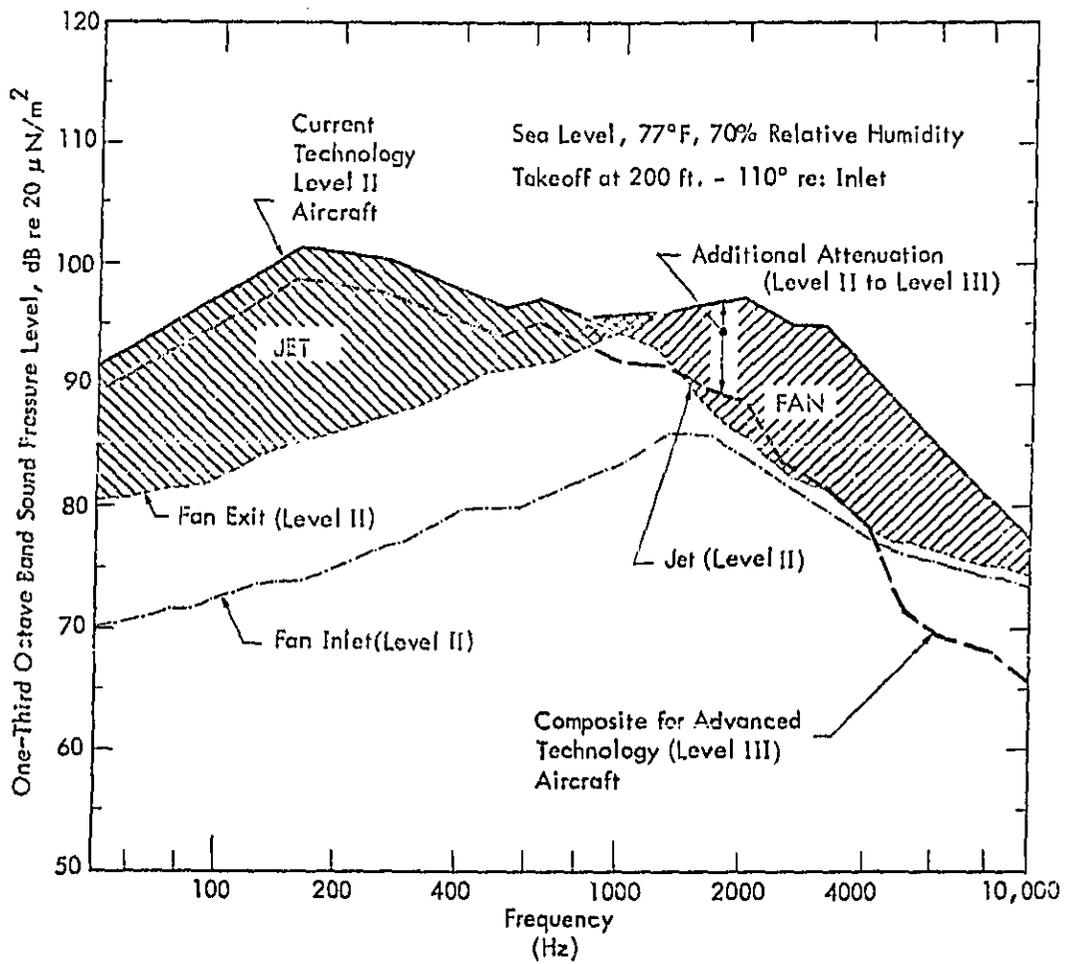
Figure 4-2. Three-Engine Wide Body Reference Spectra
