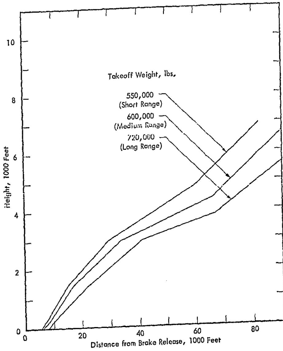
Figure B-6. Takeoff Profiles for Level III Technology, 4-Engine Aircraft
