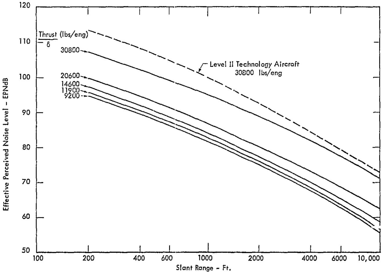
Figure B-1. Noise Curves for Level III Technology - 2 Engine Aircraft.
