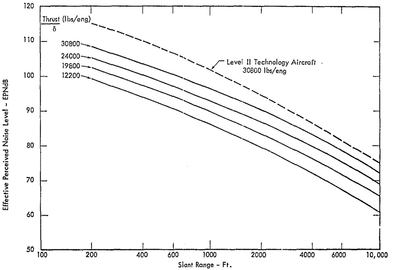
Figure B-2. Noise Curves for Level III Technology - 3 Engine Aircraft.
