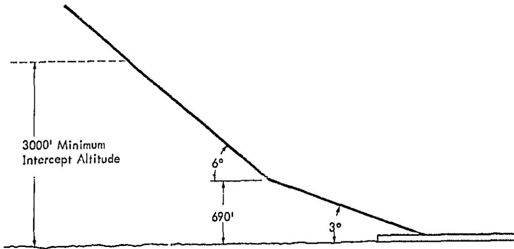
Figure 3-1. 6°/3° Glide Slope Procedure
