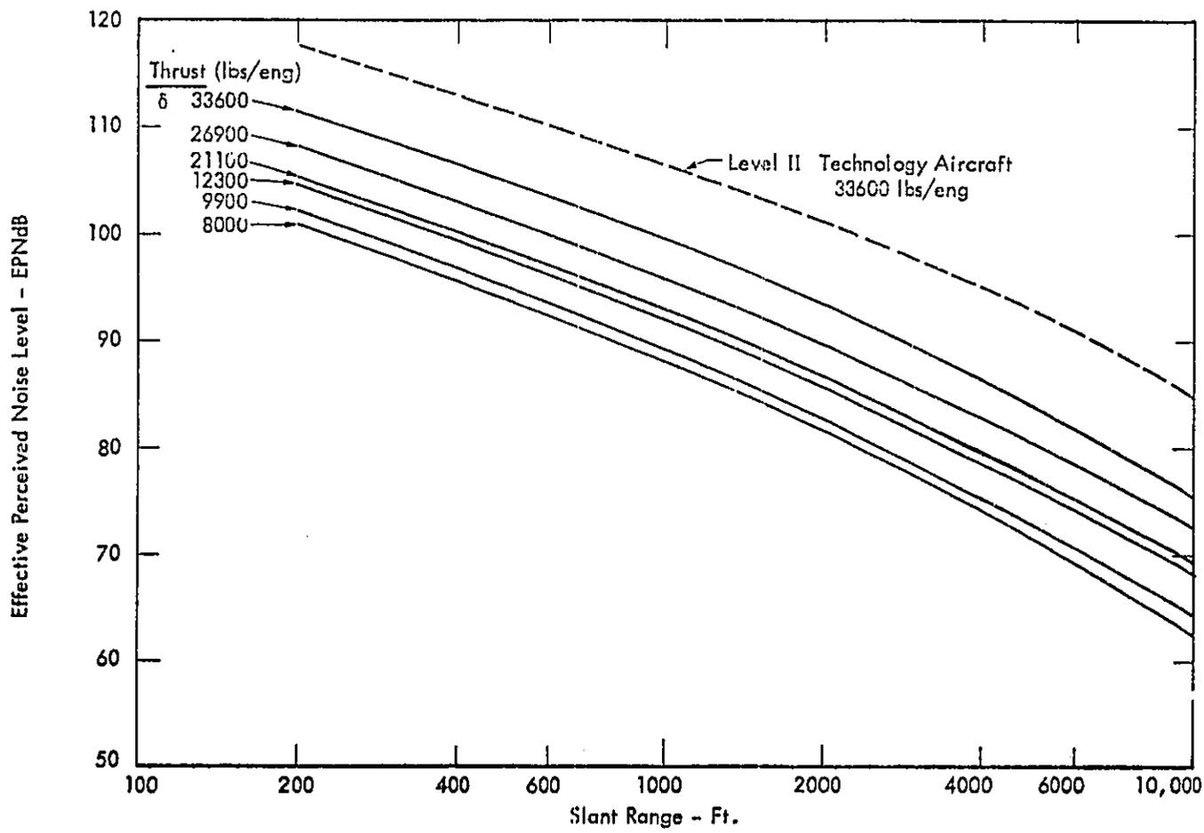
Figure B-3. Noise Curves for Level III Technology - 4 Engine Aircraft.
