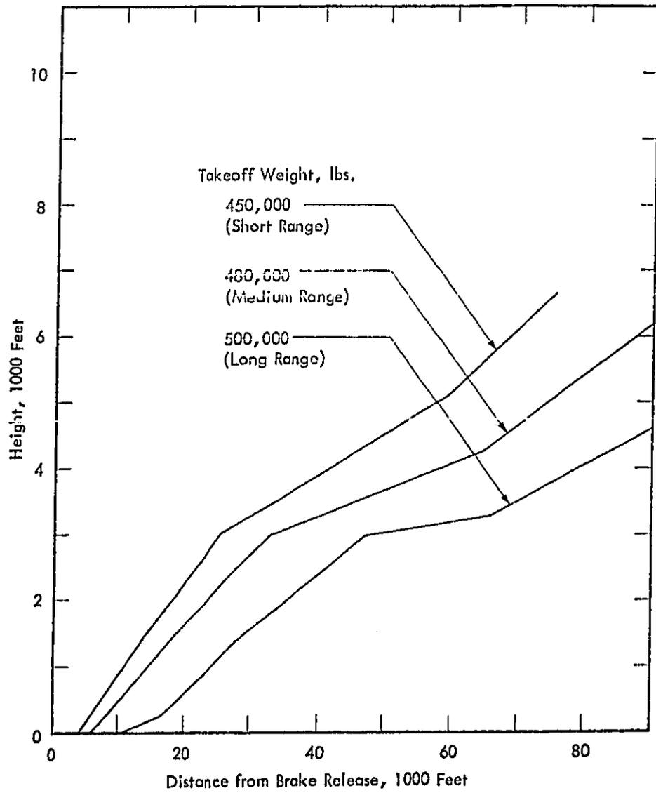
Figure B-5. Takeoff Profiles for Level III Technology, 3-Engine Aircraft
