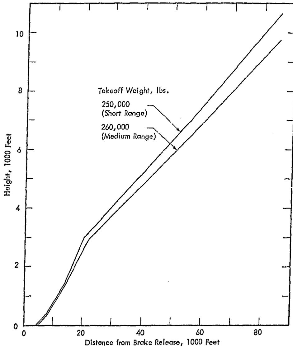
Figure B-4. Takeoff Profiles for Level III Technology, 2-Engine Aircraft
