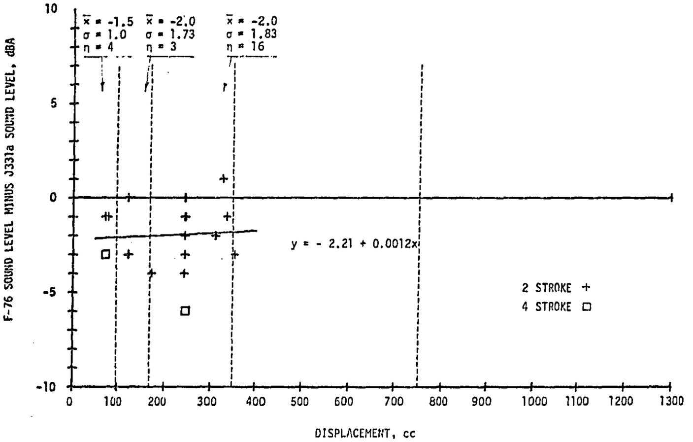
FIGURE 4-6 COMPARISON OF F-76 AND J331a SOUND LEVELS, '75 - '76 YR OF MFG OFF-ROAD (ONLY) MOTORCYCLES
