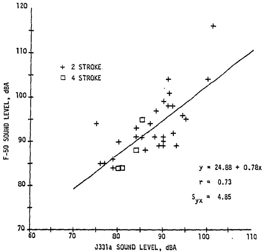
FIGURE 3-7 CORRELATION BETWEEN F-50 AND J331A TESTS,
