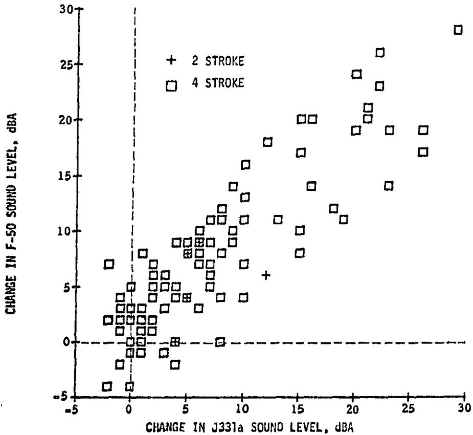
FIGURE 3-10 CORRELATION BETWEEN CHANGE IN F-50 SOUND LEVEL COMPARED TO CHANGE IN J331a SOUND LEVEL, AFTERMARKET AND MODIFIED CONFIGURATIONS REFERRED TO ORIGINAL MANUFACTURE
