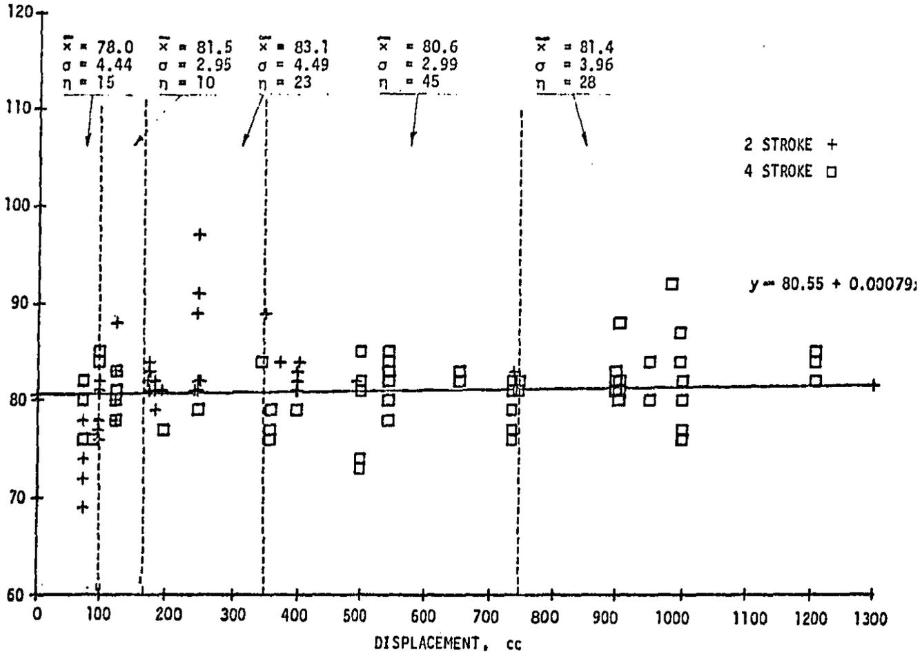
FIGURE 4-1 J331a SOUND LEVELS, STREET AND COMBINATION STREET / OFF-ROAD '75 - '76 YR. OF MFG. MOTORCYCLES
