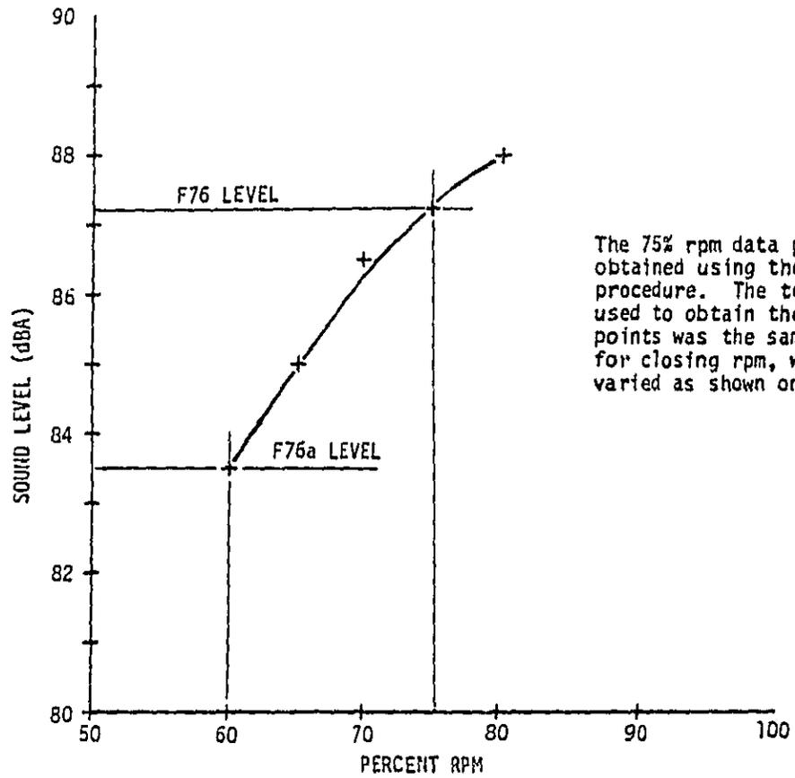
The 75% rpm data point was obtained using the F76 test procedure. The test procedure used to obtain the other data points was the same except for closing rpm, which was varied as shown on the plot.
