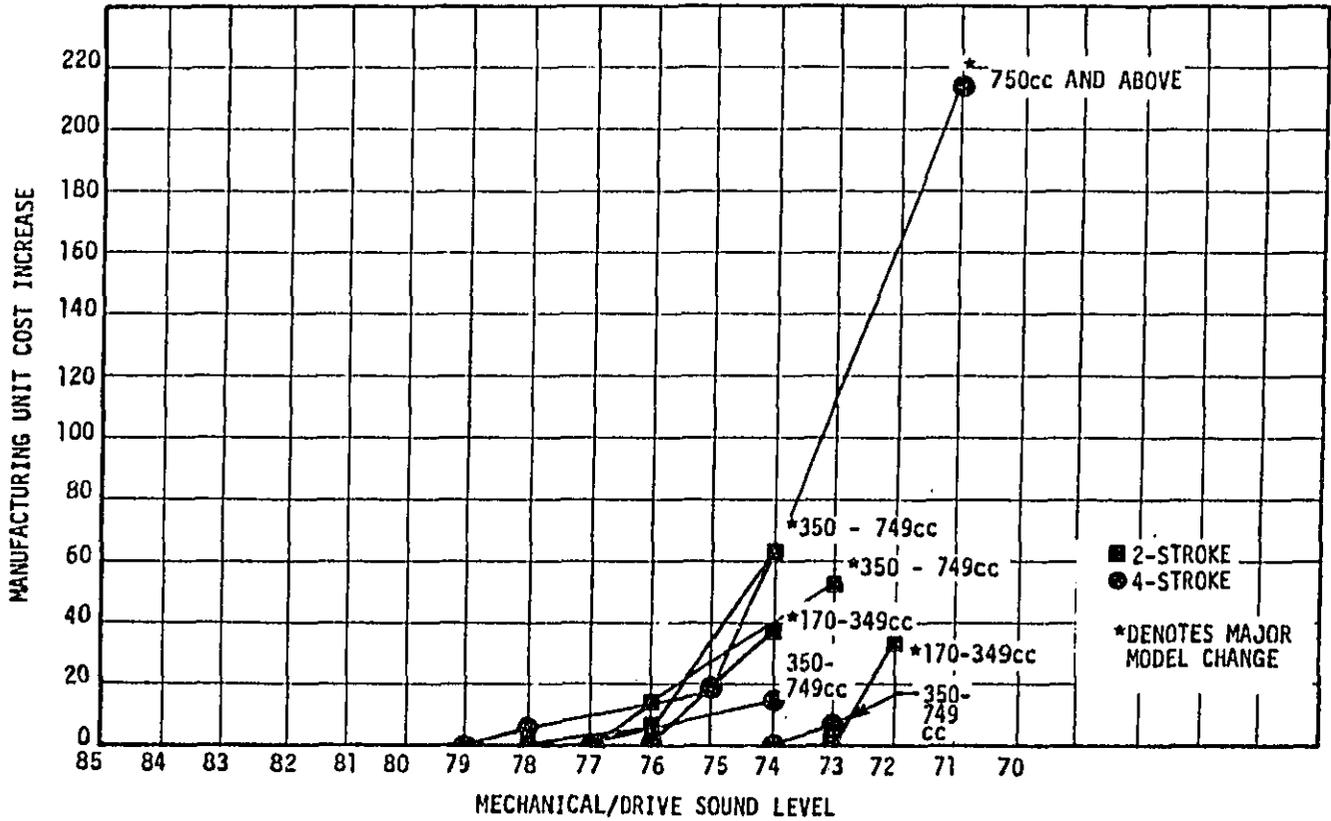
FIGURE 7-4 MECHANICAL/DRIVE MANUFACTURING UNIT COST INCREASE VS. SOUND LEVEL REDUCTION (MANUFACTURER SUPPLIED DATA)
