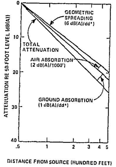
Figure 5-16. Attenuation of Point Source Noise Levels Over Open Terrain<sup>35</sup>
