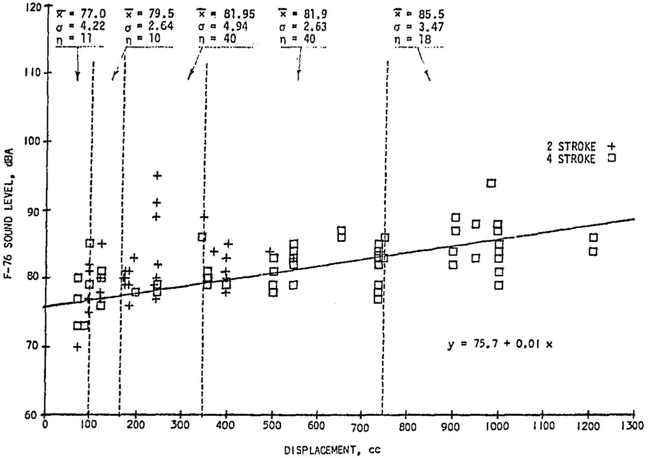
FIGURE 4-3 F-76 SOUND LEVELS, STREET AND COMBINATION STREET/OFF-ROAD '75 - '76 YR OF MFG MOTORCYCLES
