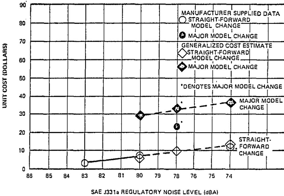
FIGURE 7-8 CATEGORY I MANUFACTURER'S AMORTIZED TOOLING COST ON A UNIT BASIS VS. REGULATORY NOISE LEVEL
