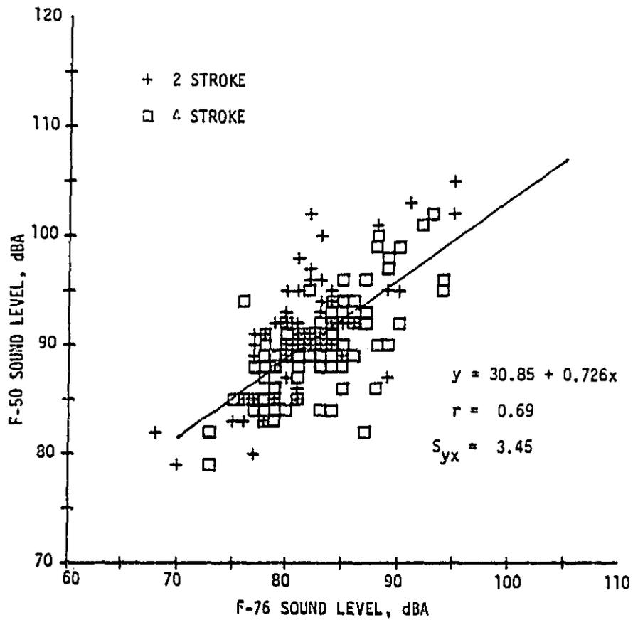
FIGURE 3-8 CORRELATION BETWEEN F-50 AND F-76 TESTS,
