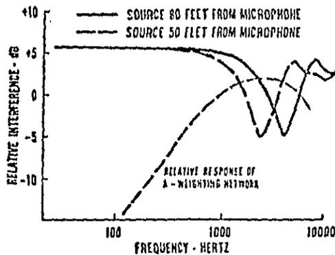
Calculated interference of third-octave band noise for a source height of one foot, microphone height of four feet, and a surface reflection of 0.9. (From Reference 3)
