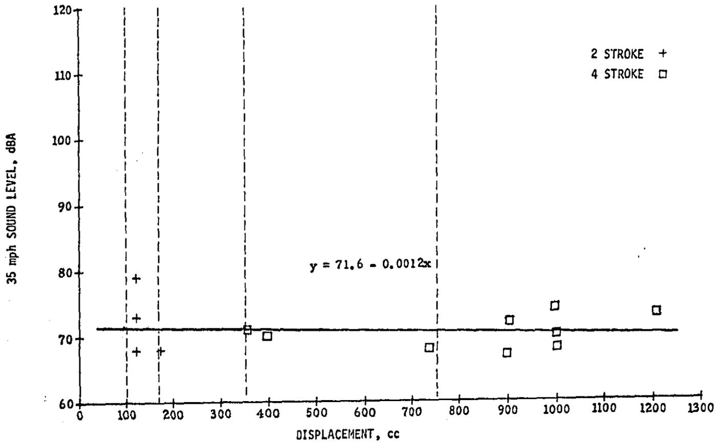
FIGURE 4-9 35 mph SOUND LEVELS, STREET AND COMBINATION STREET/OFF-ROAD '75-'76 YR. OF MFG. MOTORCYCLES
