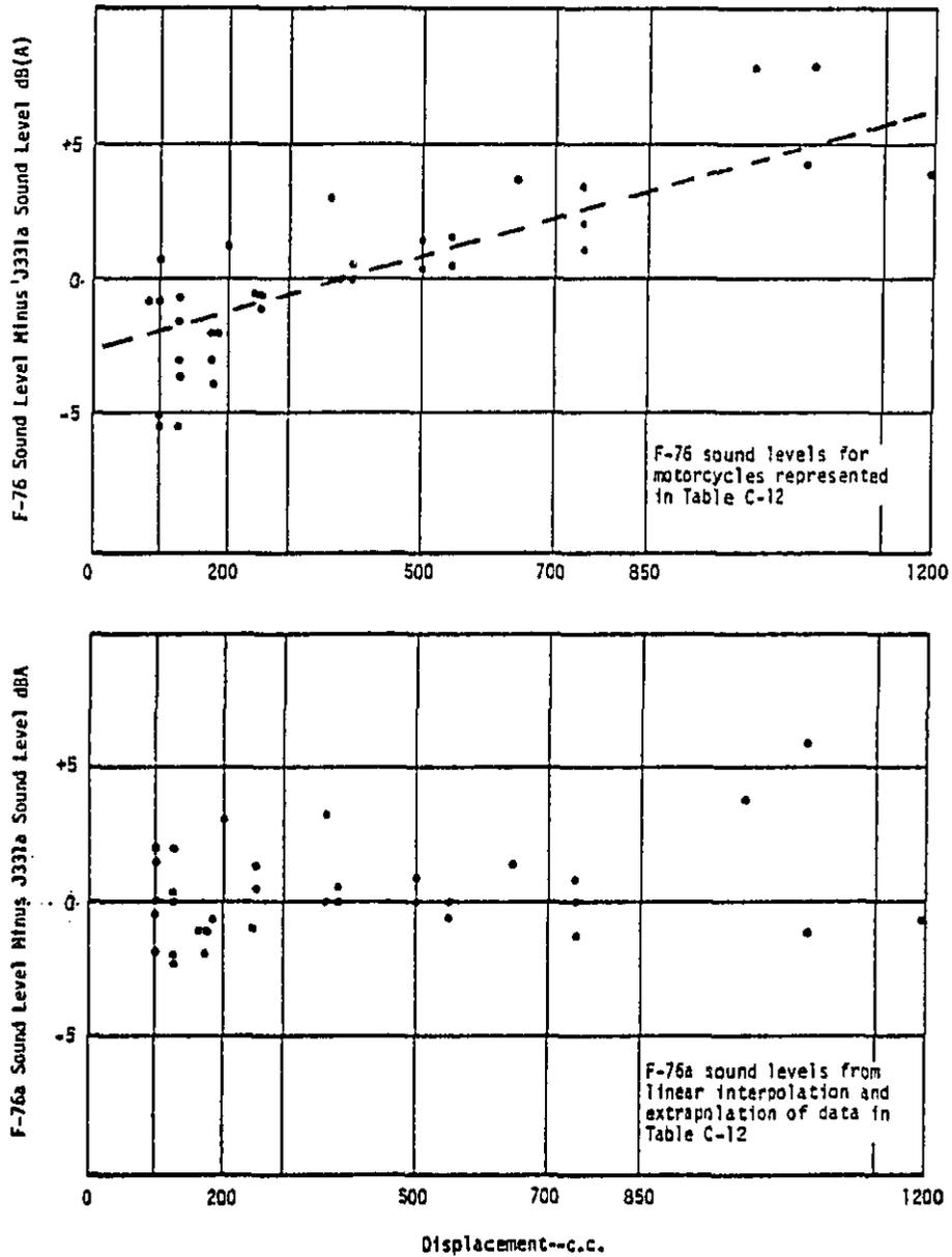
FIGURE 3-4. COMPARISON OF F76 AND F-76a SOUND LEVELS
