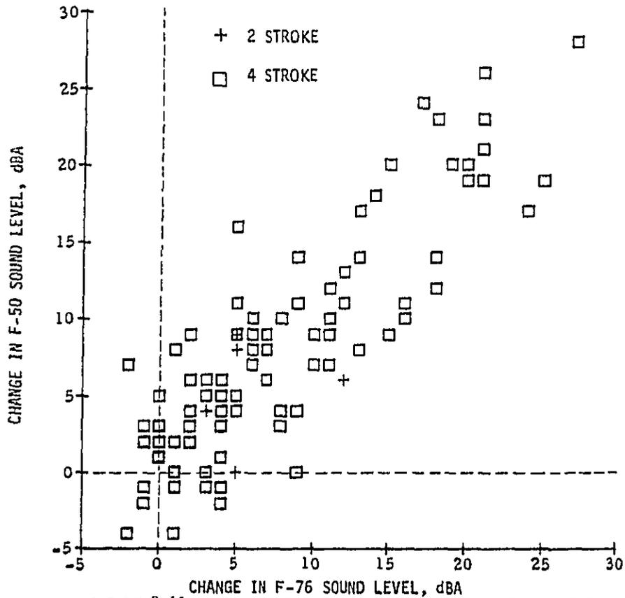
FIGURE 3-11 CORRELATION BETWEEN CHANGE IN F-50 SOUND LEVEL COMPARED TO CHANGE IN F-76 SOUND LEVEL, AFTERMARKET AND MODIFIED CONFIGURATIONS REFERRED TO ORIGINAL MANUFACTURE
