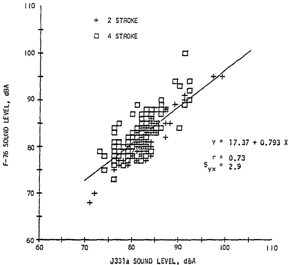
FIGURE 3-1 CORRELATION BETWEEN F-76 AND J331a TESTS, STREET AND COMBINATION STREET/OFF-ROAD '75-'76 YR. OF MFG. MOTORCYCLES
