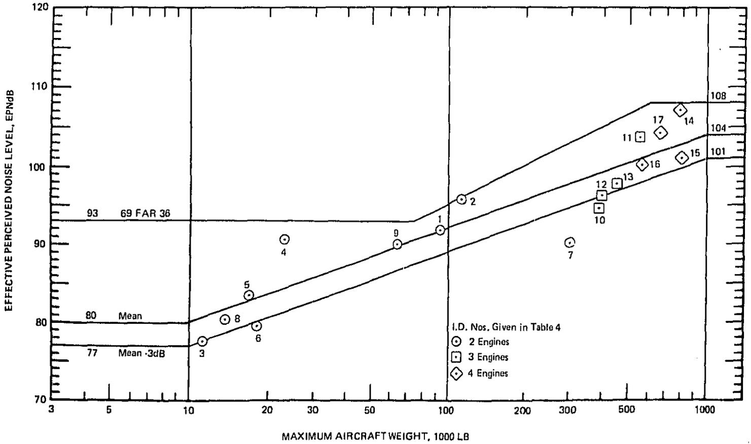
FIGURE 5. NOISE LEVELS VS WEIGHT FOR CURRENT TECHNOLOGY EXISTING AIRPLANES.
