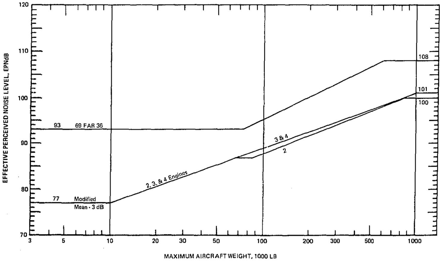
FIGURE 9. MODIFIED MEAN -3 dB NOISE LEVELS FOR AVAILABLE TECHNOLOGY AIRPLANES. (b) TAKEOFF.
