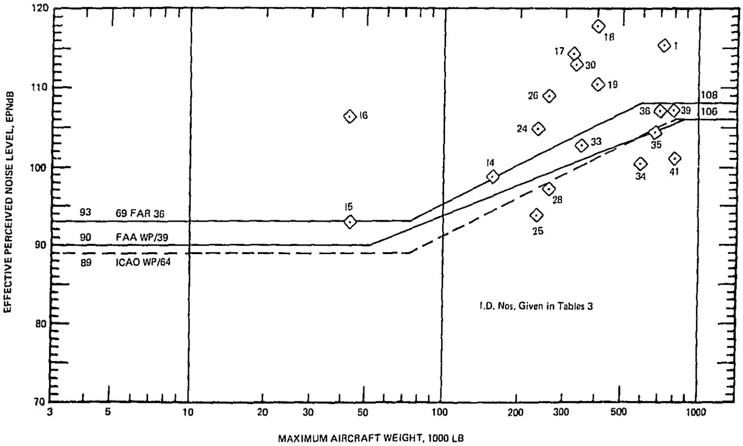
FIGURE 4. AIRPLANE NOISE LEVELS COMPARED TO FAA AND ICAO RECOMMENDATIONS (f) TAKEOFF (4 ENGINES) AT 3.5 NAUTICAL MILES (6,482 METERS).
