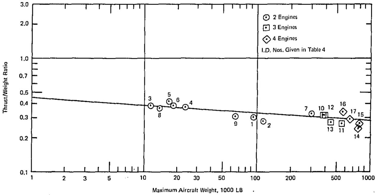
FIGURE 10. PROPULSION VS WEIGHT FOR CURRENT TECHNOLOGY AIRPLANES.
