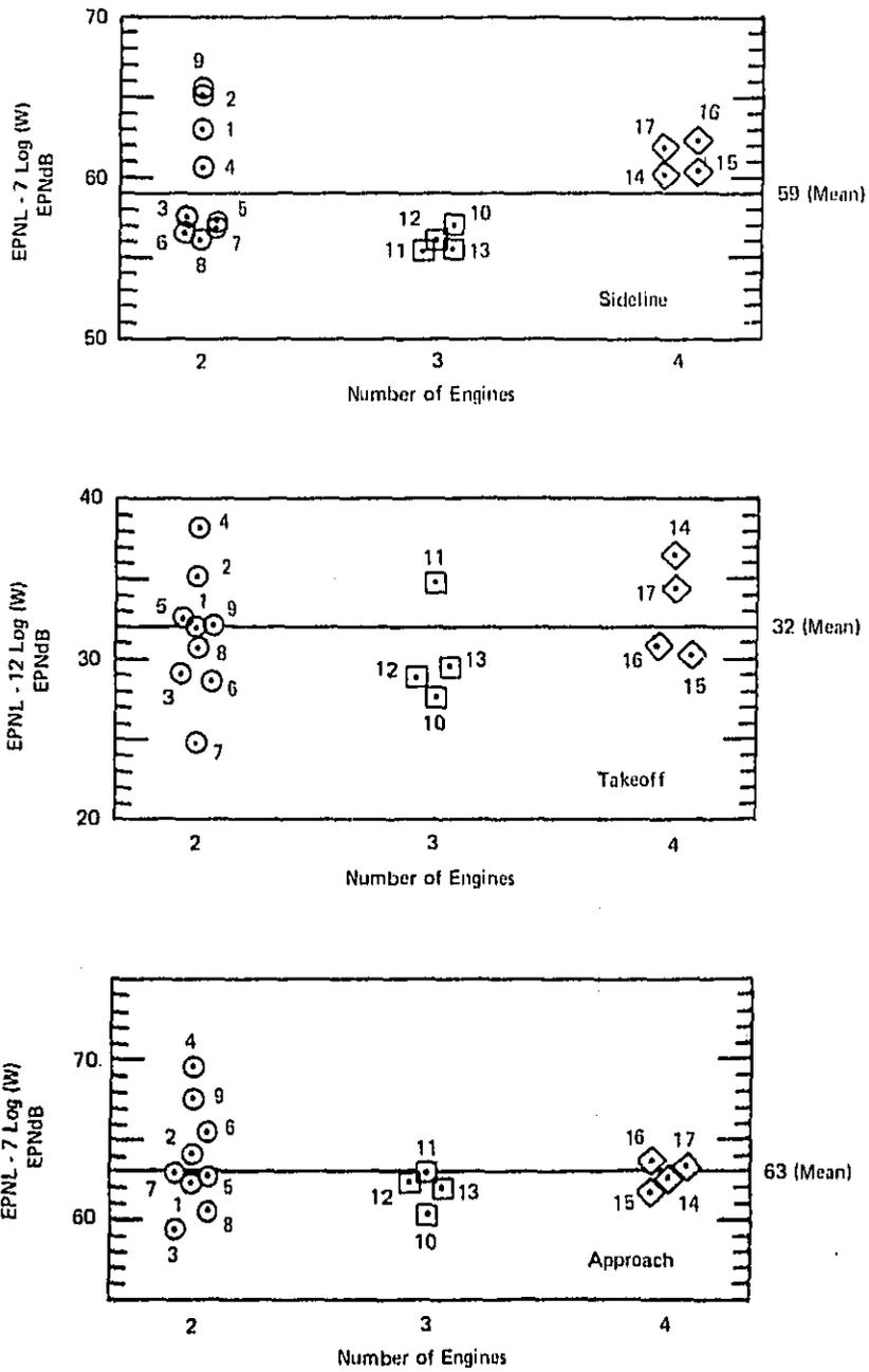
FIGURE 12. NOISE LEVELS VS NUMBER OF ENGINES FOR CURRENT TECHNOLOGY AIRPLANES.
