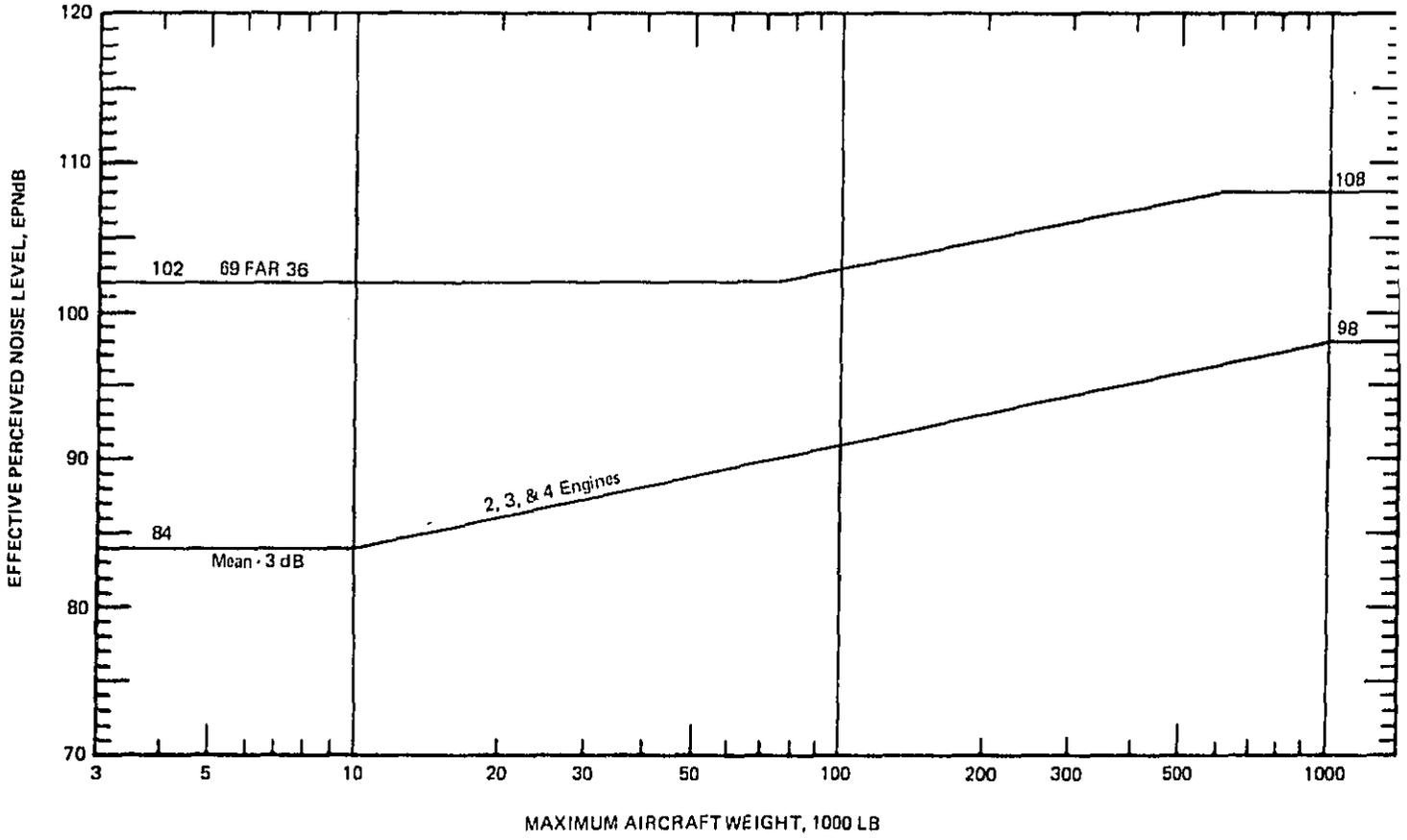
FIGURE 9. MODIFIED MEAN -3dB NOISE LEVELS FOR AVAILABLE TECHNOLOGY AIRPLANES.
