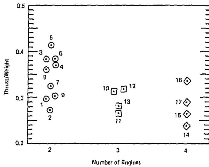
FIGURE 13. THRUST/WEIGHT RATIO VS NUMBER OF ENGINES FOR CURRENT TECHNOLOGY AIRPLANES.
