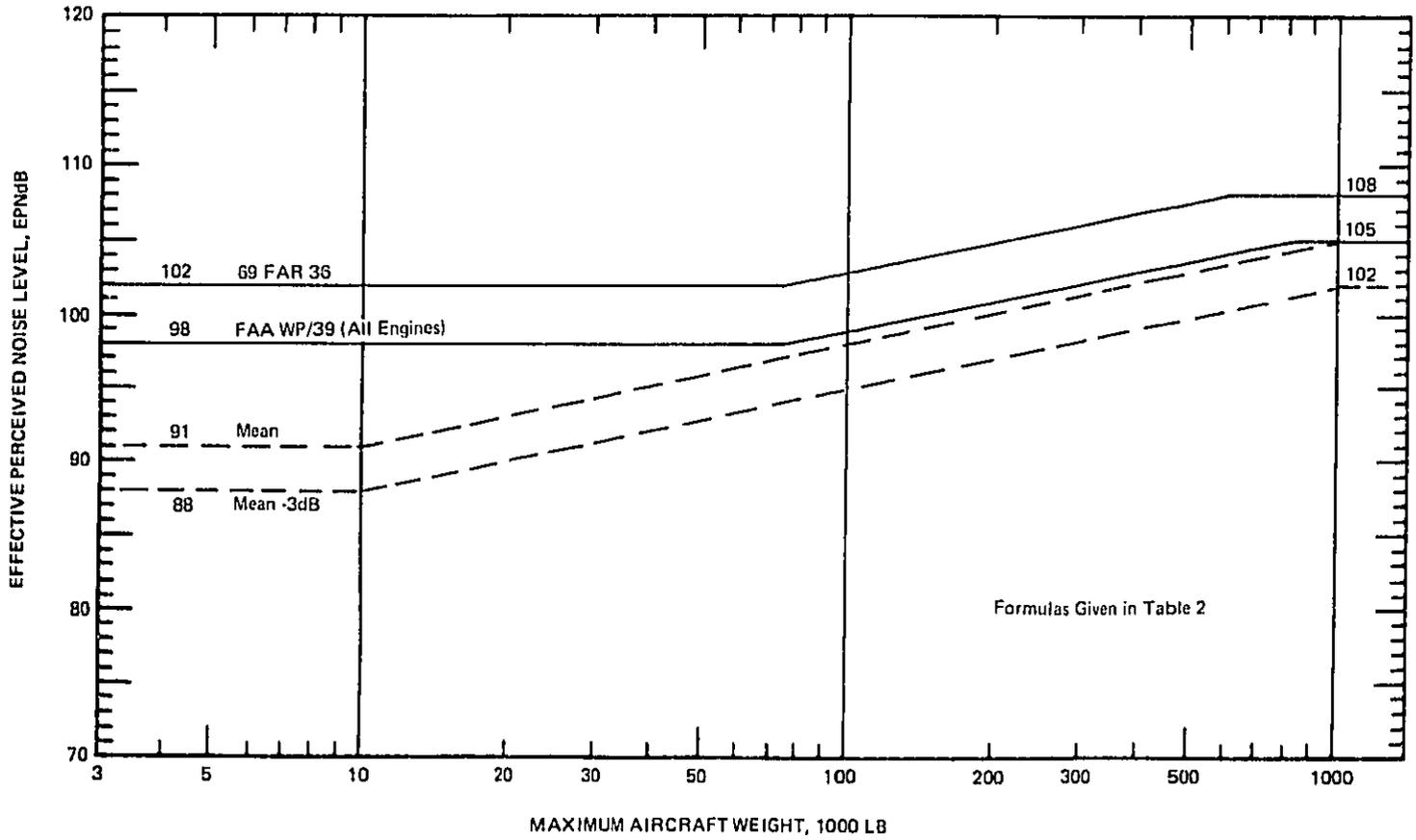
FIGURE 6. COMPARISON OF FAA LEVELS WITH MEAN LEVELS OF CURRENT TECHNOLOGY AIRPLANES.
