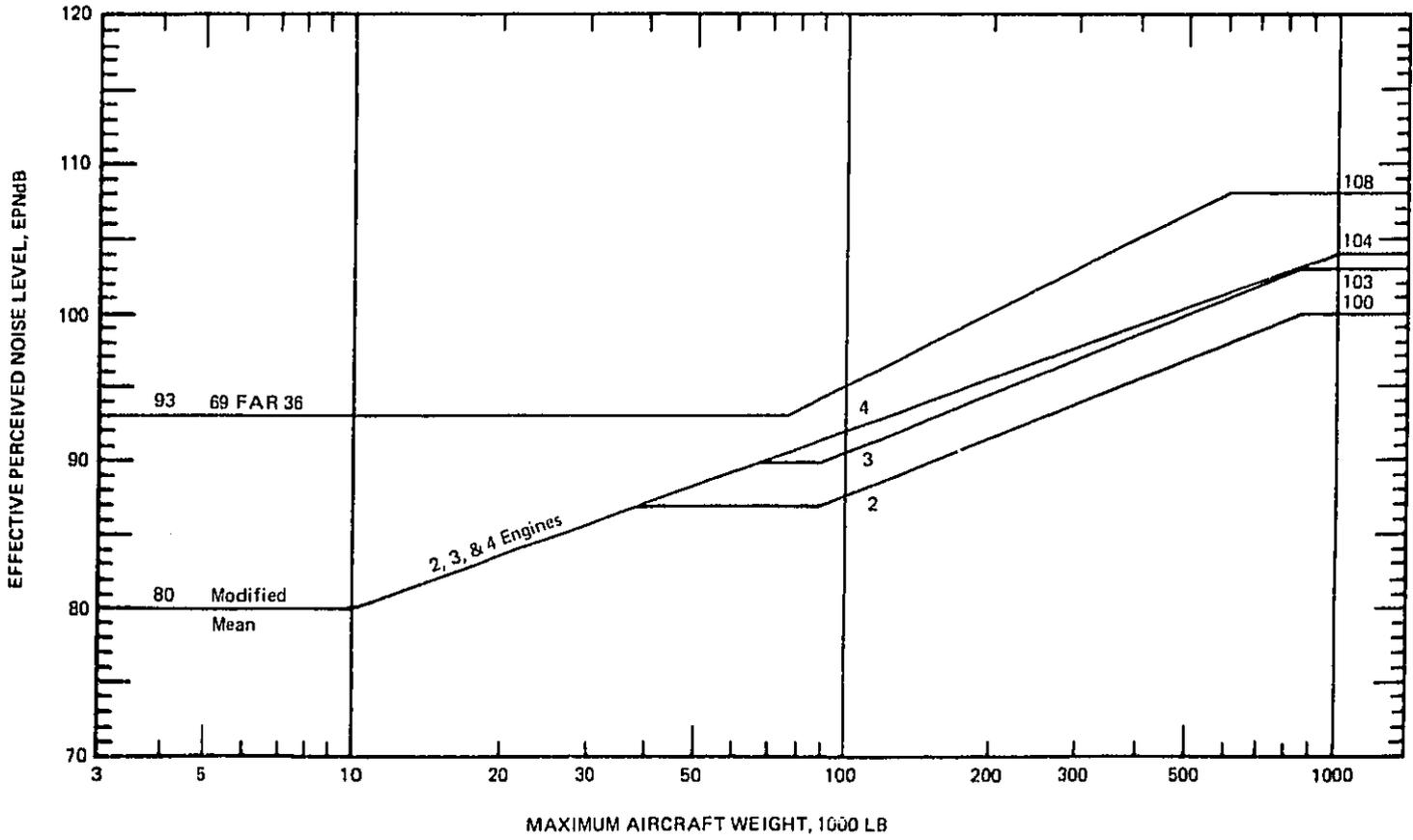
FIGURE 8. MODIFIED MEAN NOISE LEVELS FOR CURRENT TECHNOLOGY AIRPLANES.
