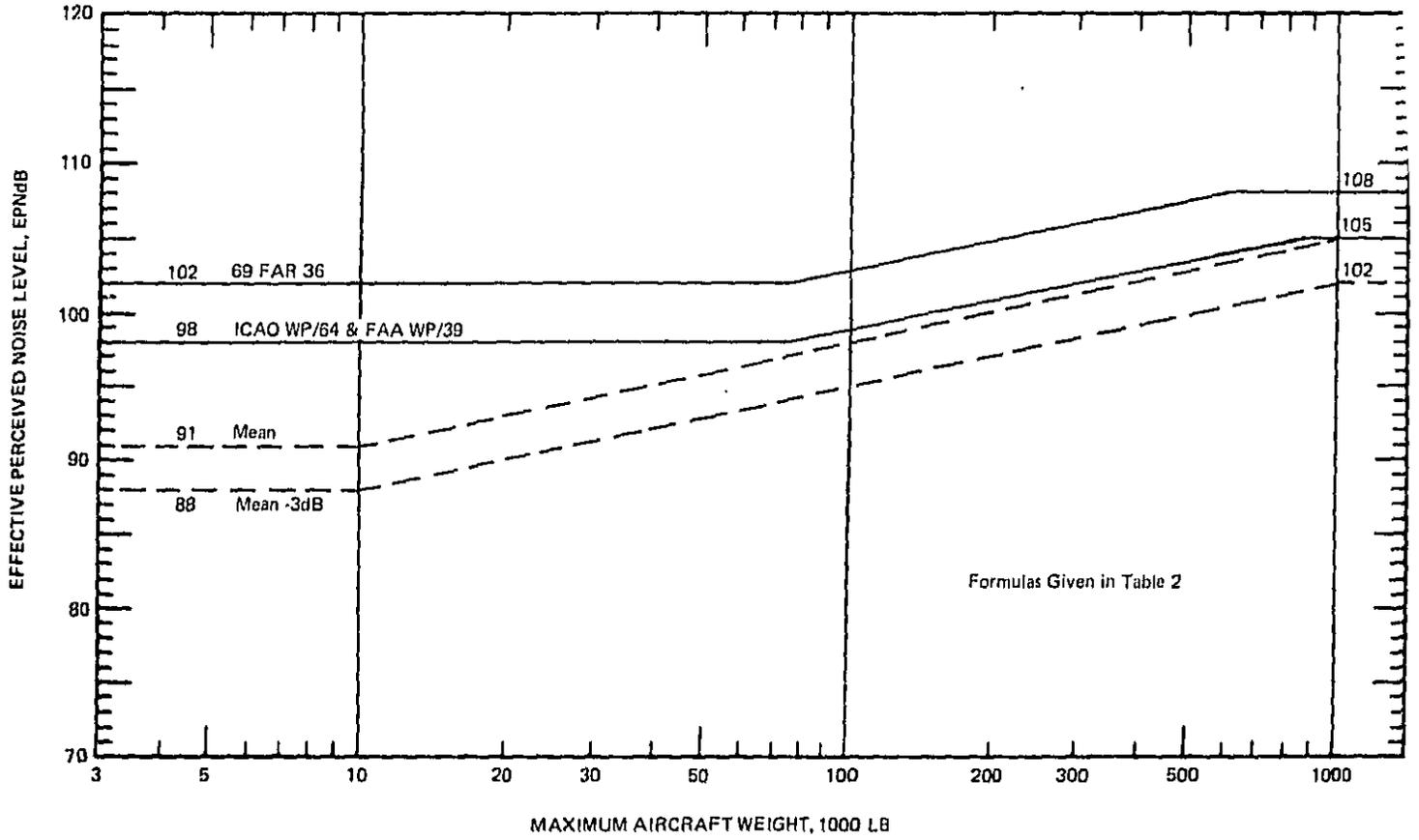
FIGURE 7. COMPARISON OF ICAO LEVELS WITH MEAN LEVELS OF CURRENT TECHNOLOGY AIRPLANES.
