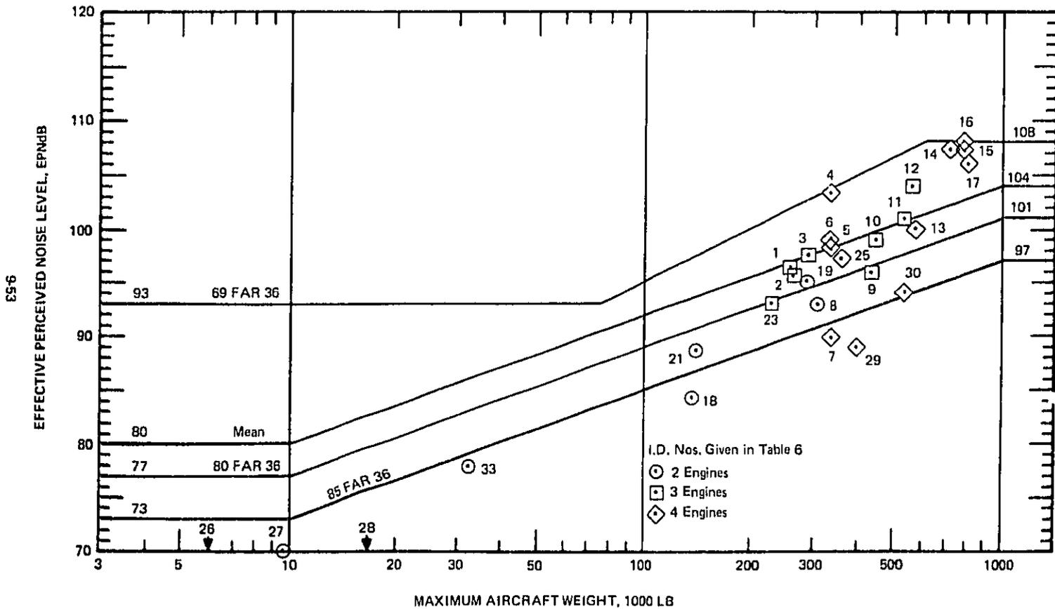
FIGURE 19. PREDICTED NOISE LEVELS FOR NEW TYPE DESIGN AIRPLANES.
