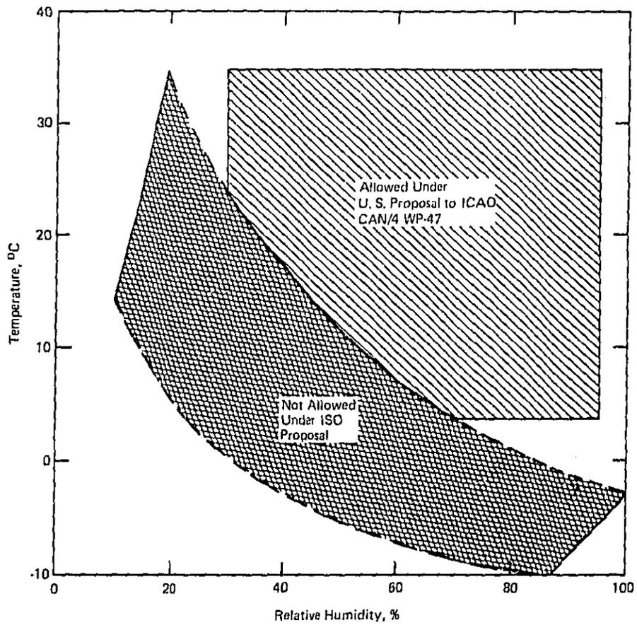
FIGURE 1. COMPARISON OF ISO AND ICAO PROPOSALS FOR TEMPERATURE AND RELATIVE HUMIDITY TEST CONDITIONS.
