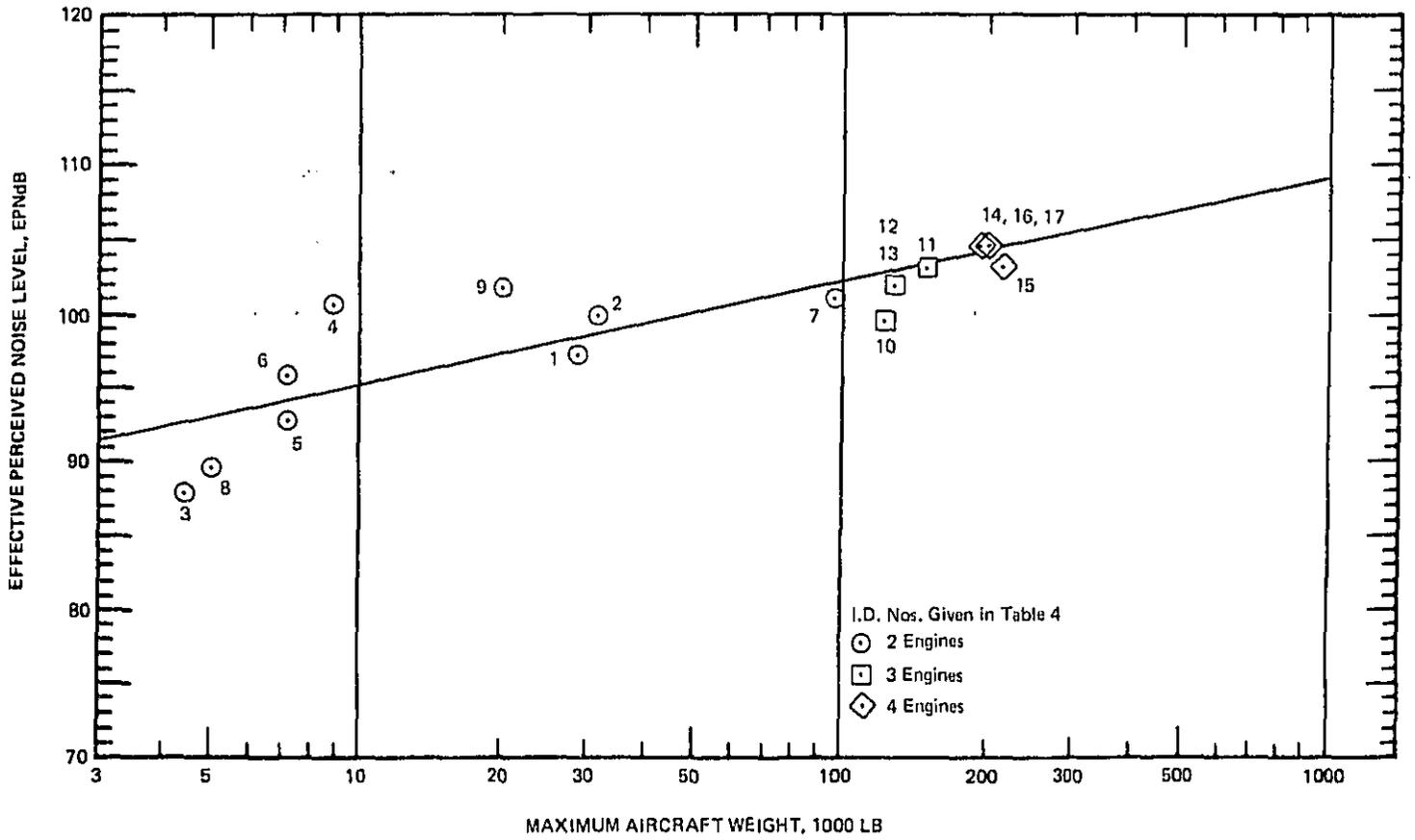
FIGURE 11. NOISE LEVELS VS THRUST FOR CURRENT TECHNOLOGY AIRPLANES.
