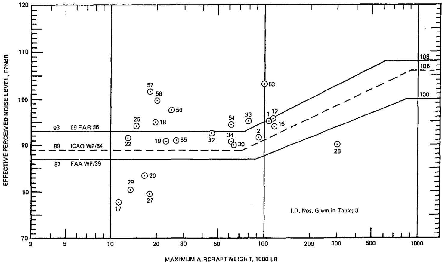
FIGURE 4. AIRPLANE NOISE LEVELS COMPARED TO FAA AND ICAO RECOMMENDATIONS.
