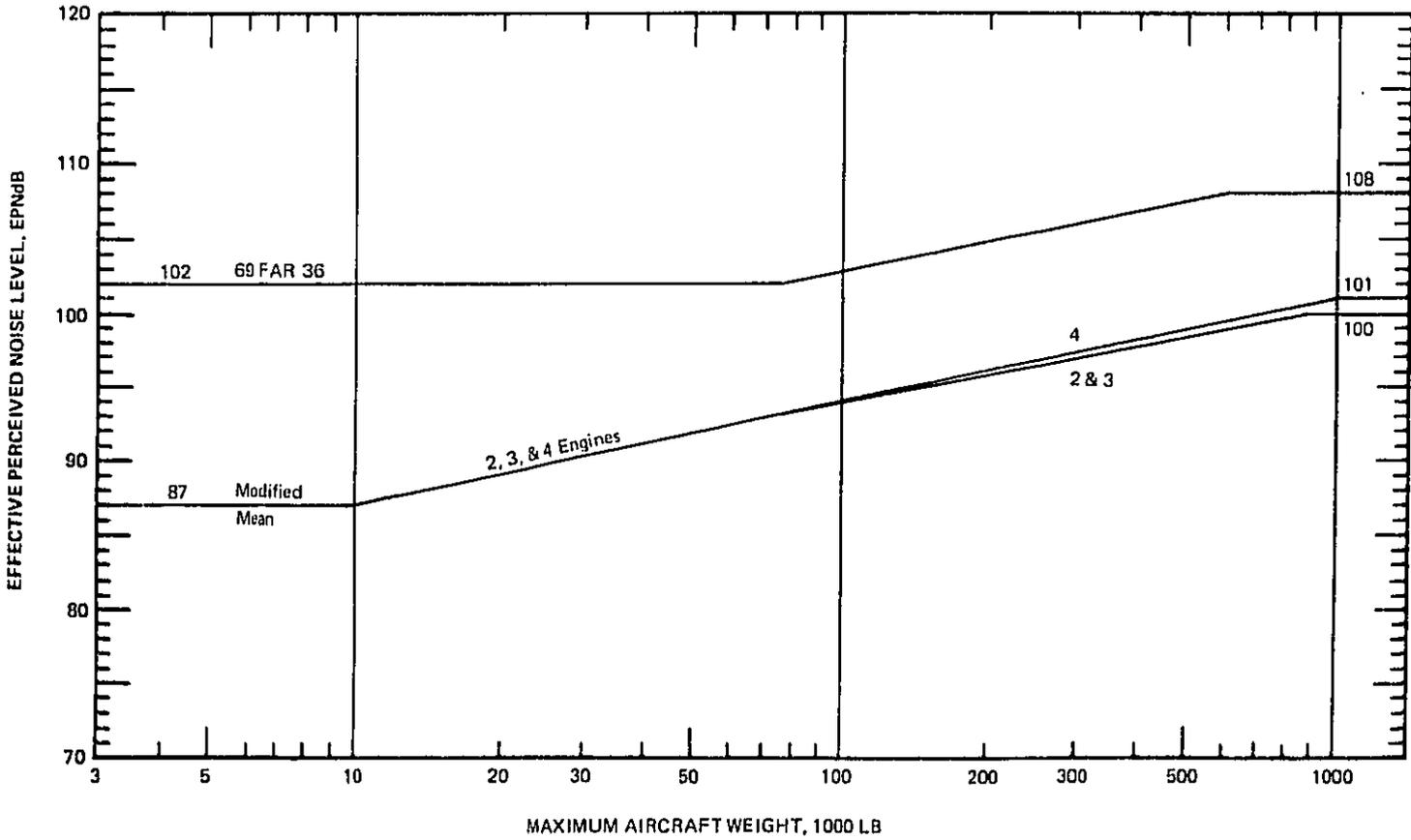
FIGURE B. MODIFIED MEAN NOISE LEVELS FOR CURRENT TECHNOLOGY AIRPLANES.
