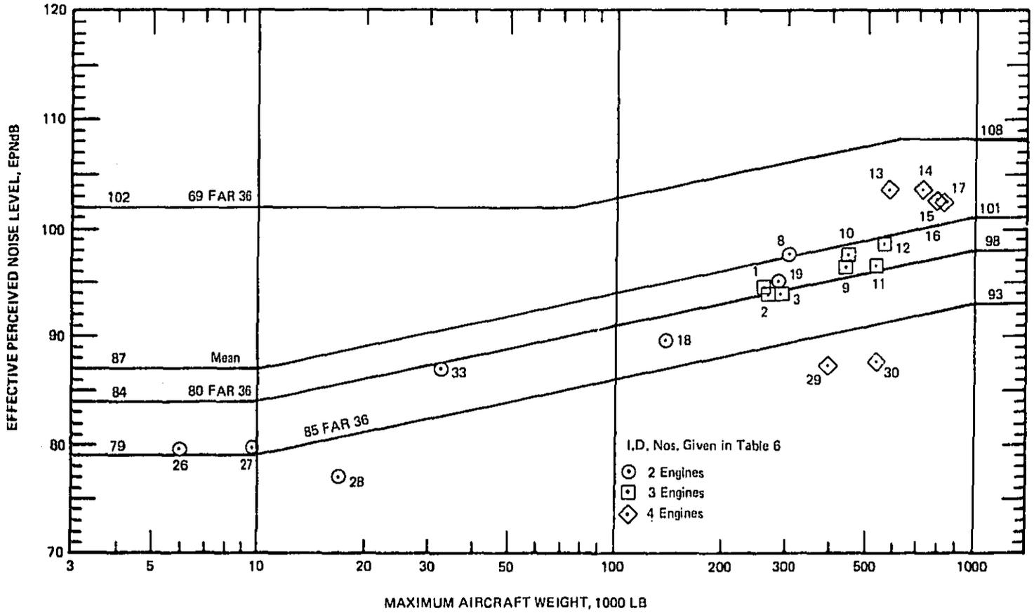
FIGURE 19. PREDICTED NOISE LEVELS FOR NEW TYPE DESIGN AIRPLANES.
