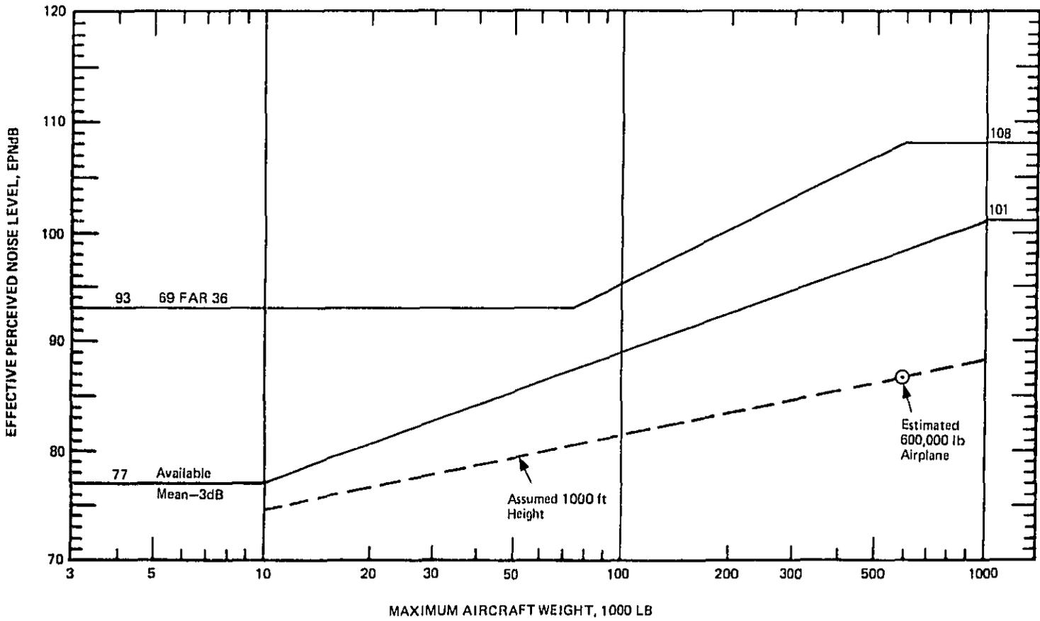
FIGURE 15. NONPROPULSIVE NOISE FLOOR FOR AERODYNAMICALLY CLEAN AIRPLANES.
