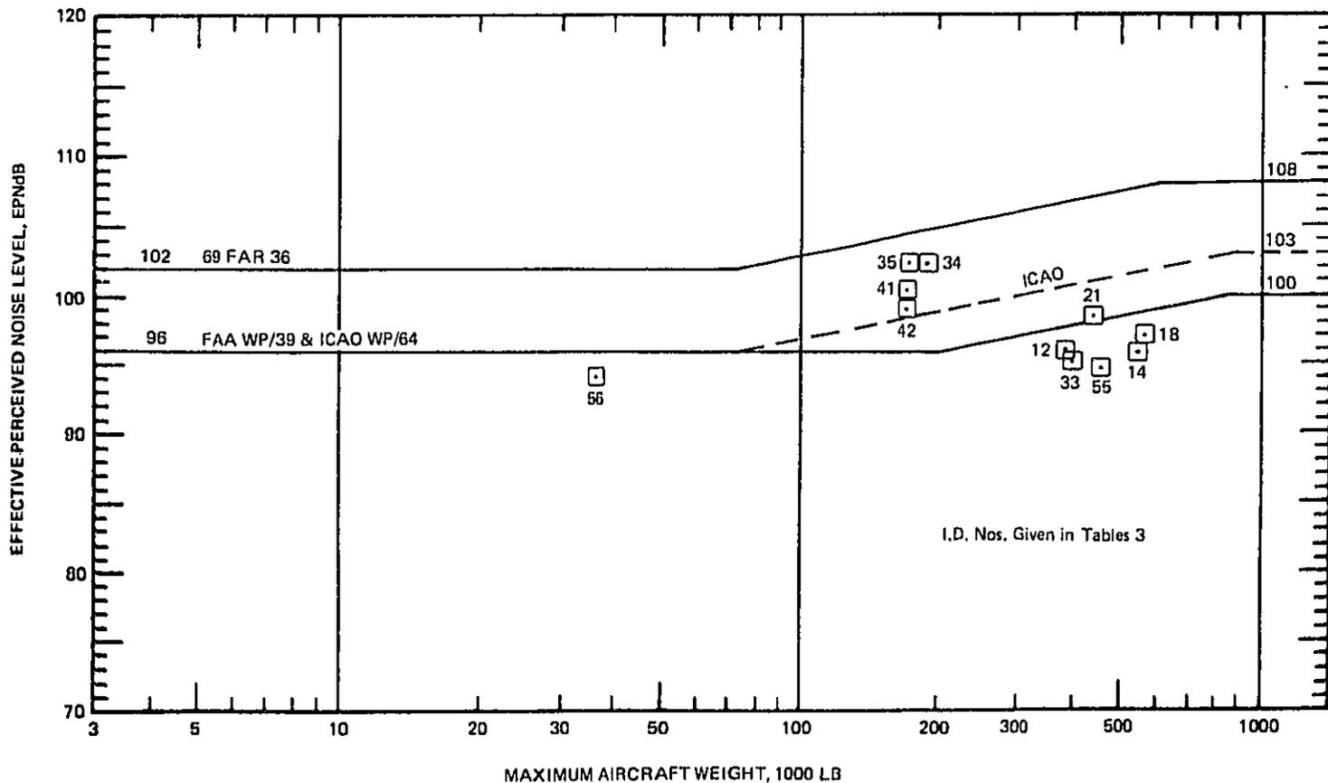
FIGURE 4. AIRPLANE NOISE LEVELS COMPARED TO FAA AND ICAO RECOMMENDATIONS.
