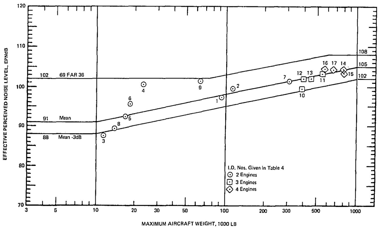
FIGURE 5. NOISE LEVELS VS WEIGHT FOR CURRENT TECHNOLOGY EXISTING AIRPLANES.
