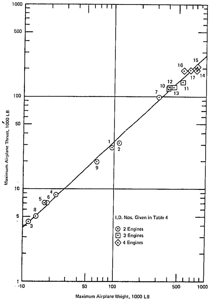
FIGURE 10. PROPULSION VS WEIGHT FOR CURRENT TECHNOLOGY AIRPLANES.
