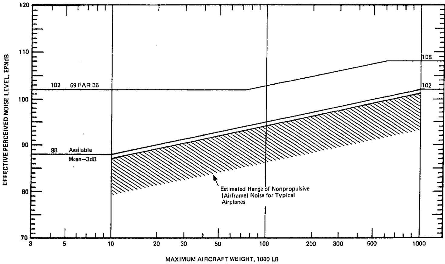
FIGURE 14. NONPROPULSIVE APPROACH NOISE FOR TYPICAL AIRPLANES.
