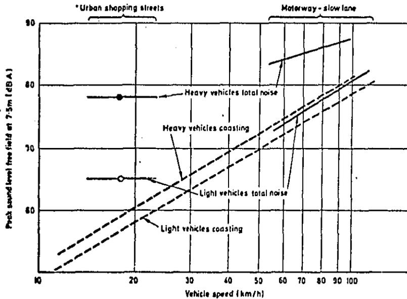
Figure 5-8. Total Vehicle Noise and Coasting Noise
