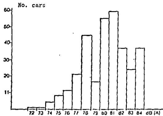
Figure 5-3. Sound Levels for Cars, Measured During Design Inspections in 1972.
