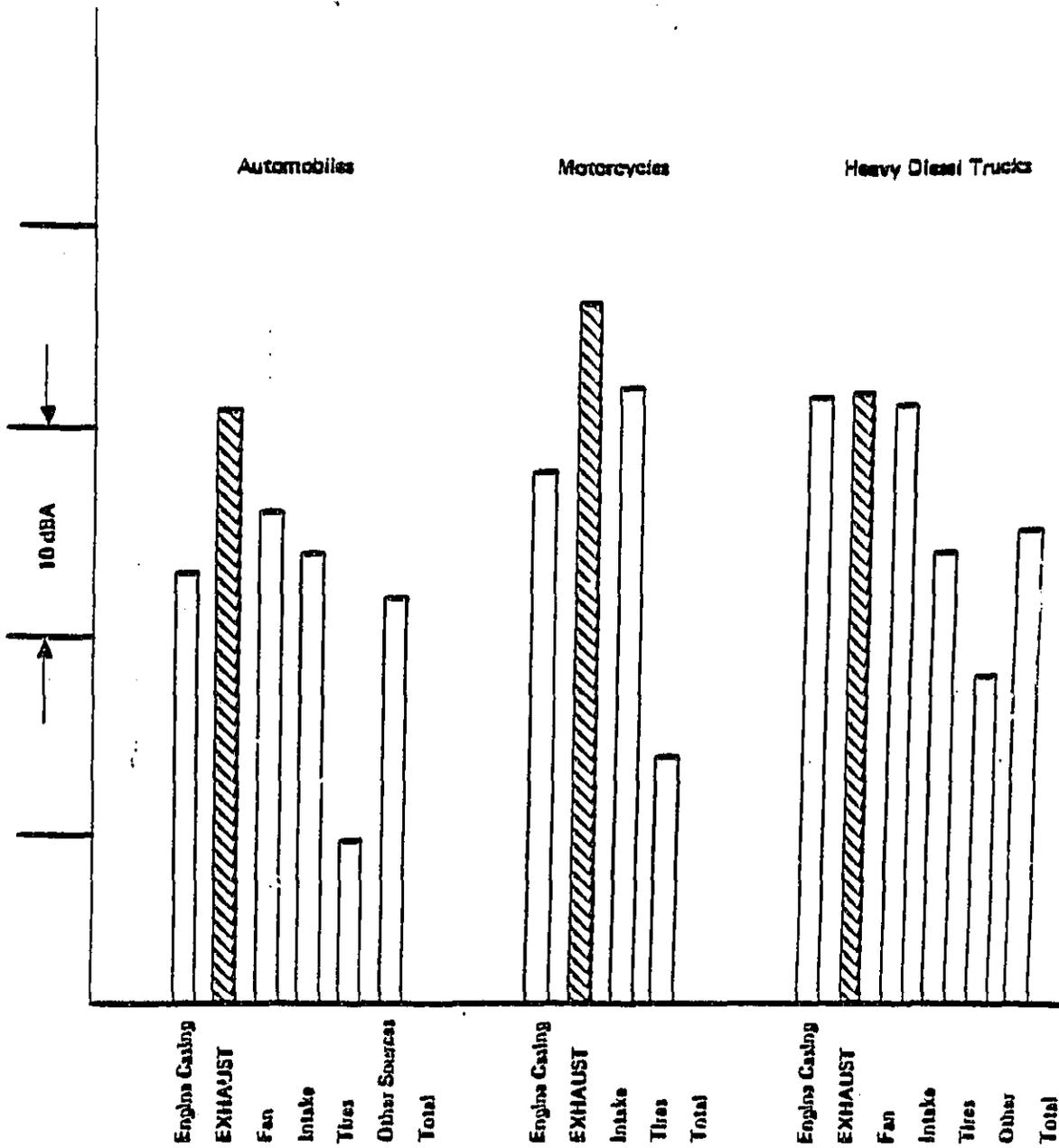
Figure 1-1: Motor Vehicle Noise Sources and Relative Noise Levels
