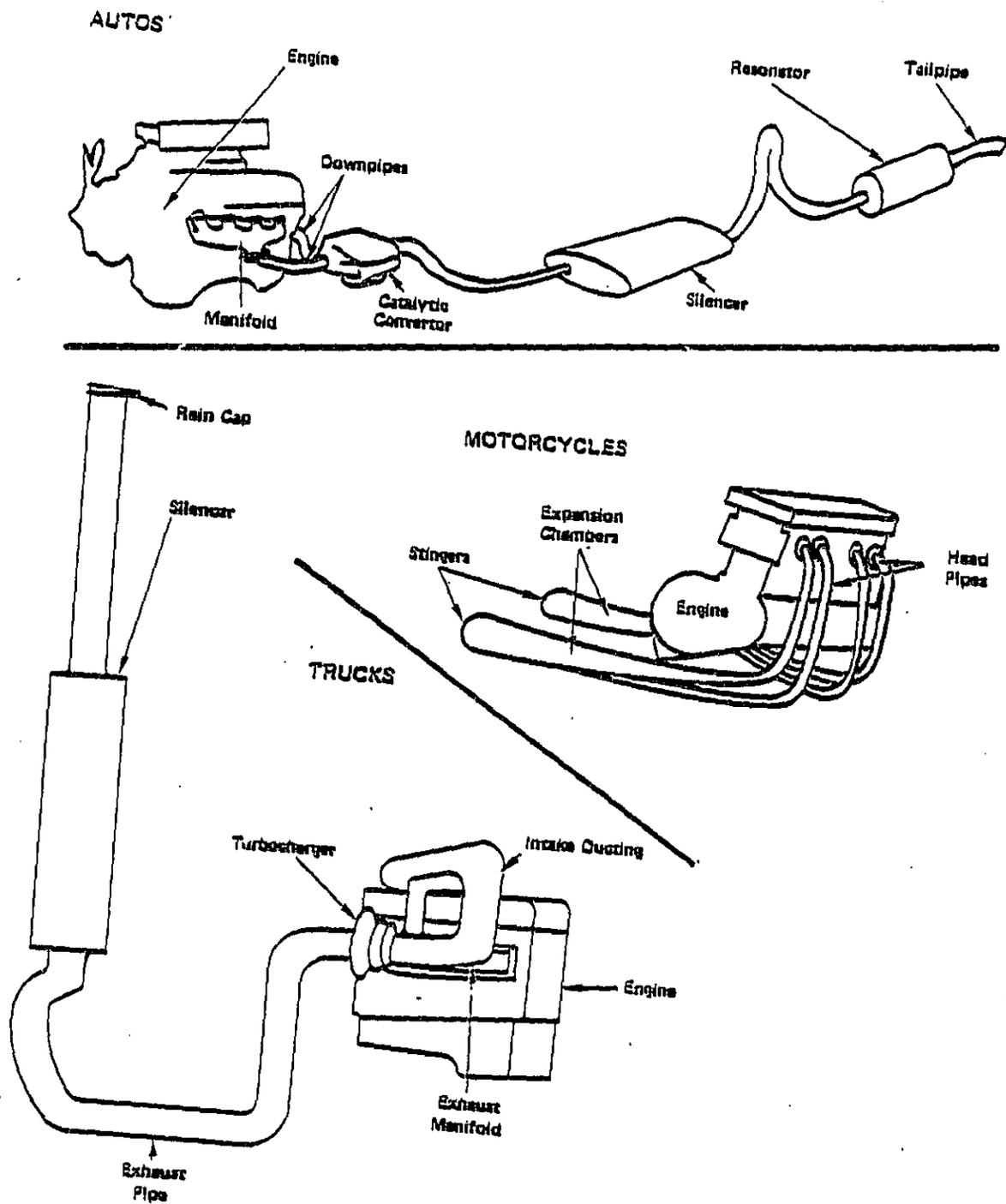
Figure 2-1: Typical Motor Vehicle Exhaust Systems
