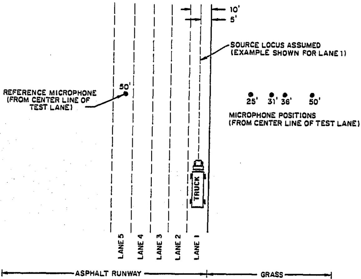
FIG. 4.2. SCHEMATIC DIAGRAM OF TEST SITE WESTFIELD-BARNES AIRPORT, WESTFIELD, MA.
