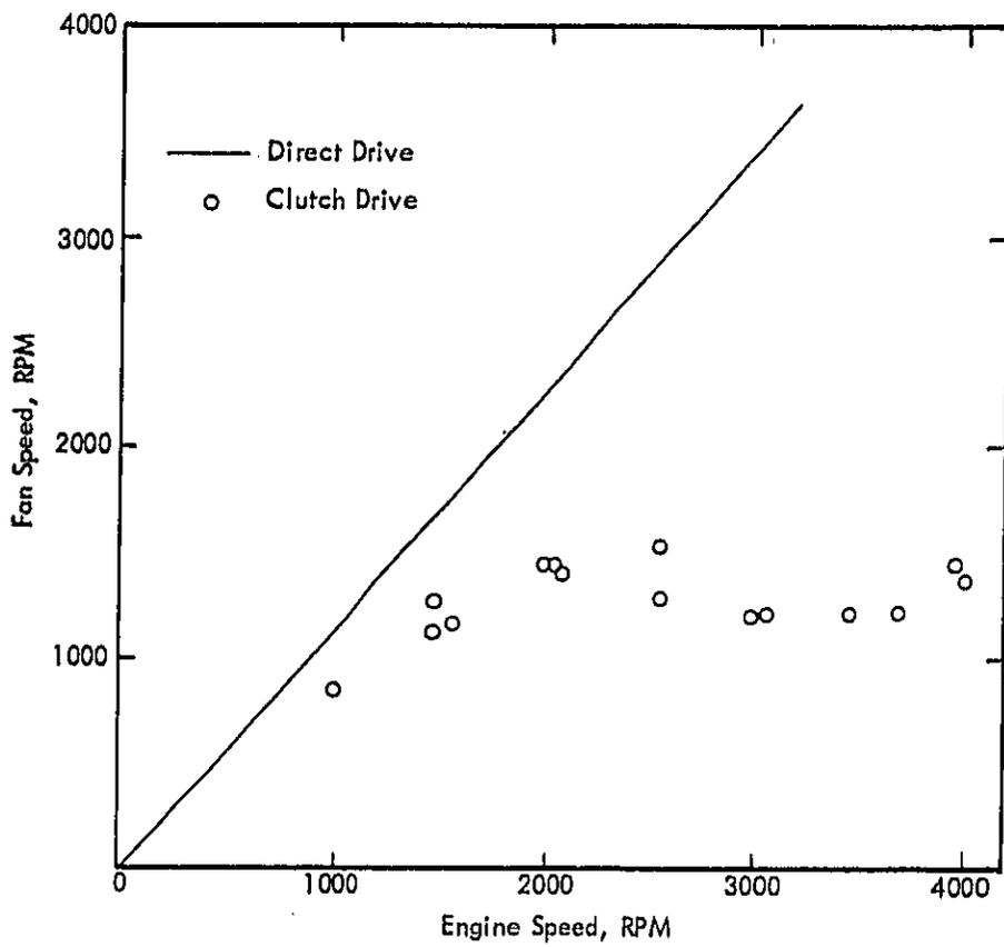
Figure 35. Speed of Clutch Fan and Direct Drive Fan, Ford F-150.
