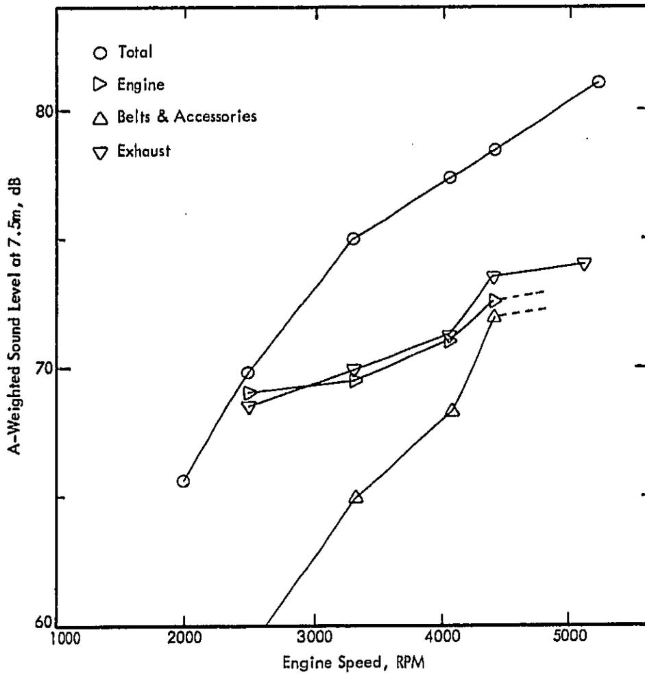
Figure 24. Noise Sources at Full Throttle, Toyota Corolla.
