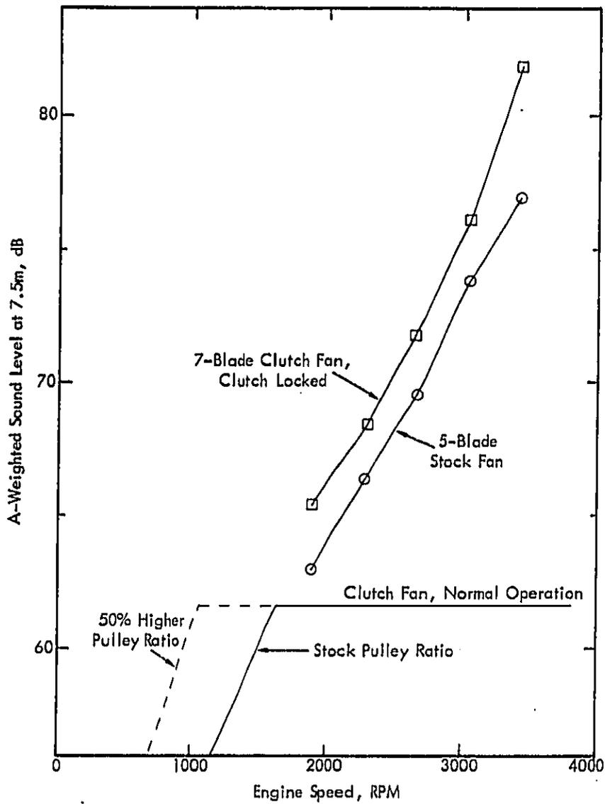
Figure 36. Noise Levels of Stock Fan and Clutch Fan, Ford F-150.
