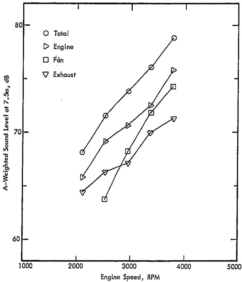
Figure 32. Noise Source Contributions at Partial Throttle, Ford Pinto.
