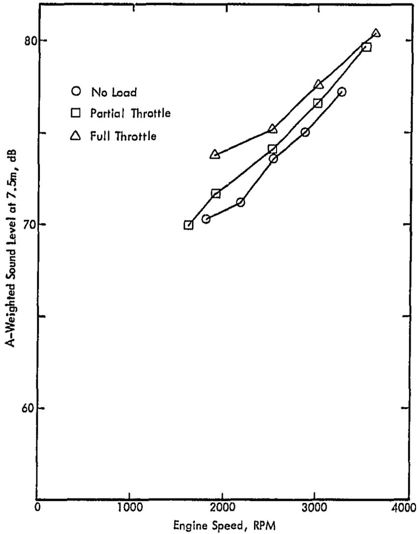
Figure 17. Sideline Noise Characteristics of Oldsmobile Diesel.
