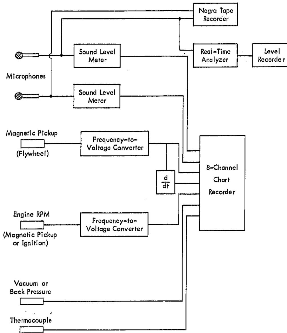
Figure 4. Block Diagram of Instrumentation and Data Acquisition System.
