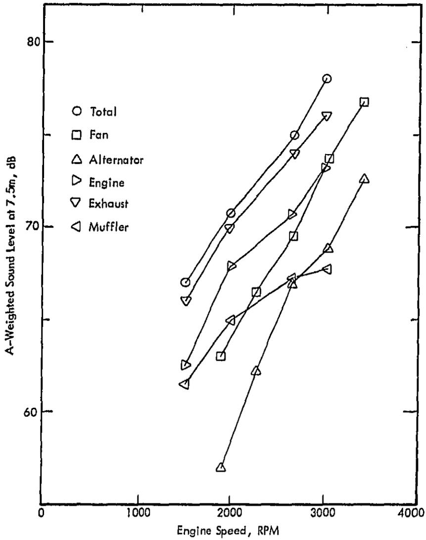
Figure 21. Noise Source Components at Full Throttle, Ford F-150.
