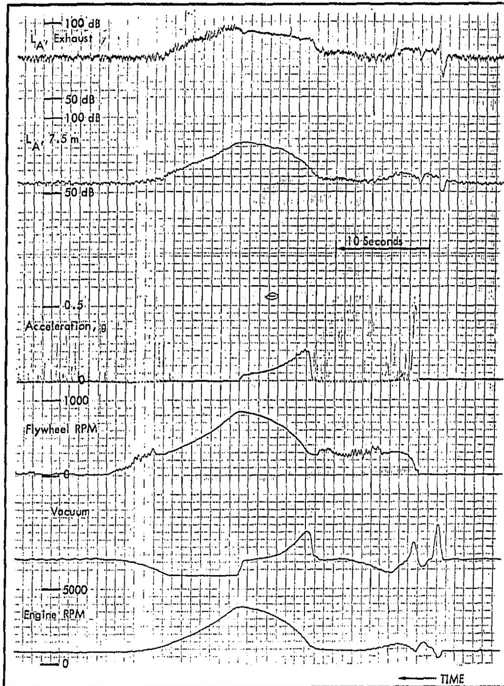
Figure 13. Typical Strip Chart Record, Ford F-150, Partial Throttle (Time - right to left).
