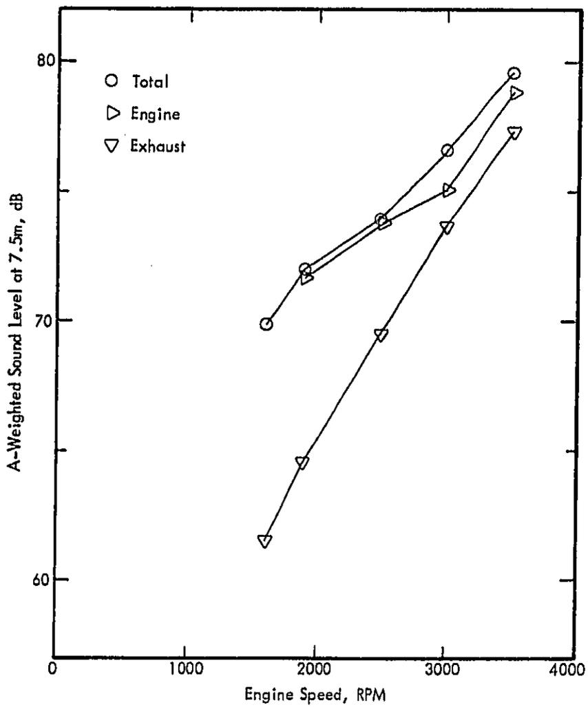
Figure 29. Noise Source Characteristics at Partial Throttle, Oldsmobile Diesel.
