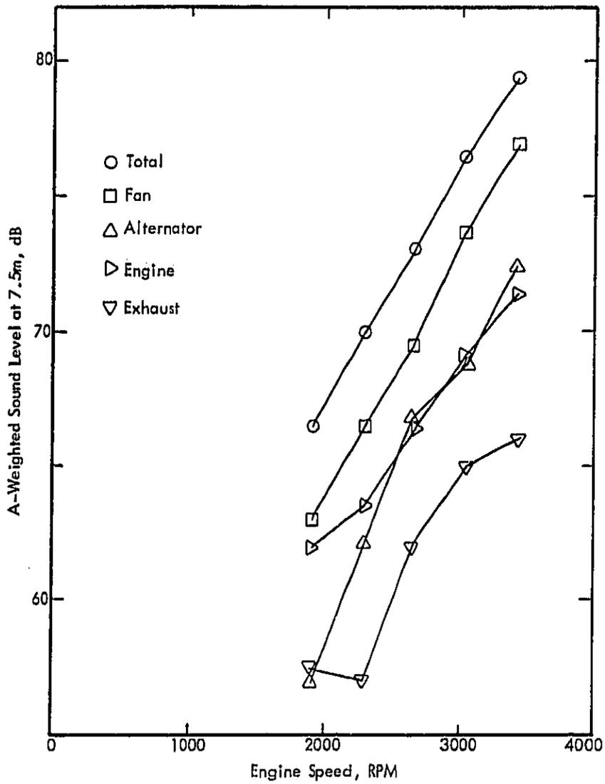
Figure 19. Noise Source Components at No Load, Ford F-150.
