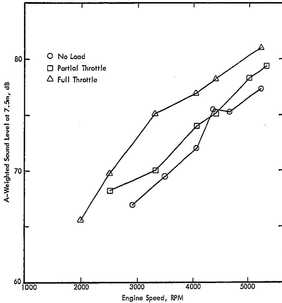
Figure 15. Sideline Noise Characteristics of Toyota Corolla.
