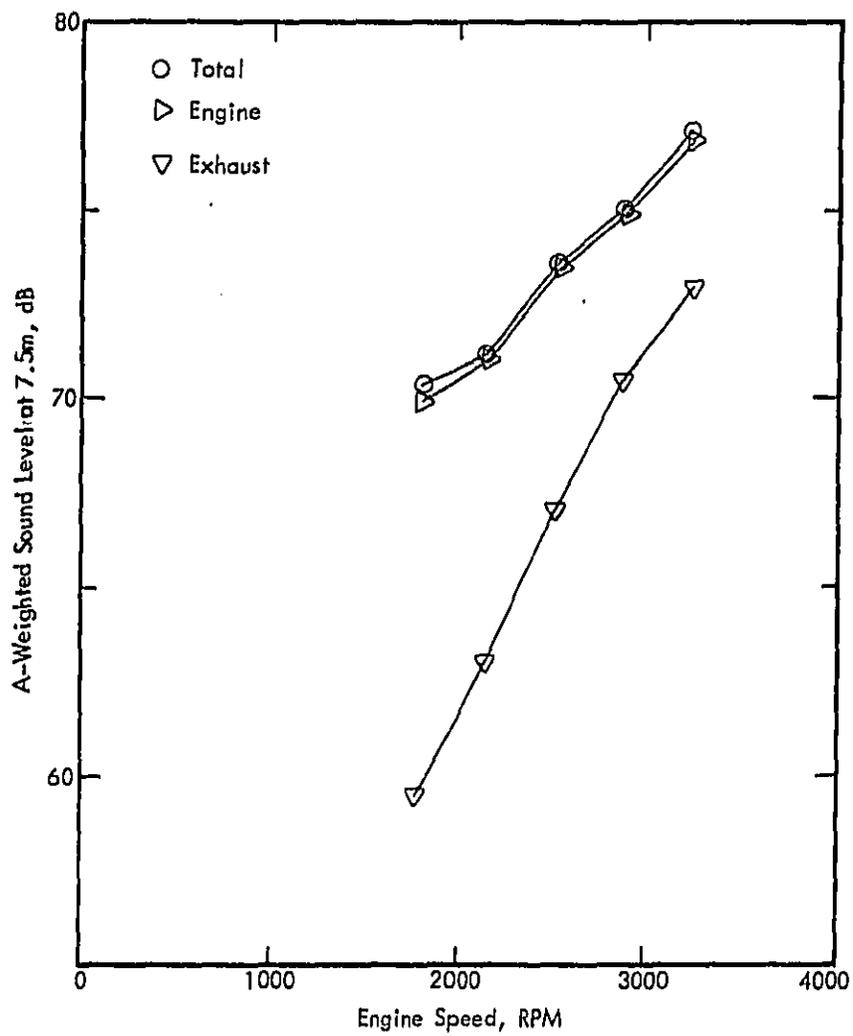
Figure 28. Noise Source Characteristics at No Load, Oldsmobile Diesel.
