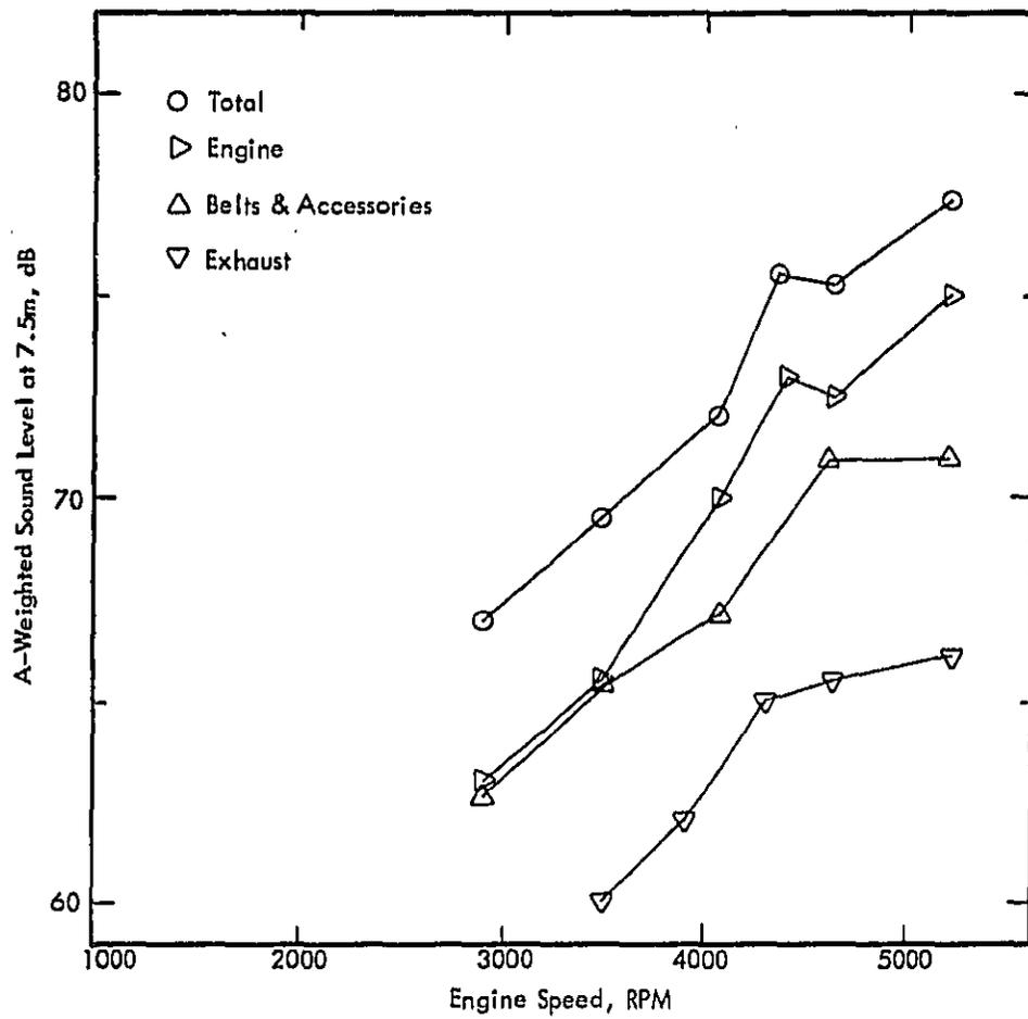
Figure 22. Noise Source Components at No Load, Toyota Corolla.
