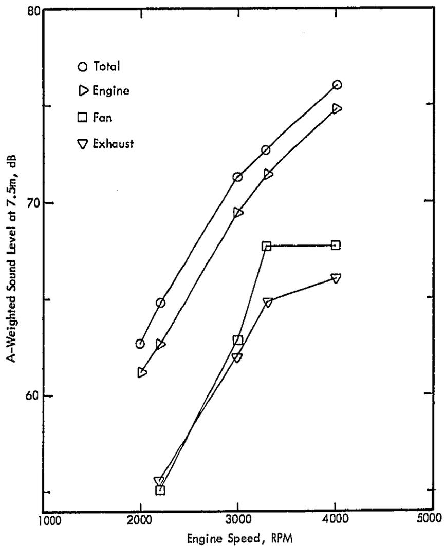
Figure 26. Noise Source Components at Partial Throttle, Chevrolet Chevette.
