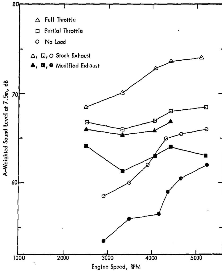
Figure 38. Comparison Between Stock and Modified Exhaust Systems, Toyota Corolla.
