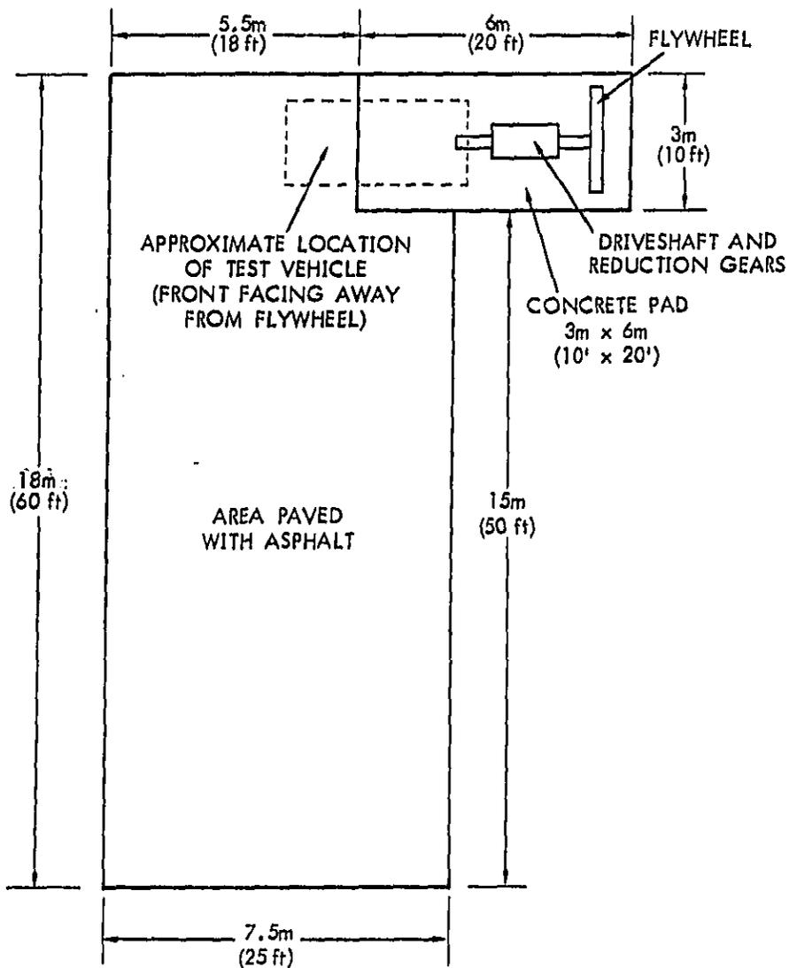
Figure 1. Layout of Inertial Dynamometer Facility.
