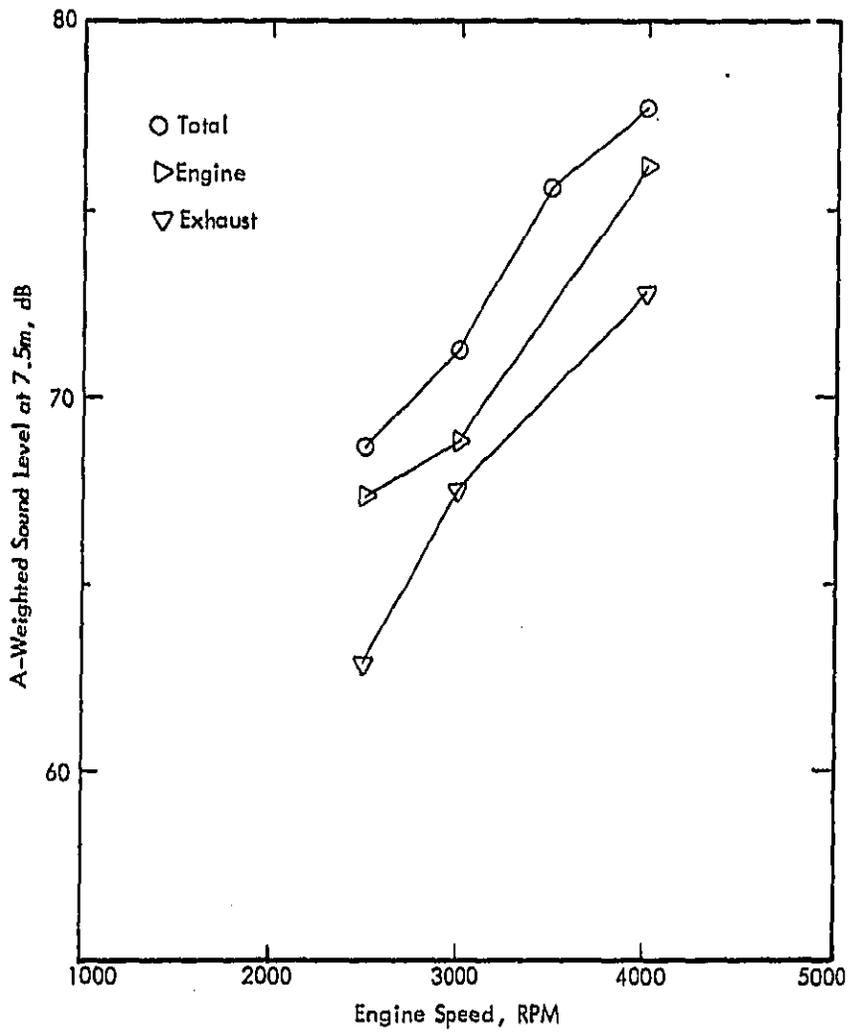
Figure 27. Noise Source Components at Full Throttle, Chevrolet Chevette.
