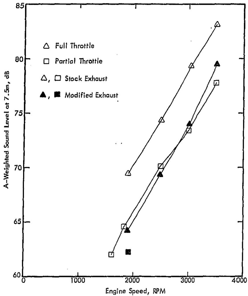
Figure 39. Comparison Between Stock and Modified Exhaust Systems, Oldsmobile Diesel.
