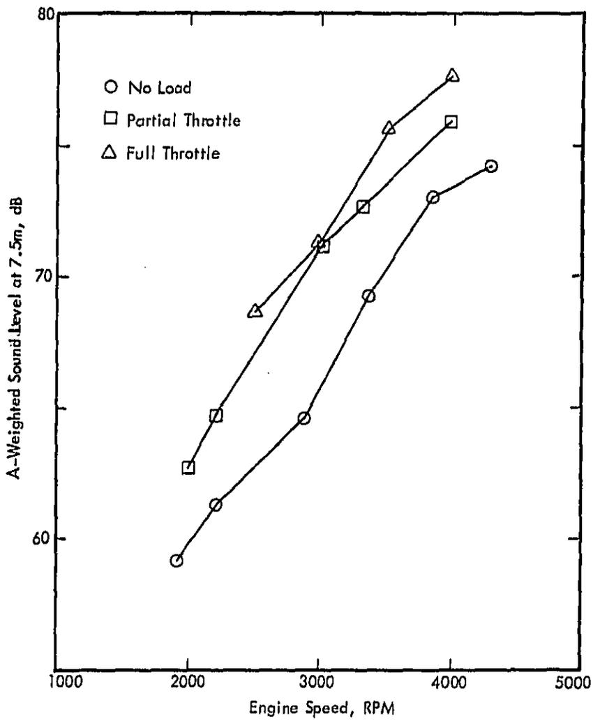
Figure 16. Sideline Noise Characteristics of Chevrolet Chevette.
