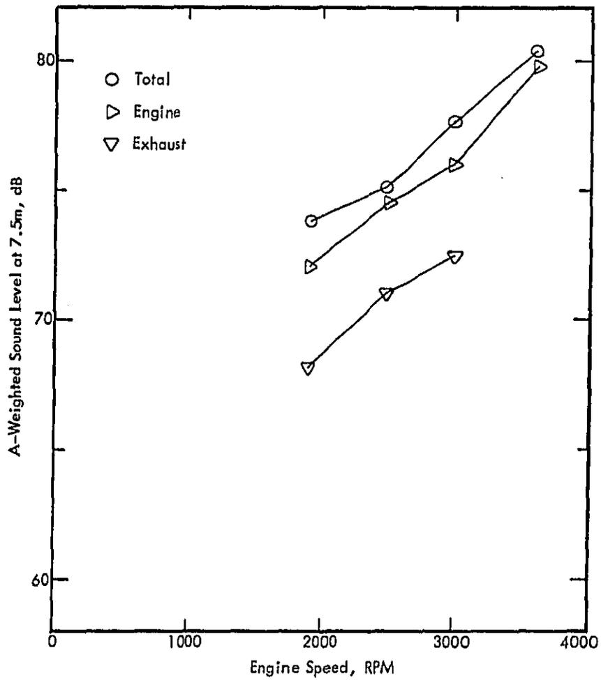
Figure 30. Noise Source Characteristics at Full Throttle, Oldsmobile Diesel.
