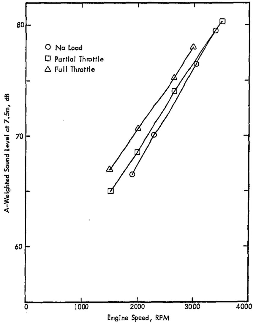
Figure 14. Sideline Noise Characteristics of Ford F-150.
