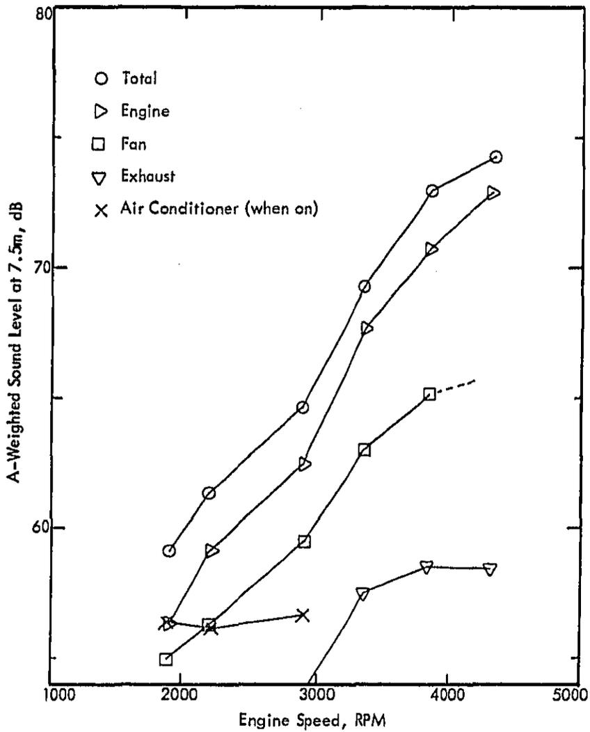
Figure 25. Noise Source Components at No Load, Chevrolet Chevette.
