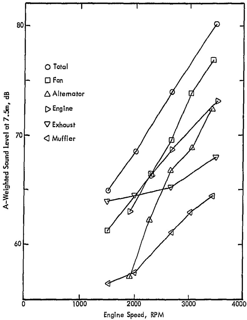
Figure 20. Noise Source Components at Partial Throttle Ford F-150.
