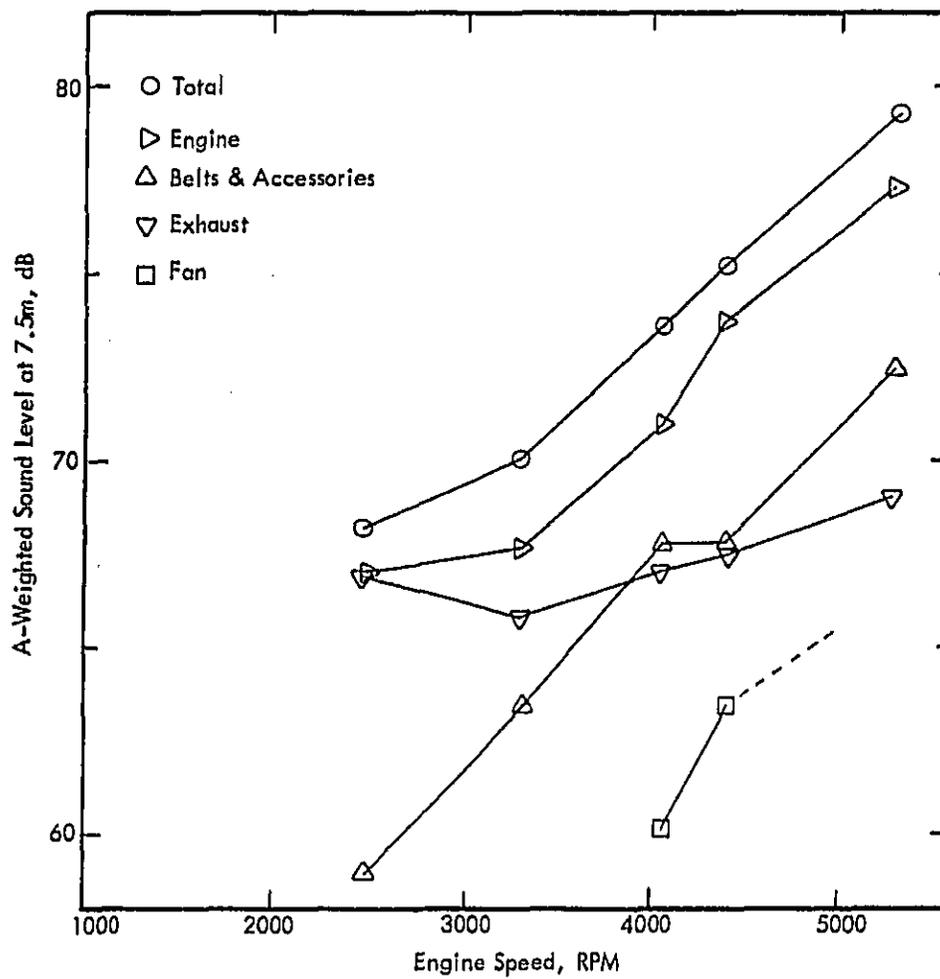
Figure 23. Noise Sources at Partial Throttle, Toyota Corolla.
