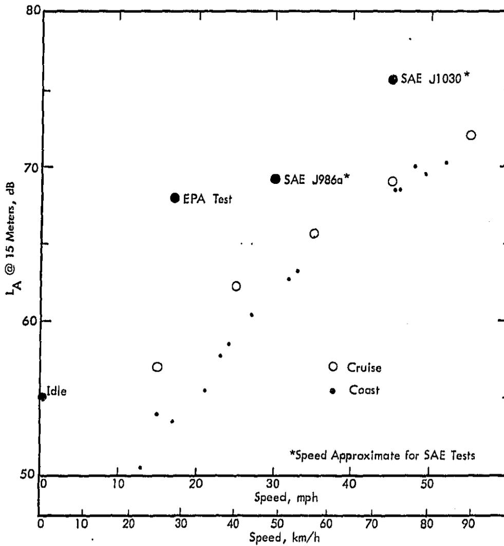
Figure A-3. Cruise and Coast Noise Levels, Turbocharged Diesel Volkswagen Rabbit.
