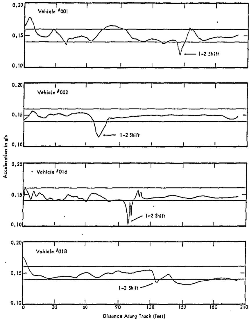
Figure 5.4. Acceleration Traces for Automatics Operating Under Condition 1.0.
