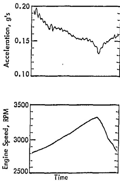
Figure 6.6. Example of Strip-Chart Recording of Engine Speed and Acceleration.
