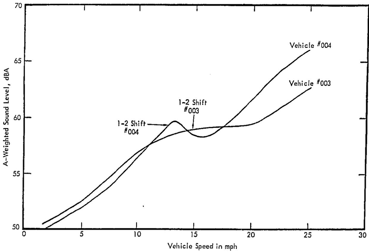
Figure 5.12. Vehicle Sound Levels Before and After the Shift Point.
