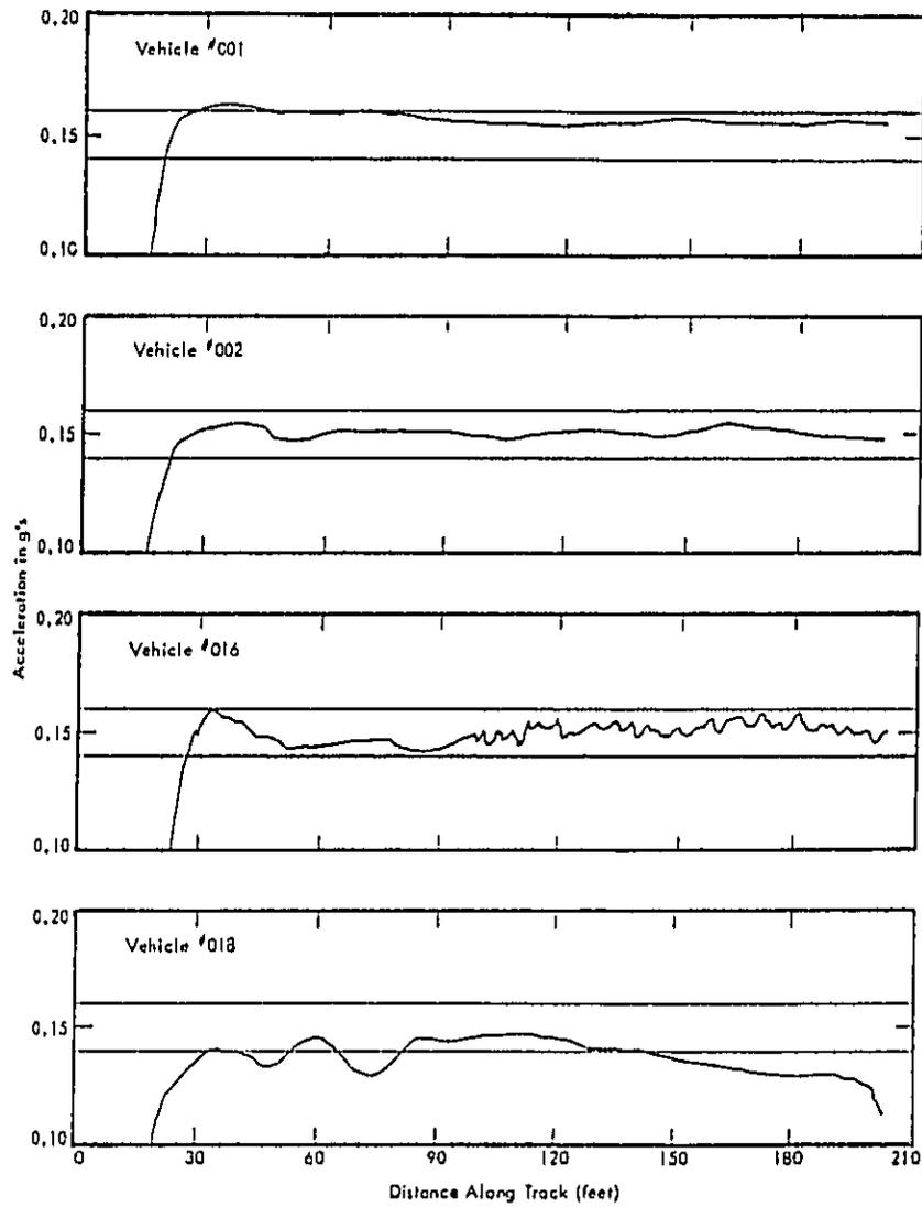
Figure 5.6. Acceleration Traces for Automatics Operating Under Condition 3.0.
