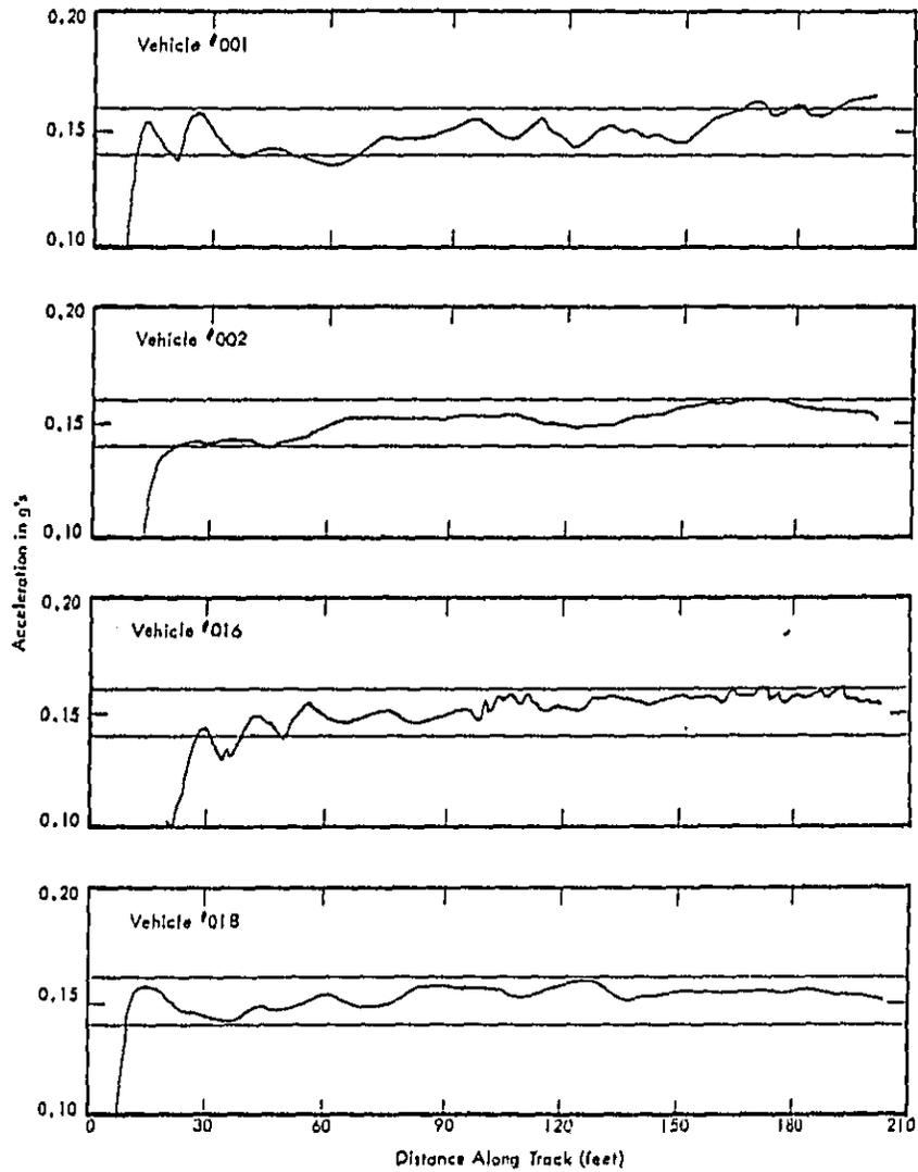
Figure 5.5. Acceleration Traces for Automatics Operating Under Condition 2.0.
