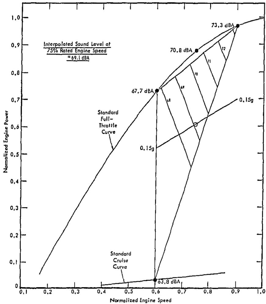
Figure 5.23. Modified Interpolation Graph for Vehicle #011.
