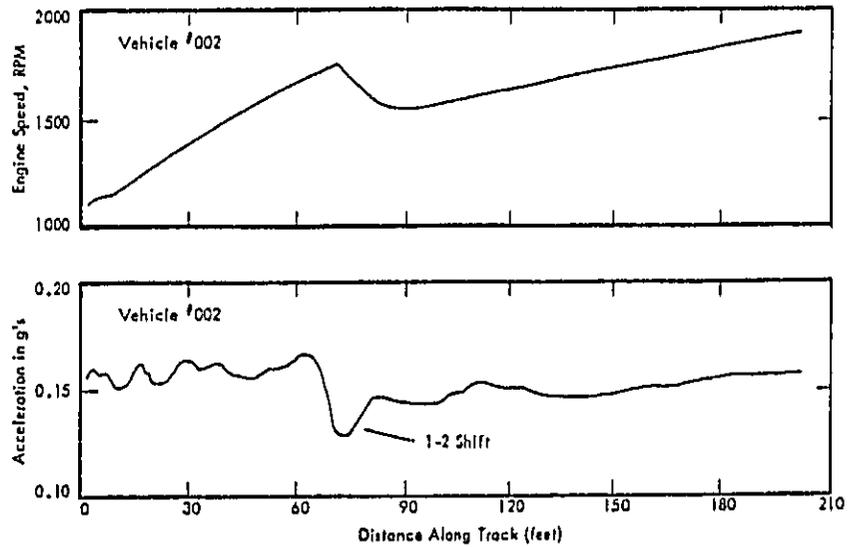
Figure 5.9. Engine Speed and Acceleration Traces for Vehicle #002.
