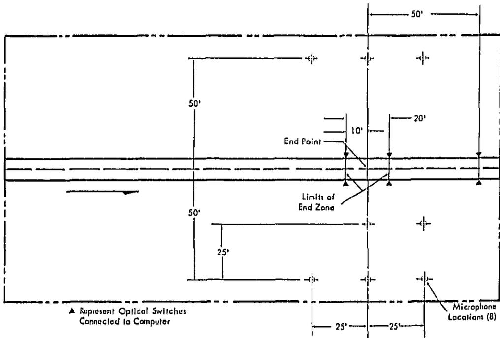
Figure 6.5. Test Section Layout for Preliminary Implementation of Test Procedure.
