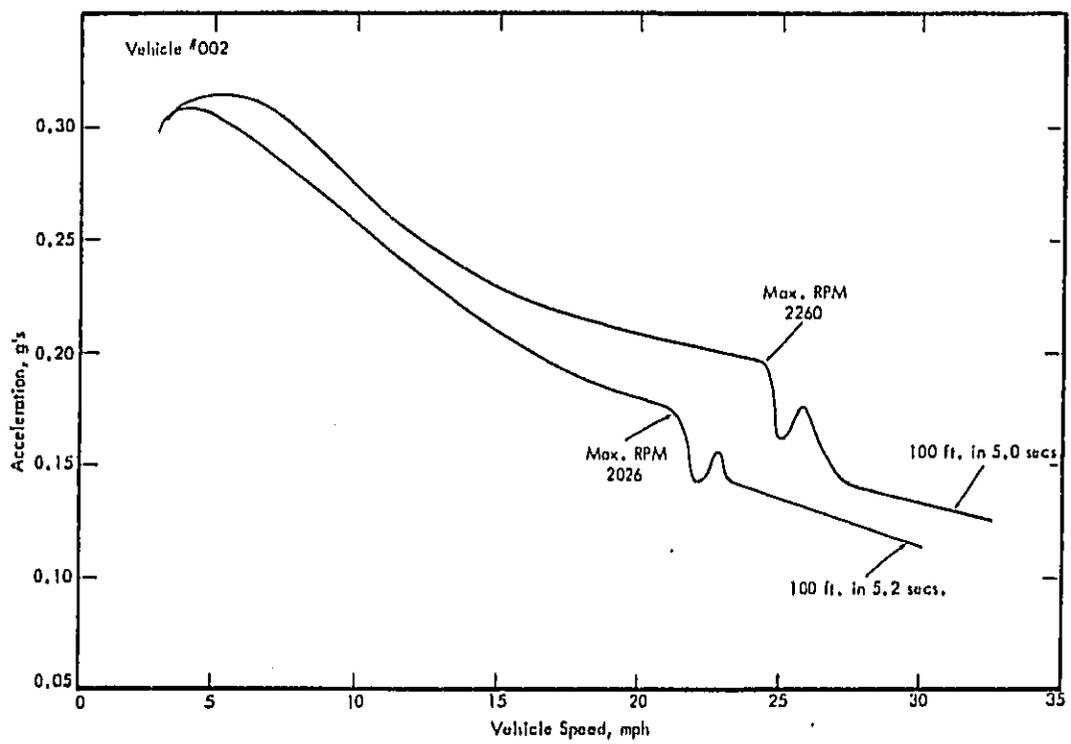
Figure 5.24. Constant-Throttle Shift Characteristics for Vehicle #002.
