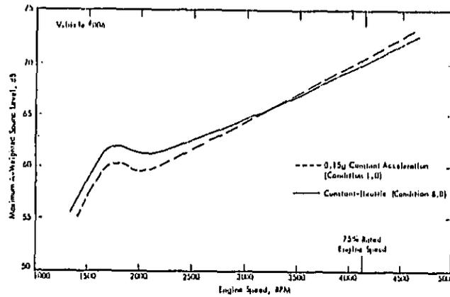
Figure 5.29. Comparison of Sound Levels Under Constant Acceleration and Constant Throttle for Vehicle #006.
