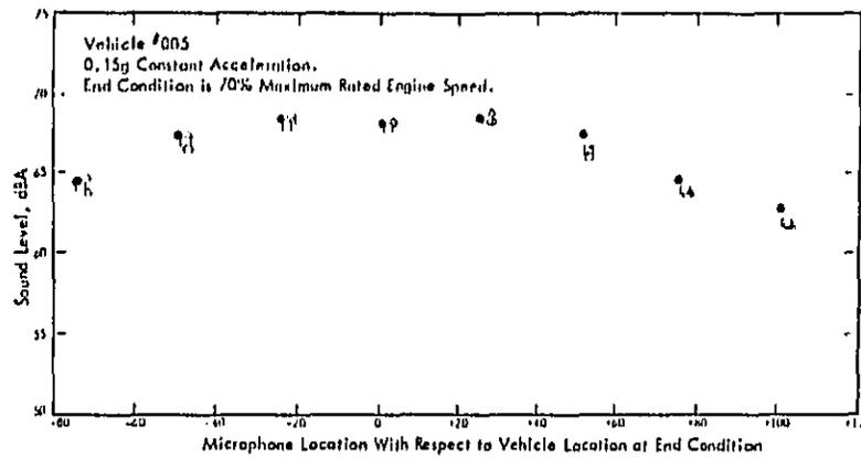
Figure 6.2. Sensitivity of Microphone Location for Vehicle #005.
