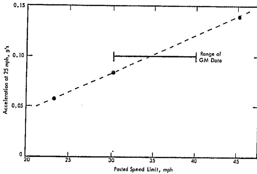
Figure 3.2. Typical Light Vehicle Acceleration at 25 mph as a Function of Posted Speed Limit.
