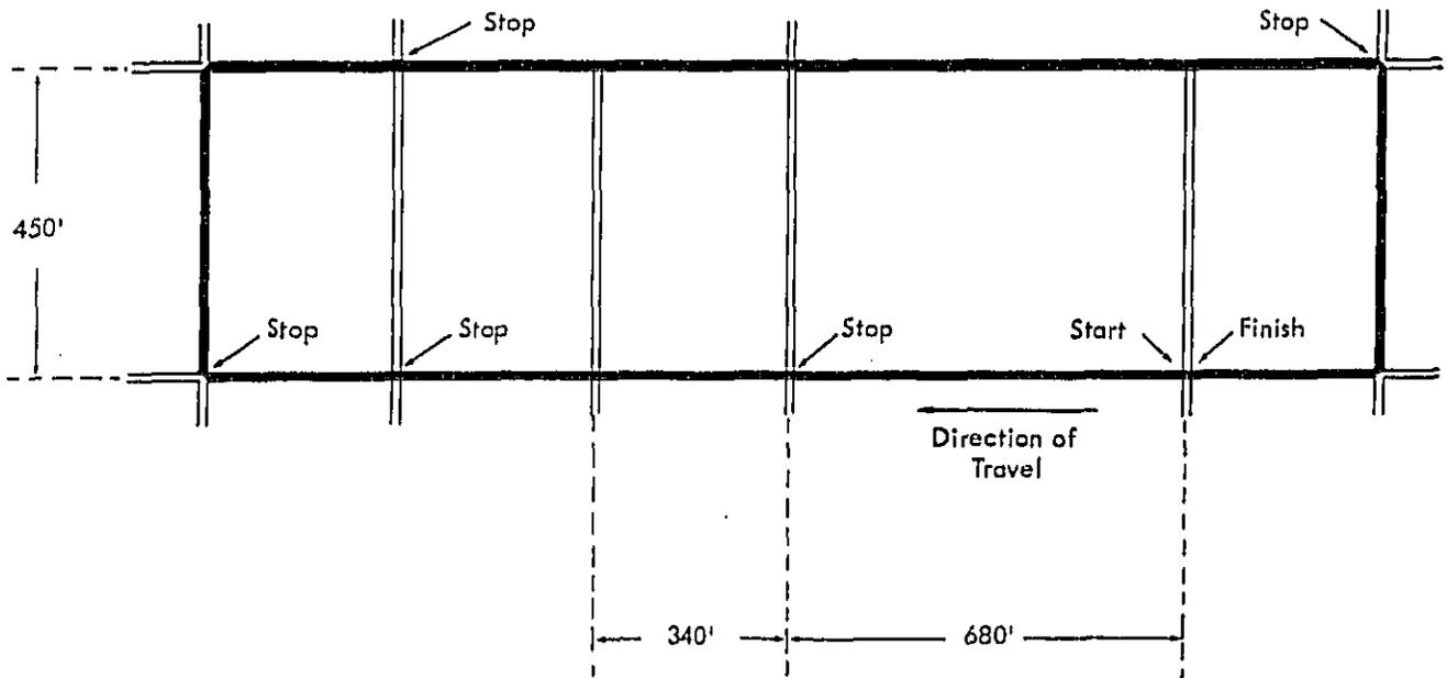
Figure 4.1. Layout of Test Route for Marana Vehicle Operation Measurements
