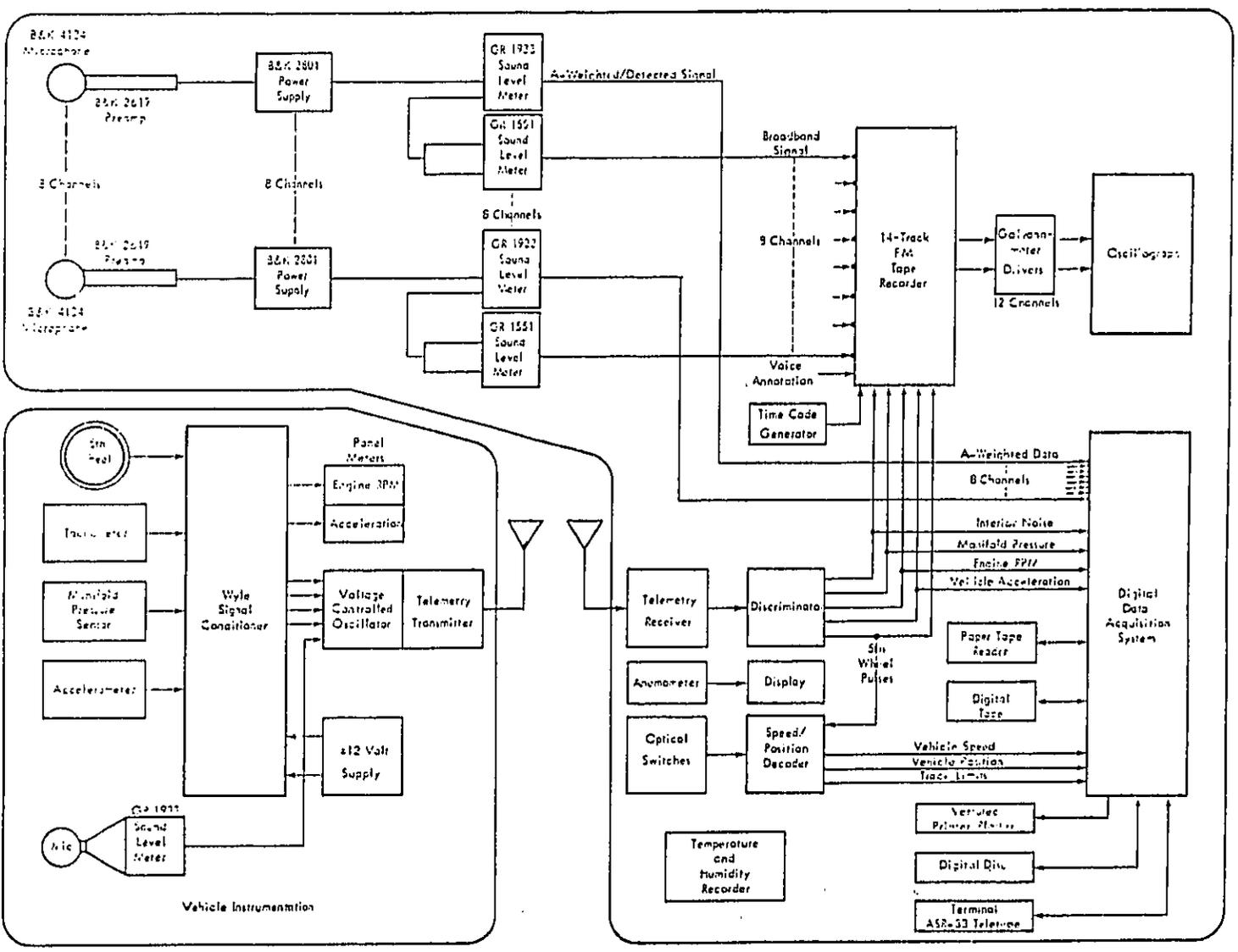
Figure C.1. Data Acquisition and Reduction Instrumentation -- EPA Light Vehicle Test Facility
