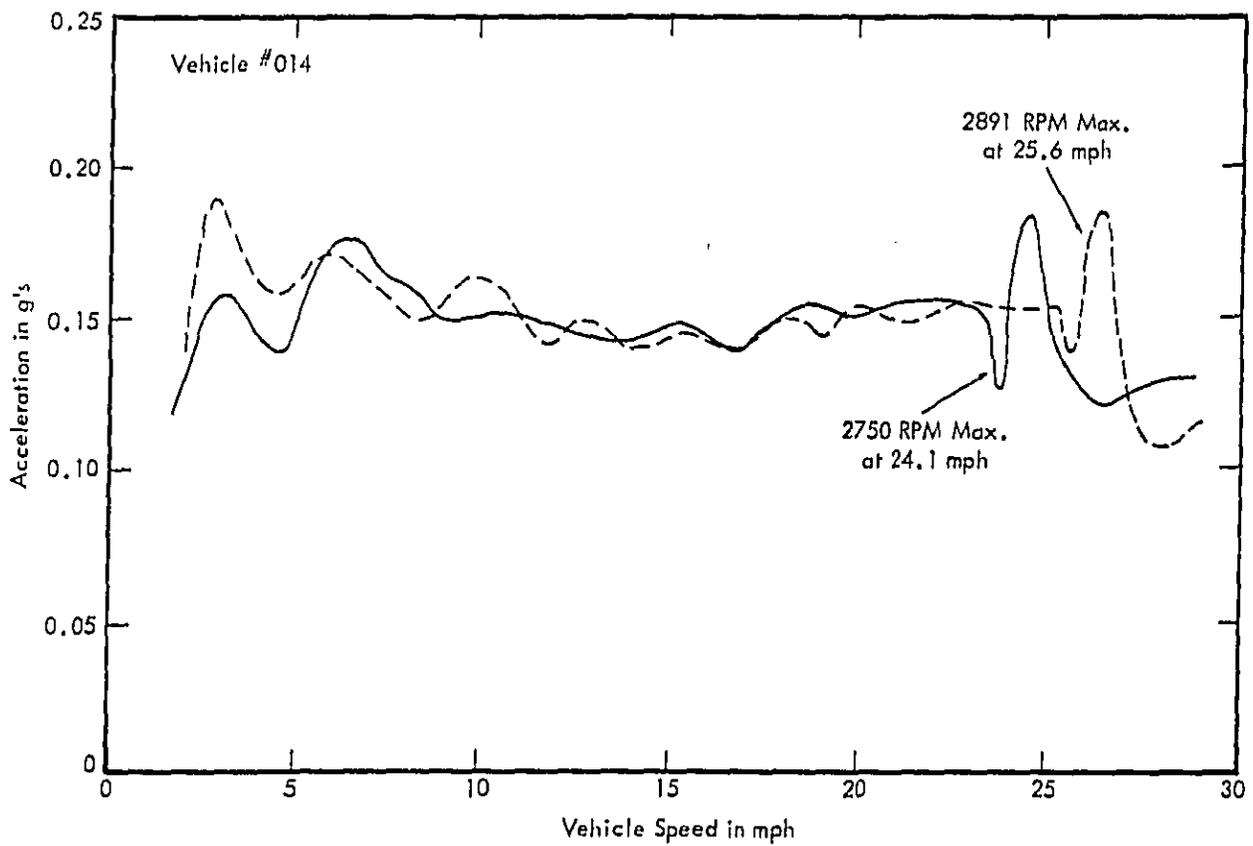
Figure 5.7. Variation in Vehicle Parameters at the Shift Point — Vehicle #014.
