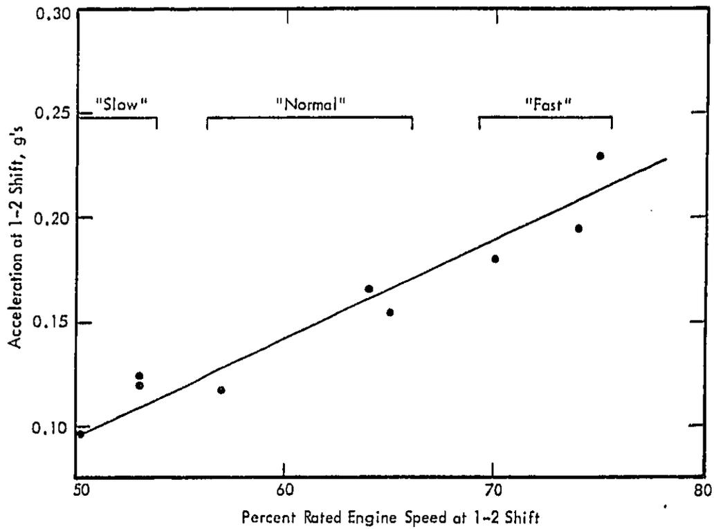
Figure 4.3. Acceleration as a Function of Normalized Engine Speed at 1-2 Shift for Uninfluenced Driving Operations of Manual Transmission Vehicles.
