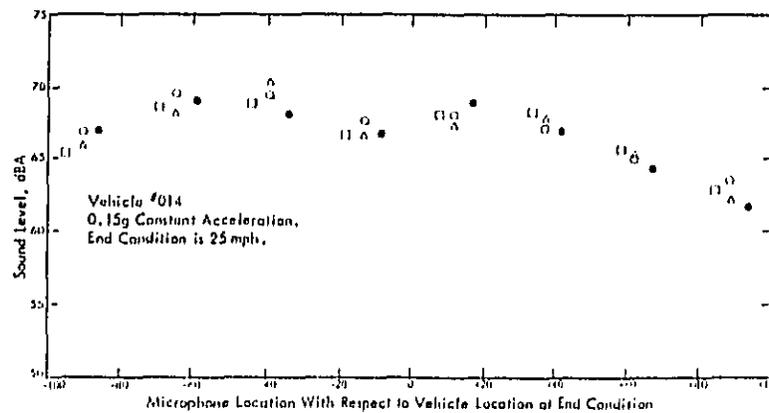
Figure 6.4. Sensitivity of Microphone Location for Vehicle #014.
