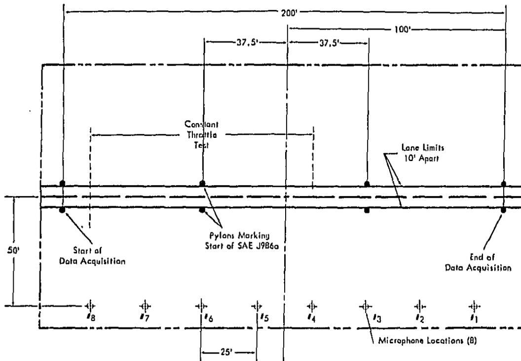
Figure 5.2. Test Section Layout for Noise Tests.
