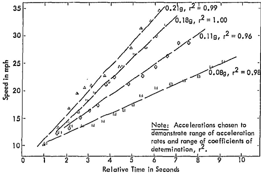
Figure B-3. Speed Versus Time — Application of Linear Approximation.
