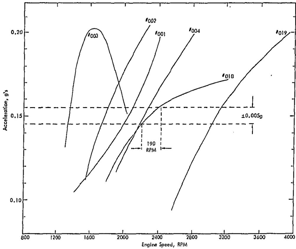
Figure 6.1. Acceleration as a Function of Engine Speed at the 1-2 Shift Point for Different Constant-Throttle Settings.
