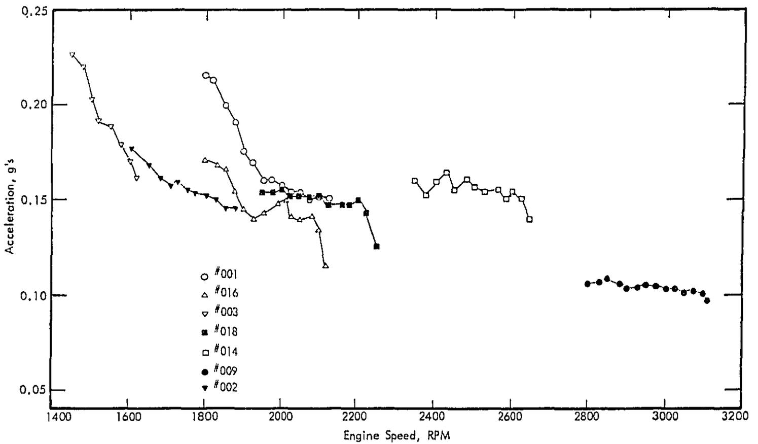
Figure 5.28. Acceleration as a Function of Engine Speed for a Single Constant-Throttle Operation Near the 1-2 Shift.
