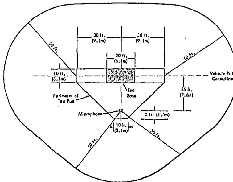
Figure 7.1. Layout of Test Site for the Urban Acceleration Noise Test Procedure.
