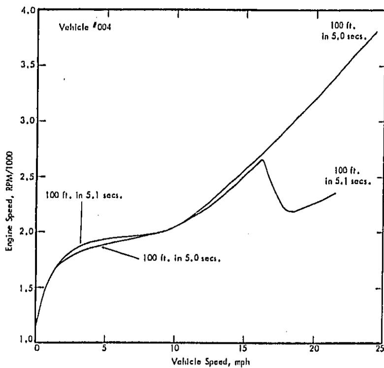
Figure 5.26. Engine Speed History for Constant-Throttle Operation of Vehicle #004.
