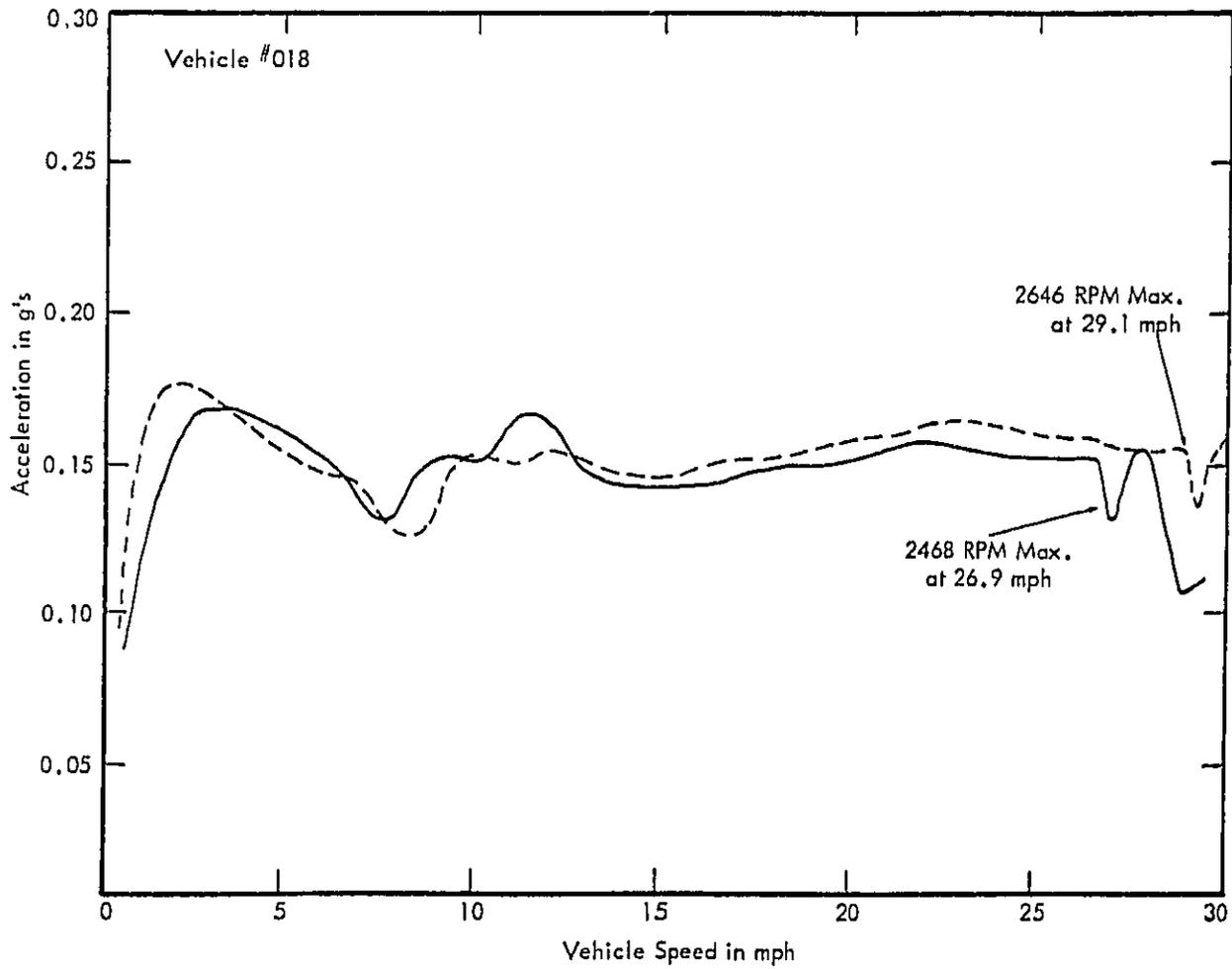
Figure 5.8. Variation in Vehicle Parameters at the Shift Point - Vehicle #018.
