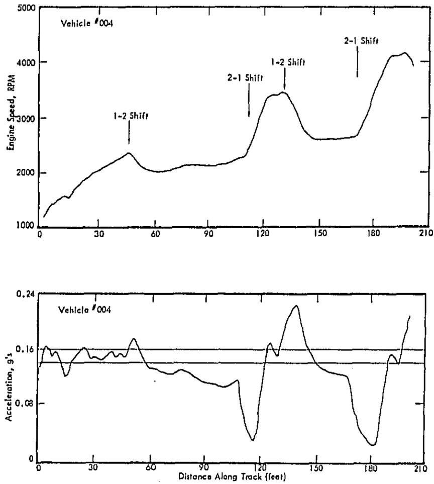
Figure 5.11. Characteristics of Vehicle #004 Under Constant Acceleration.
