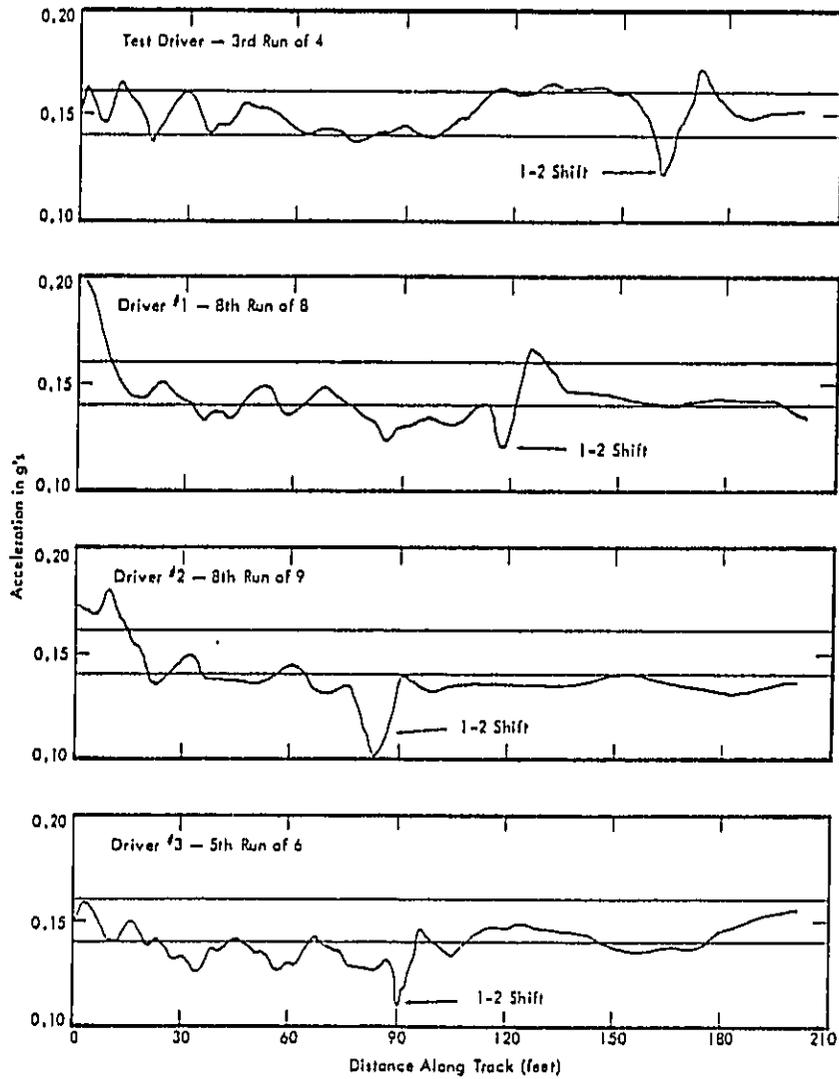
Figure 5.14. Acceleration Traces for Automatics Operated by Different Drivers.
