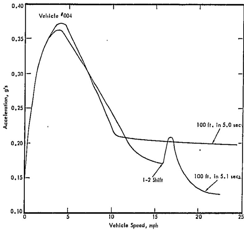
Figure 5.25. Constant-Throttle Shift Characteristics for Vehicle #004.
