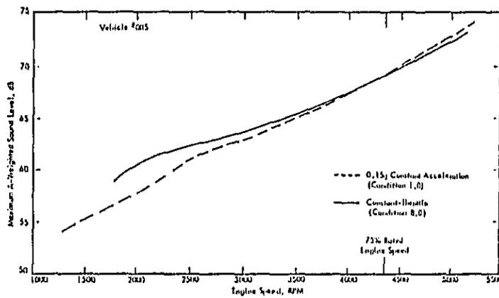
Figure 5.30. Comparison of Sound Levels Under Constant Acceleration and Constant Throttle for Vehicle #005.
