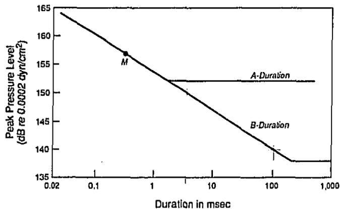
FIGURE 1 The 1968 Impulse Noise Criterion
