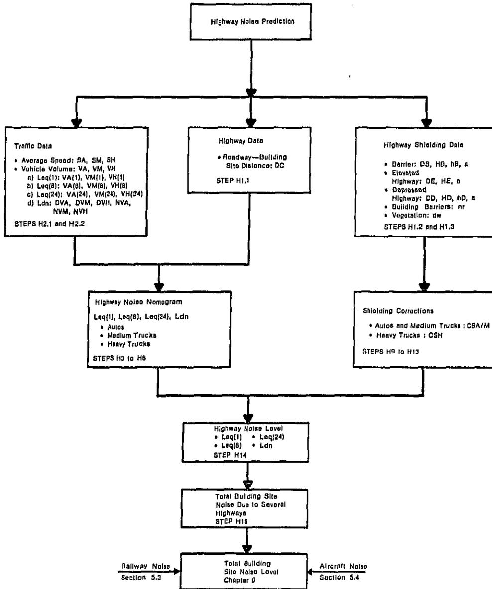
Figure 5.2-3. Highway Noise Prediction Flow Diagram.
