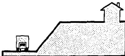
Figure 5.1-3. Shielding by a Depressed Highway or Railway.
