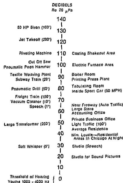
Figure 3-2. Typical A-weighted Sound Pressure Levels [4].
