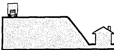
Figure 5.1-4. Shielding by an Elevated Highway or Railway.
