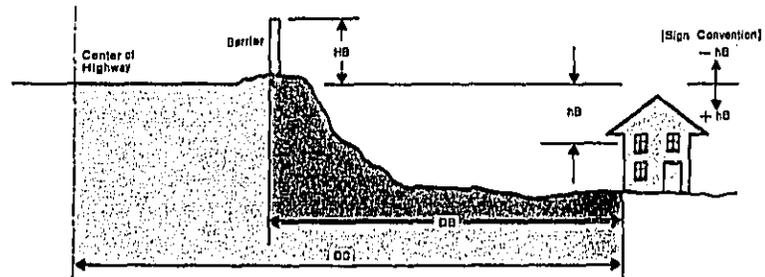
(a) Barrier linear dimensions. Be sure to note the sign convention for  $h_B$ ; positive below the plane of the roadway and negative above.
