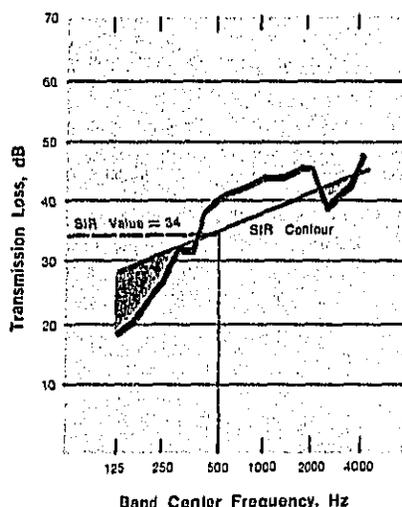
Figure B-6. Example of curve-fitting technique for determination of SIR value of a test specimen based upon one-third octave band transmission loss data. SIR contour is  $-3$  dB/octave straight line with ordinate intercept at 500 Hz equal to the test specimen SIR value.
