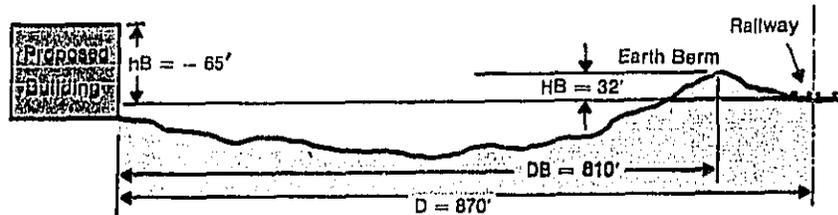
Figure 5.5-11. Cross-Section Showing Railway Earth Berm.
