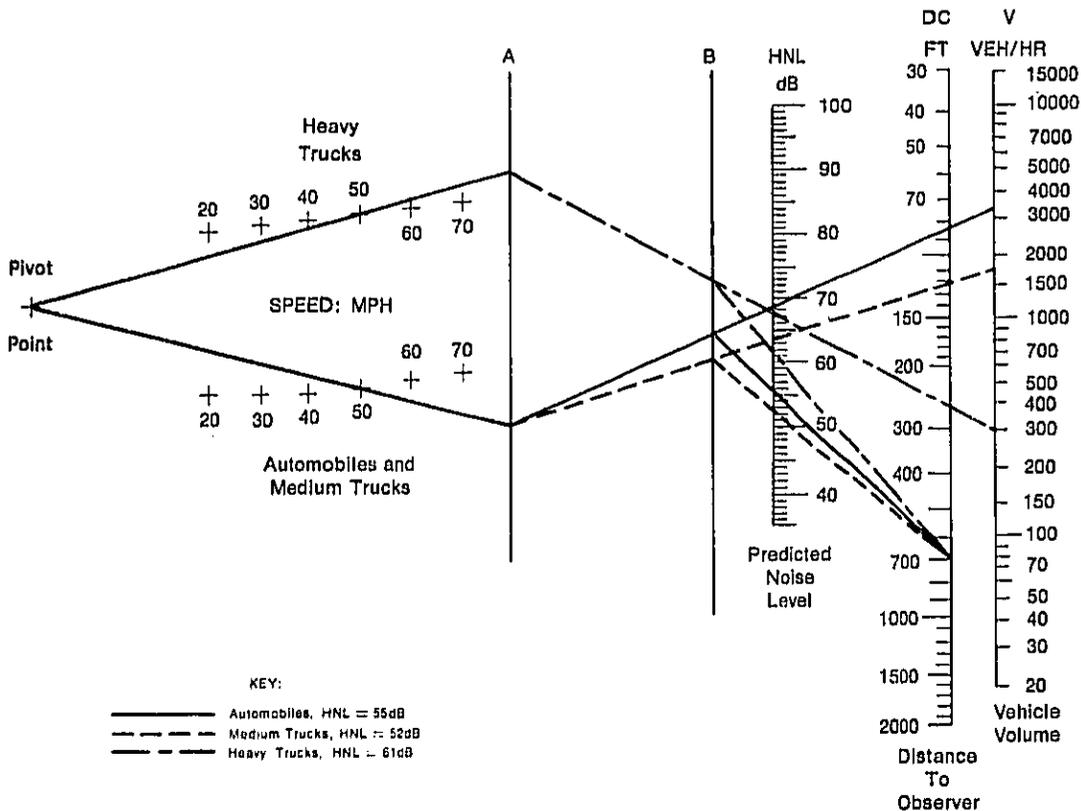
Figure 5.5-7. Highway Noise Nomogram for Highway #1 of Example.
