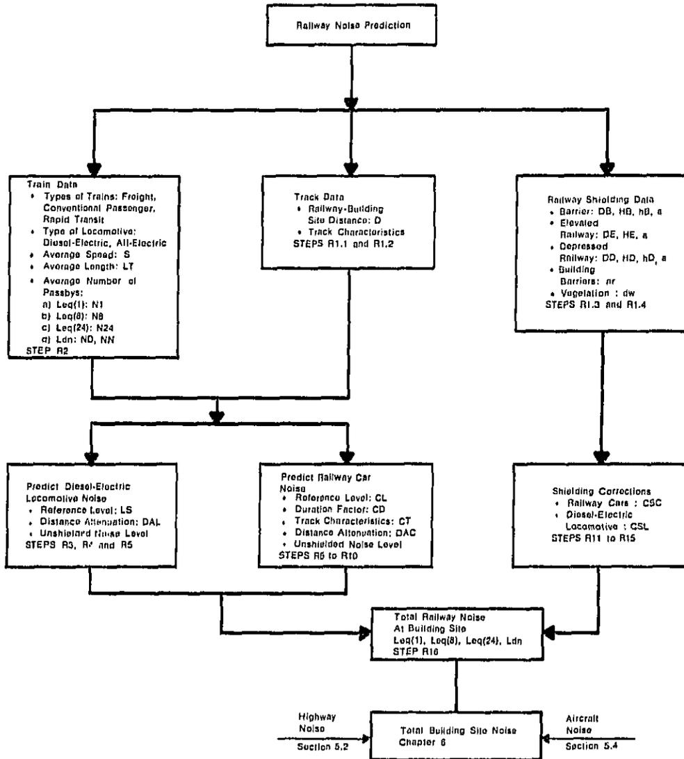
Figure 5.3-1. Railway Noise Prediction Flow Diagram.
