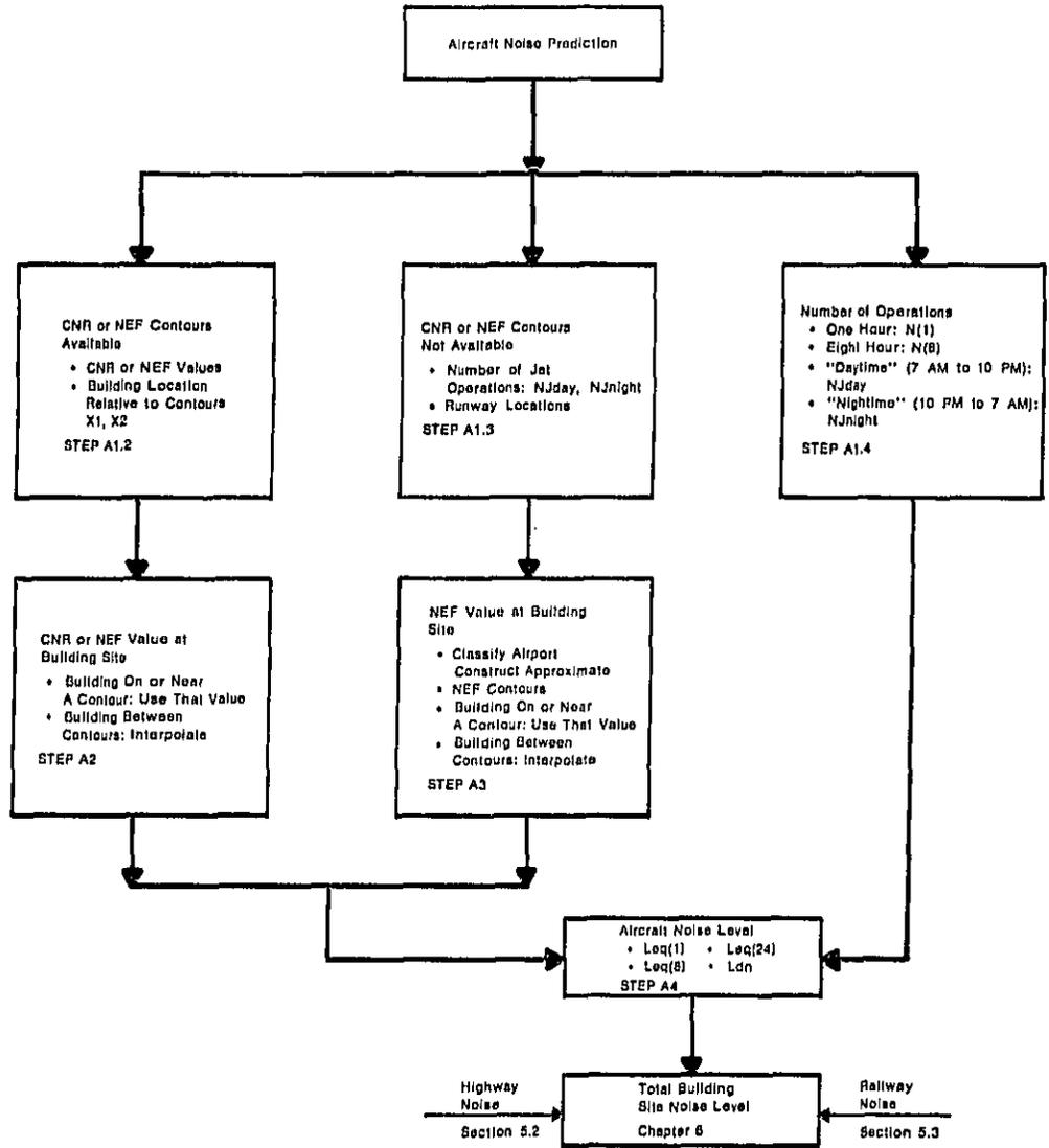
Figure 5.4-3. Aircraft Noise Prediction Flow Diagram.
