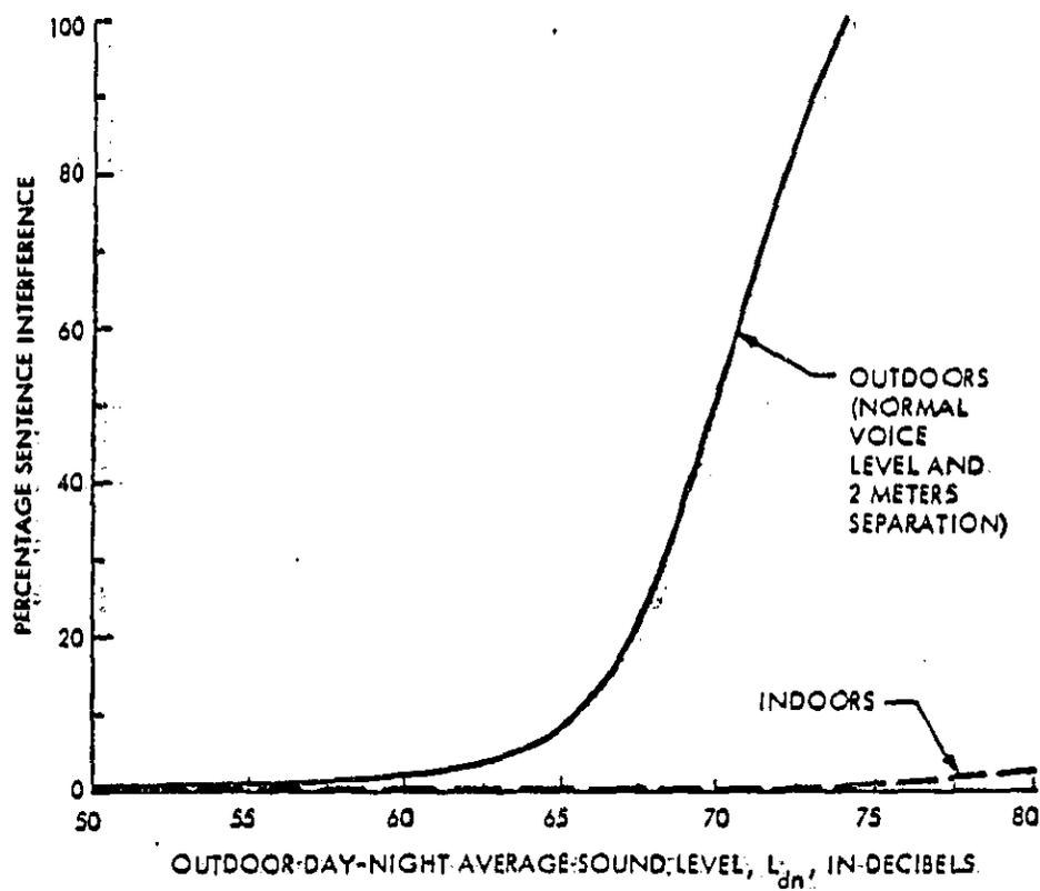
**Figure-17:** Maximum Percentage Interference with Sentences as a Function of the Day-Night Average Noise Level. (Percentage Interference Equals 100 Minus Percentage Intelligibility, and  $L_{dn}$  is Based on  $L_d + 3$ )
