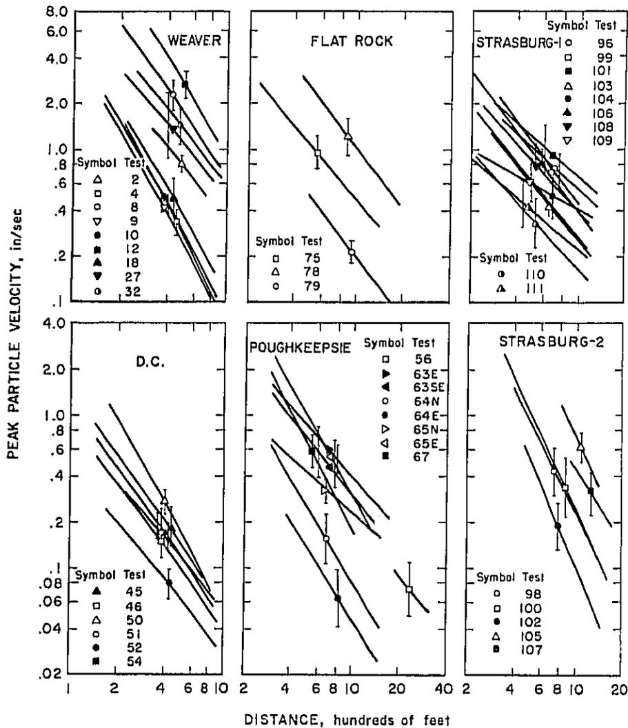
Figure 4.9.—Peak particle velocity versus distance, radial component.
