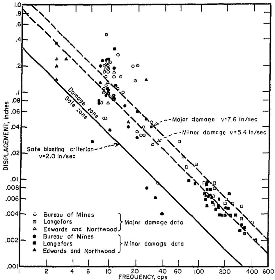
Figure 3.4.—Displacement versus frequency, combined data with recommended safe blasting criterion.
