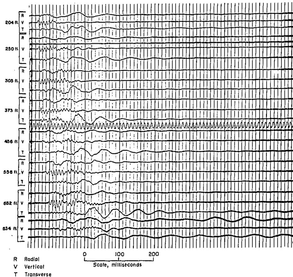
Figure 4.3.—Vibration records for 7-hole, 9-millisecond-delayed blast.
