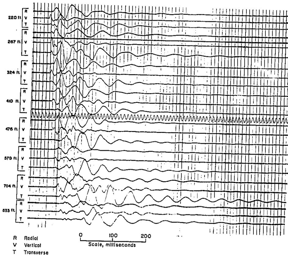
Figure 4.1.—Vibration records for 1-hole blast.
