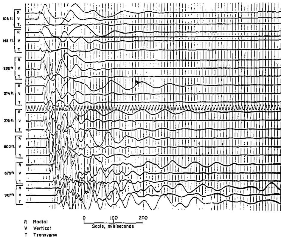
Figure 4.2.—Vibration records for 7-hole instantaneous blast.
