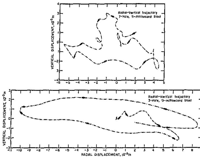
Figure 4.31.—Radial-Vertical particle motion trajectories, 900 feet from 3-hole, and 7-hole, 9-millisecond-delayed blasts.
