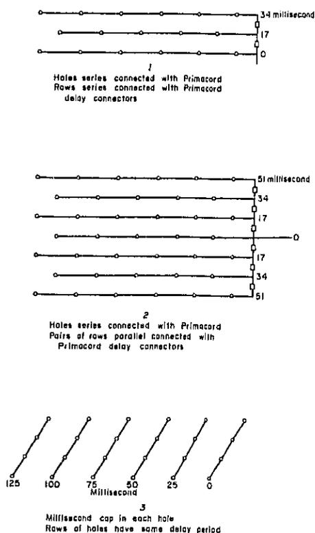
Figure 4.18.—Three methods of initiating blasts.
