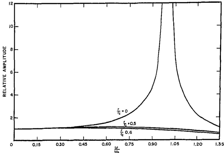
Figure 2.3.—Theoretical response curves for a typical acceleration transducer.
