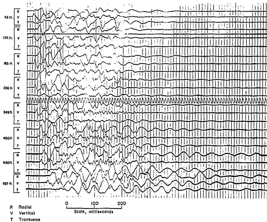
Figure 4.4.—Vibration records for 7-hole, 34-millisecond-delayed blast.
