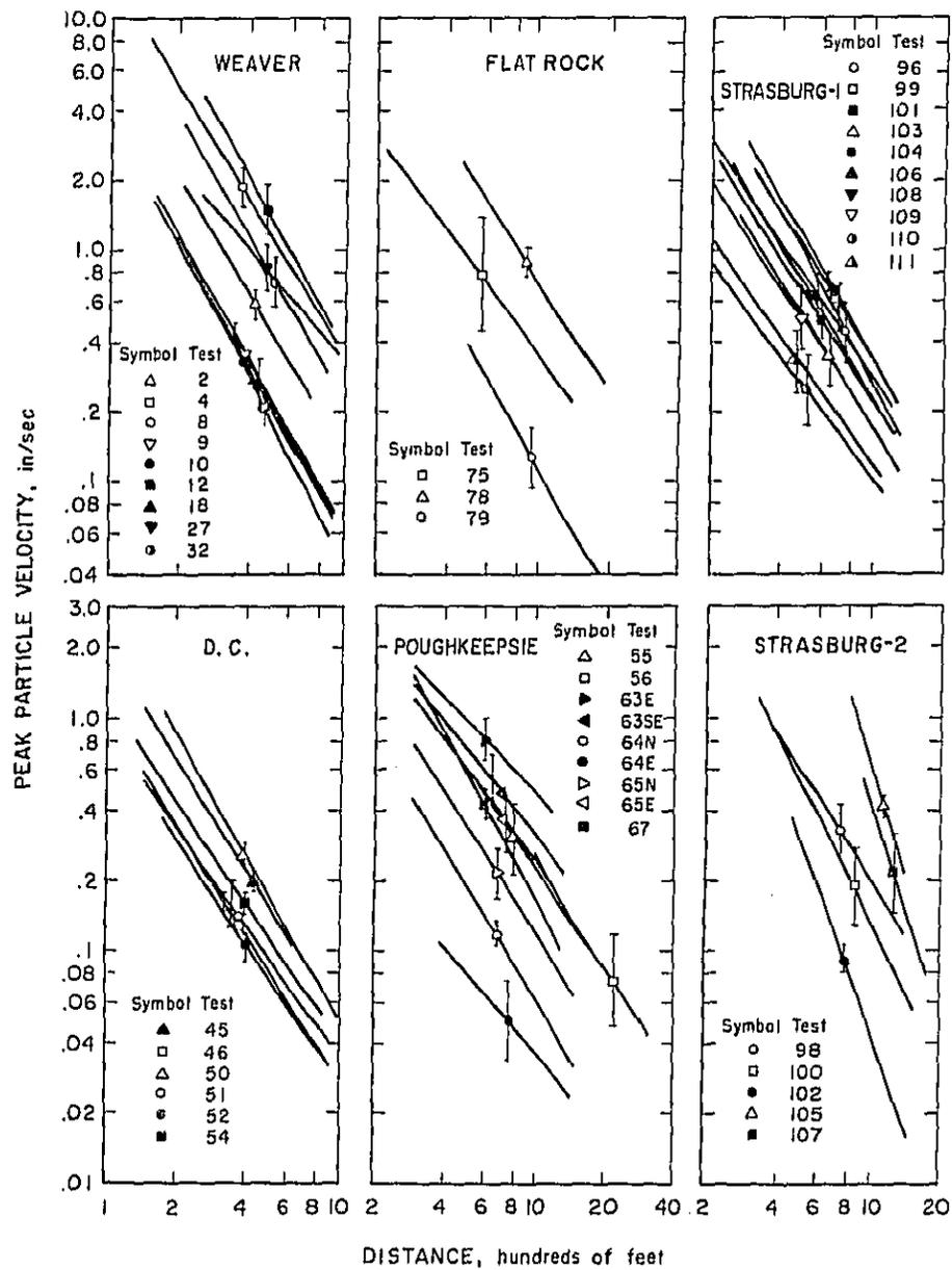
Figure 4.10.—Peak particle velocity versus distance, vertical component.
