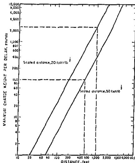
Figure 6.3.—Nomogram for estimating safe charge and distance limits for scaled distances of 20 and 50 ft/lb<sup>1/4</sup>.
