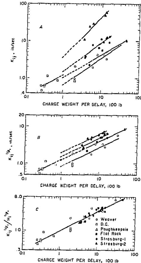
Figure 4.14.—Particle velocity intercepts versus charge weight per delay, transverse component.
