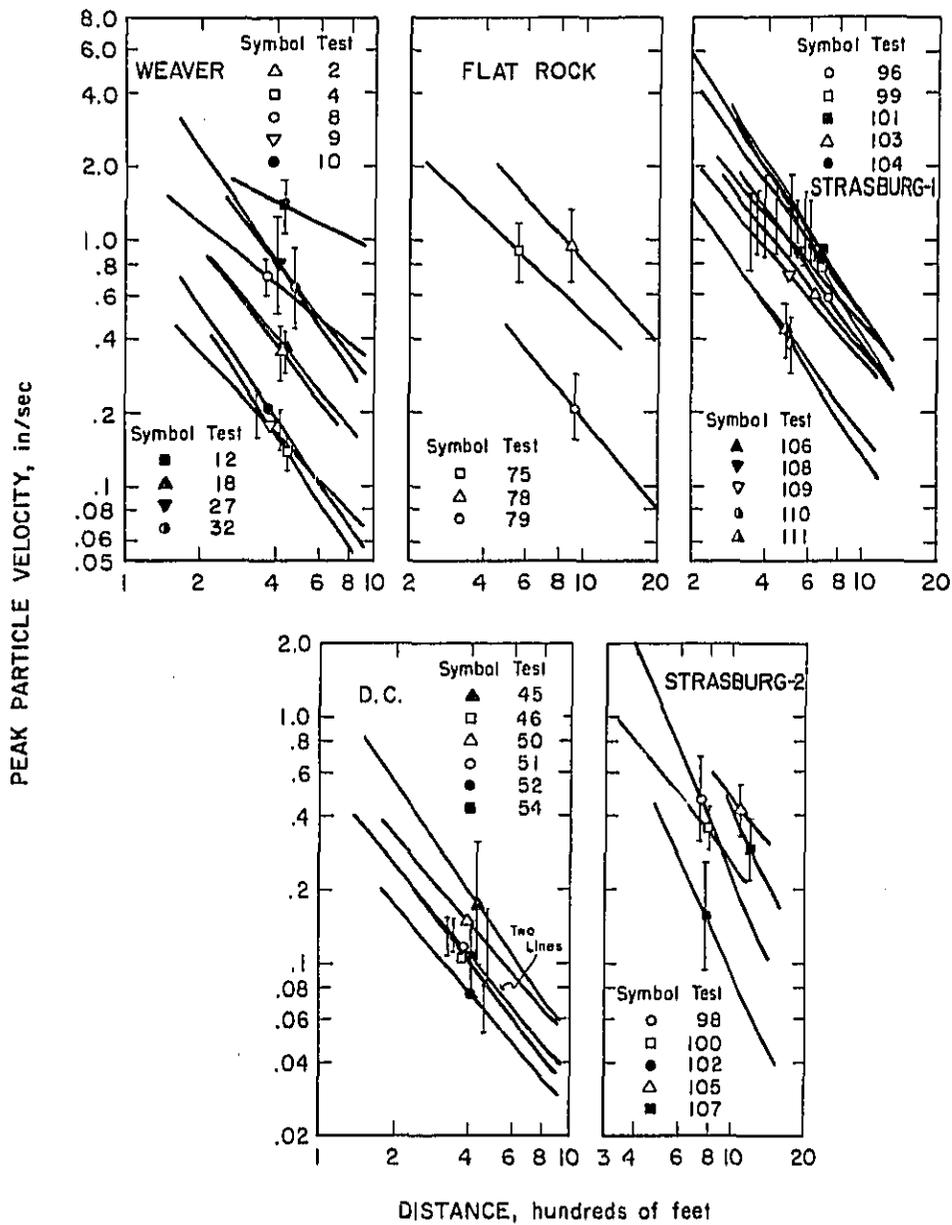
Figure 4.11.—Peak particle velocity versus distance, transverse component.
