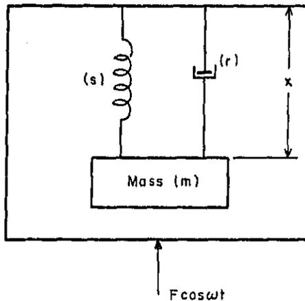
Figure 2.1.—Mass-spring-dashpot model of a seismic transducer.
