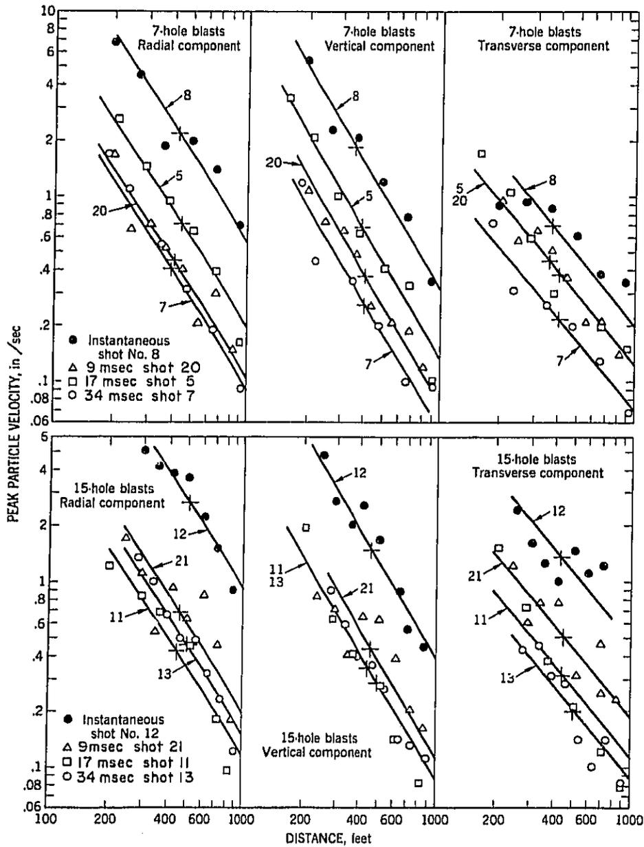
Figure 4.6.—Particle velocity versus distance for 7- and 15-hole blasts.
