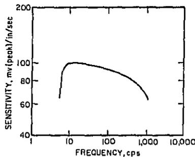
Figure 2.7.—Frequency response curve of velocity gage.
