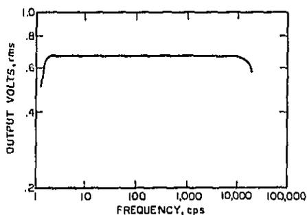
Figure 2.6.—Frequency response curve of linear amplifier.
