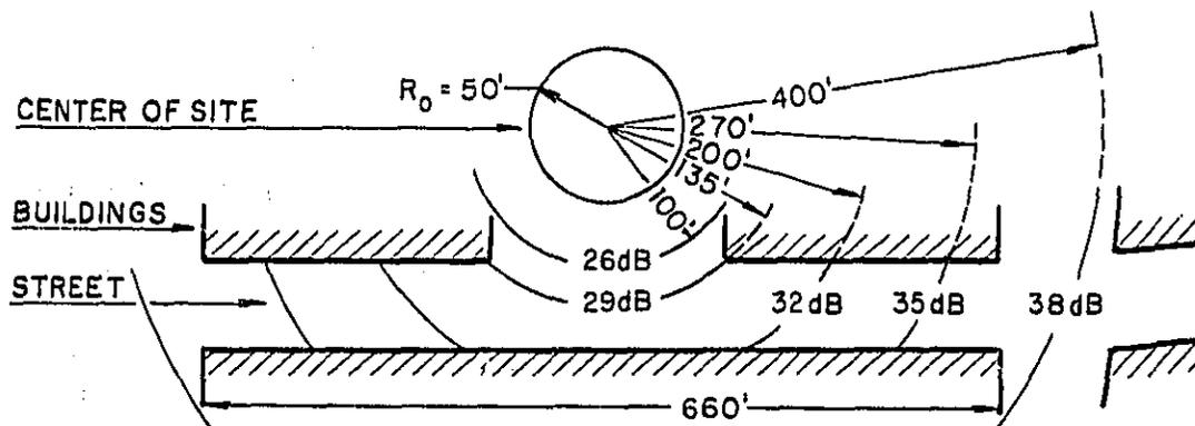
FIG. 20. CONSTRUCTION SITE GEOMETRY AND ATTENUATION CONTOURS FOR A STATIONARY POPULATION WITHIN BUILDINGS. (SEE APPENDIX B FOR METHOD OF COMPUTATION.)
