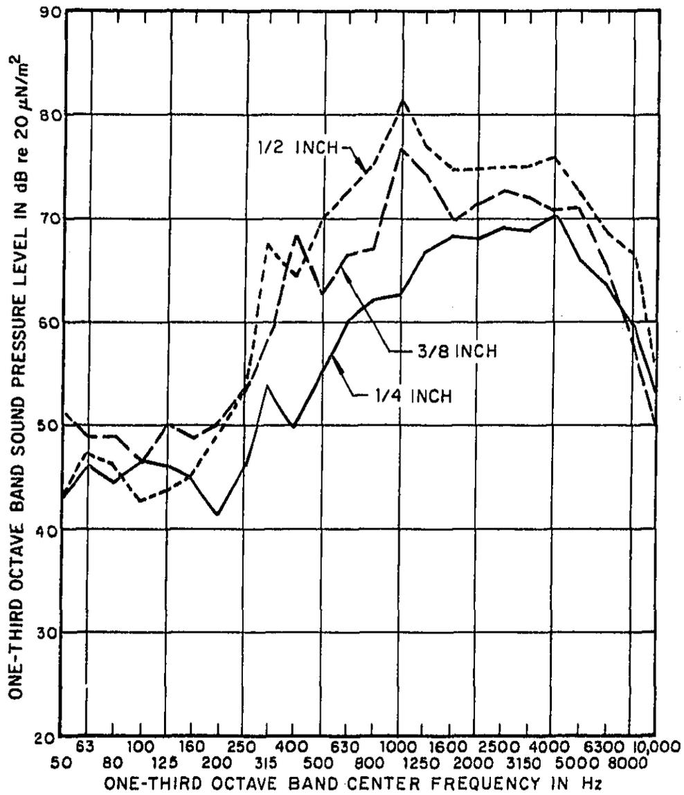
FIG. A.24 SOUND PRESSURE LEVELS FROM THREE DRILLS
