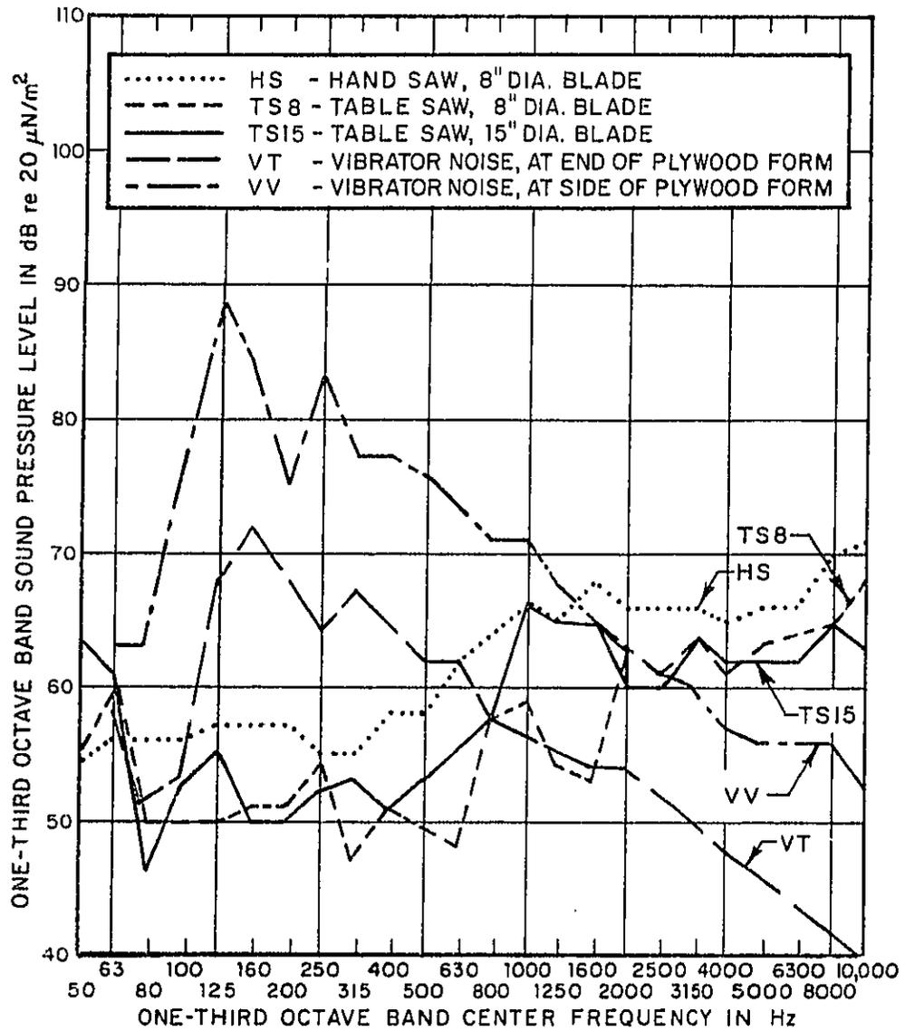
FIG. A.6 SOUND PRESSURE LEVELS FROM VIBRATOR AND SAWS
