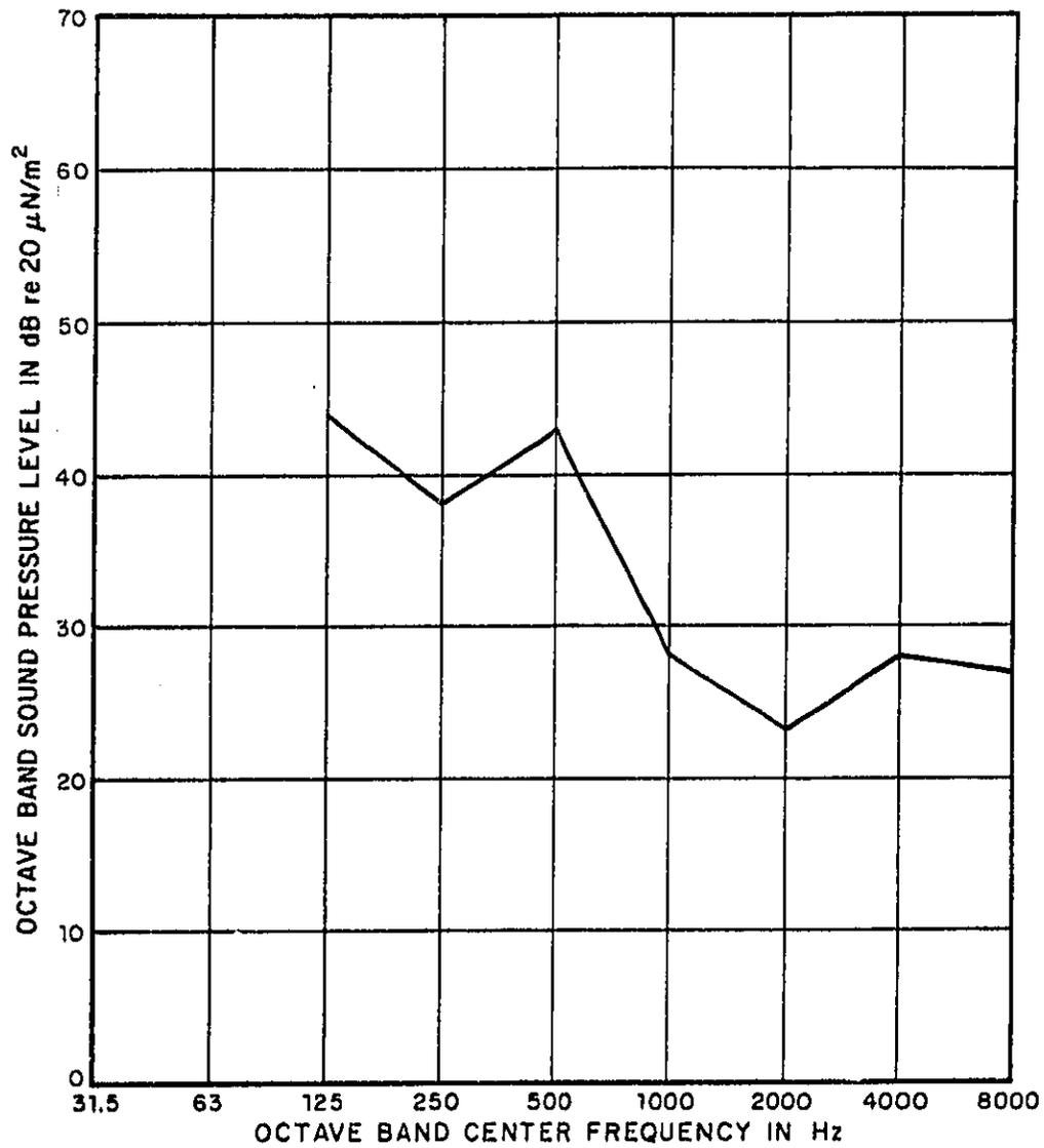
FIG. A.61 SOUND PRESSURE LEVELS FROM BALLASTS
