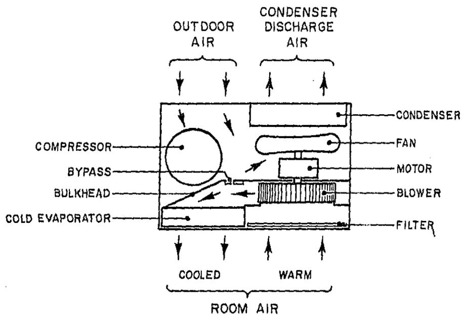
FIG. 5. SCHEMATIC VIEW OF A TYPICAL ROOM AIR CONDITIONER.
