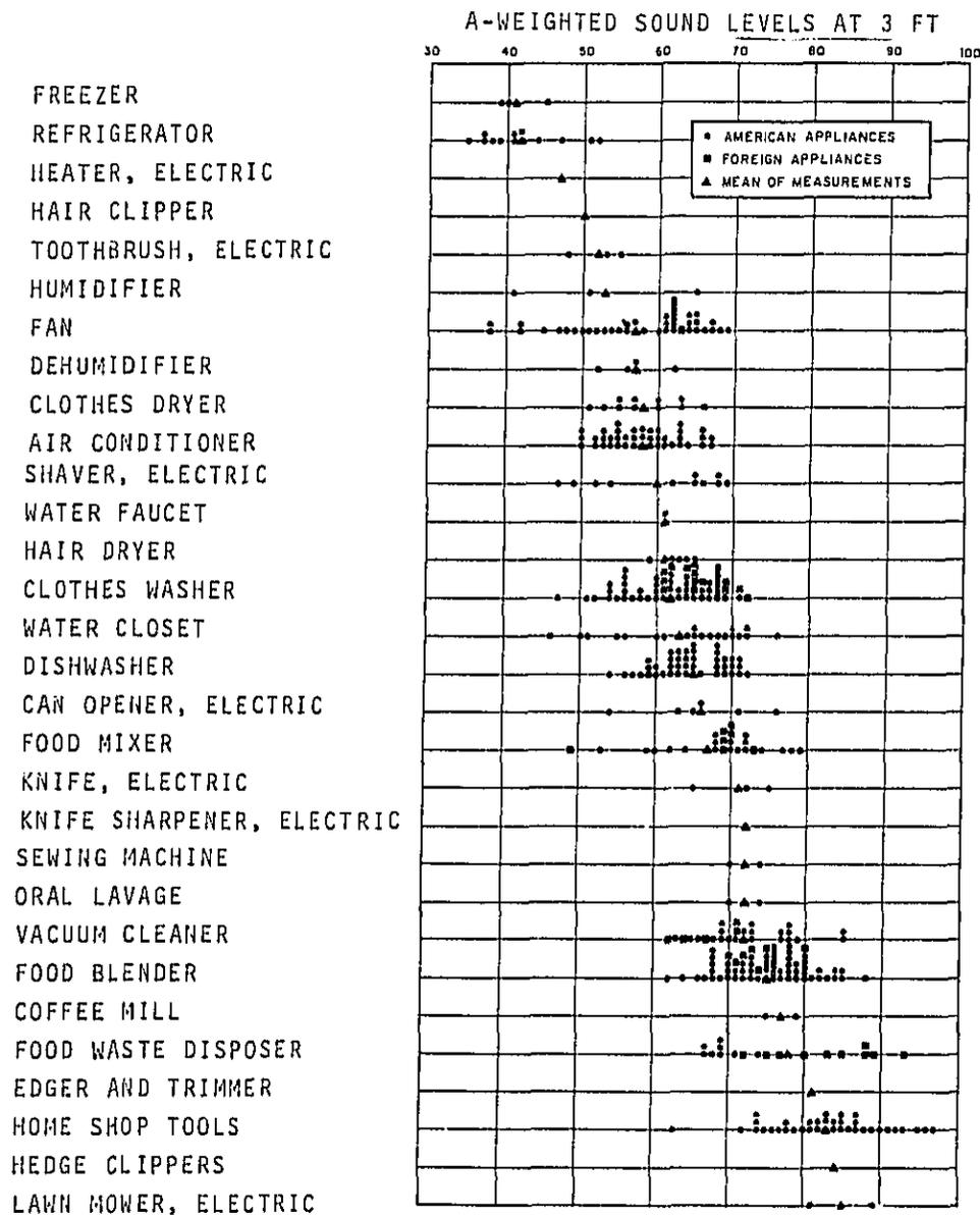
FIG. 3. A SUMMARY OF NOISE LEVELS FOR APPLIANCES MEASURED AT A DISTANCE OF 3 FT.
