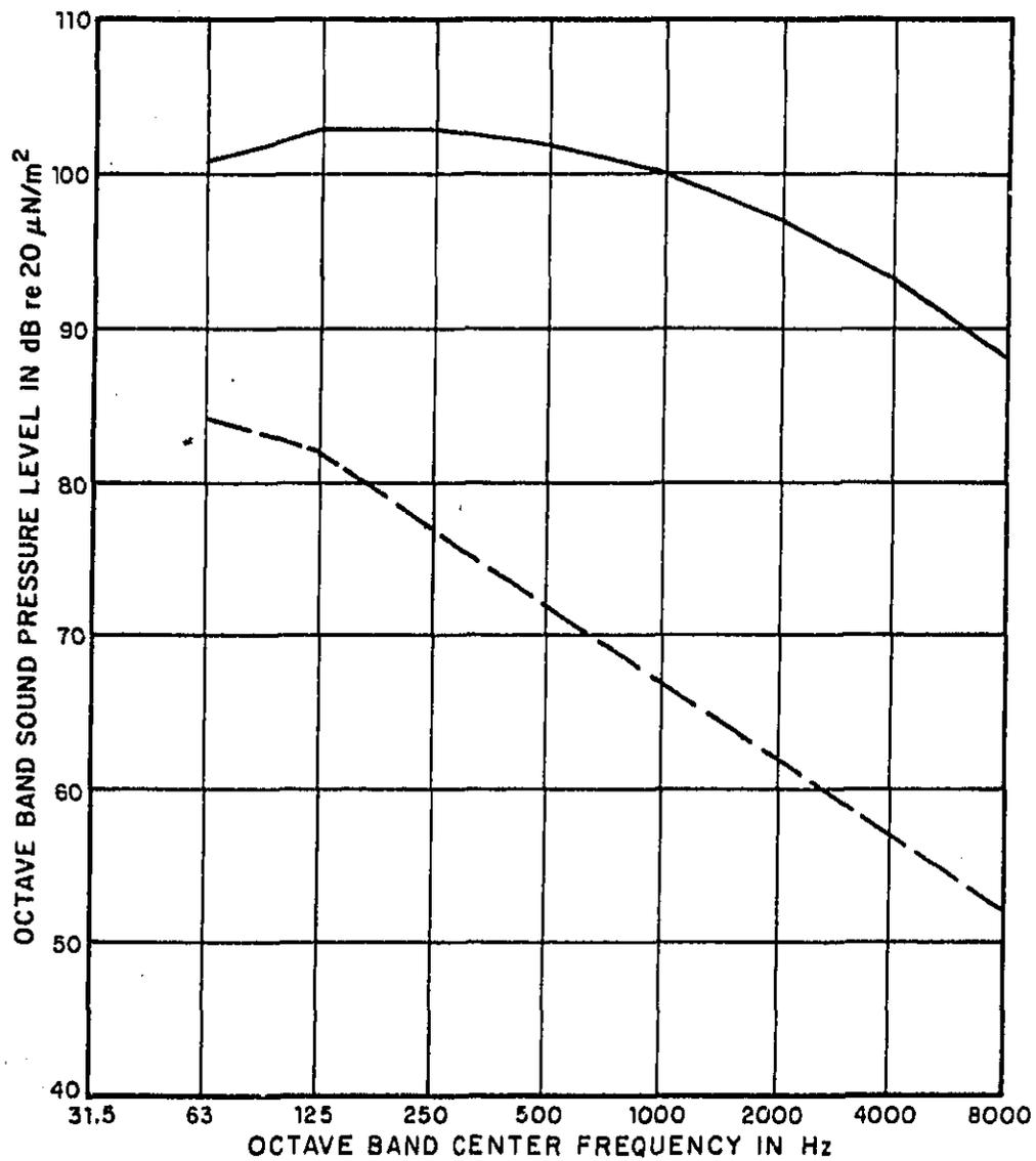
FIG. A.45 RANGE OF SOUND PRESSURE LEVELS FROM FANS
