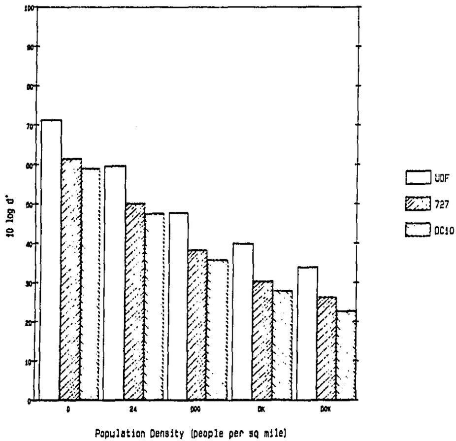
Figure 4-1: Comparison of Predicted Audibility of Three Types of En Route Aircraft Noise and Five Levels of Population Density (Cruise Noise Level Normalized to 50 dBA)
