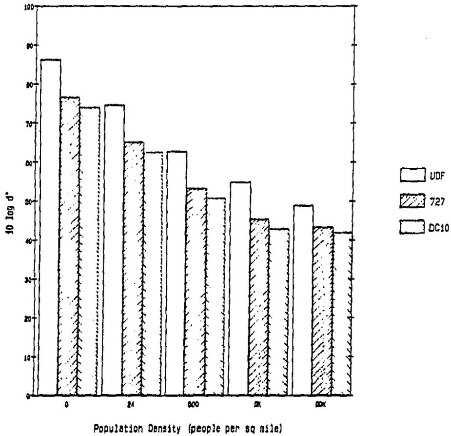
**Figure 4-4: Comparison of Predicted Audibility of Three Types of En Route Aircraft Noise and Five Levels of Population Density (Cruise Noise Level Normalized to 65 dBA)**
