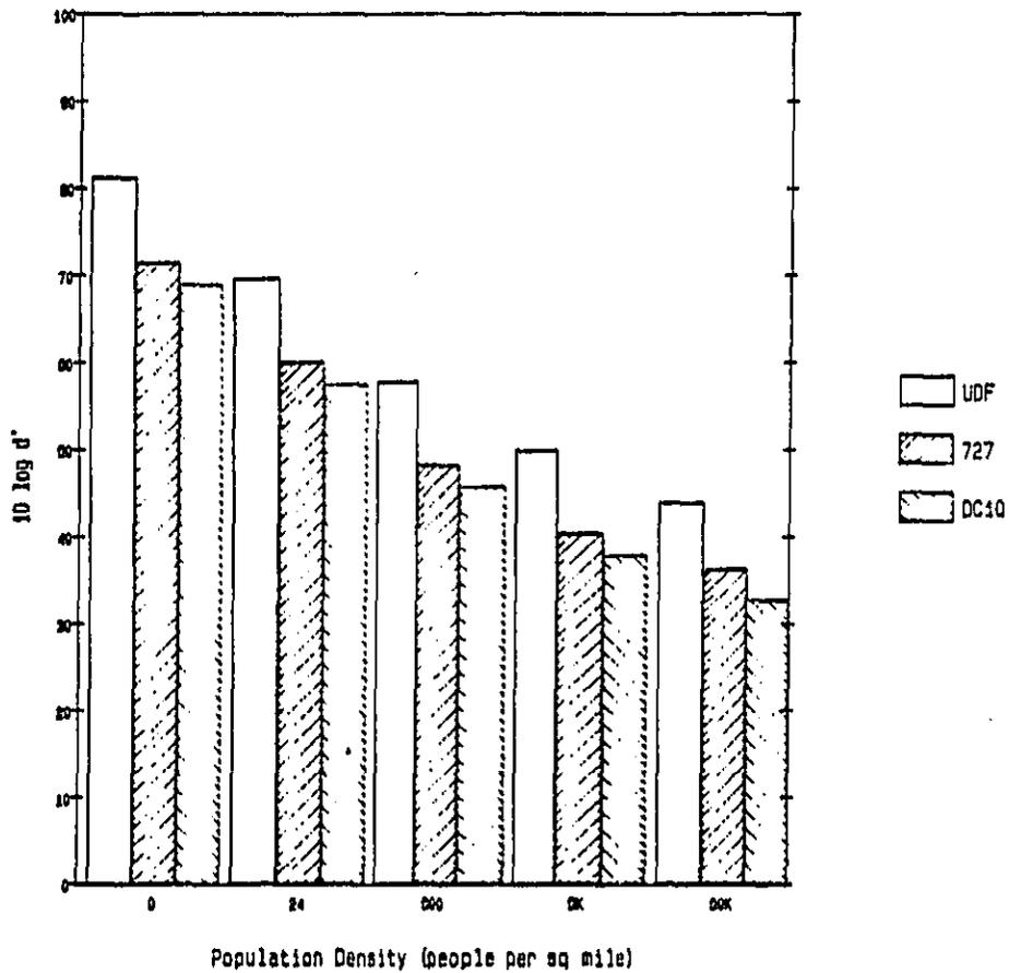
Figure 4-3: Comparison of Predicted Audibility of Three Types of En Route Aircraft Noise and Five Levels of Population Density (Cruise Noise Level Normalized to 60 dBA)
