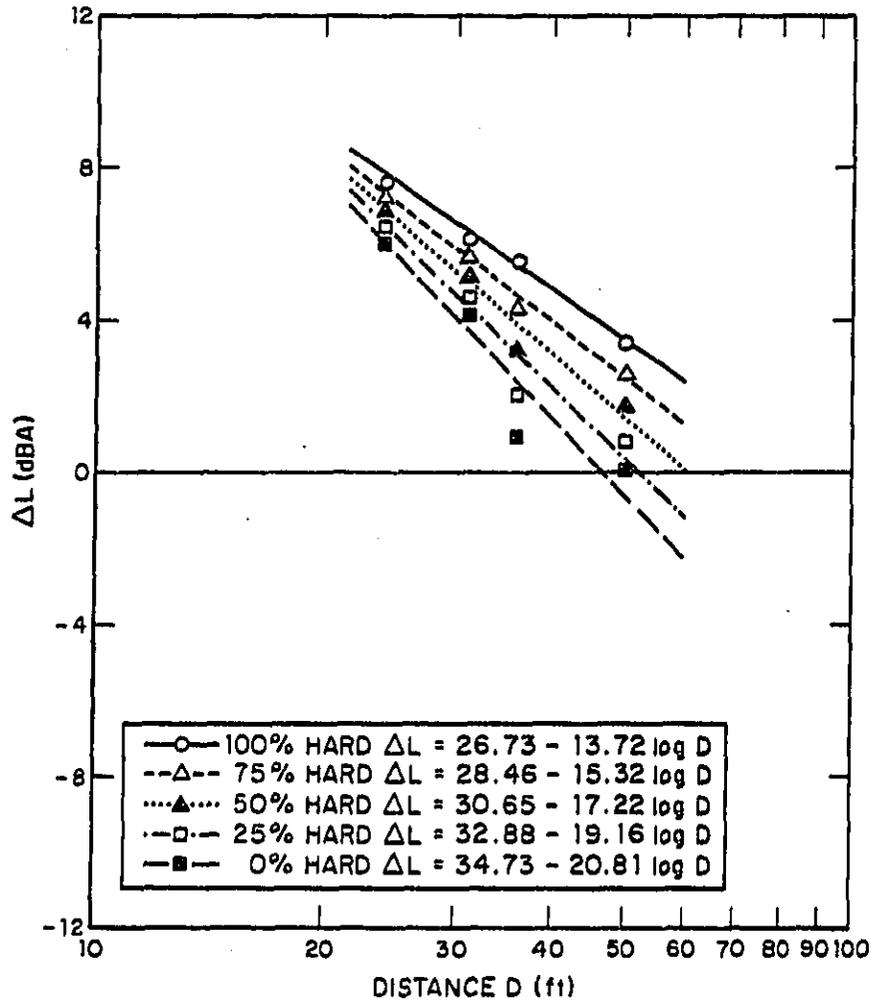
FIG. 5.11. HARD SITE/SOFT SITE NOISE LEVEL DIFFERENCES AS A FUNCTION OF MICROPHONE DISTANCE: GAS PASSBYS - 45 MPH - RIGHT SIDE.
