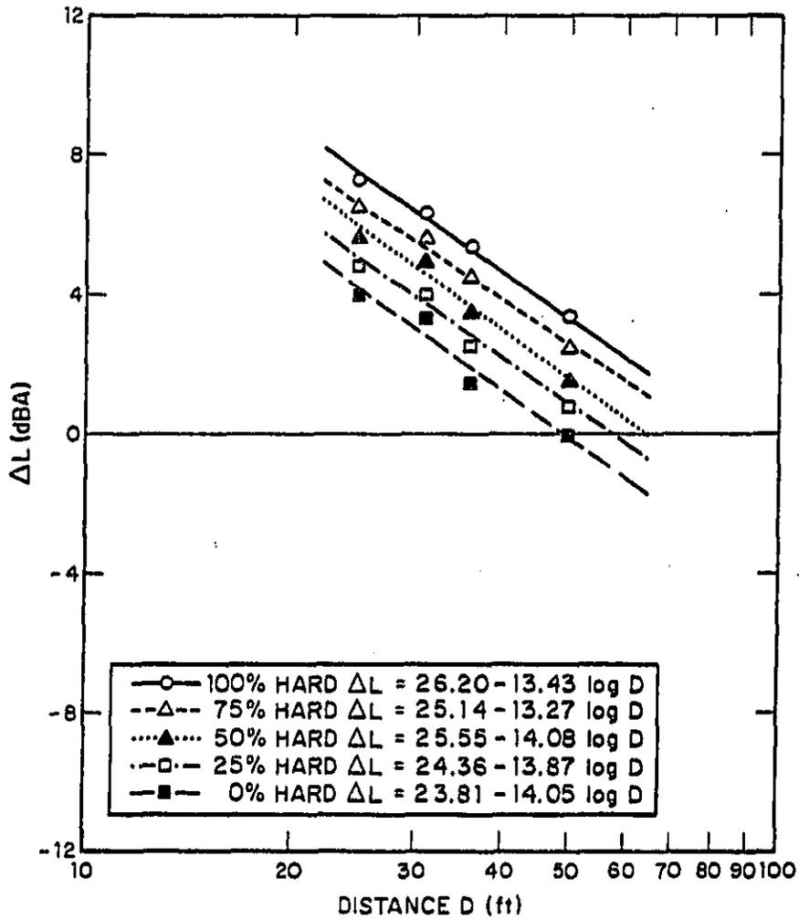
FIG. 5.8. HARD SITE/SOFT SITE NOISE LEVEL DIFFERENCES AS A FUNCTION OF MICROPHONE DISTANCE: DIESEL PASSBYS - 45 TO 50 MPH - LEFT SIDE.
