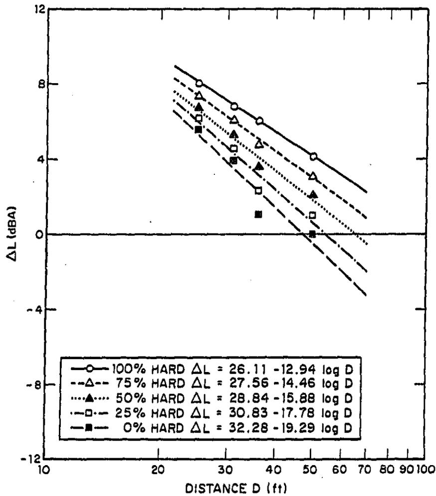
FIG. 5.14. HARD SITE/SOFT SITE NOISE LEVEL DIFFERENCES AS A FUNCTION OF MICROPHONE DISTANCE: TOTAL PASSBYS.
