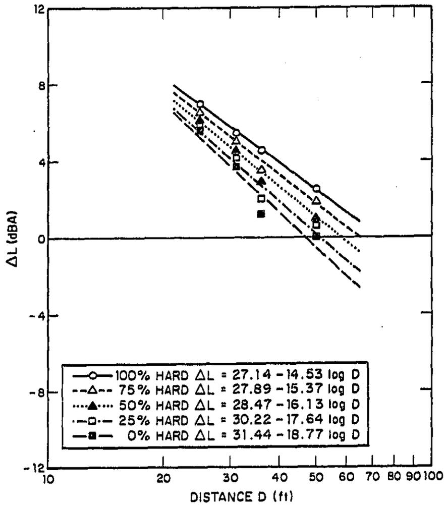
FIG. 5.6. HARD SITE/SOFT SITE NOISE LEVEL DIFFERENCES AS A FUNCTION OF MICROPHONE DISTANCE: DIESEL PASSBYS - 30 TO 35 MPH - LEFT SIDE.
