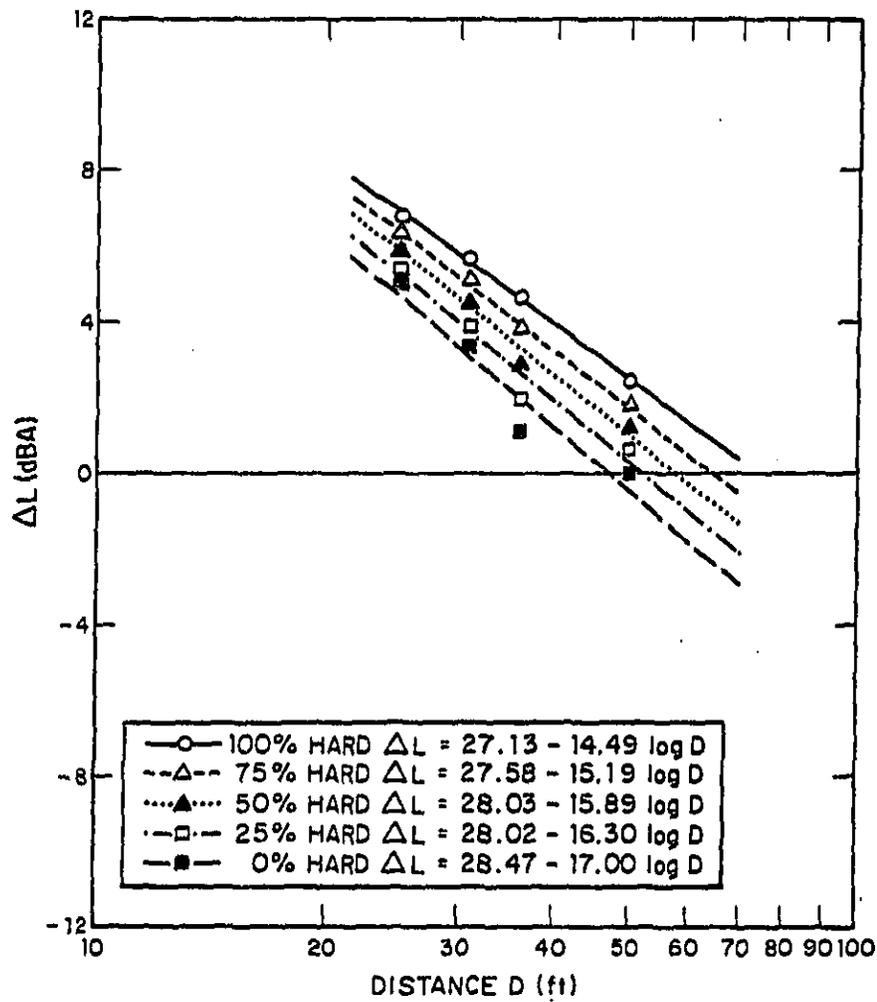
FIG. 5.5. HARD SITE/SOFT SITE NOISE LEVEL DIFFERENCES AS A FUNCTION OF MICROPHONE DISTANCE: DIESEL PASSBYS - 35 MPH - RIGHT SIDE.
