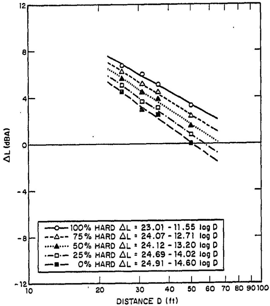
FIG. 5.13. HARD SITE/SOFT SITE NOISE LEVEL DIFFERENCES AS A FUNCTION OF MICROPHONE DISTANCE: TOTAL IMI.
