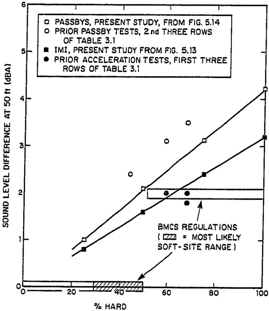
FIG. 6.1. COMPARISON OF RESULTS FROM PRESENT EXPERIMENTS WITH THOSE OF PREVIOUS STUDIES, AT 50 FT. HARD SITE MINUS SOFT SITE NOISE LEVEL DIFFERENCE vs PERCENTAGE OF SITE HARDNESS.
