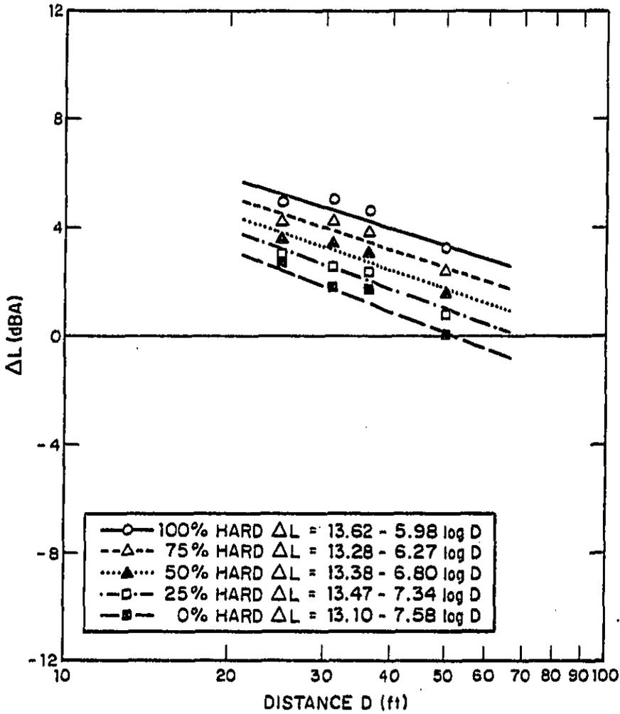
FIG. 5.2. HARD SITE/SOFT SITE NOISE LEVEL DIFFERENCES AS A FUNCTION OF MICROPHONE DISTANCE: IMI - DIESEL - LEFT SIDE.
