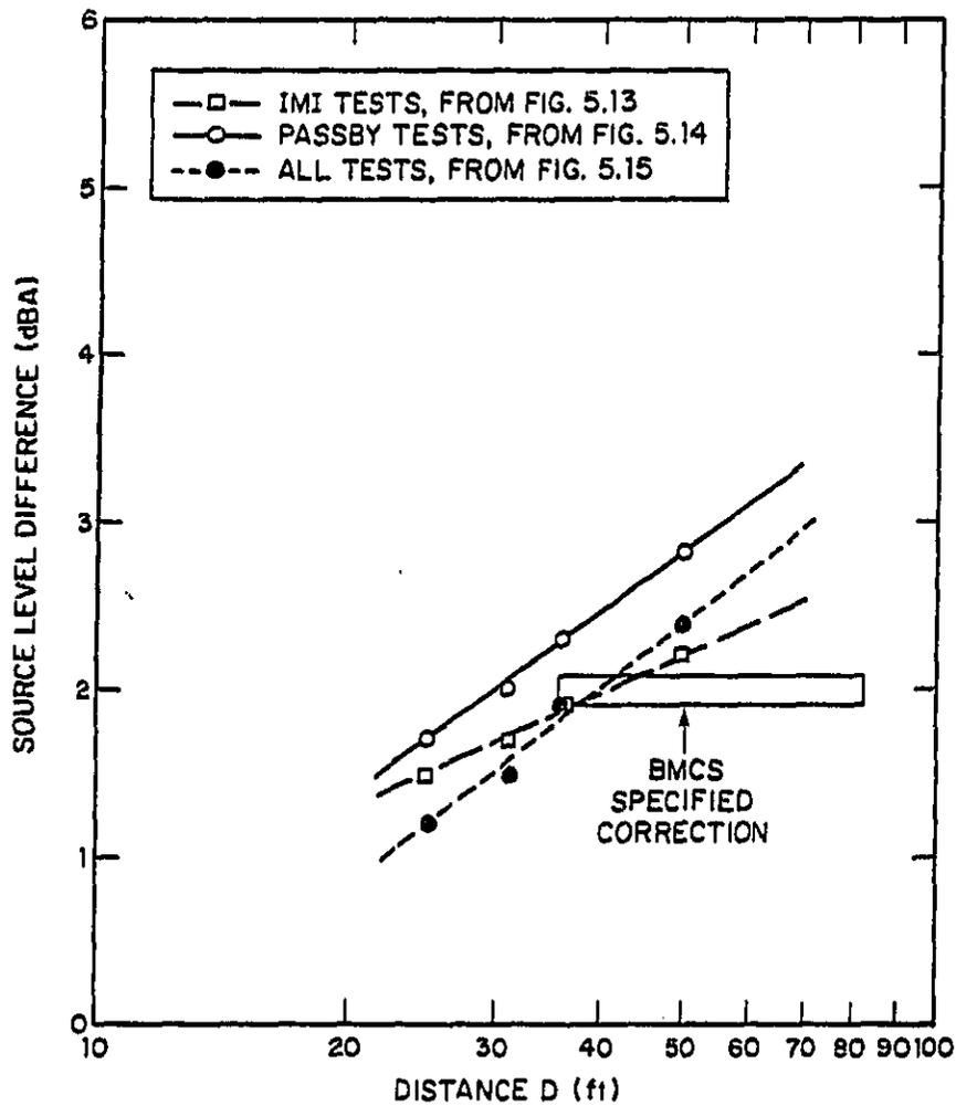
FIG. 6.2. SOUND LEVEL DIFFERENCE BETWEEN A 100% HARD SITE AND A TYPICAL "SOFT" (i.e., 32% HARD) SITE, AS A FUNCTION OF MICROPHONE DISTANCE.
