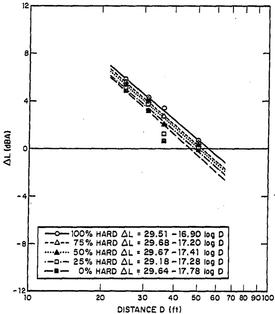
FIG. 5.7. HARD SITE/SOFT SITE NOISE LEVEL DIFFERENCES AS A FUNCTION OF MICROPHONE DISTANCE: DIESEL PASSBYS - 45 TO 55 MPH - RIGHT SIDE.
