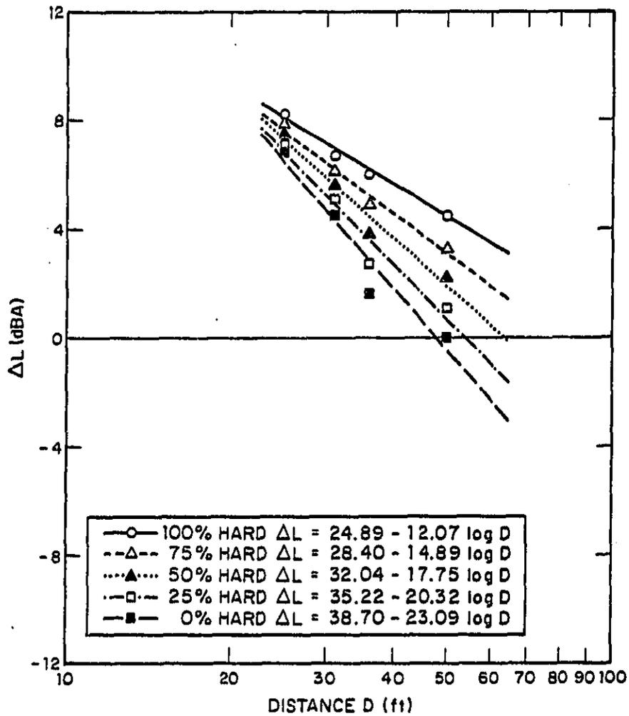
FIG. 5.12. HARD SITE/SOFT SITE NOISE LEVEL DIFFERENCES AS A FUNCTION OF MICROPHONE DISTANCE: GAS PASSBYS - 40 MPH - LEFT SIDE.
