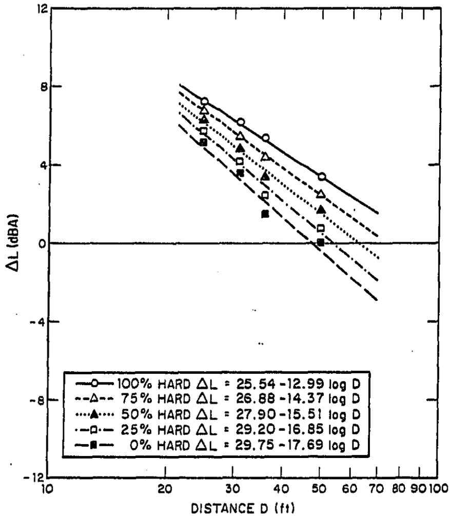
FIG. 5.15. HARD SITE/SOFT SITE NOISE LEVEL DIFFERENCES AS A FUNCTION OF MICROPHONE DISTANCE: ALL DATA.
