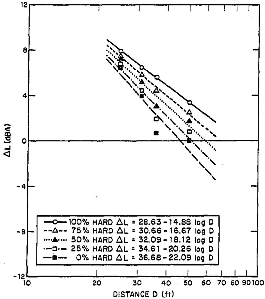
FIG. 5.9. HARD SITE/SOFT SITE NOISE LEVEL DIFFERENCES AS A FUNCTION OF MICROPHONE DISTANCE: GAS PASSBYS - 35 MPH - RIGHT SIDE.
