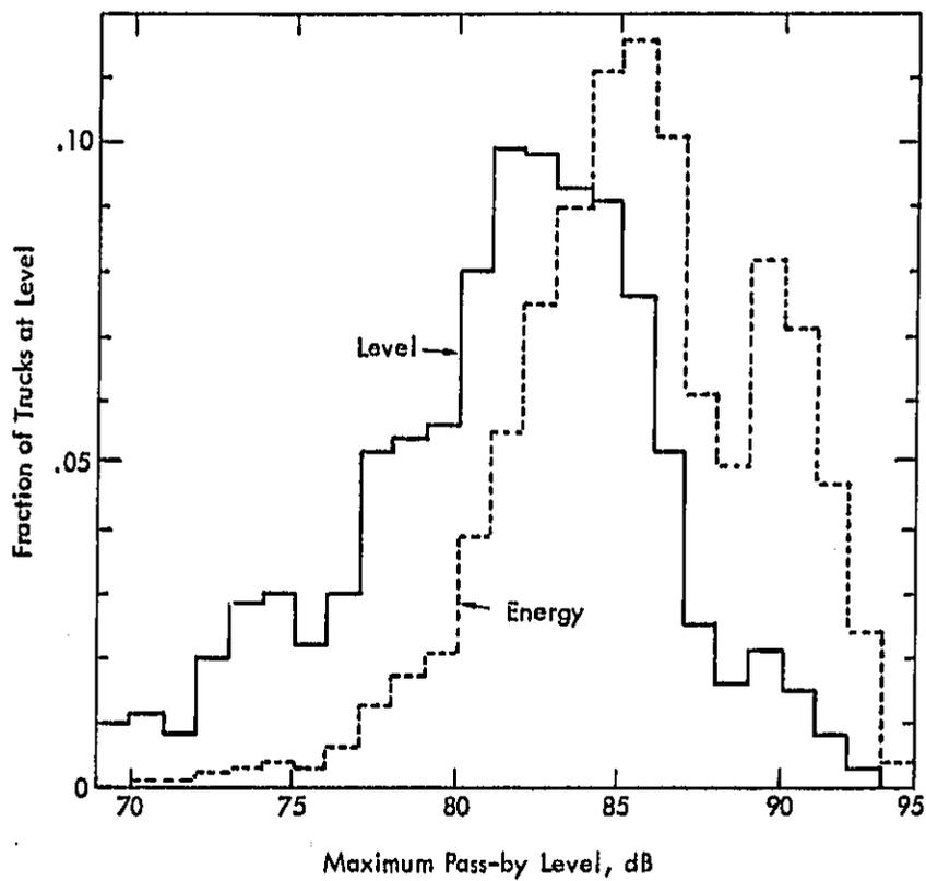
Figure 2. Noise Level and Energy Distributions of Trucks at Low Speeds (Based on the Noise Level Distribution Shown in Figure 1)
