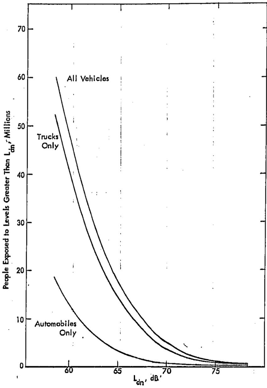
Figure 8. Noise Exposure Due to Automobiles Alone and Trucks Alone, 1970
