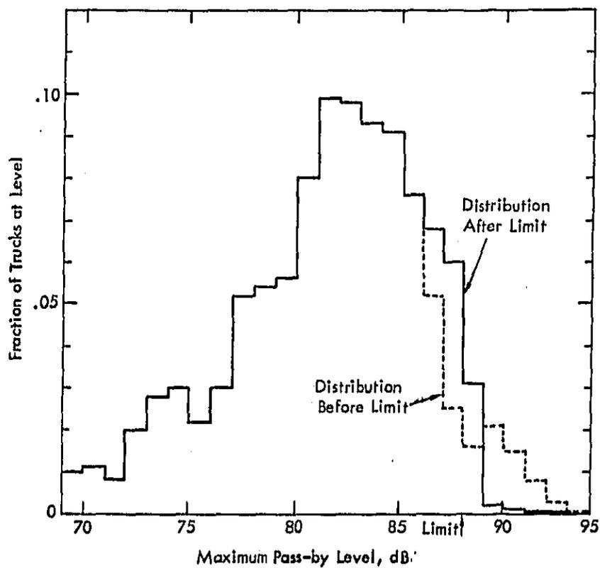
Figure 3. Effect of Operating Limit on Truck Noise Level Distribution
