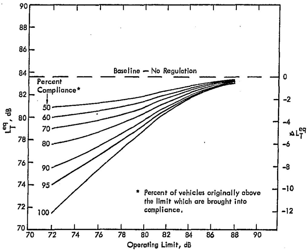
Figure 17. Effect of Operating Limit on  $L_{T}^{eq}$  at Low Speeds
