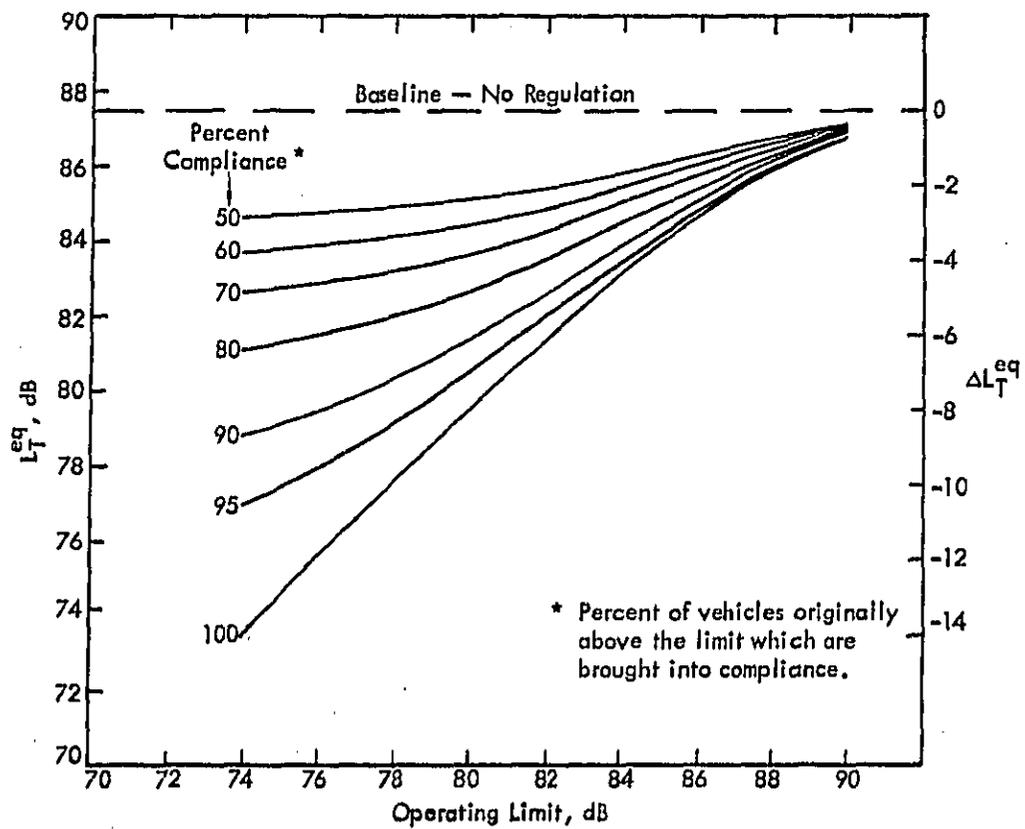
Figure 18. Effect of Operating Limit on  $L_{T}^{eq}$  at High Speeds
