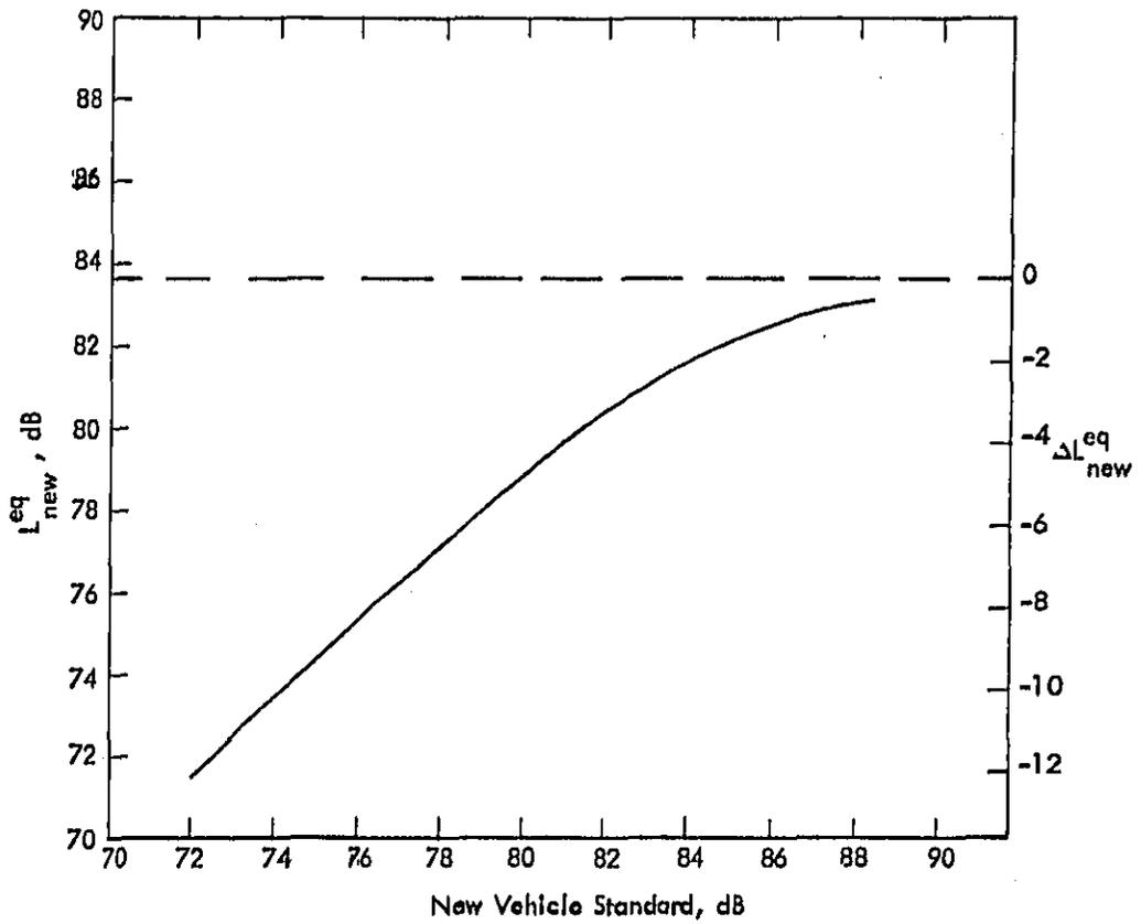
Figure 19. Effect of New Vehicle Standard on  $L_{eq}$  of New Trucks at Low Speeds
