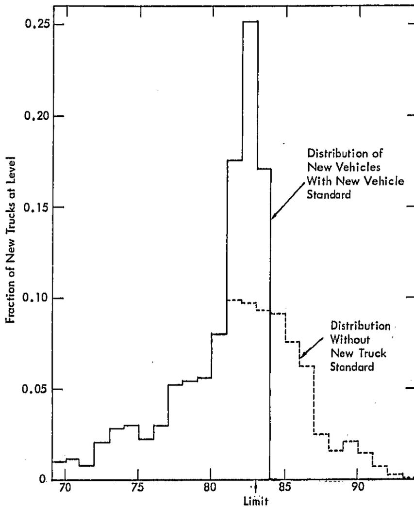
Figure 4. Effect of New Vehicle Standard on Distribution of New Truck Noise Levels at Low Speeds.
