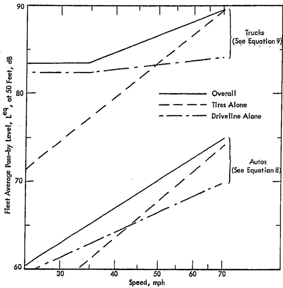
Figure 6. Automobile and Truck Noise Levels, and Decomposition Into Driveline and Tire Components
