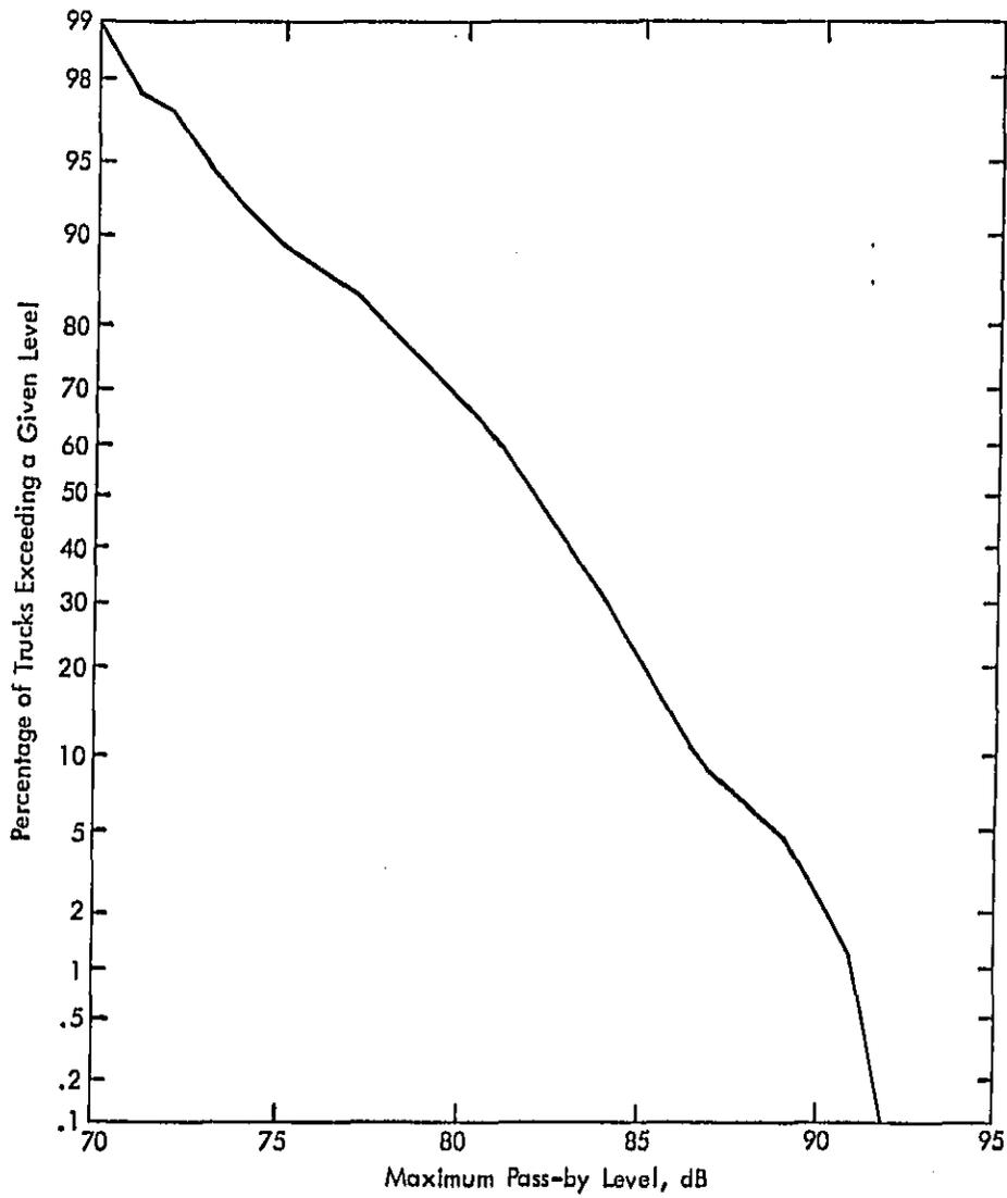
Figure 1. Noise Level Distribution of Trucks in Speed Zones Less Than 35 mph (56 kmh), Based on Data in Reference 4.
