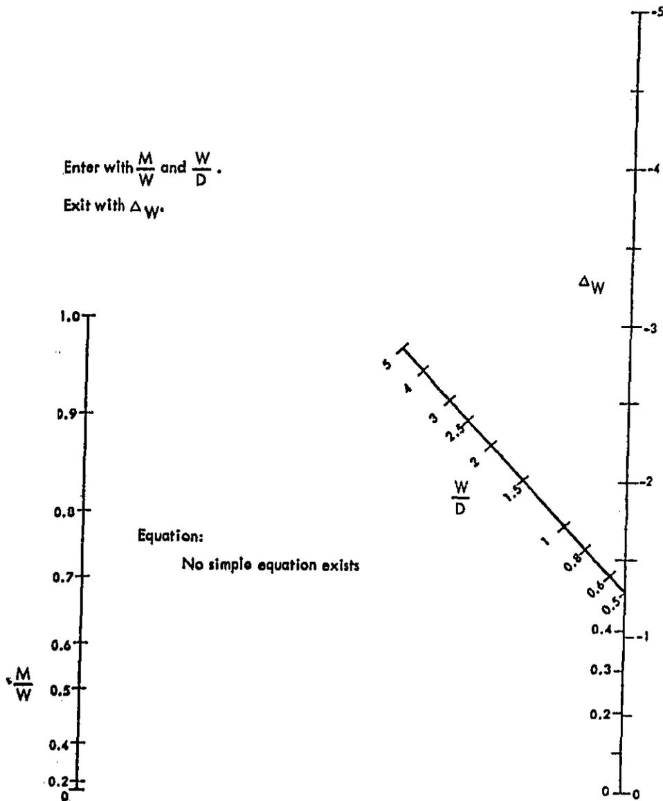
Nomogram A4. Calculation of Correction Factor  $\Delta_W$  for Road Geometry.
