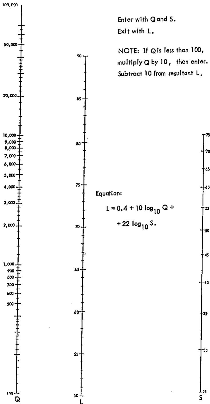
Nomogram A1. Calculation of Base Noise Level, L.
