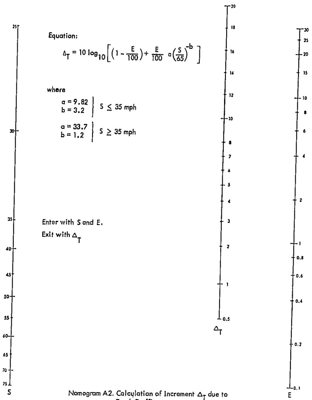
Nomogram A2. Calculation of Increment  $\Delta_T$  due to Truck Traffic.
