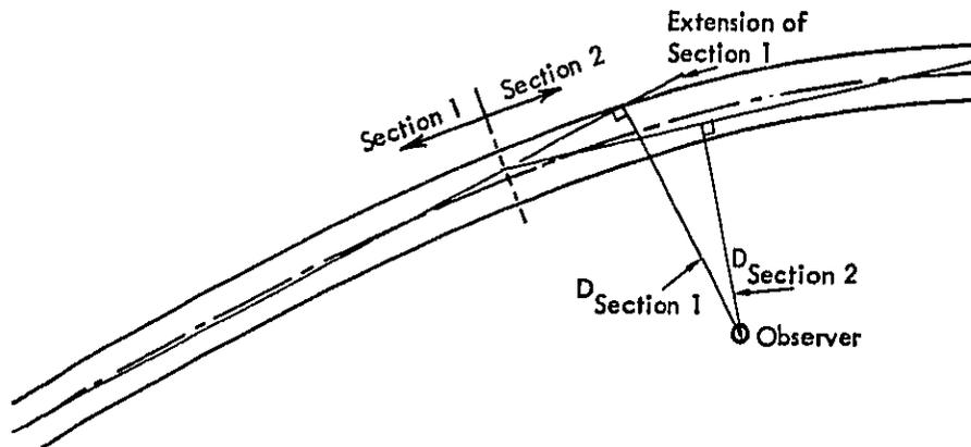
Figure A-3. Curved Roadway Approximated by Two Straight Sections
