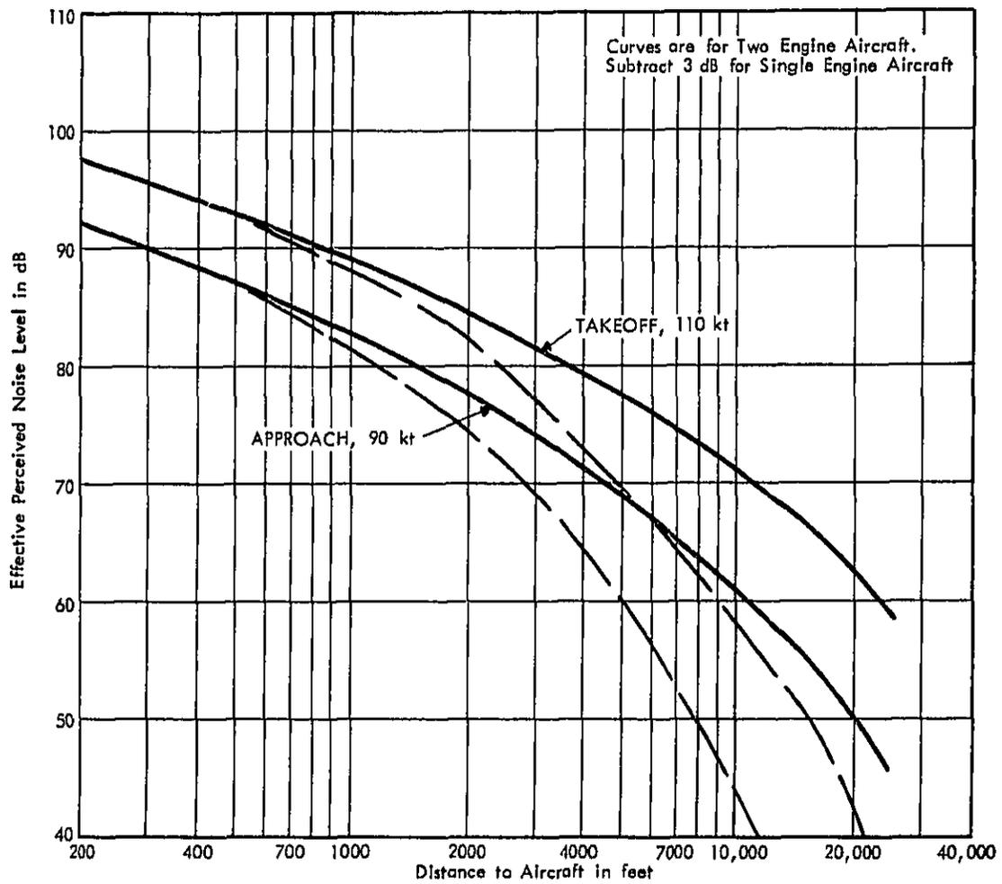
FIGURE A-19 VARIATION IN EFFECTIVE PERCEIVED NOISE LEVELS WITH DISTANCE - ONE AND TWO PISTON ENGINE PROPELLER AIRCRAFT (LESS THAN 12,500 LBS MAX. GROSS WEIGHT)
