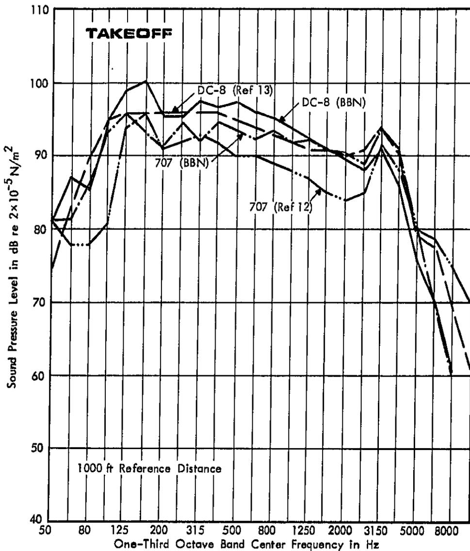
FIGURE 5. NOISE SPECTRA FOR DEVELOPMENT OF EPNL VS DISTANCE CURVES - DC-8 AND 707 TAKEOFFS
