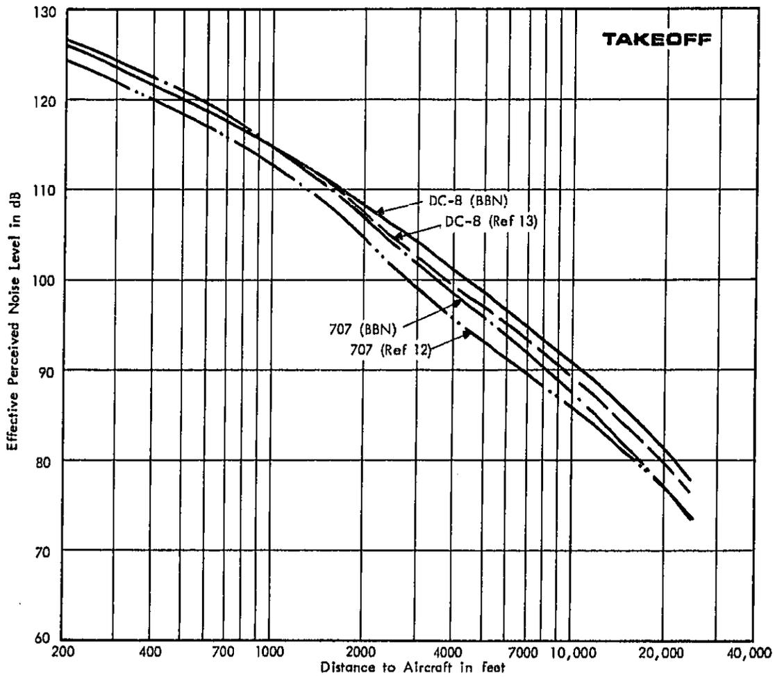
FIGURE 3. COMPARISON OF EPNL VS DISTANCE CURVES BASED ON NOISE SPECTRA FROM DIFFERENT SOURCES - DC-8 AND 707 TAKEOFFS
