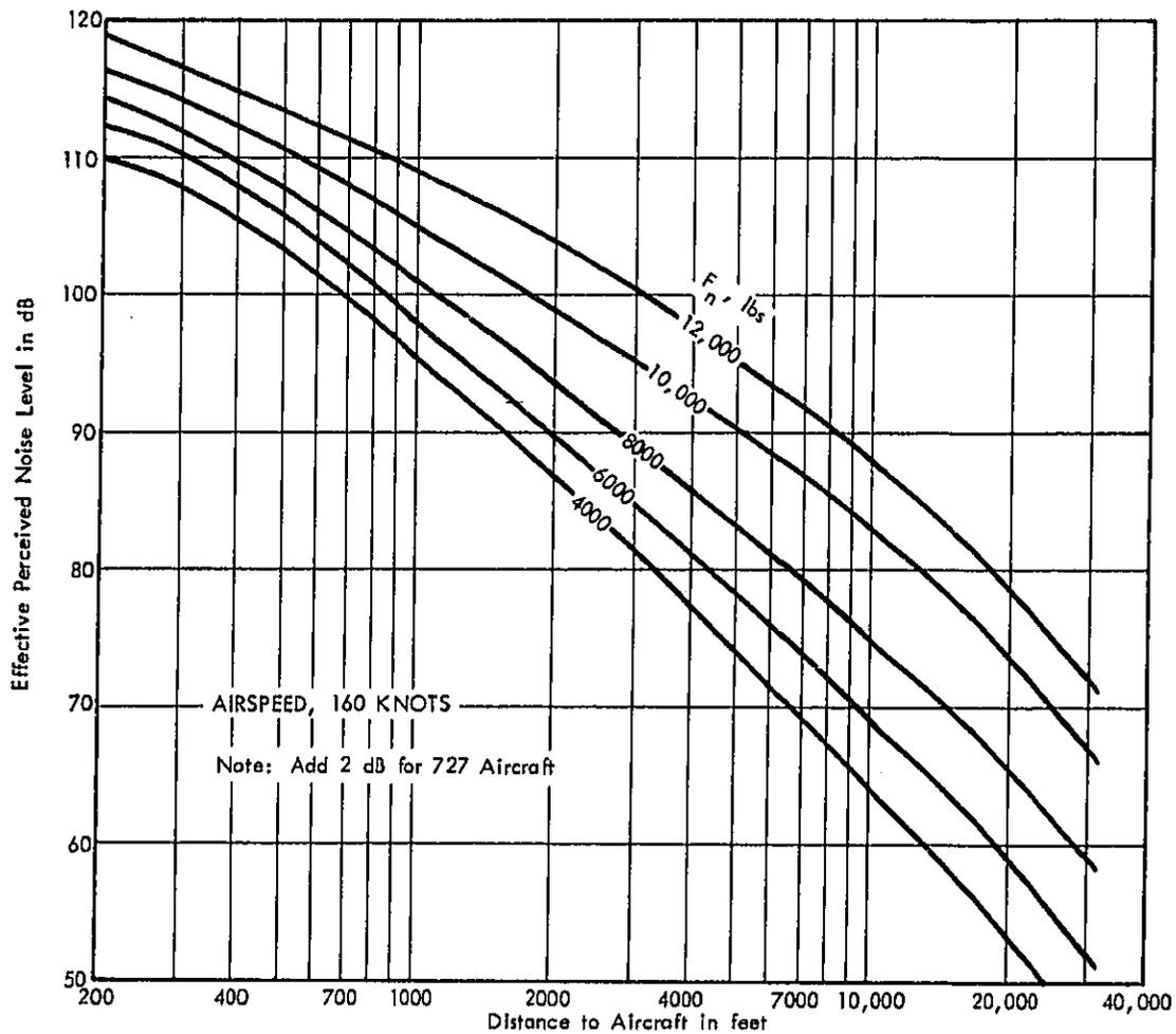
FIGURE A-3 VARIATION IN EFFECTIVE PERCEIVED NOISE LEVELS WITH DISTANCE - TWO AND THREE ENGINE LBPR TURBOFAN TRANSPORT AIRCRAFT - 737, DC-9 AND 727 AIRCRAFT WITH JT8D SERIES ENGINES
