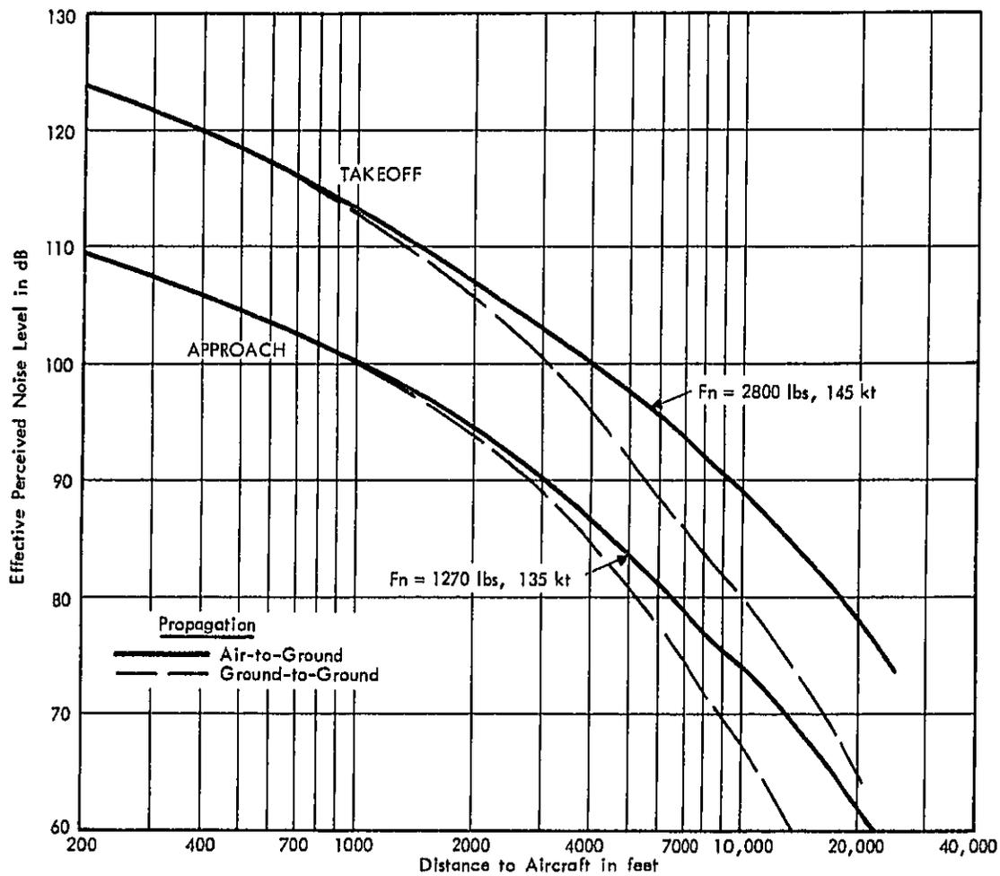
FIGURE A-12 VARIATION IN EFFECTIVE PERCEIVED NOISE LEVELS WITH DISTANCE - BUSINESS JET AIRCRAFT - LOCKHEED JETSTAR 1/C-140 WITH FOUR PT 12A-6A TURBOJET ENGINES
