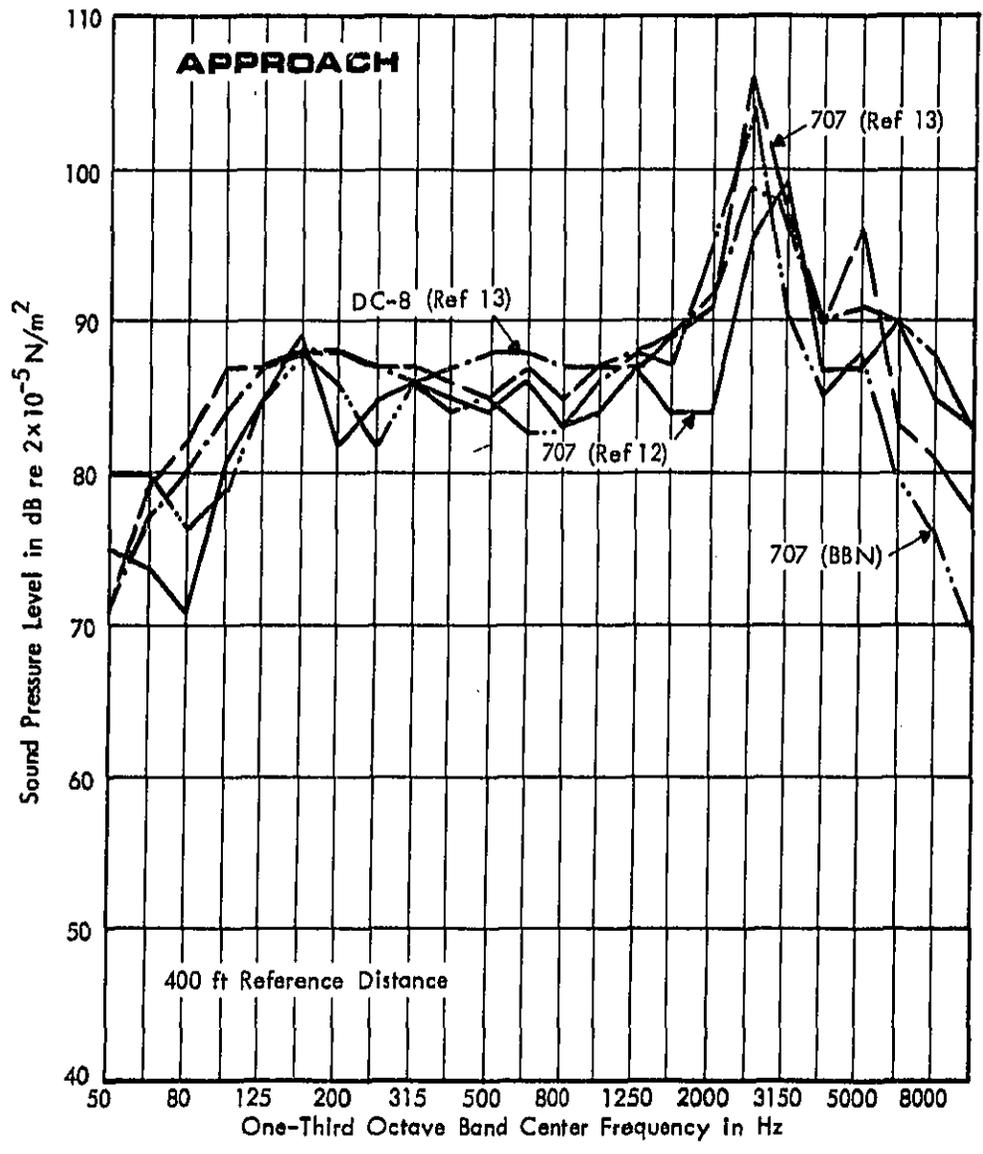
FIGURE 6. NOISE SPECTRA FOR DEVELOPMENT OF EPNL VS DISTANCE CURVES - DC-8 AND 707 APPROACH
