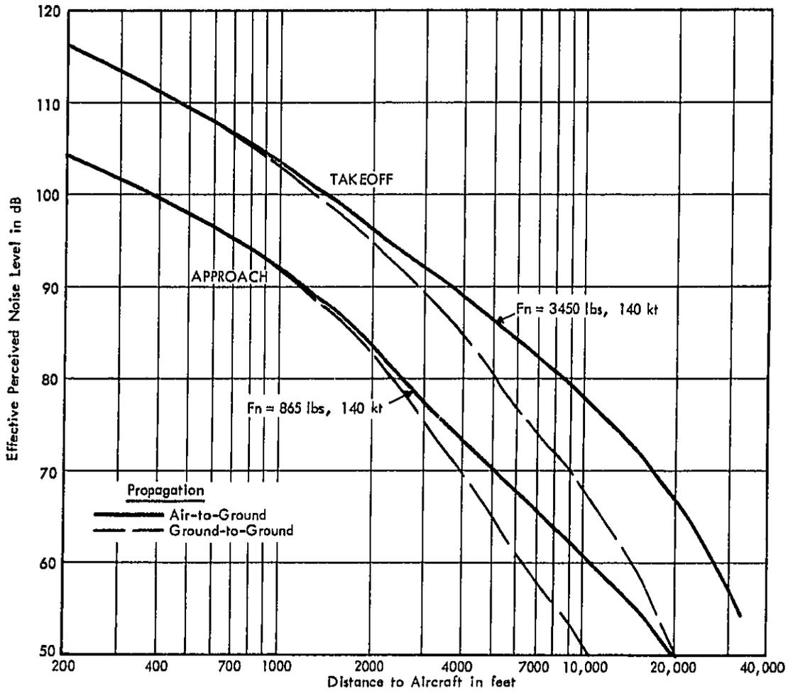
FIGURE A-14 VARIATION IN EFFECTIVE PERCEIVED NOISE LEVELS WITH DISTANCE - BUSINESS JET AIRCRAFT - NORTH AMERICAN SABRE 80 WITH TWO CJ 700-2D-2 TURBOFAN ENGINES
