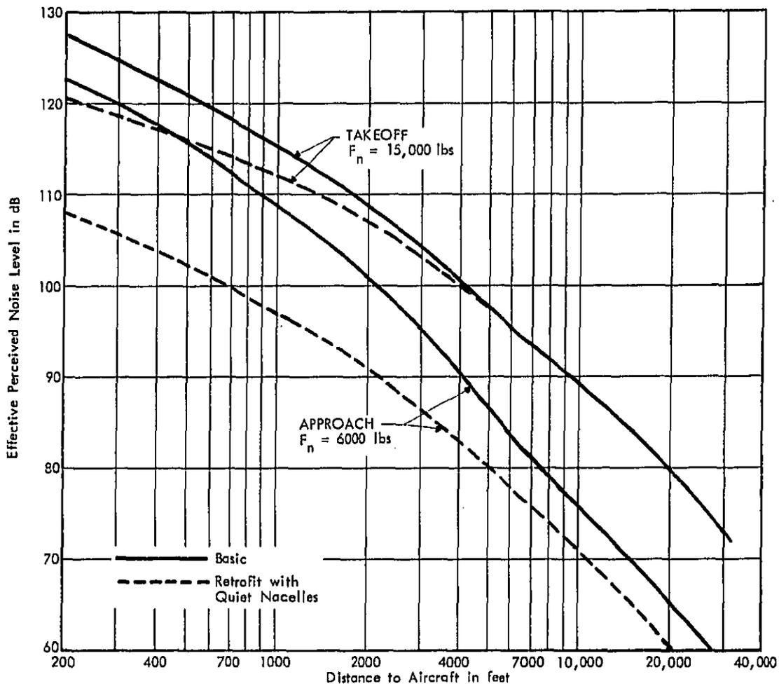
FIGURE 11. COMPARISON OF TYPICAL TAKEOFF AND APPROACH NOISE FOR 707 AND DC-8 AIRCRAFT WITH AND WITHOUT QUIET NACELLE RETROFIT
