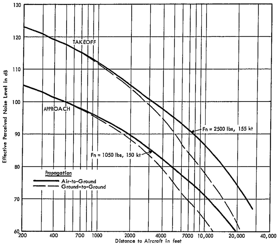
FIGURE A-10 VARIATION IN EFFECTIVE PERCEIVED NOISE - BUSINESS JET AIRCRAFT - GATES LEARJET 24 AND 25 WITH TWO CJ610-6 TURBOJET ENGINES
