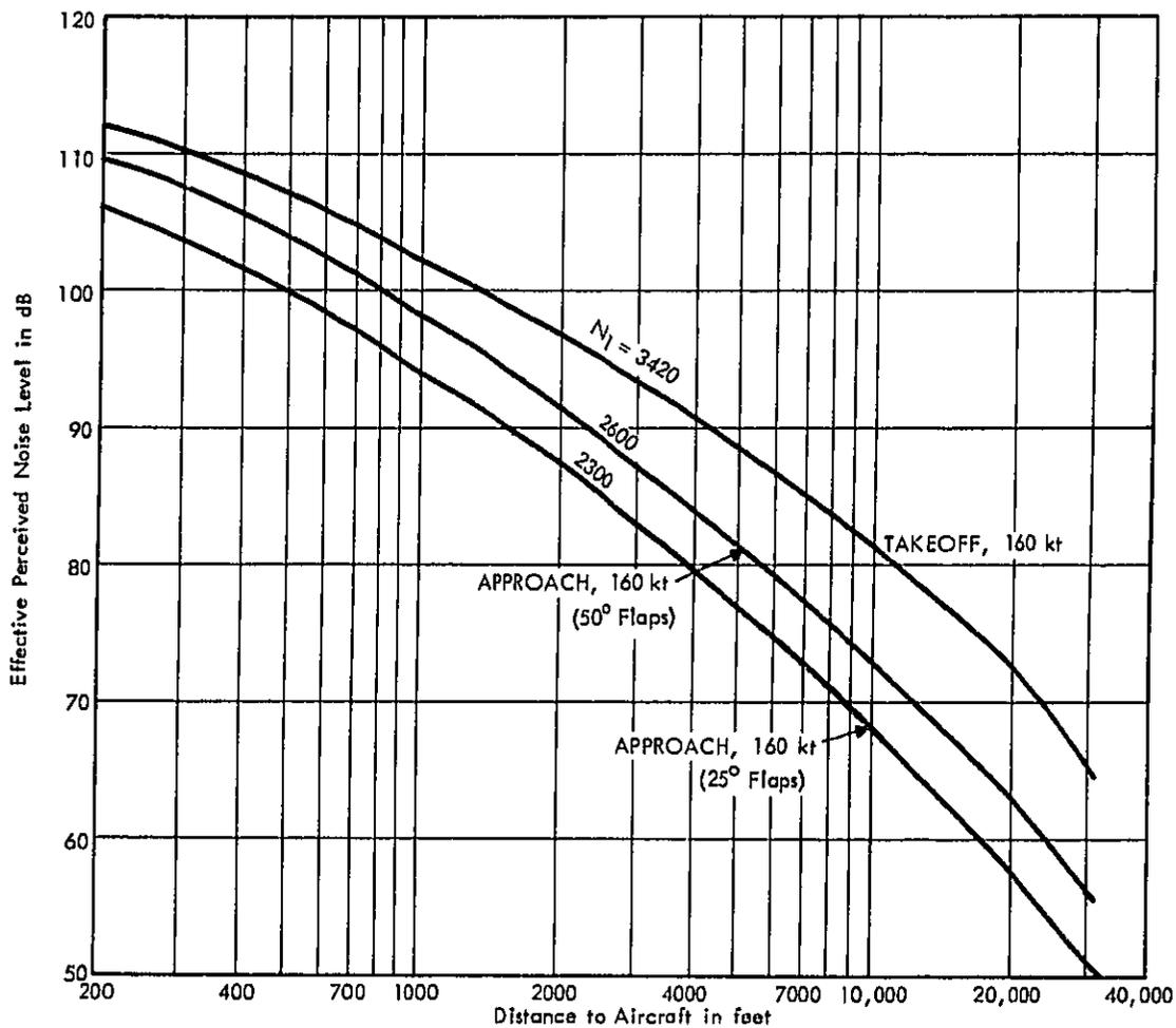
FIGURE A-5 VARIATION IN EFFECTIVE PERCEIVED NOISE LEVELS WITH DISTANCE - THREE ENGINE HBPR TURBOFAN TRANSPORT AIRCRAFT - DC-10 AIRCRAFT WITH CF-6 SERIES ENGINES
