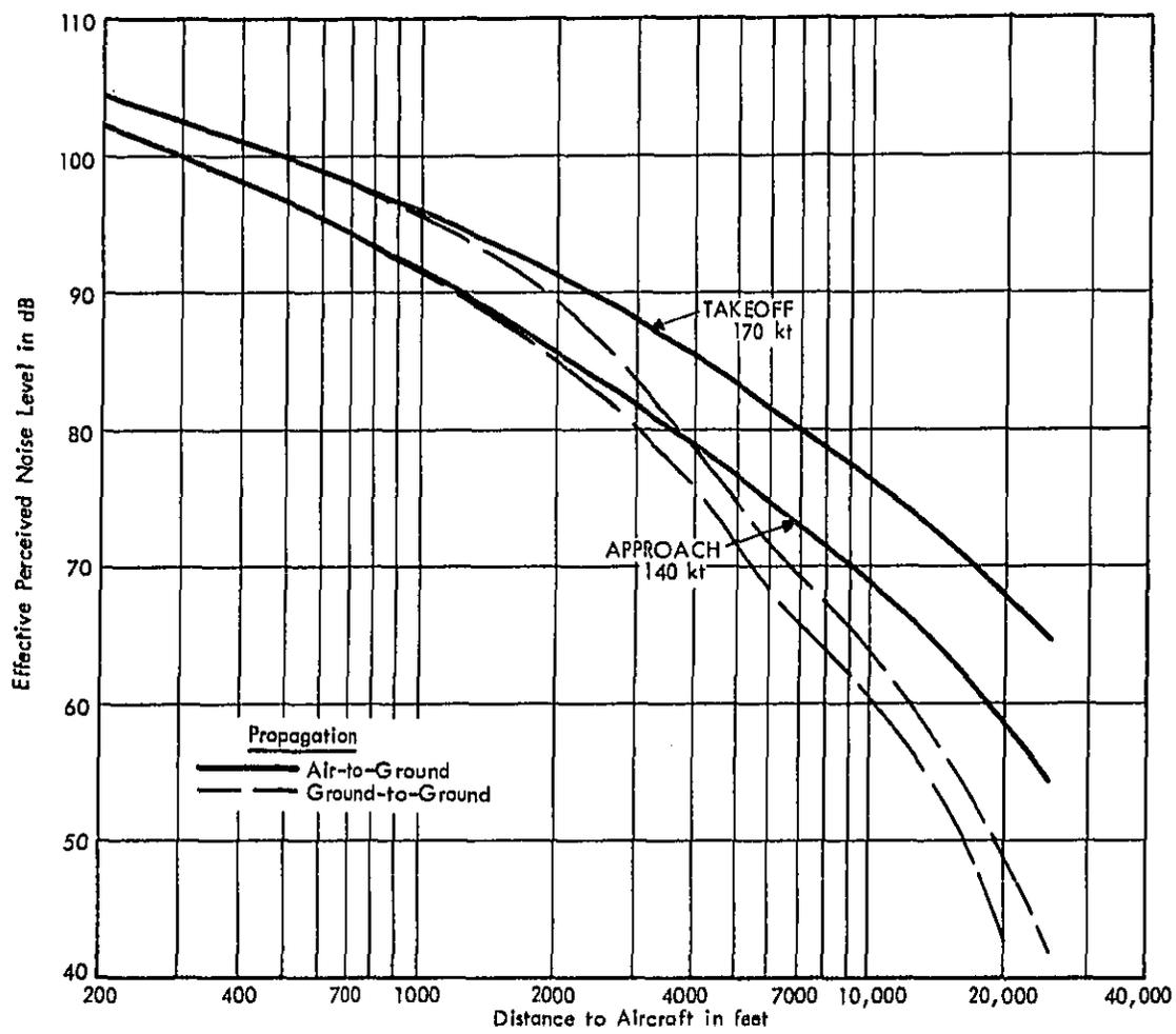
FIGURE A-15 VARIATION IN EFFECTIVE PERCEIVED NOISE LEVELS WITH DISTANCE - FOUR ENGINE TURBOPROP TRANSPORT AIRCRAFT - LOCKHEED ELECTRA, C 130 HERCULES
