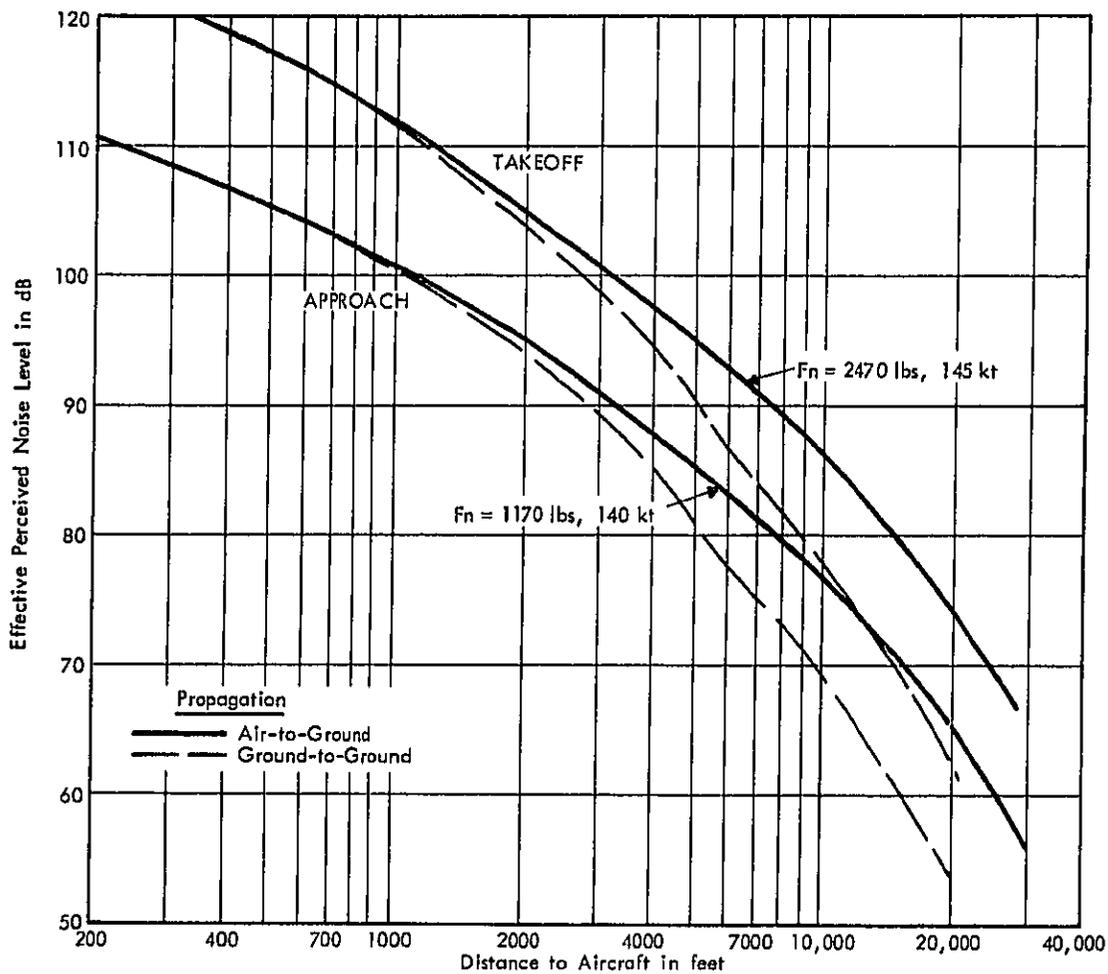
FIGURE A-8 VARIATION IN EFFECTIVE PERCEIVED NOISE LEVELS WITH DISTANCE - BUSINESS JET AIRCRAFT - COMMODORE JET COMMANDER 1121 WITH TWO CJ610-5 TURBOJET ENGINES
