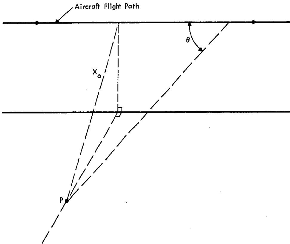
FIGURE 1. SIMPLIFIED LEVEL FLIGHT GEOMETRY FOR CALCULATING EPNL VALUES AT VARYING DISTANCES
