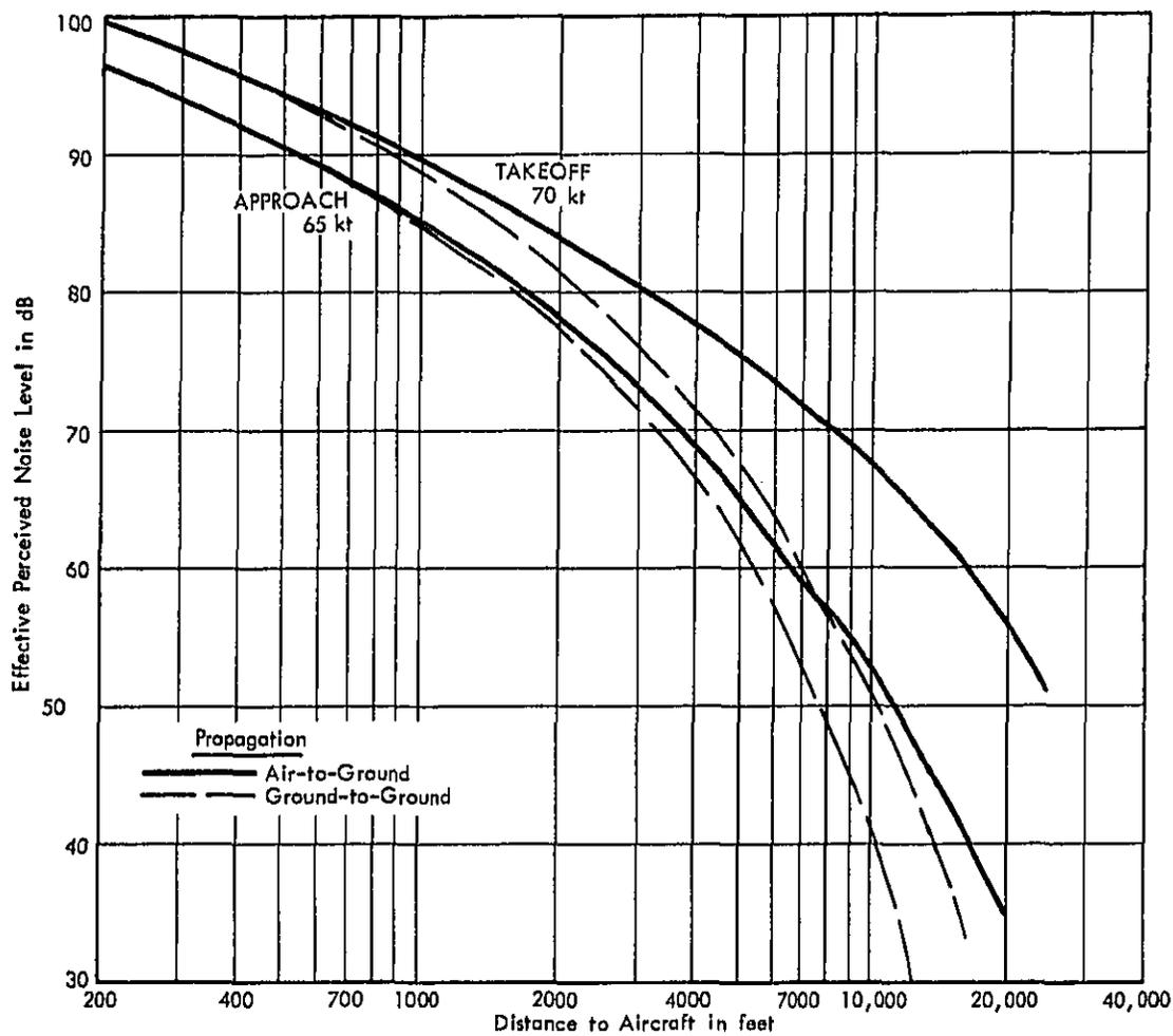
FIGURE A-17 VARIATION IN EFFECTIVE PERCEIVED NOISE LEVELS WITH DISTANCE - TWO ENGINE TURBOPROP AIRCRAFT - DCH-6 TWIN OTTER
