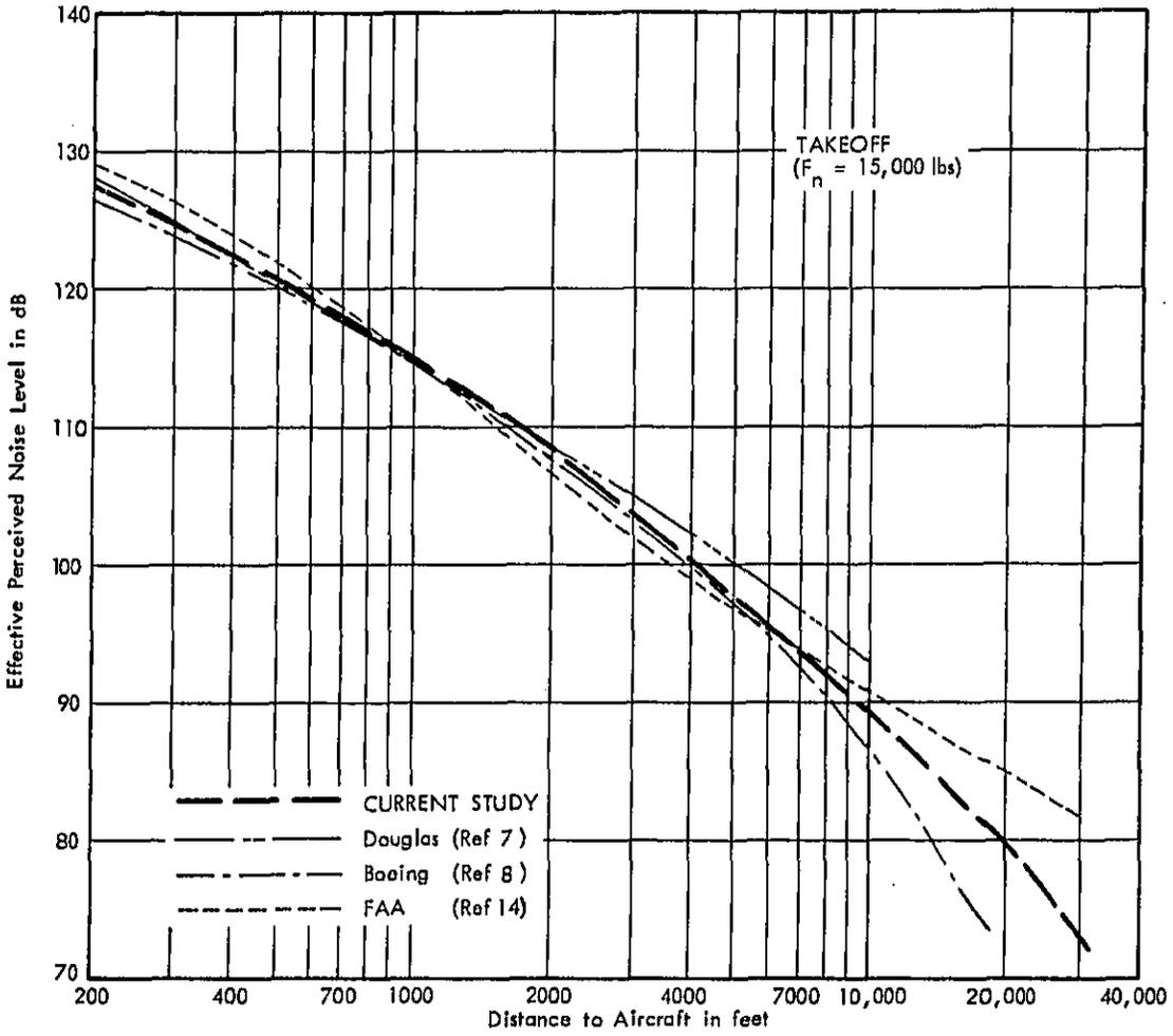
FIGURE 7. COMPARISON OF EPNL VERSUS DISTANCE CURVES FROM DIFFERENT SOURCES - 707 AND DC-8 AIRCRAFT WITH JT3D SERIES ENGINES - TAKEOFF
