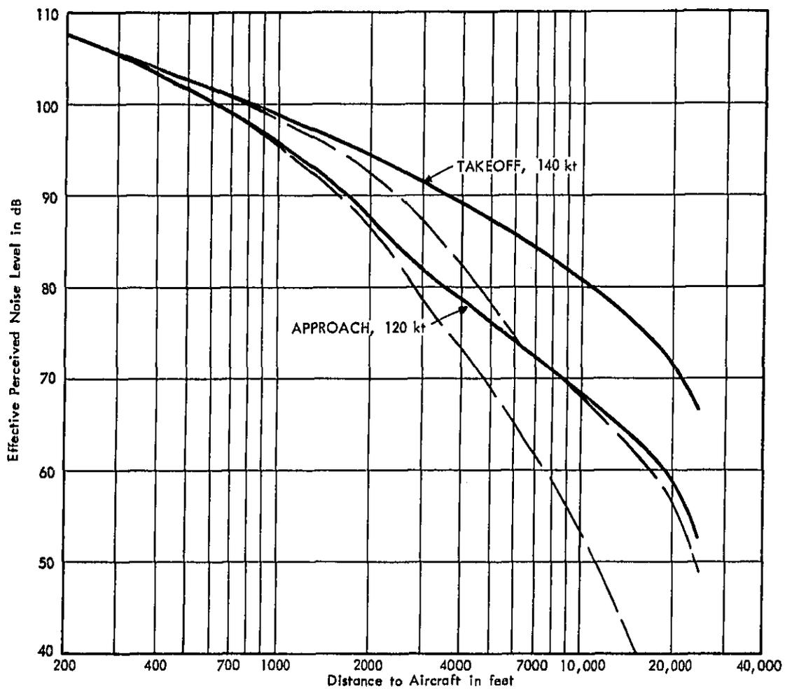
FIGURE A-16 VARIATION IN EFFECTIVE PERCEIVED NOISE LEVELS WITH DISTANCE - TWO ENGINE TURBOPROP AIRCRAFT WITH DART ENGINES (F27, HS 748)
