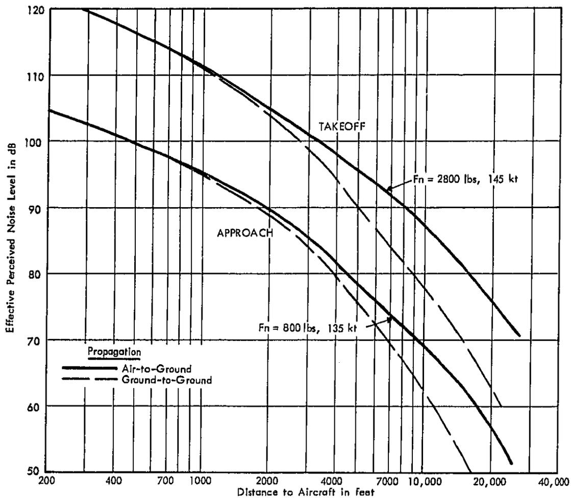
FIGURE A-13 VARIATION IN EFFECTIVE PERCEIVED NOISE LEVELS WITH DISTANCE - BUSINESS JET AIRCRAFT - NORTH AMERICAN SABRE 60 WITH TWO PT12A-B TURBOJET ENGINES
