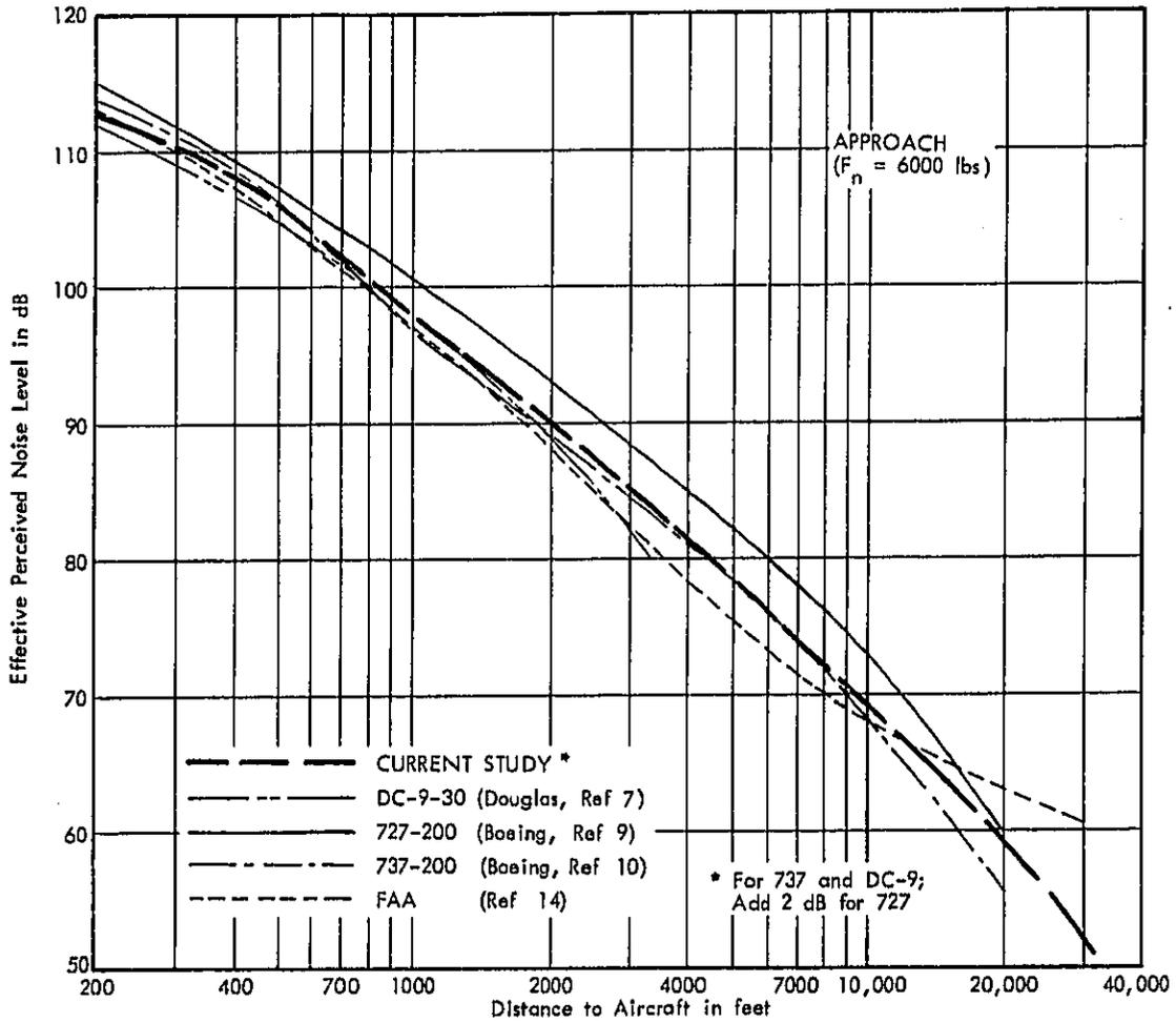
FIGURE 10. COMPARISON OF EPNL VERSUS DISTANCE CURVES FROM DIFFERENT SOURCES - 737, DC-9 AND 727 AIRCRAFT WITH JT8D SERIES ENGINES - APPROACH
