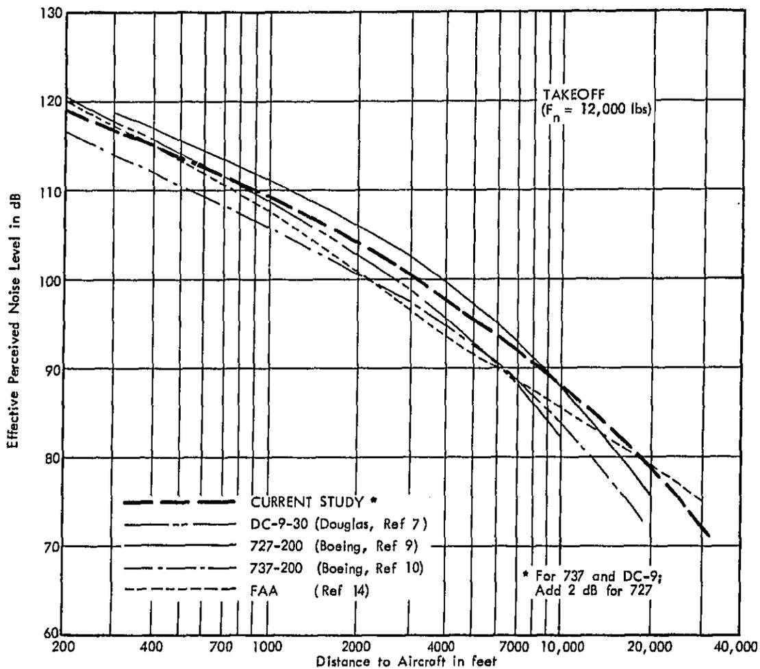
FIGURE 9. COMPARISON OF EPNL VERSUS DISTANCE CURVES FROM DIFFERENT SOURCES - 737, DC-9 AND 727 AIRCRAFT WITH JT8D SERIES ENGINES - TAKEOFF
