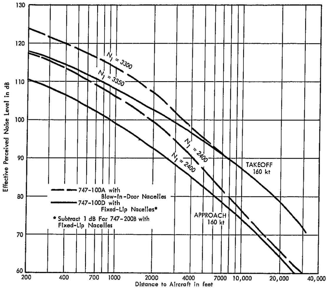
FIGURE A-4 VARIATION IN EFFECTIVE PERCEIVED NOISE LEVELS WITH DISTANCE - FOUR ENGINE HBPR TURBOFAN TRANSPORT AIRCRAFT - 747 AIRCRAFT WITH JT9D SERIES ENGINES
