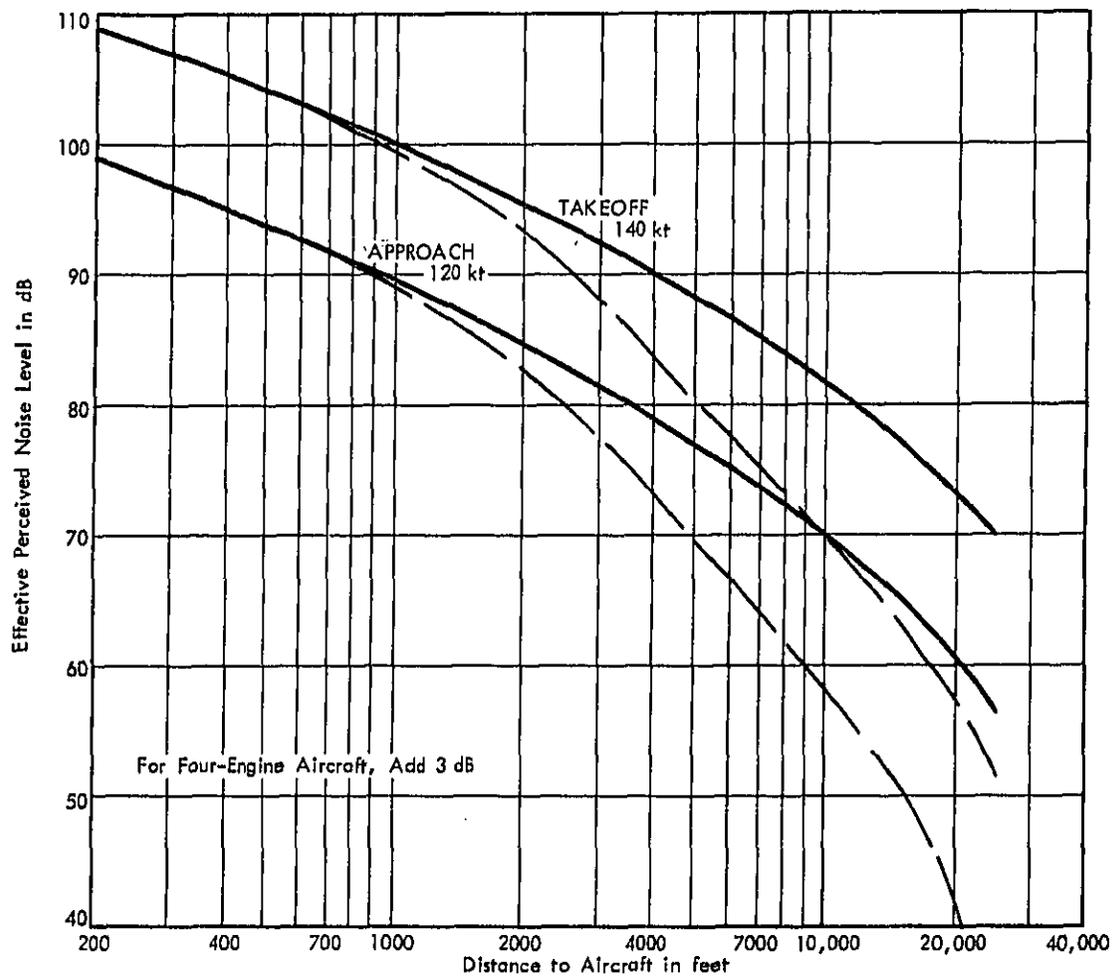
FIGURE A-18 VARIATION IN EFFECTIVE PERCEIVED NOISE LEVELS WITH DISTANCE - TWO ENGINE PISTON TRANSPORT AIRCRAFT (MORE THAN 12,000 LBS MAX GROSS WEIGHT)
