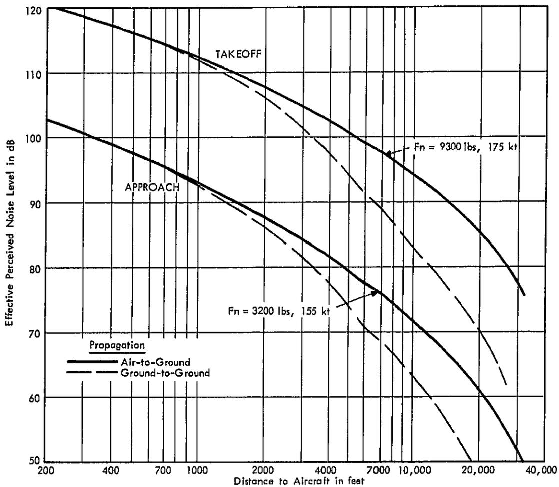
FIGURE A-11 VARIATION IN EFFECTIVE PERCEIVED NOISE LEVELS WITH DISTANCE - BUSINESS JET AIRCRAFT - GRUMMAN GULFSTREAM II WITH TWO SPEY 511-B TURBOJET ENGINES
