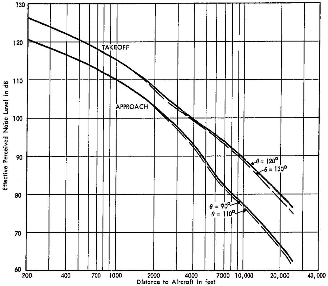
FIGURE 2. COMPARISON OF EPNL VS DISTANCE CURVES FOR DIFFERENT ASSUMED ANGLES OF PNLTM NOISE RADIATION - DC-8 AIRCRAFT NOISE DATA
