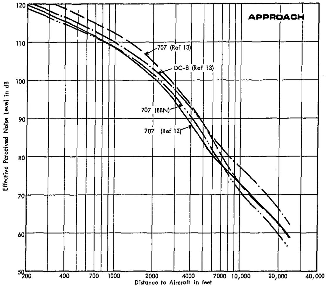
FIGURE 4. COMPARISON OF EPNL VS DISTANCE CURVES BASED ON NOISE SPECTRA FROM DIFFERENT SOURCES - DC-8 AND 707 APPROACHS
