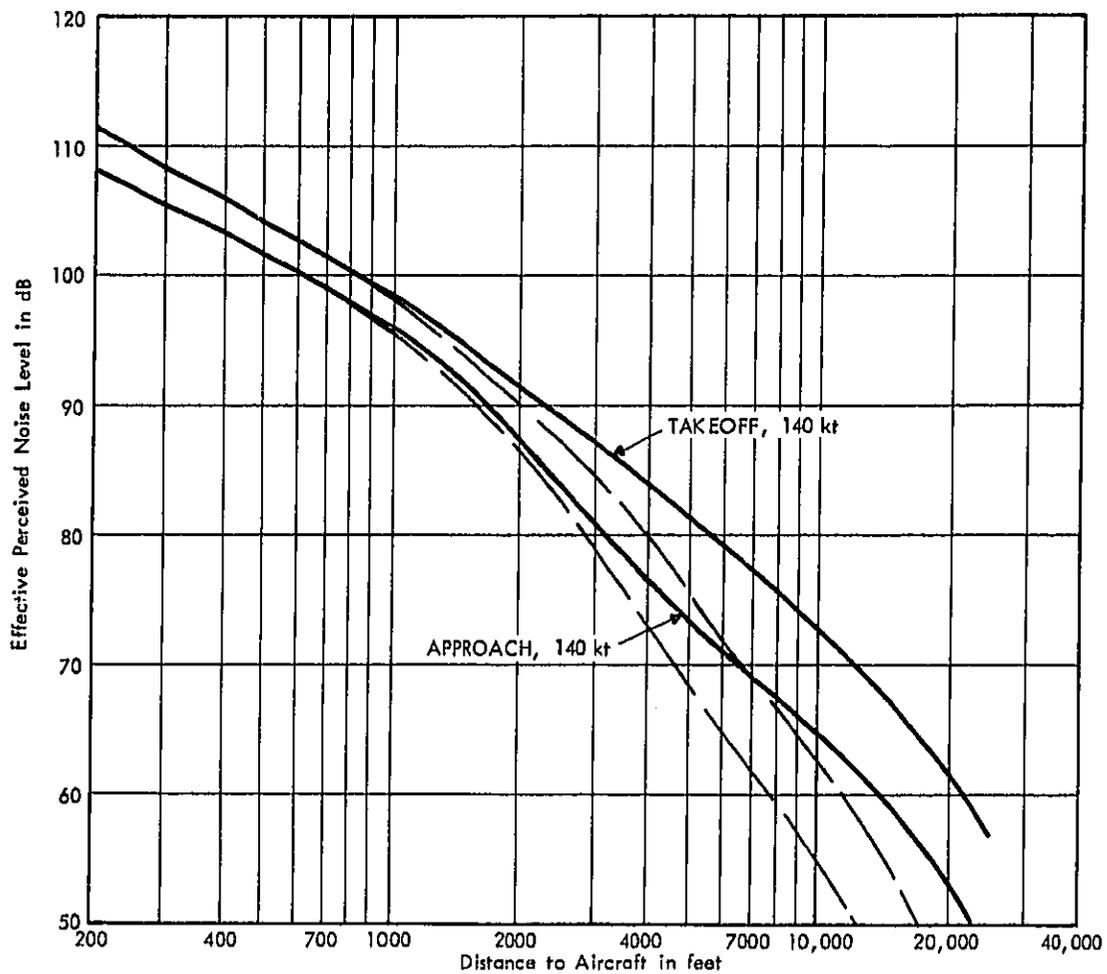
FIGURE A-9 VARIATION IN EFFECTIVE PERCEIVED NOISE LEVELS WITH DISTANCE - DASSAULT FANJET FALCON WITH TWO CJ700-2B TURBOFAN ENGINES
