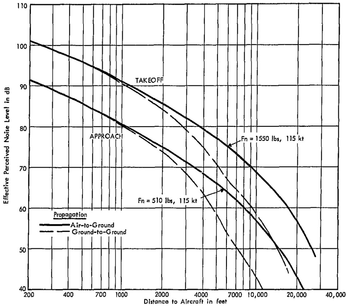
FIGURE A-7 VARIATION IN EFFECTIVE PERCEIVED NOISE LEVELS WITH DISTANCE - BUSINESS JET AIRCRAFT - CESSNA CITATION WITH TWO JT15D-1 TURBOFAN ENGINES
