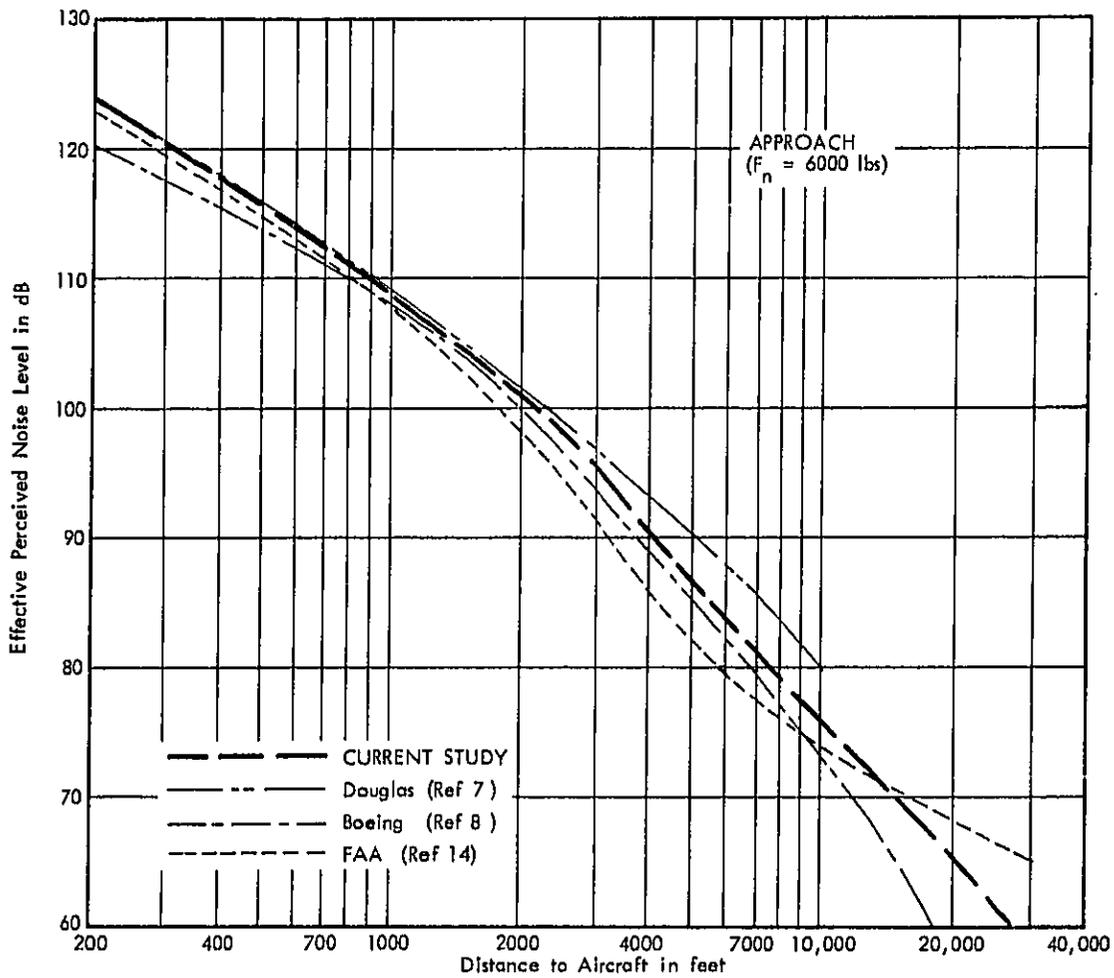
FIGURE 8. COMPARISON OF EPNL VERSUS DISTANCE CURVES FROM DIFFERENT SOURCES - 707 AND DC-8 AIRCRAFT WITH JT3D SERIES ENGINES- APPROACH
