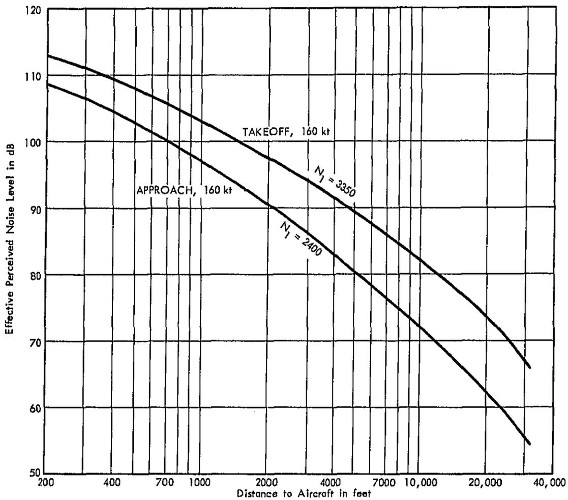
FIGURE A-6 VARIATION IN EFFECTIVE PERCEIVED NOISE LEVELS WITH DISTANCE - THREE ENGINE HBPR TURBOFAN TRANSPORT AIRCRAFT - DC-10 AIRCRAFT WITH JT8D SERIES ENGINES
