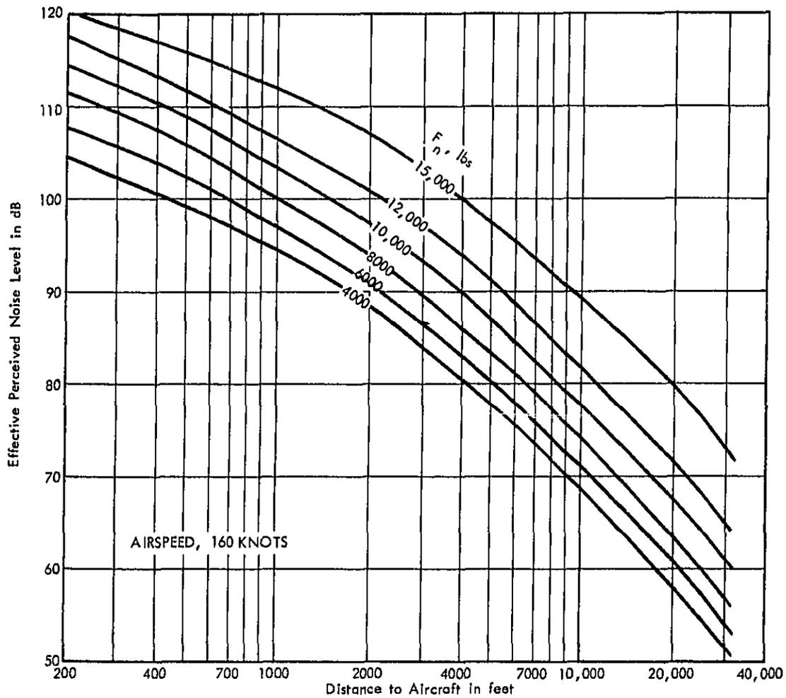
FIGURE A-2 VARIATION IN EFFECTIVE PERCEIVED NOISE LEVELS WITH DISTANCE - FOUR ENGINE LBPR TURBOFAN TRANSPORT AIRCRAFT RETROFIT WITH LINED NACELLES - 707 AND DC-8 AIRCRAFT WITH JT3D SERIES ENGINES
